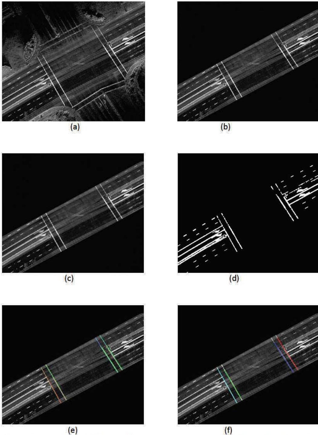
**Figure 7:** (a) is the original image; (b) is the image masked by trajectories; (c) is the smoothed image of (b); (d) is binary image of (c); (e) shows the line segments of PHT algorithm overlaid on the original image; (f) shows the final line segments after clustering.
