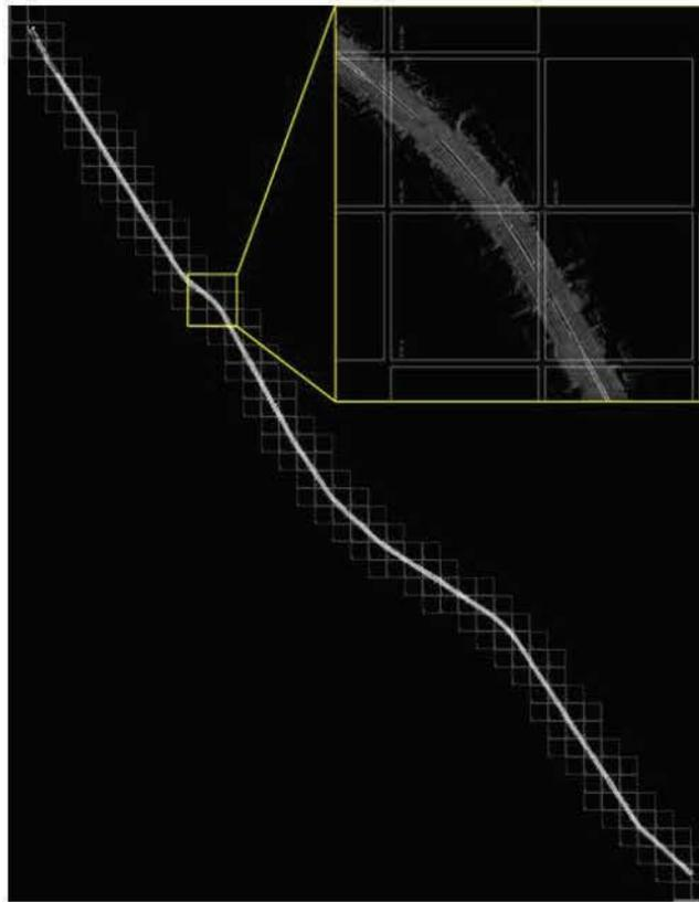
**Figure 6:** The bird's eye view intensity image of the whole trajectory is demonstrated. The north direction is pointing down, and the east direction is pointing right. Each small square represents the region of a block file.
