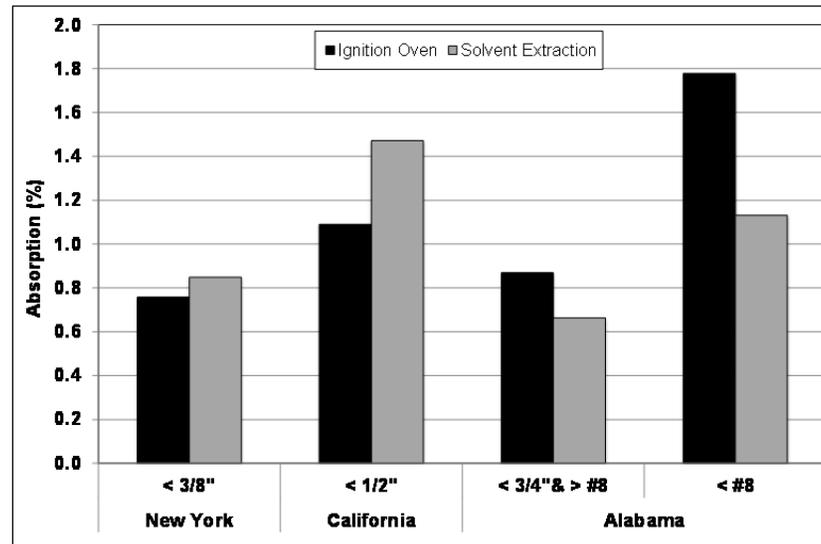
Figure 8.7: Absorption of RAP aggregate.
