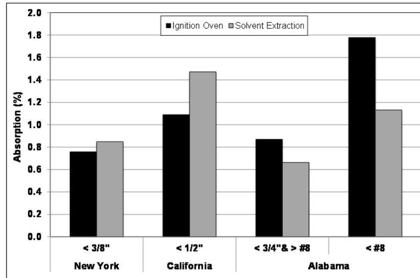
Figure 8.7: Absorption of RAP aggregate.
