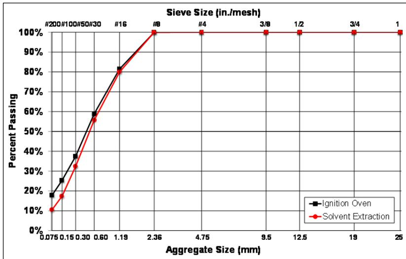
Figure 8.19: Fine aggregate gradation of California RAP.
