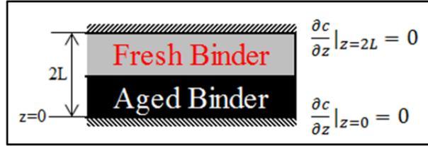
**Figure 5.6: Defined boundary conditions of diffusion specimen.**
