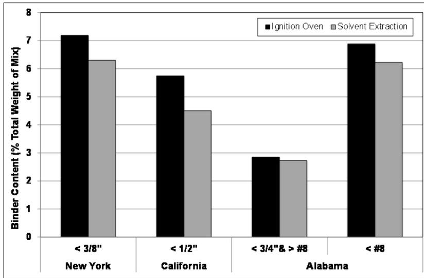
Figure 8.5: RAP asphalt binder contents.
