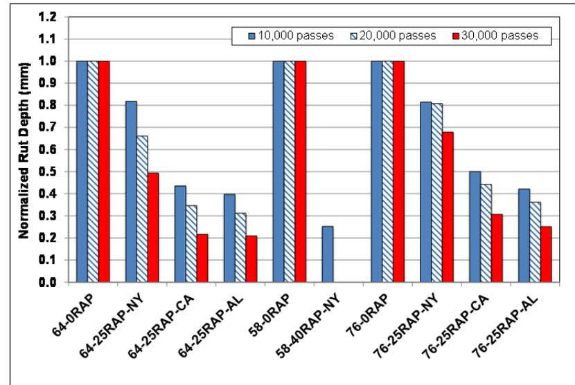
Figure 10.18: Normalized Hamburg Wheel-Track Test rut depth.
