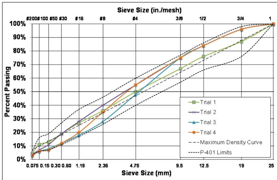
Figure 8.8: Gradation curves for trial aggregate structures.
