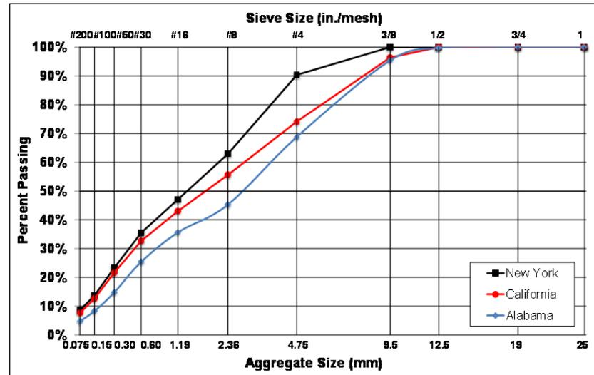
Figure 8.4: Comparison of RAP aggregate gradations by solvent extraction.
