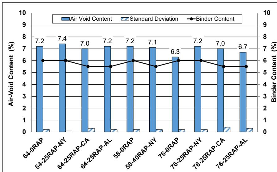
Figure 10.13: Average air-void contents of Asphalt Pavement Analyzer specimens.
