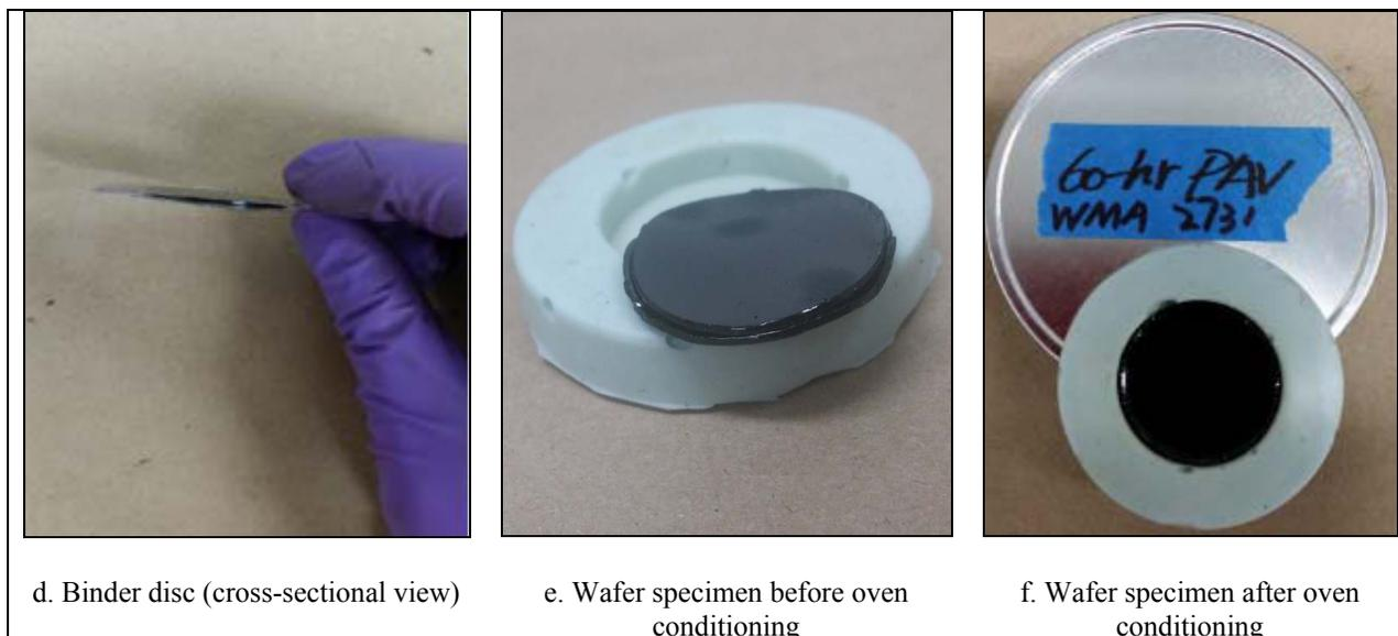
**Figure 5.1: DSR contact-blending test sample preparation procedure (*continued*).**
