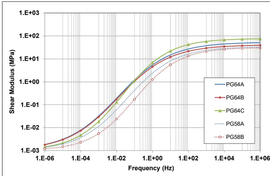
**Figure 7.6: Shear moduli of virgin asphalt binders (20°C).**
