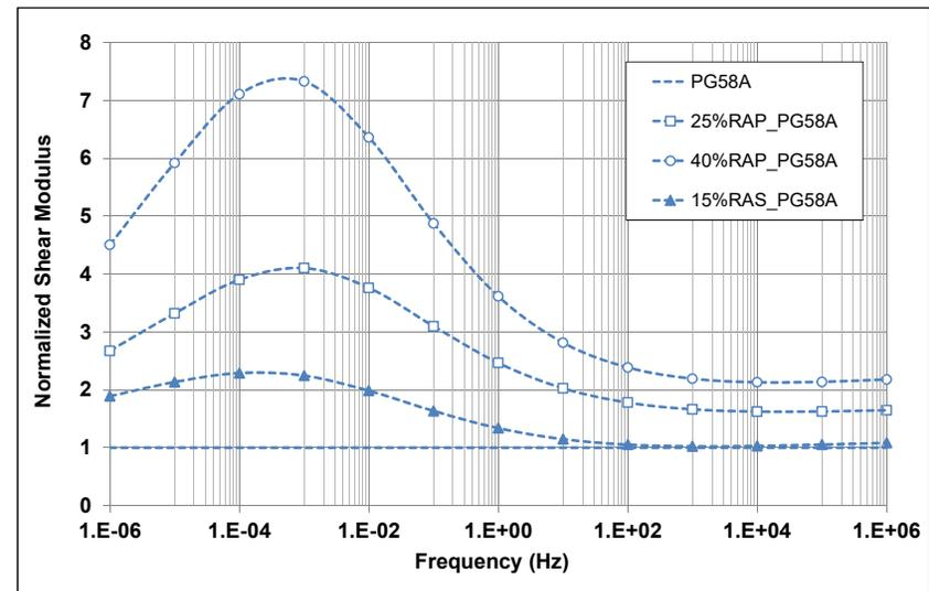
Figure 7.20: PG 58-22-A: Shear and normalized modulus master curves of FAM mixes.
