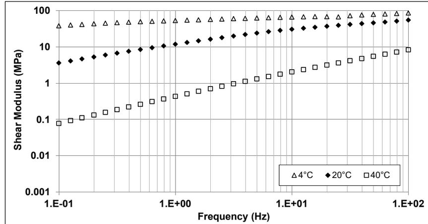
Figure 4.1: Example of measured shear modulus of an asphalt binder at 20 $^{\circ}\text{C}$ .
