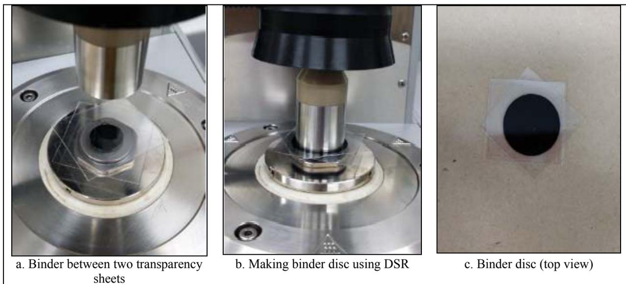
**Figure 5.1: DSR contact-blending test sample preparation procedure.**
