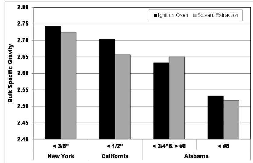
Figure 8.6: Bulk specific gravity of RAP aggregate.
