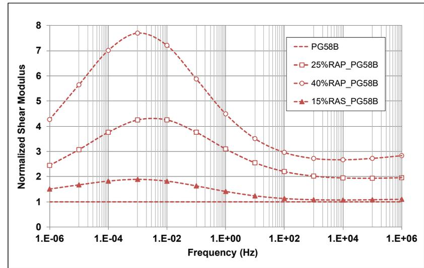
Figure 7.22: PG 58-22-B: Shear and normalized modulus master curves of FAM mixes.
