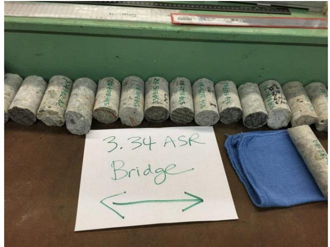
Figure 2.9: Concrete cores for visual inspection.
