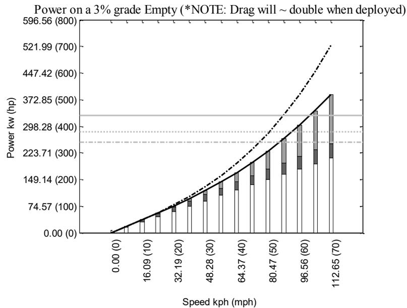
Figure 78. Power demand on for an empty TowPlow on 3% grade
