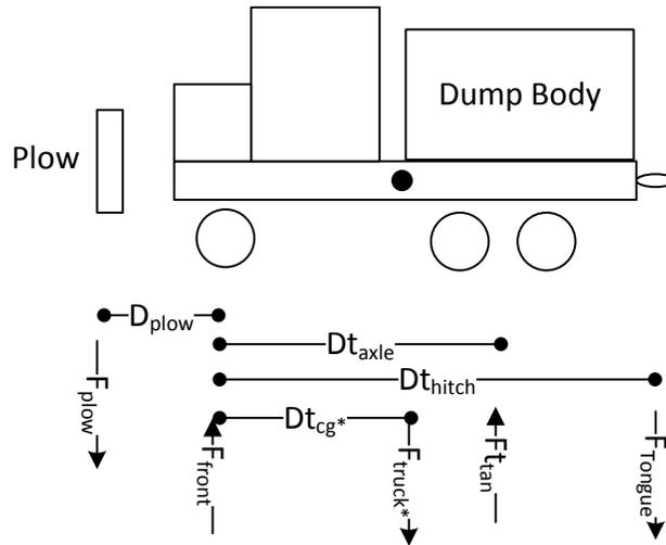
Figure 88. Prime mover truck free body diagram
