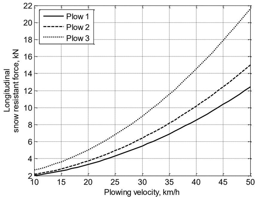
Figure 58. Longitudinal snow resistant forces of the plows
