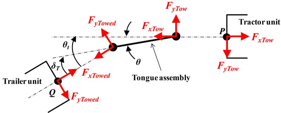
Figure 39. Scheme of the tongue assembly and forces
