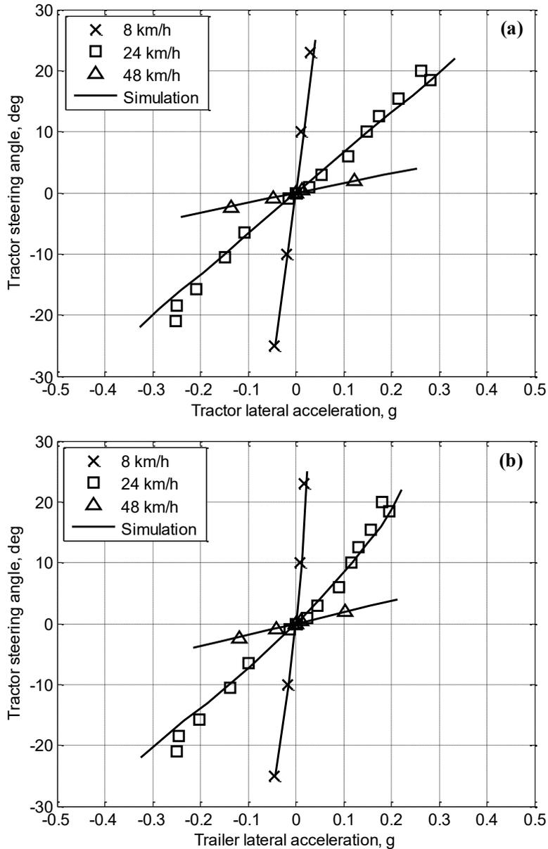
**Figure 49. Steady-state test results compared with simulation results**
