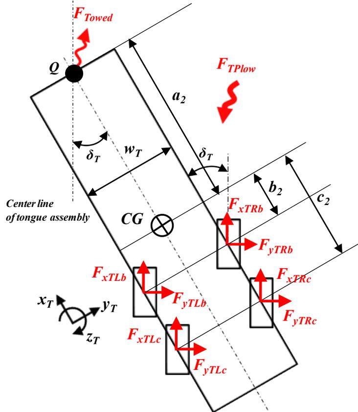
Figure 38. Scheme of the trailer unit and forces
