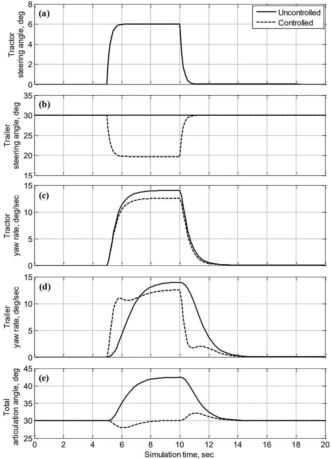
**Figure 35. Simulation results of the TowPlow comparing uncontrolled and controlled system for the pulse input: (a) Tractor steering angle, (b) Trailer steering angle, (c) Tractor yaw rate, (d) Trailer yaw rate, (e) Total articulation angle**
