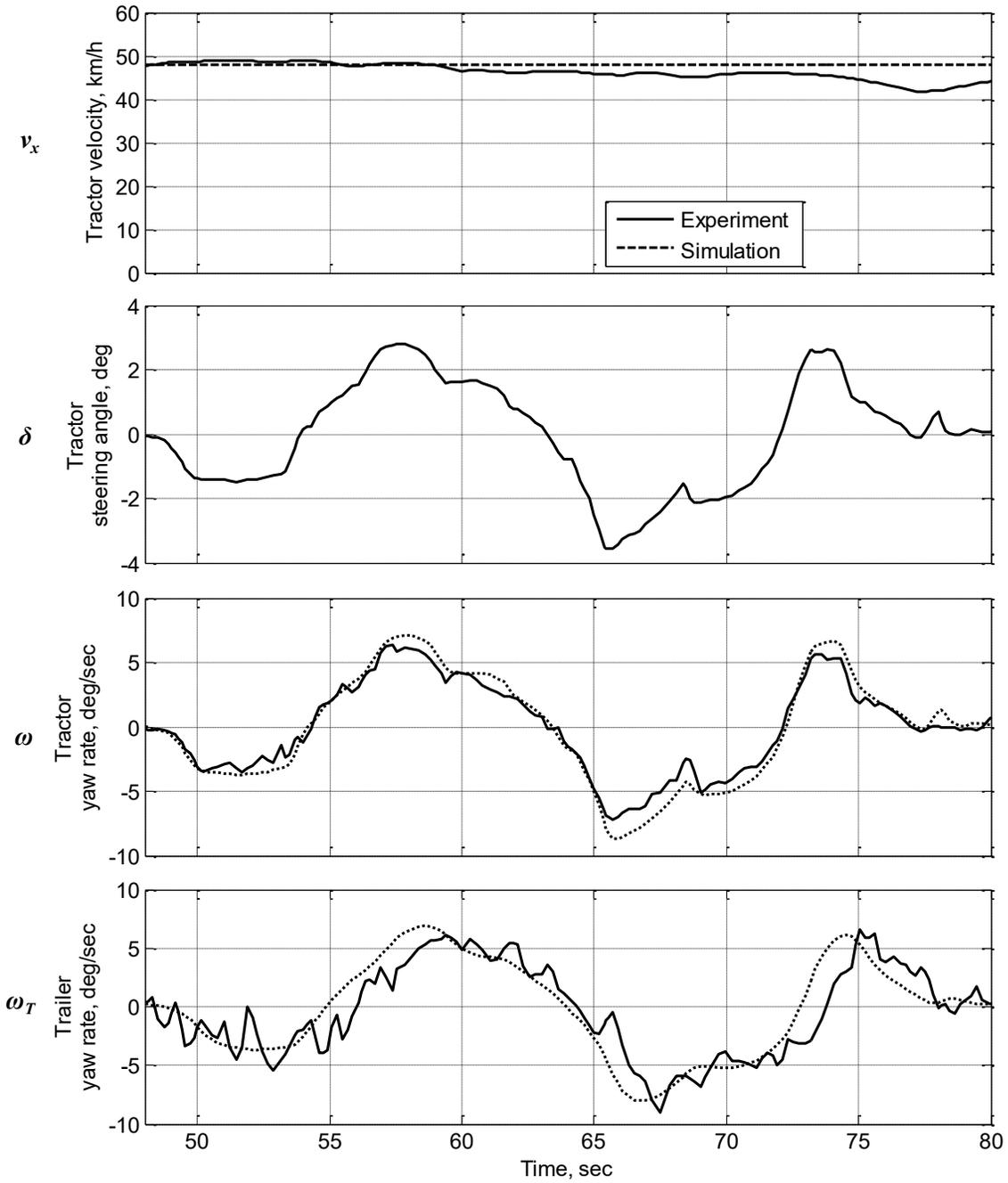
Figure 52. Transient test results compared with simulation results
