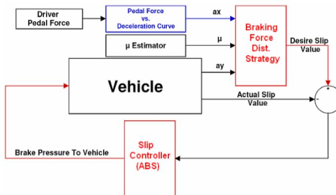
Figure 21. Control scheme of active braking control in [33]
