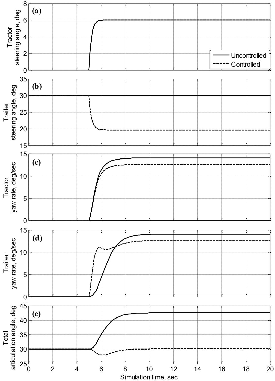
**Figure 34. Simulation results of the TowPlow comparing uncontrolled and controlled system for the step input: (a) Tractor steering angle, (b) Trailer steering angle, (c) Tractor yaw rate, (d) Trailer yaw rate, (e) Total articulation angle**
