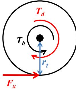
Figure 45. Free body diagram for a driving wheel
