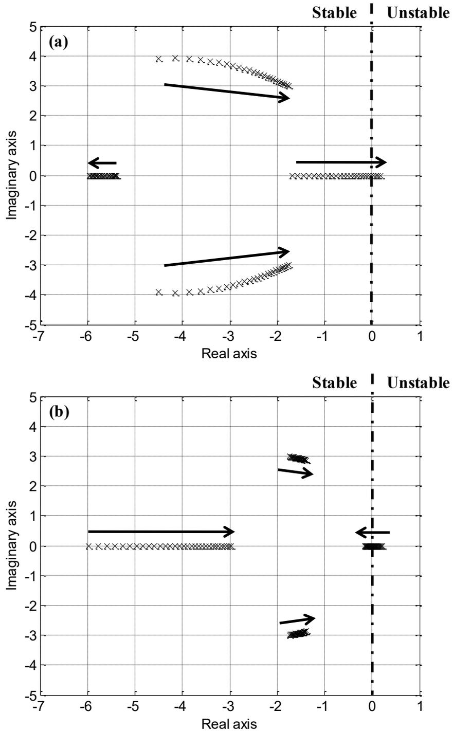
**Figure 31. Locus of the eigenvalues of the matrix  $M^{-1}A$  with varying inertias: (a) Minimum tractor inertia with varying trailer inertia, (b) Maximum trailer inertia with varying tractor inertia**
