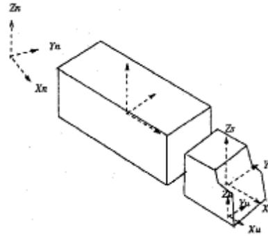
Figure 15. Coordinate system for the articulated vehicle by Chieh and Tomizuka [10]
