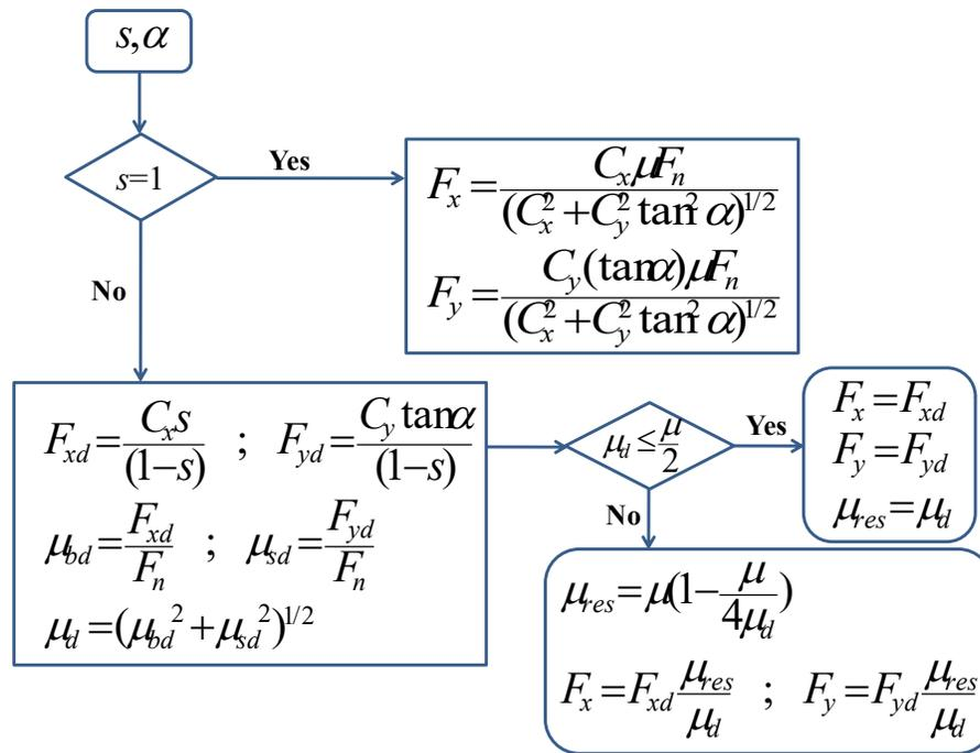
Figure 40. Flow chart of the tire force calculation [26]
