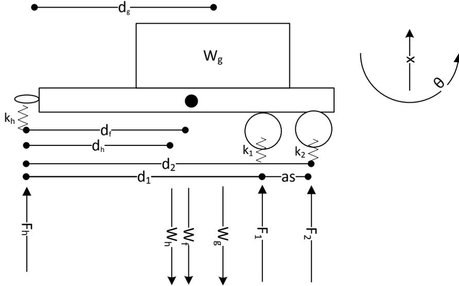
**Figure 89. Free body diagram for the indeterminate analysis of the TowPlow trailer**
