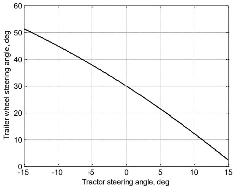
Figure 25. Tractor steering angle vs. Trailer wheel steering angle for constant total articulation angle  $\theta_t = 30^\circ$
