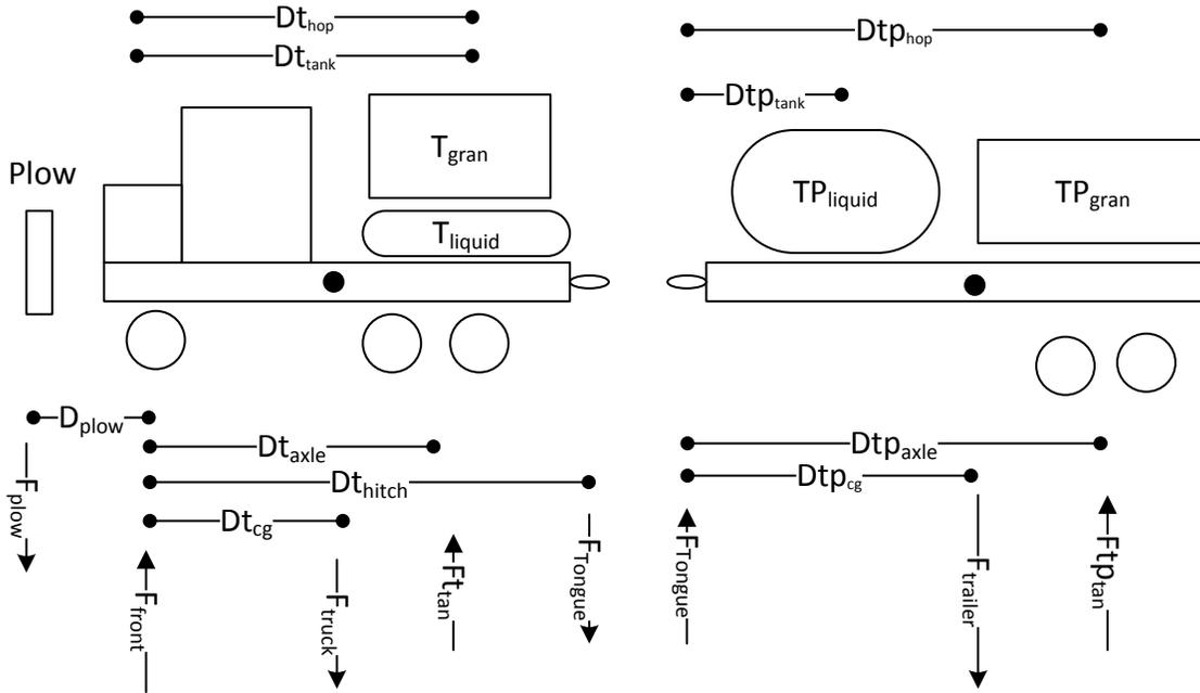
Figure 84. Free body diagram of TowPlow2
