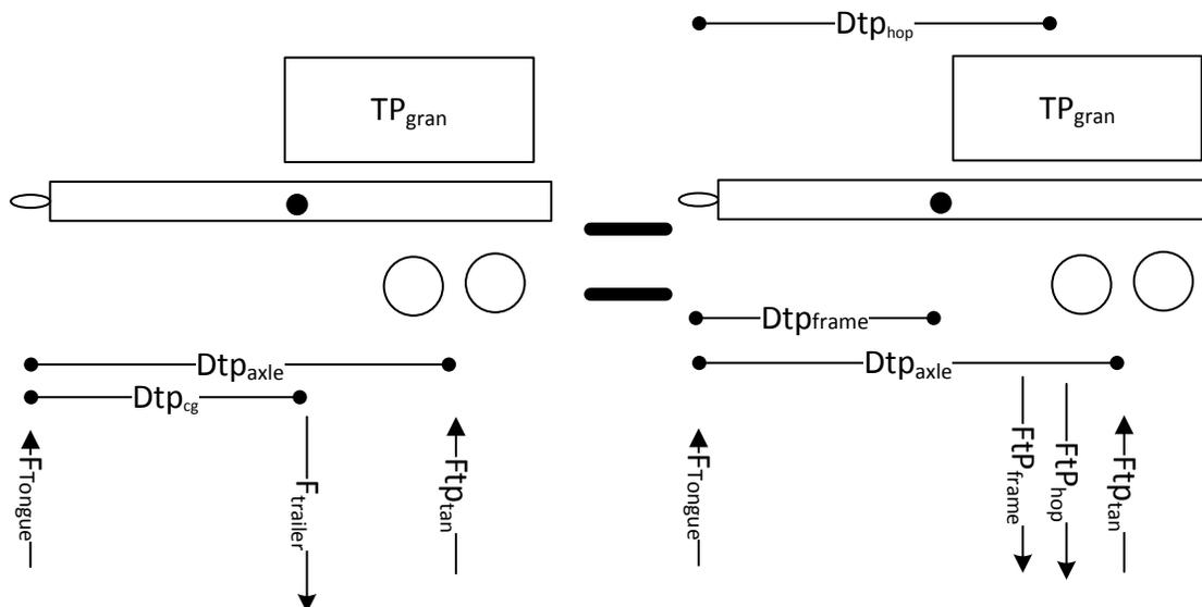
Figure 85. TowPlow2 trailer free body diagrams
