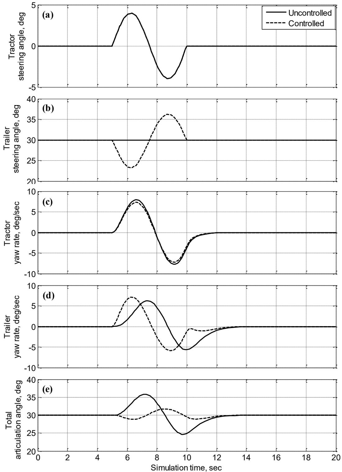
**Figure 36. Simulation results of the TowPlow comparing uncontrolled and controlled system for the sine input: (a) Tractor steering angle, (b) Trailer steering angle, (c) Tractor yaw rate, (d) Trailer yaw rate, (e) Total articulation angle**
