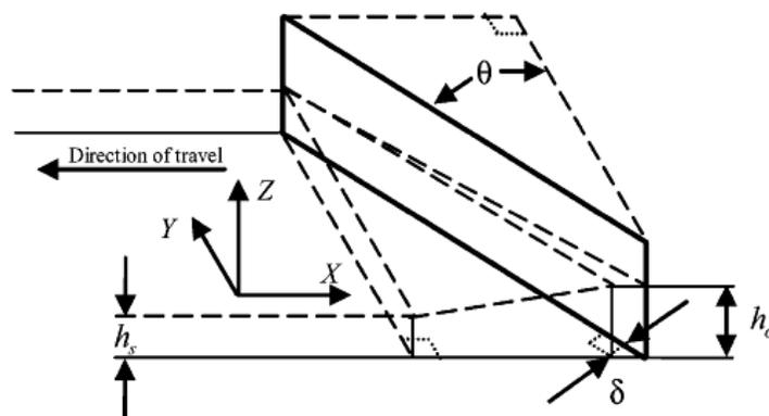
Figure 20. Control volume in front of the plow by Ravani et al. [49]
