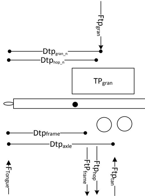
**Figure 86. Free body diagram for computing new weights after moving the sander.**
