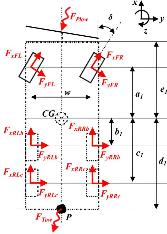
Figure 37. Scheme of the tractor unit and forces
