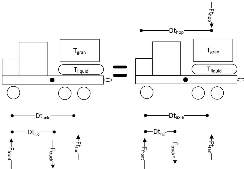
Figure 87. Free body diagram for the prime mover truck
