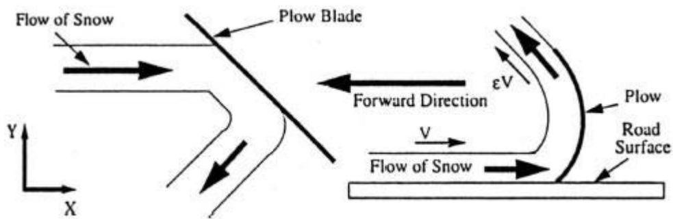
Figure 19: Kaku's snow flow assumption in snow resistance model [34]
