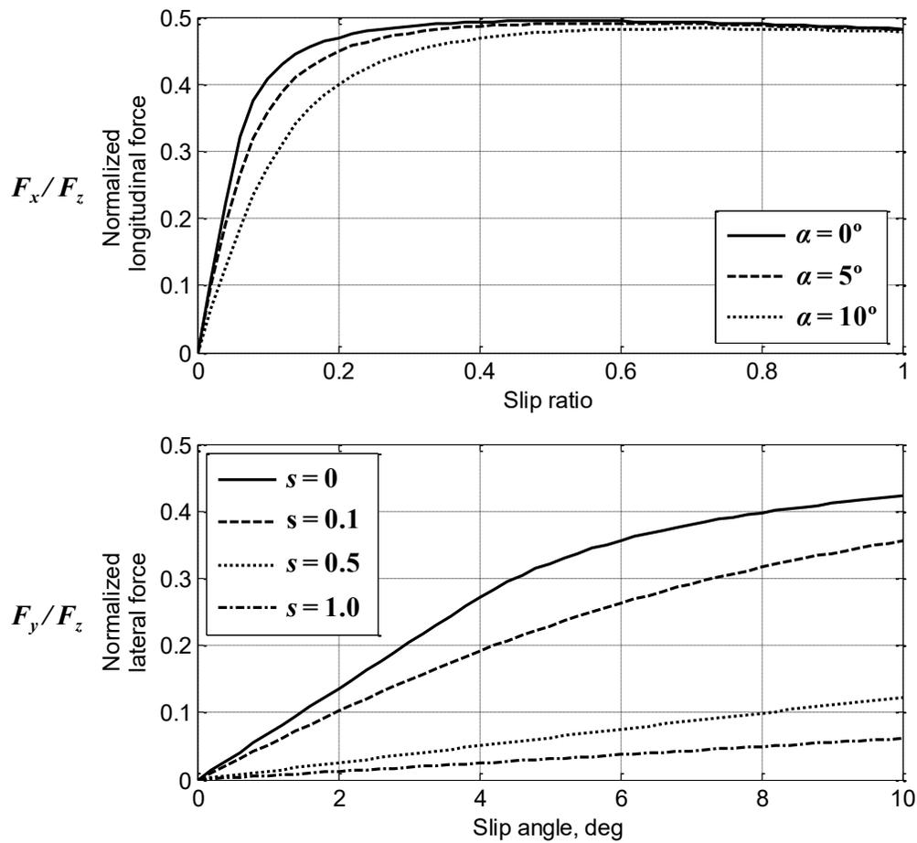
**Figure 41. Computed longitudinal and lateral tire forces**
