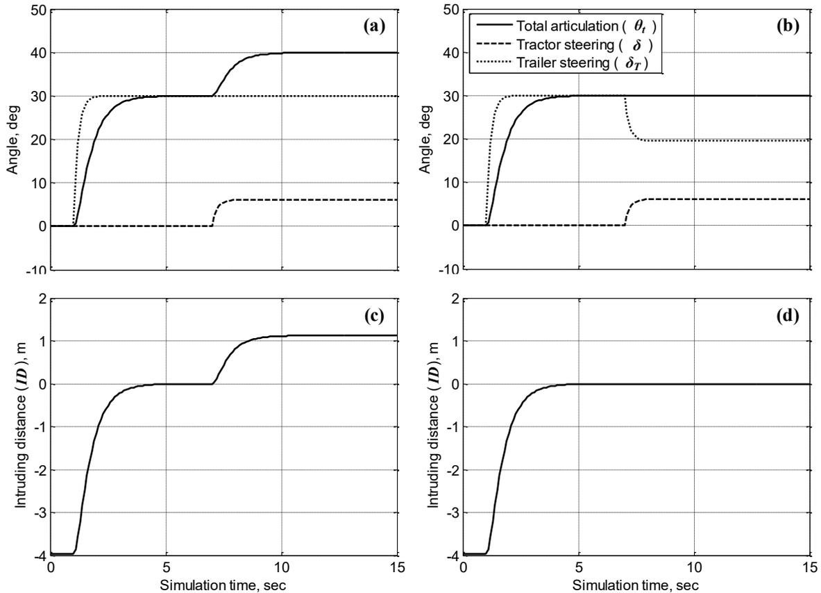
**Figure 26. Simulation results of the constant radius turning: (a) angles without trailer corrective steering, (b) angles with trailer corrective steering, (c) intruding distance without trailer corrective steering, (d) intruding distance with trailer corrective steering**
