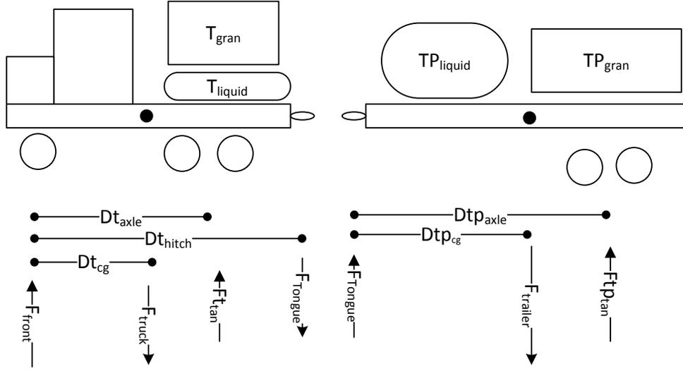
**Figure 83. Free body diagram of TowPlow2**
