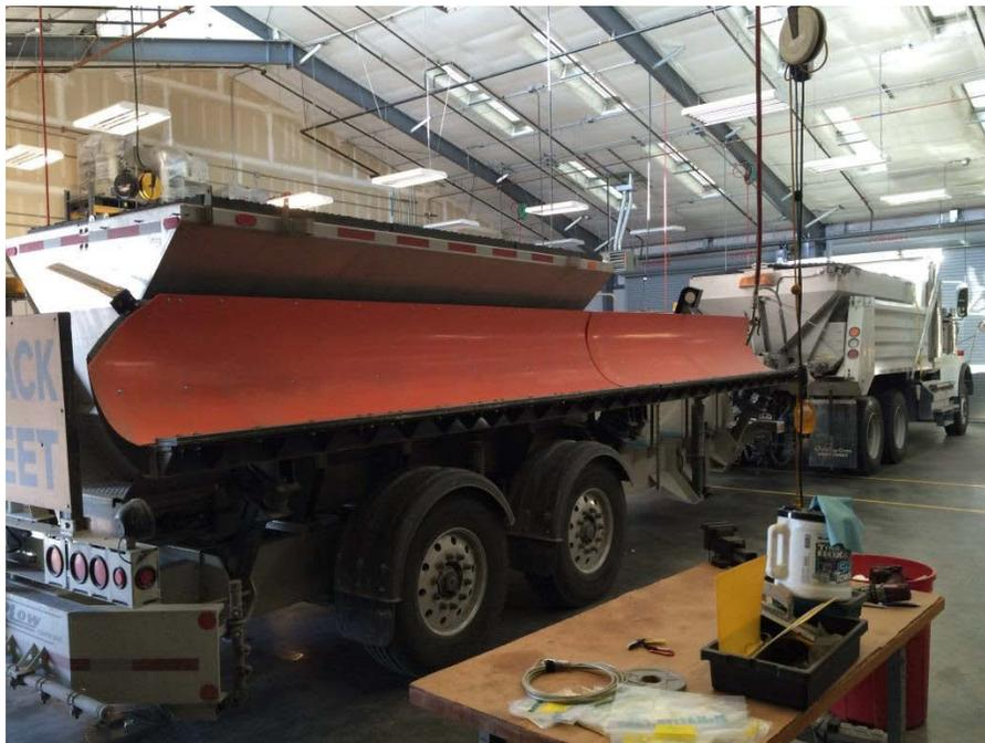
**Figure 5. The as-delivered TowPlow2**
