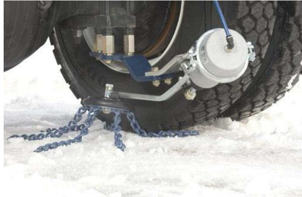
Figure 3. Onspot chain system [www.onspot.com]
