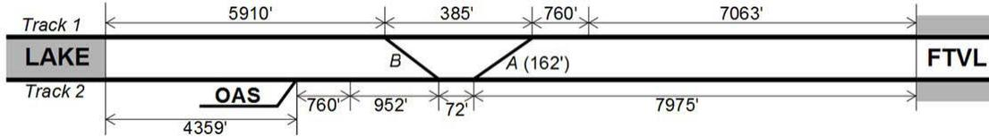
**Figure 3-3:** Rail Track Geometry at Access Point to Oakland Annex Shop (OAS) for section between Fruitvale (FTVL) and Lake Merritt (LAKE)
