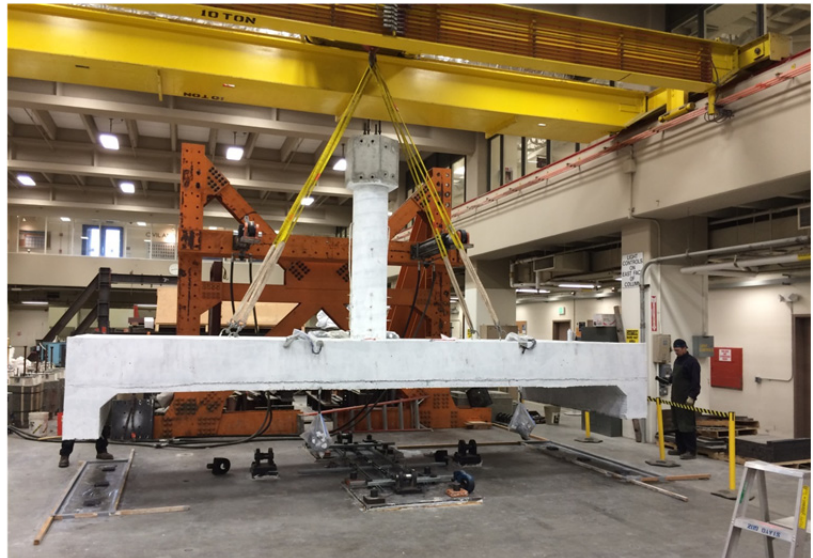
Figure D.4 Moving the first specimen from where it was constructed to where it was tested using the laboratory overhead 10-ton crane.
