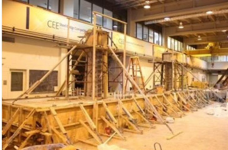
Figure C.14 Finished construction of the two specimens after three stages and being left to cure for 21 days before removing the formwork.
