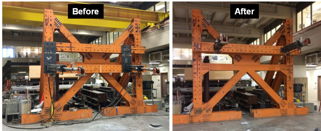
Figure D.1 Reconfiguring the reaction frame and horizontal actuators at the Structures Laboratory at University of California, Berkeley, to match the height of the test specimens.
