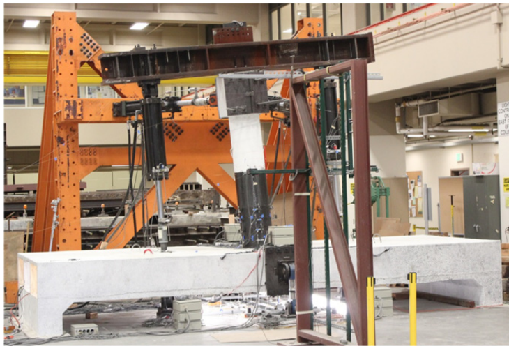
Figure 6.13 Overview of repaired Specimen No. 1 cyclic loading test set-up when loading is in progress and applied in longitudinal direction.
