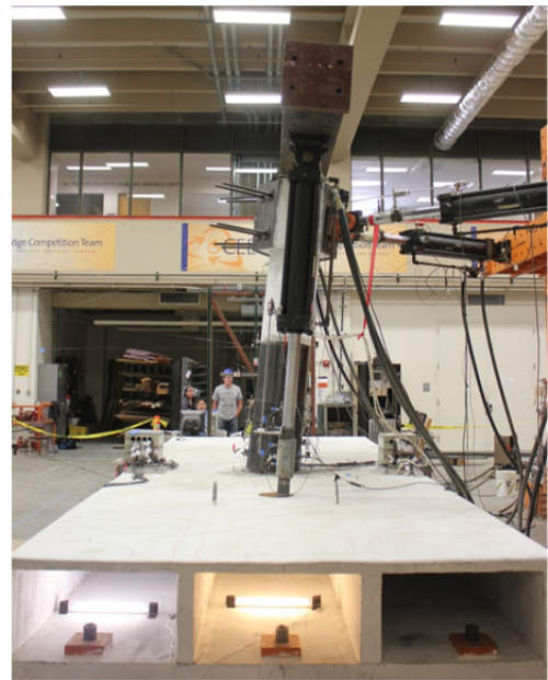
Figure 6.12 Overview of repaired Specimen No. 1 cyclic loading test set-up when loading is in progress and applied in transverse direction.
