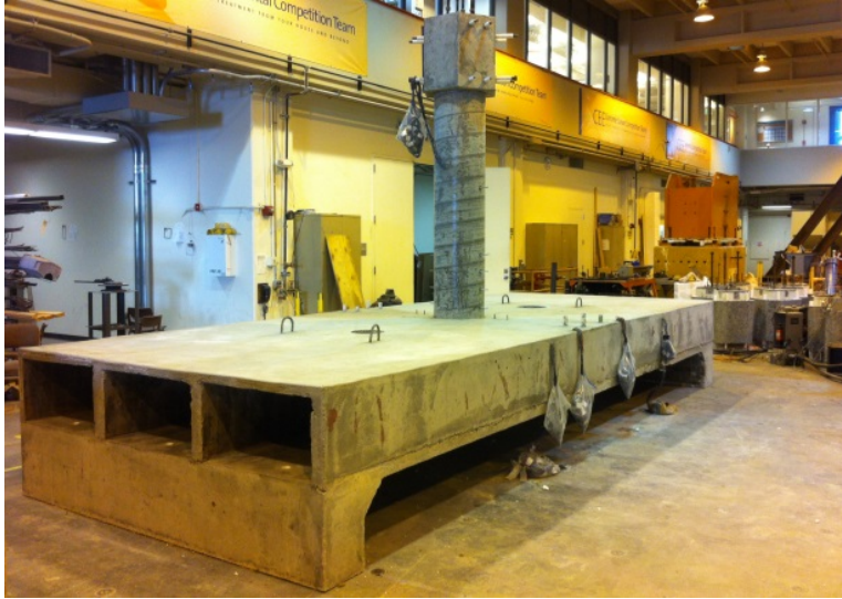
Figure C.17 A view of one of the two constructed box-girder subassembly specimens after all formwork removal.
