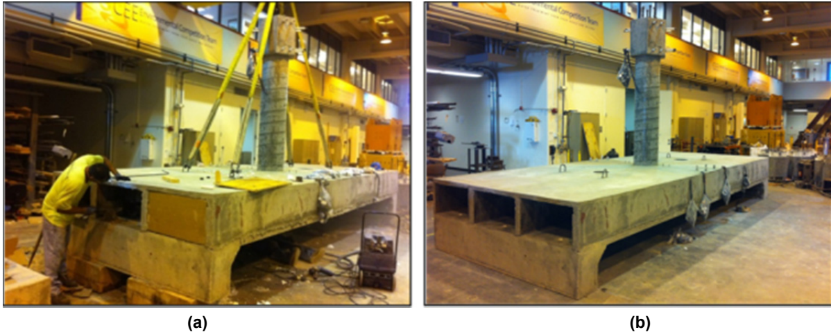
Figure 3.22 (a) Removing the cardboard boxes used to create the box-girder cells and (b) final specimen configuration.
