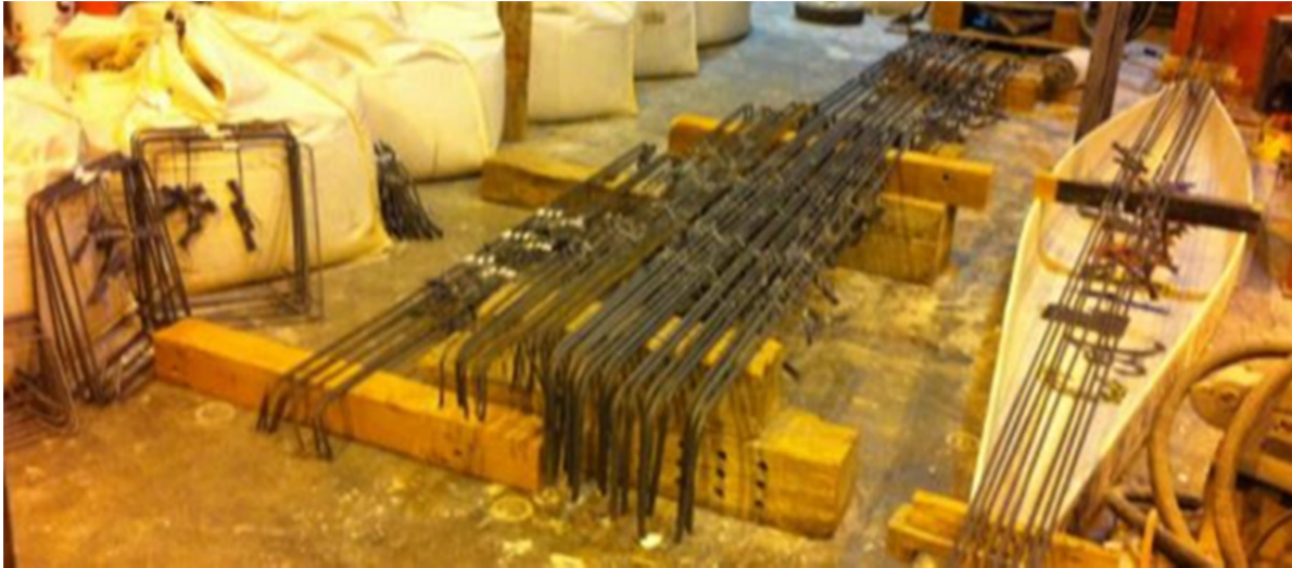
Figure 3.42 Instrumented specimen's beam and slab reinforcement bars.
