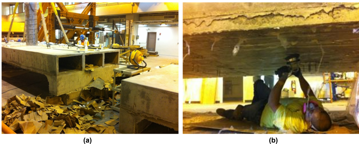
Figure C.16 (a) Remnants of the cardboard boxes from inside the box-girder cells; and (b) grinding any styrofoam or plastic wrap stuck to the concrete surface.
