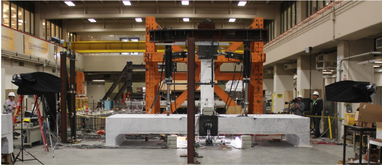
Figure D.13 Overview of the test set-up and final cameras and flash light installations.
