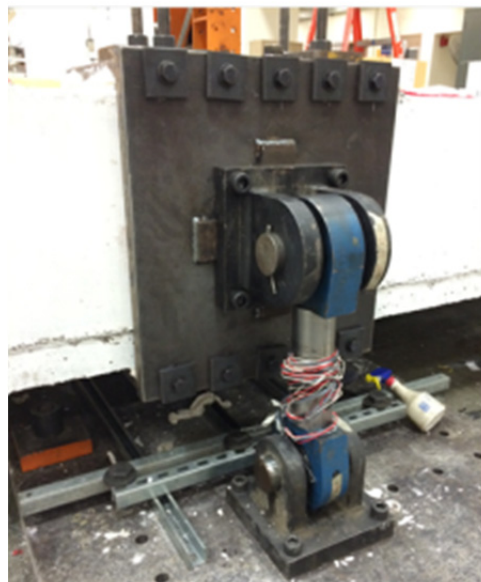
Figure 3.12 Vertical 1D calibrated strut used at the specimen's cap beam ends.
