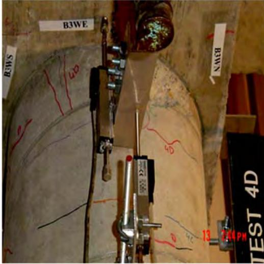
Damage State 3 (after test 4D)
