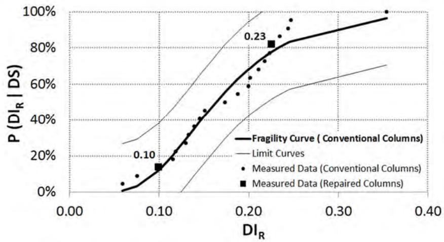
Figure 6-2. Resistance fragility curve for DS2 in conventional columns
