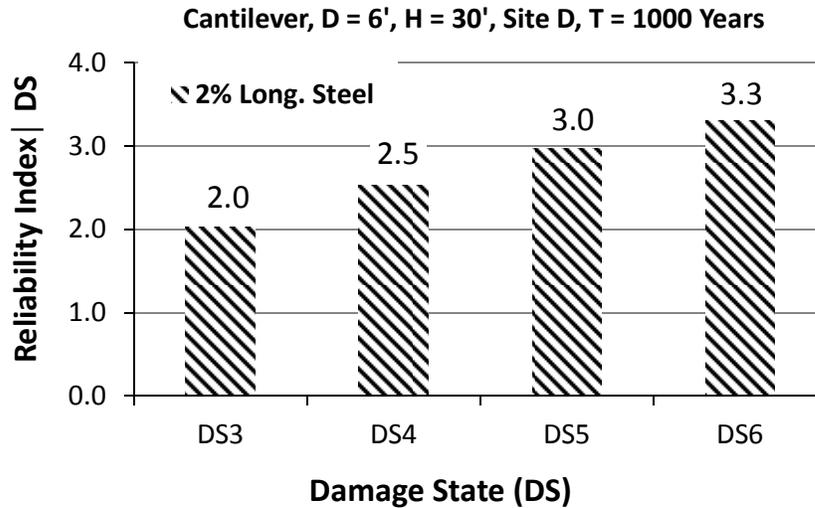
Figure A- 1. Reliability indices for SCB designed for DI = 0.35
