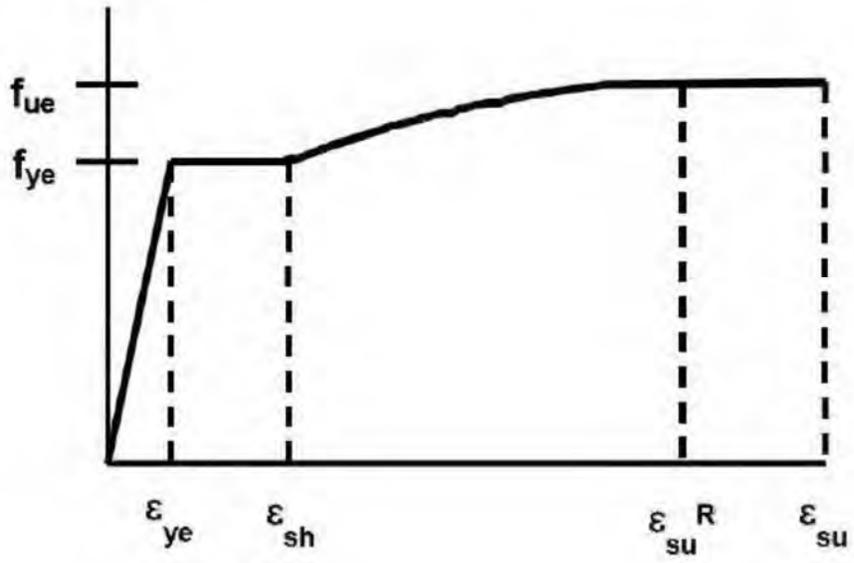
Figure 4-10. Steel stress strain model
