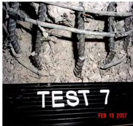
Damage State 6 (after test 7)
