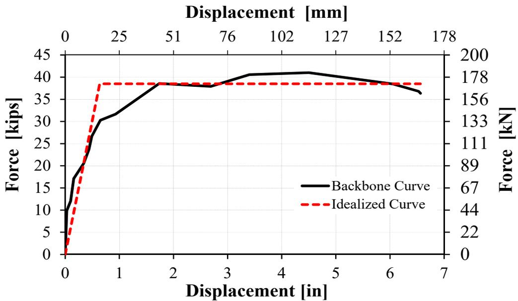
Figure 3-20. Bent 3 measured envelope and idealized force-displacement curve
