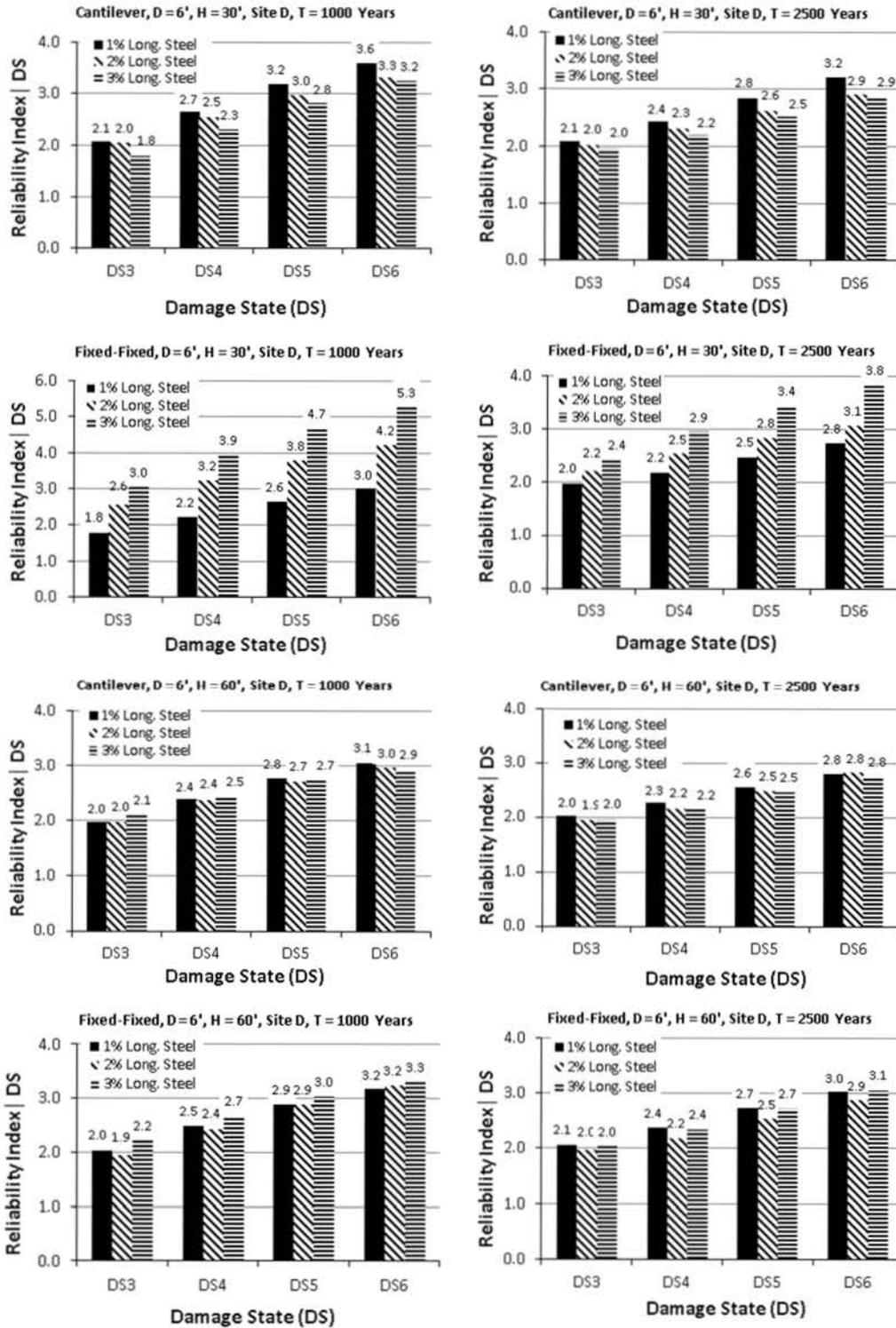
Figure 4-22. Reliability indices for SCBs with six foot diameter columns for Site D
