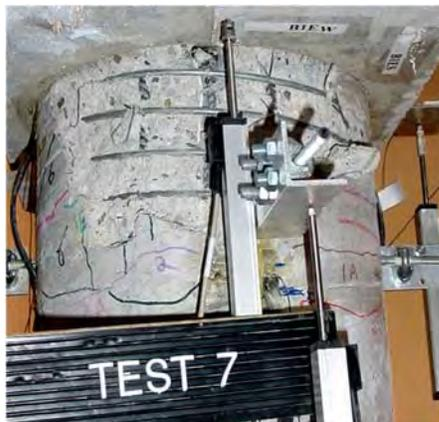
Damage State 5 (after test 7)
