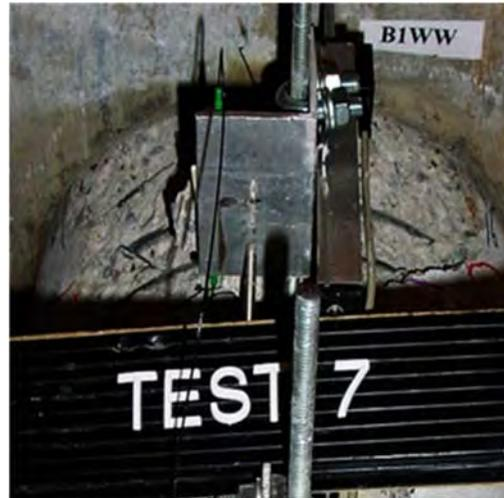
Damage State 3 (after test 7)
