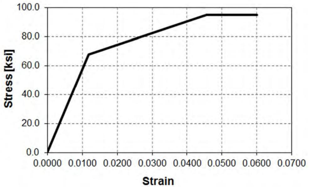
Figure 6-5. Modified stress-strain relationship for steel used for cantilever SCB
