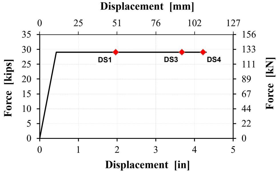
Figure 3-23. Idealized pushover curve and damage states for bent 2 East column
