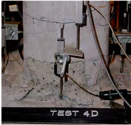
Damage State 3 (after test 4D)
