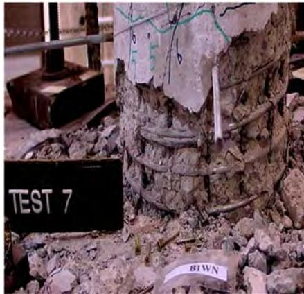
Damage State 5 (after test 7)
