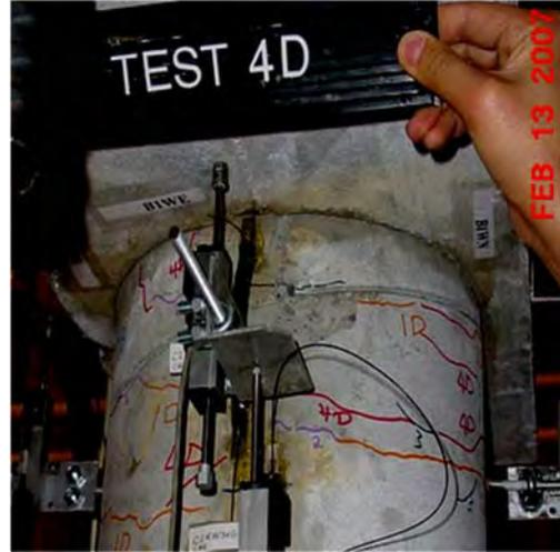
Damage State 2 (after test 4D)
