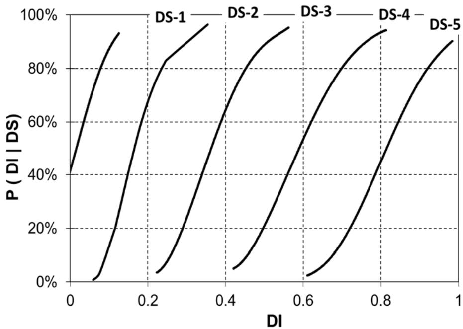
Figure 2-2. Correlation between damage states and damage indices
