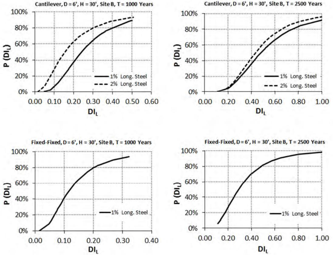
Figure 4-19. Fragility curves for SCBs with six foot diameter columns for Site B/C
