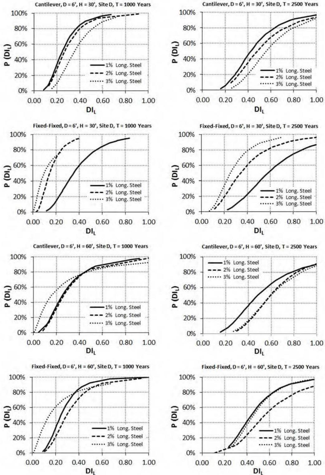
Figure 4-21. Fragility curves for SCBs with six foot diameter columns for Site D
