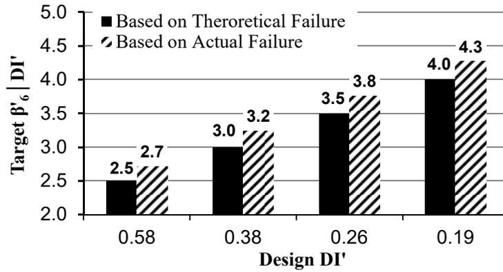
Figure 5-3. The target  $\beta'_6$  for a given design  $DI'$  for SCBs
