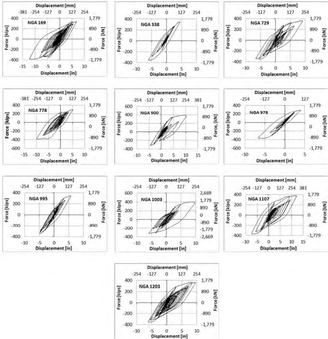
Figure 4-15. Force-displacement hysteresis curves for far-field GMs
