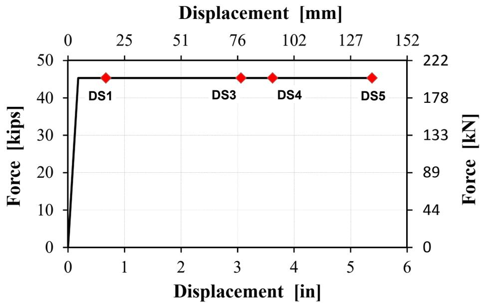
Figure 3-22. Idealized pushover curve and damage states for bent 1 West column
