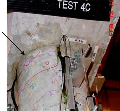
Damage State 2 (after test 4C)
