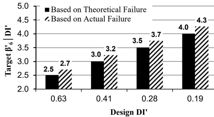
Figure 5-4. The target  $\beta'_6$  for a given design  $DI'$  for TCBs
