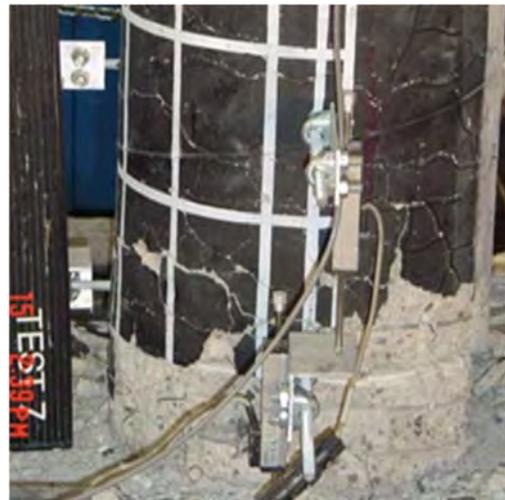
Damage State 4 (after test 7)
