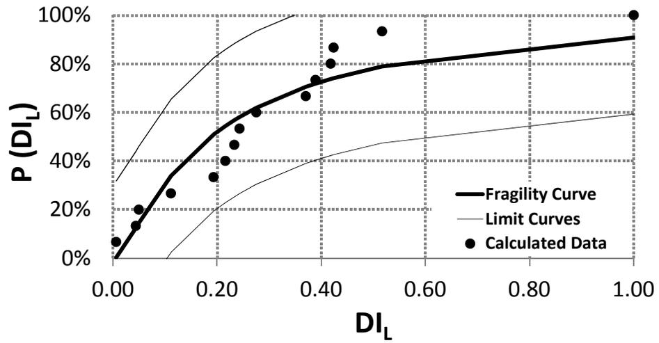
Figure 6-8. Fragility curve for  $DI_L$  for the repaired column
