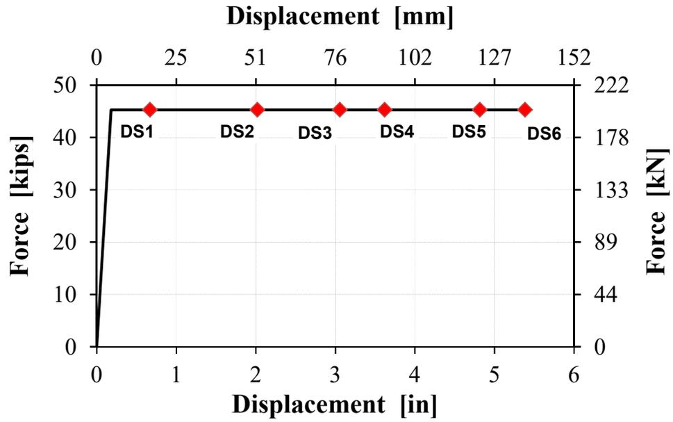
Figure 3-21. Idealized pushover curve and damage states for bent 1 East column
