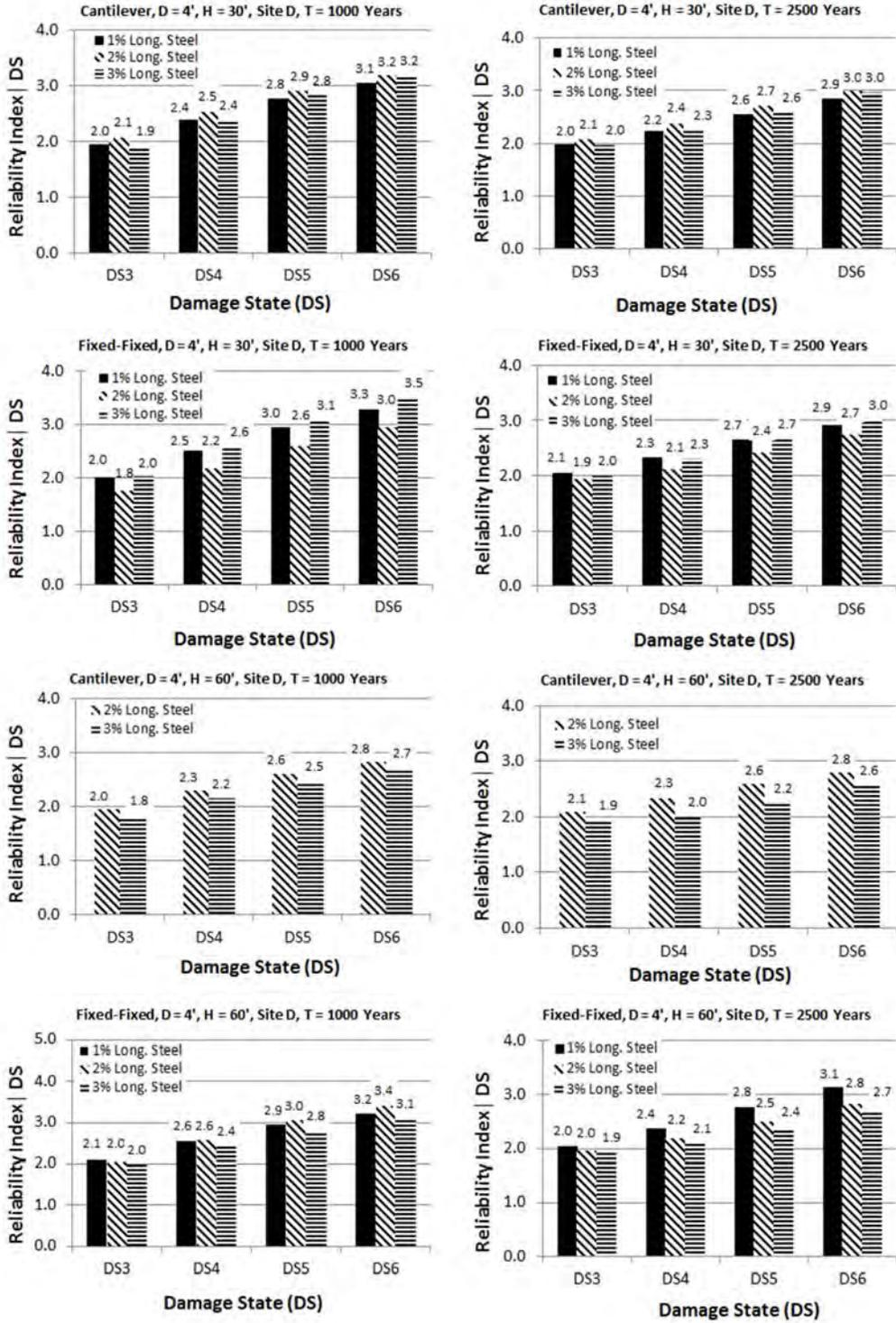
Figure 4-18. Reliability indices for SCBs with four foot diameter columns for Site D
