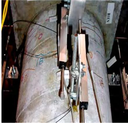
Damage State 1 (after test 1D)
