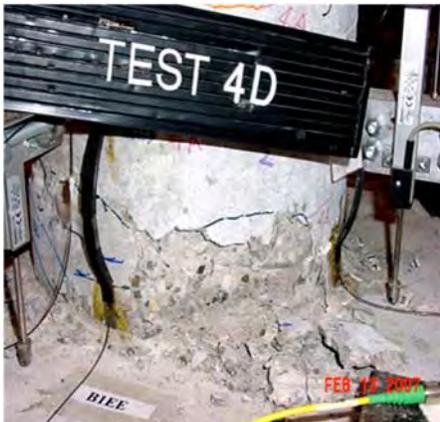
Damage State 3 (after test 4D)
