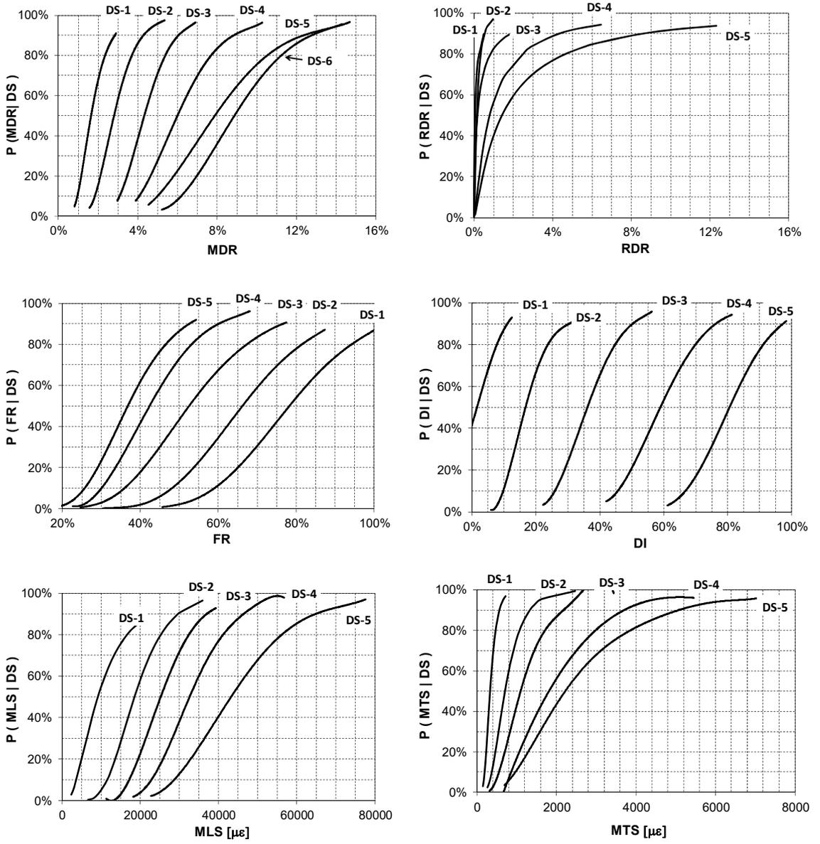
Figure 3-27. Combined fragility curves of response parameters
