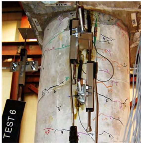
Damage State 3 (after test 6)
