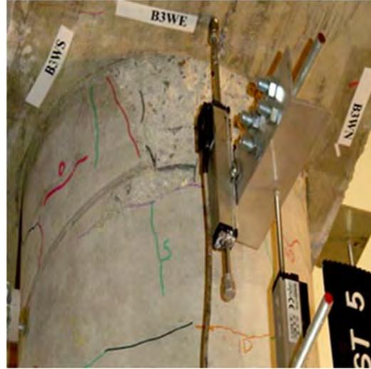
Damage State 4 (after test 5)
