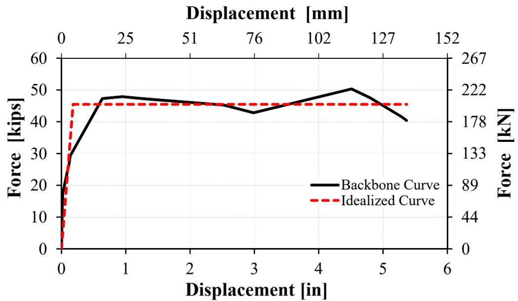
Figure 3-16. Bent 1 measured envelope and idealized force-displacement curve
