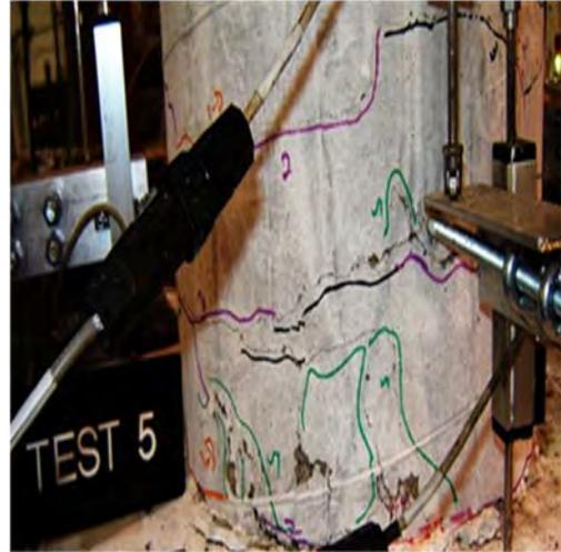
Damage State 2 (after test 5)
