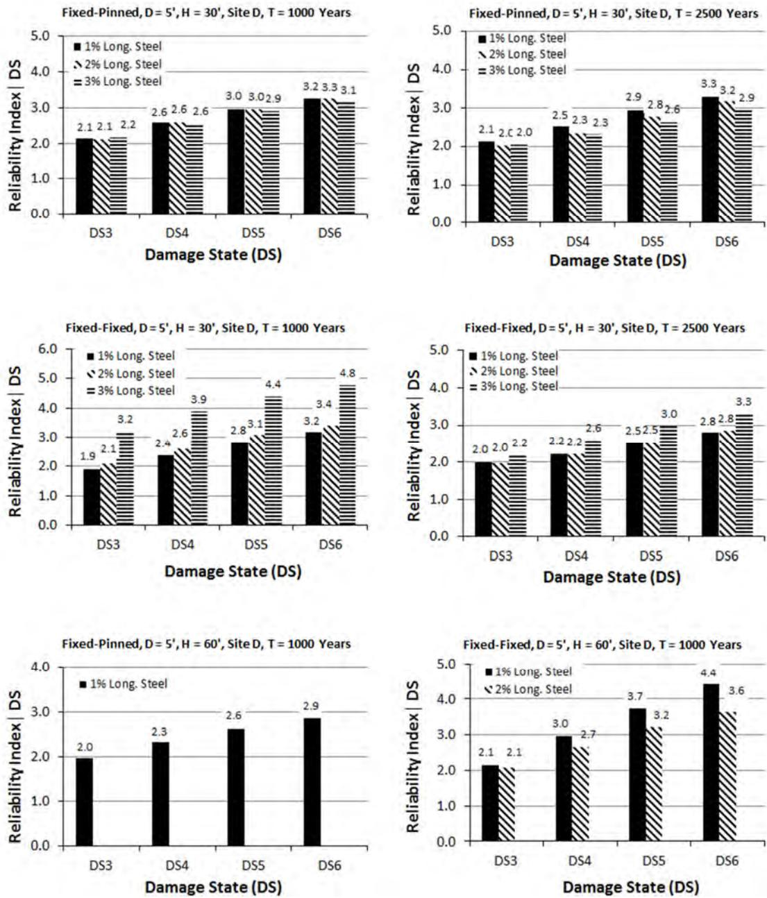
Figure 4-28. Reliability indices for TCBs with five foot diameter columns for Site D
