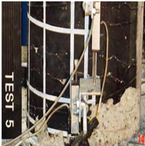
Damage State 3 (after test 5)
