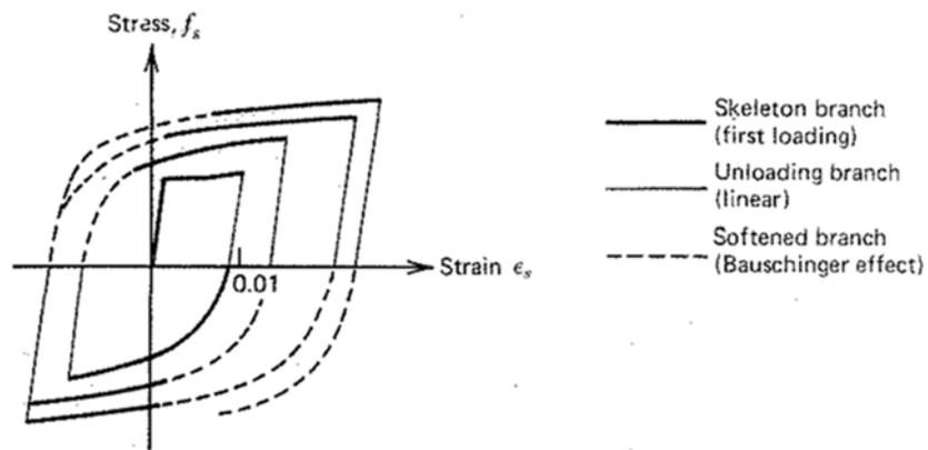
Figure 6-3. Stress-strain curves for steel with reversed loading (Park and Paulay 1975)
