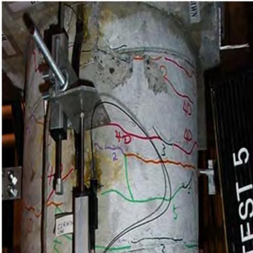
Damage State 3 (after test 5)
