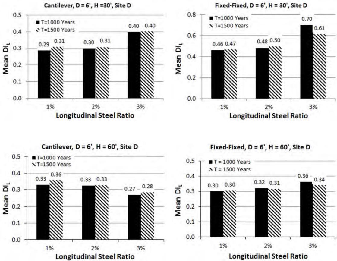
Figure 4-24. Mean  $D_{IL}$  for T=1000 and 1500-year earthquake
