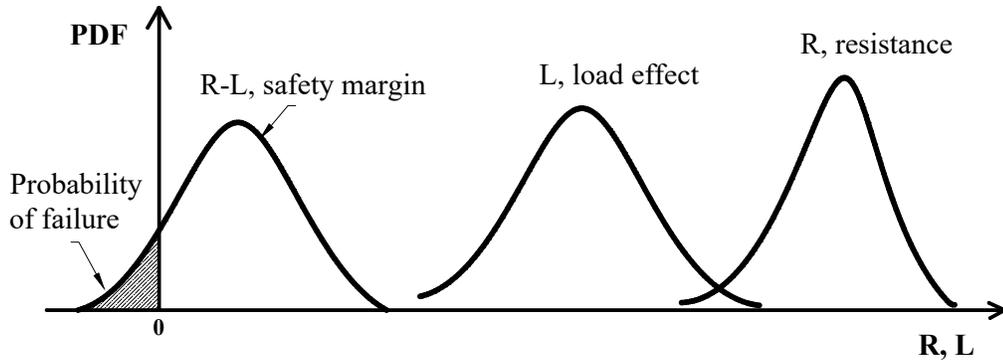
Figure 2-4. Probability distribution functions of load, resistance, and safety margin (Nowak & Collins 2000).
