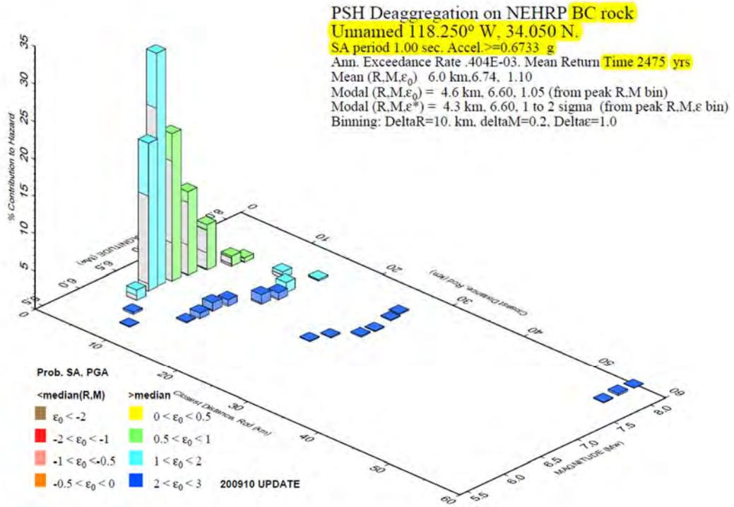
GMT 2014 Feb 7 18:46:12 Distance (R), magnitude (M), epsilon (E0,E) deaggregation for a site on rock with average  $v_s=760$  m/s top 30 m. USGS CGMT PSHA2008 UPDATE Bins with 0.05% contrib. omitted
