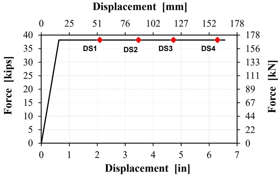
Figure 3-25. Idealized pushover curve and damage states for bent 3 East column
