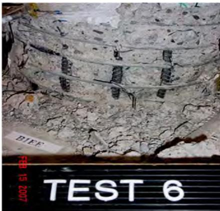
Damage State 5 (after test 6)
