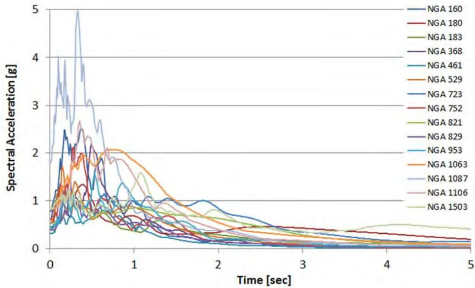
Figure 4-4. Near-field ground motions response spectrum of site class D
