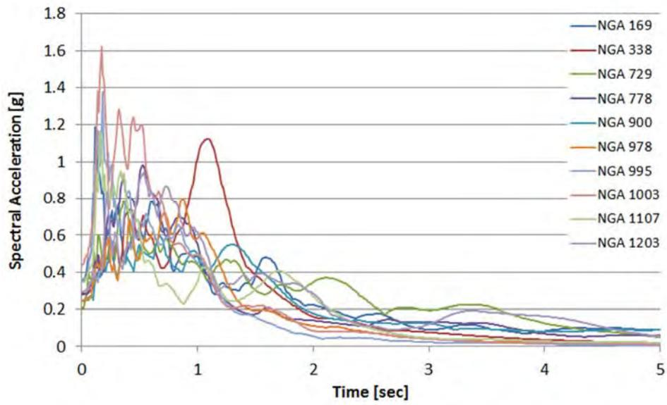
Figure 4-3. Far-field ground motions response spectrum of site class D
