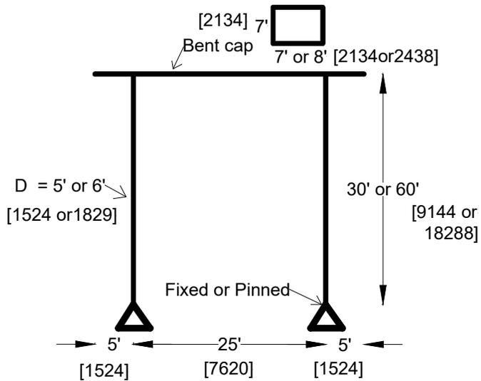
Figure 4-13. Typical two column bents configuration
