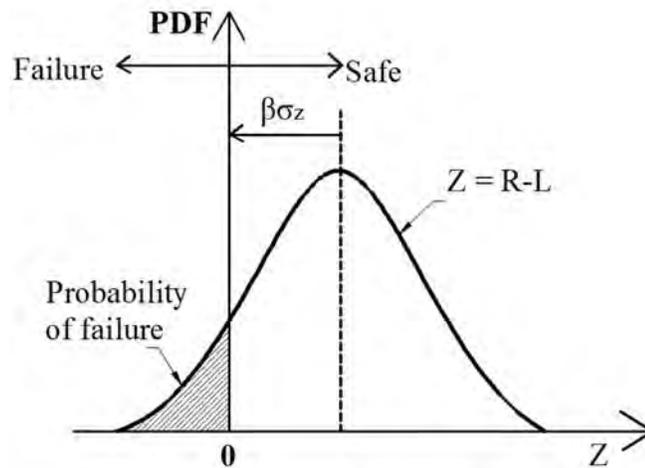
Figure 2-5. Graphical representation of reliability index and probability of failure (Cornell 1969)
