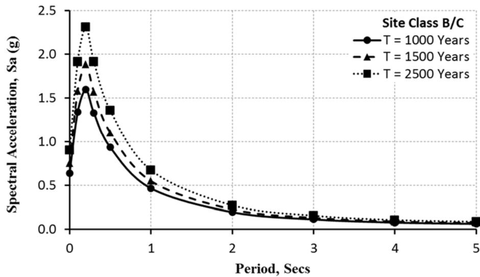
Figure 4-7. Design spectrum for site class B/C
