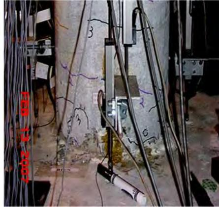
Damage State 2 (after test 3)
