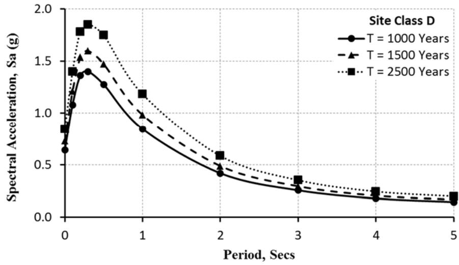
Figure 4-8. Design spectrum for site class D
