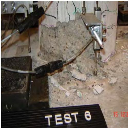
Damage State 3 (after test 6)
