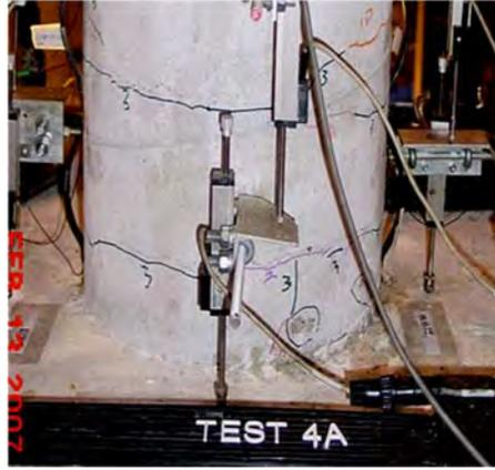
Damage State 2 (after test 4A)
