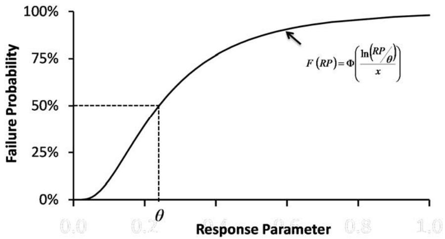
Figure 2-3. Fragility curve using lognormal distribution
