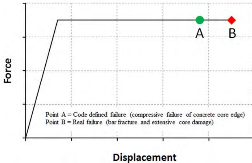
Figure 5-2. Definition of column failure
