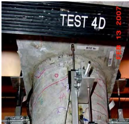
Damage State 3 (after test 4D)
