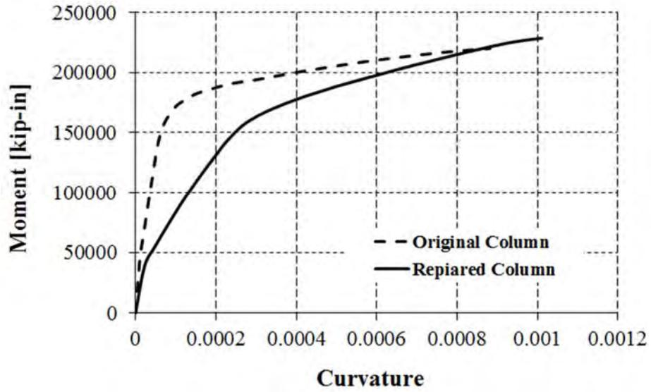
Figure 6-6. Moment curvature curves for the original and repaired columns
