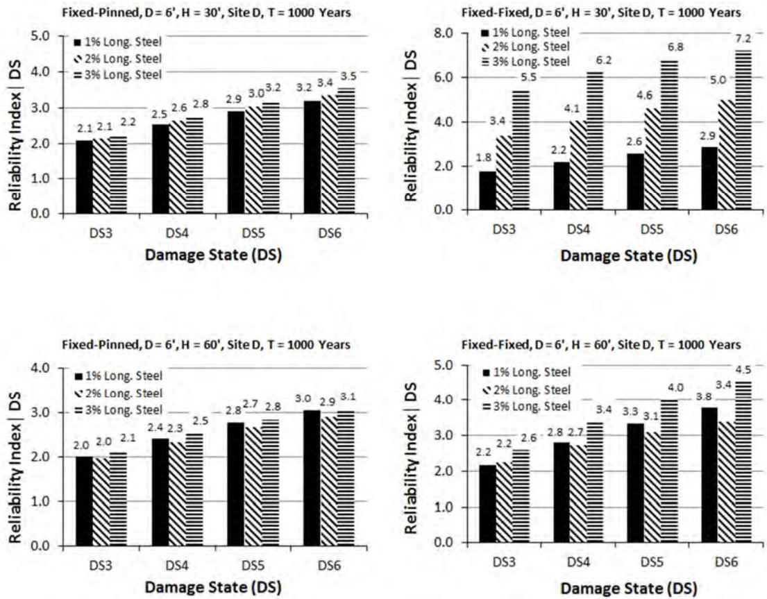
Figure 4-30. Reliability indices for TCBs with six foot diameter columns for Site D
