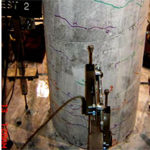
Damage State 1 (after test 2)
