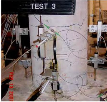
Damage State 1 (after test 3)
