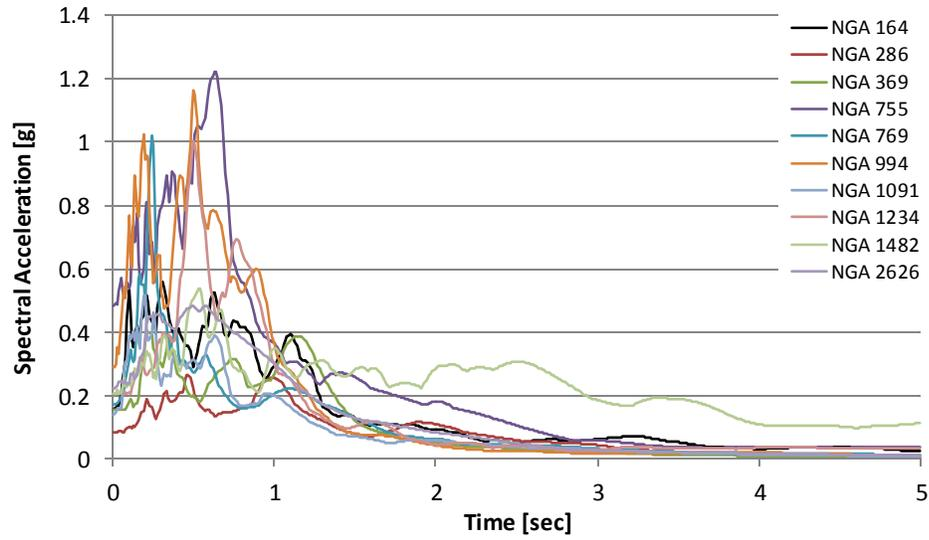
Figure 4-1. Far-field ground motions response spectrum of site class B/C
