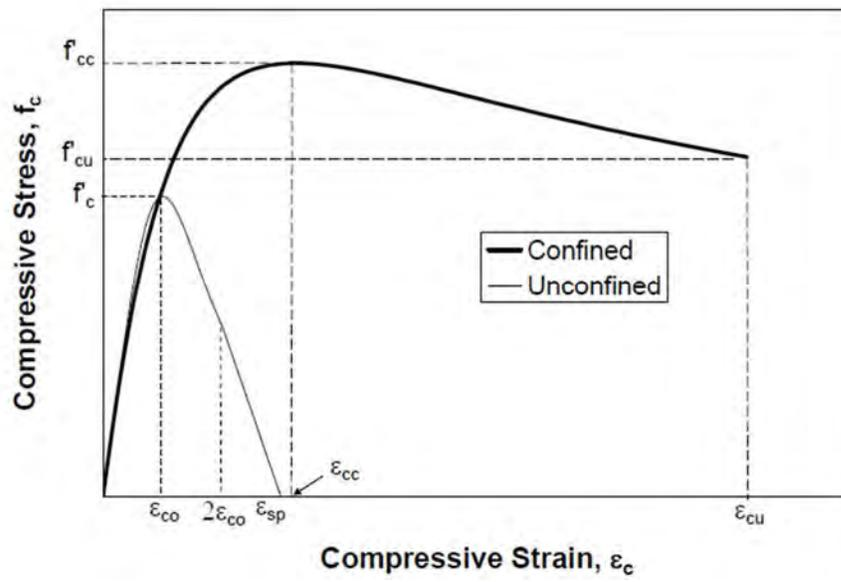
Figure 4-9. Mander's confined and unconfined concrete model
