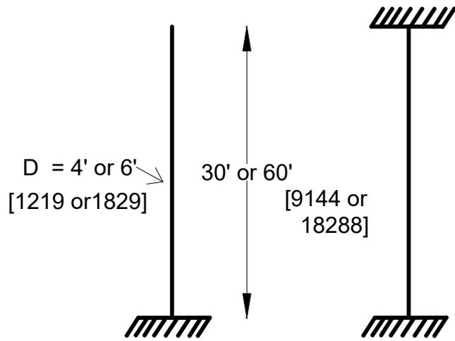
Figure 4-12. Typical single column bents configuration
