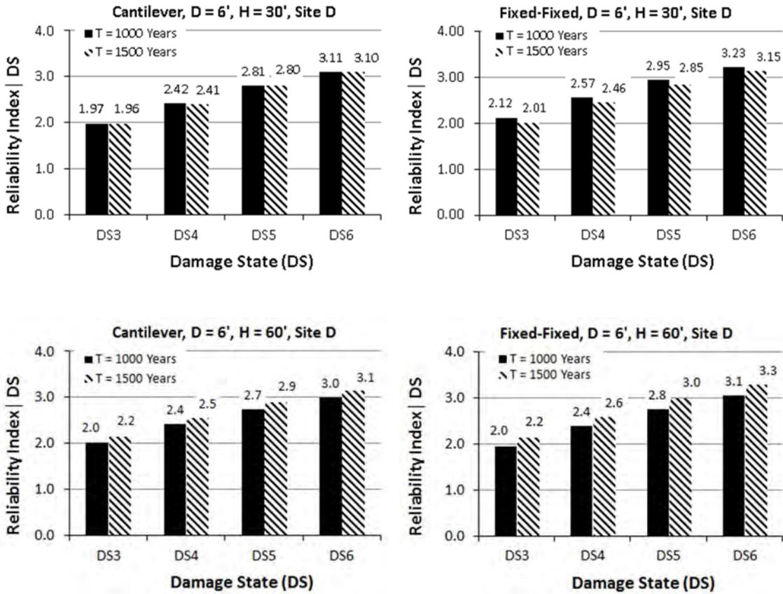
Figure 4-26. Reliability indices for T=1000 and 1500-year earthquake
