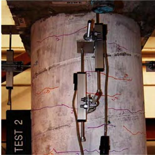
Damage State 1 (after test 2)
