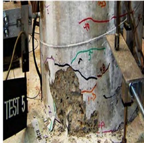
Damage State 3 (after test 5)
