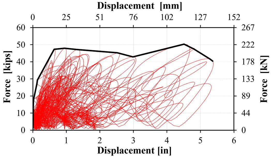
Figure 3-15. Bent 1 measured force-displacement hysteresis curves and envelope
