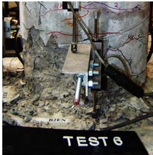
Damage State 4 (after test 6)
