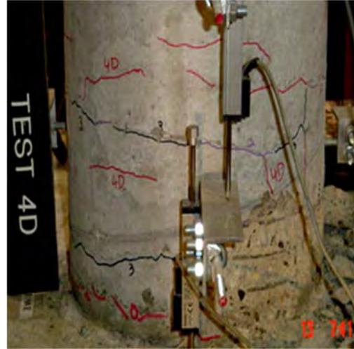
Damage State 4 (after test 4D)
