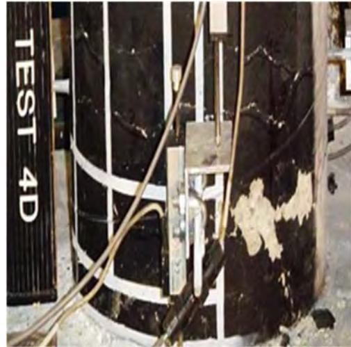
Damage State 2 (after test 4D)
