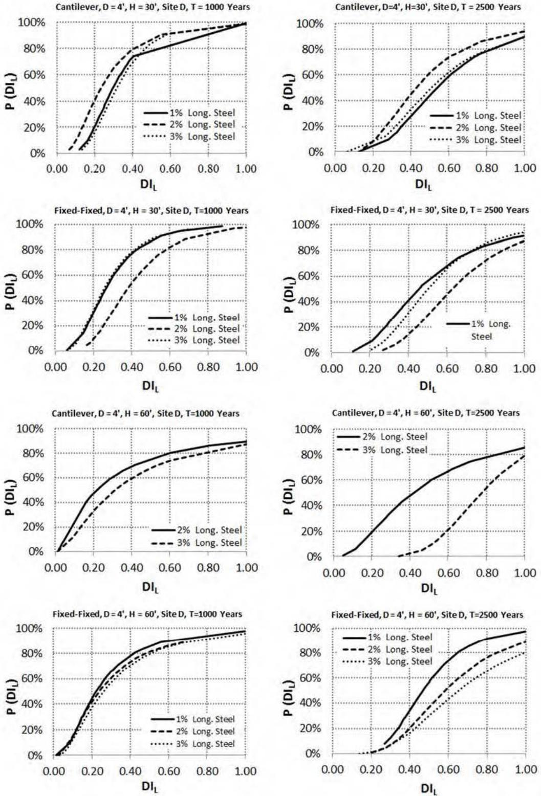
Figure 4-17. Fragility curves for SCBs with four foot diameter columns for Site D
