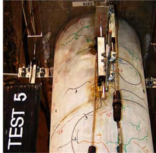
Damage State 2 (after test 5)
