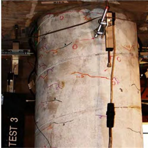
Damage State 1 (after test 3)
