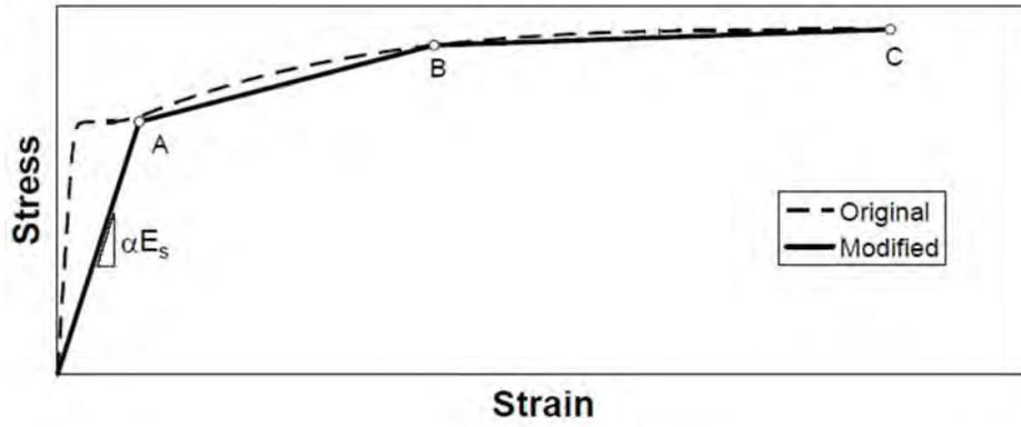
Figure 6-4. Original and modified stress-strain relationship for steel (Vosooghi and Saiidi 2010)
