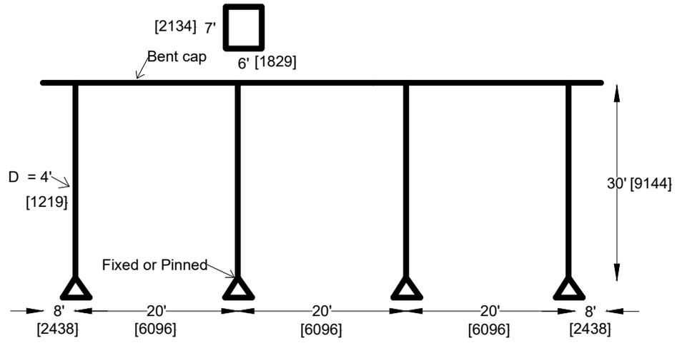
Figure 4-14. Typical four Column Bents configuration
