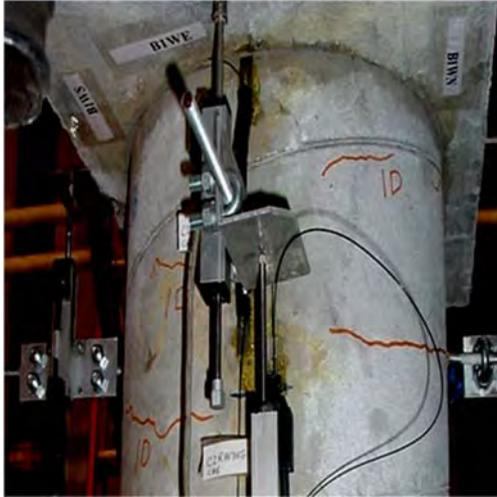
Damage State 1 (after test 1D)
