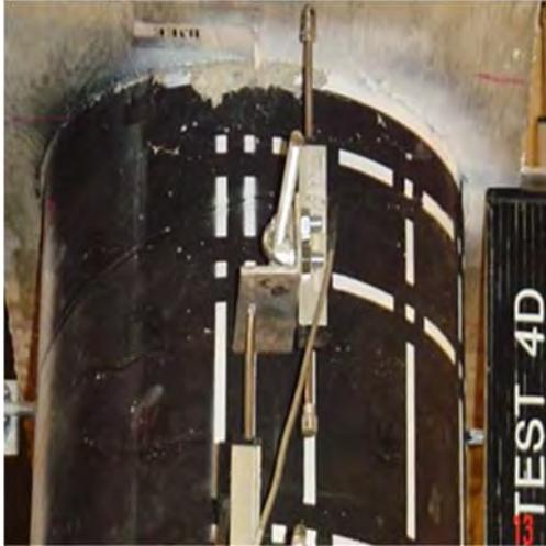
Damage State 2 (after test 4D)
