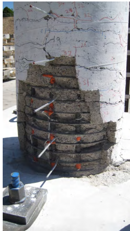
Figure 5.7- PNC (Left) and CIP (Right) Columns Plastic Hinge Damage after Testing
