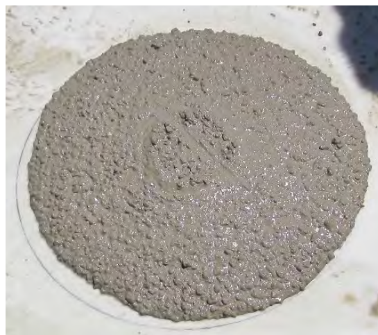
Figure 3.12- Visual Stability Index (VSI) Evaluation for SCC Mix Used in PNC/GCDP Columns
