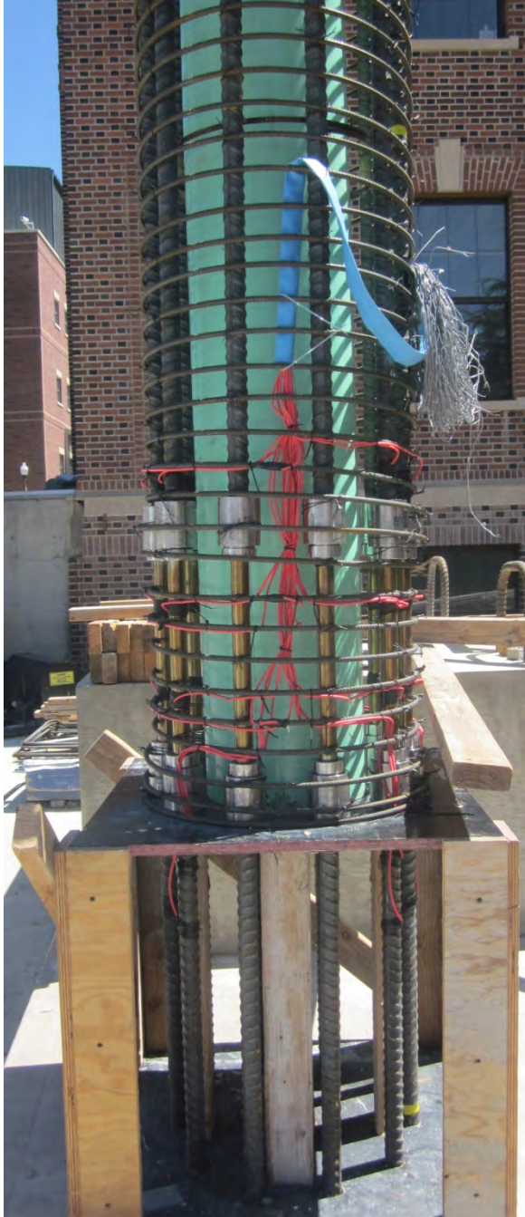
Figure 3.27- Bar Cage in HCS Model
