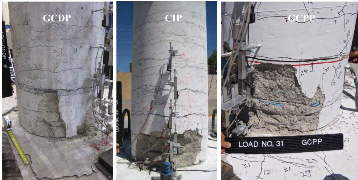
Figure 5.14- GCDP, CIP, and GCPP Columns Plastic Hinge Damage at Second Push of 5% Drift
