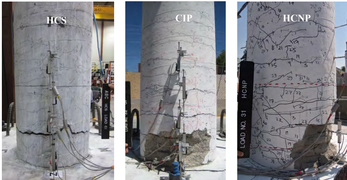
Figure 5.26- HCS, CIP, and HCNP Columns Plastic Hinge Damage at Second Push of 5% Drift
