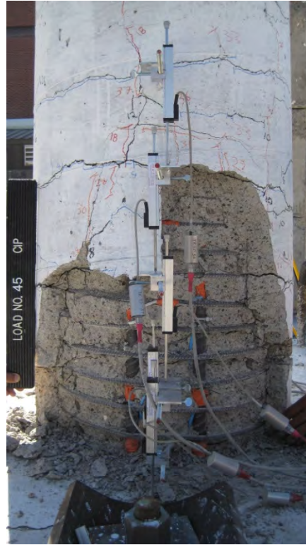
Figure 5.6- PNC (Left) and CIP (Right) Columns Plastic Hinge Damage at Last Pull of 10% Drift
