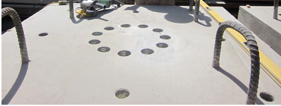
Figure 3.8- Precast Footing with Embedded Ducts in PNC Model
