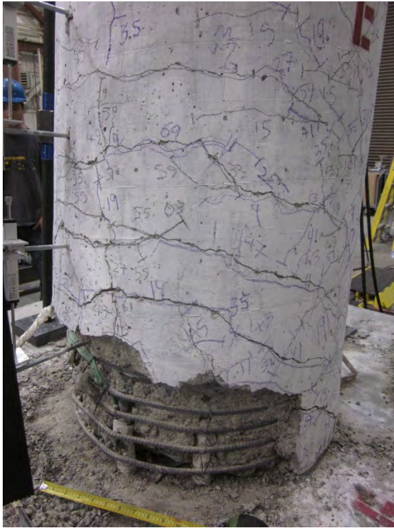
Figure 5.6- PNC (Left) and CIP (Right) Columns Plastic Hinge Damage at Last Pull of 10% Drift
