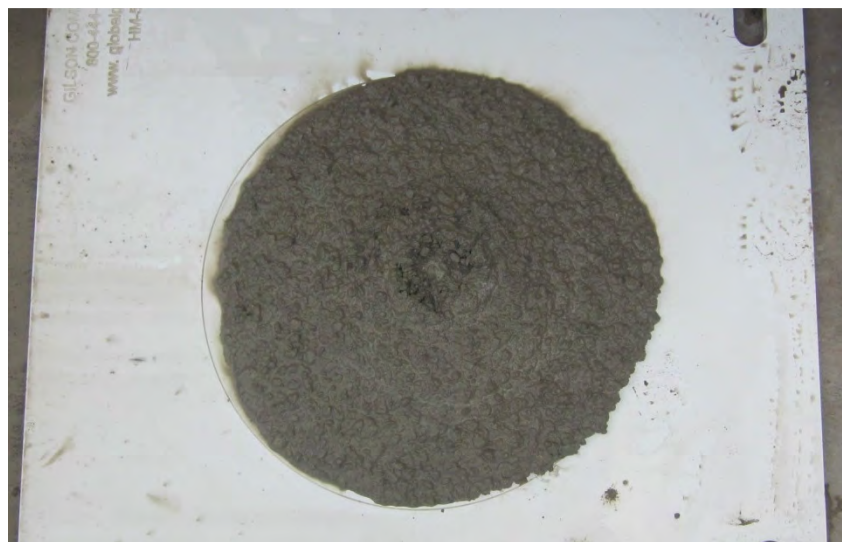
Figure 3.33- Visual Stability Index (VSI) Evaluation for SCC Mix in HCS Column
