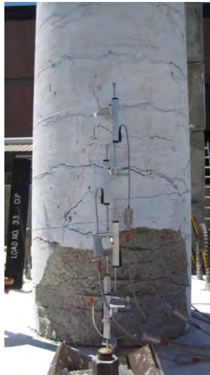
Figure 5.2- PNC (Left) and CIP (Right) Columns Plastic Hinge Damage at Second Pull of 5% Drift
