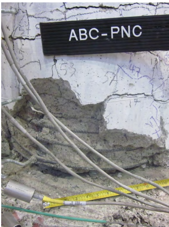
Figure 5.3- PNC (Left) and CIP (Right) Columns Plastic Hinge Damage at Second Push of 8% Drift
