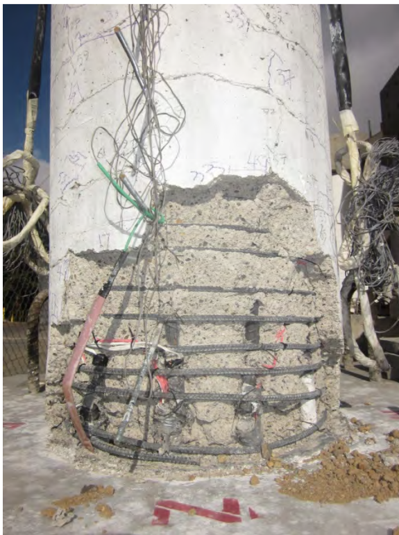
Figure 5.7- PNC (Left) and CIP (Right) Columns Plastic Hinge Damage after Testing
