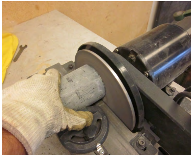
(b) End Grinding
