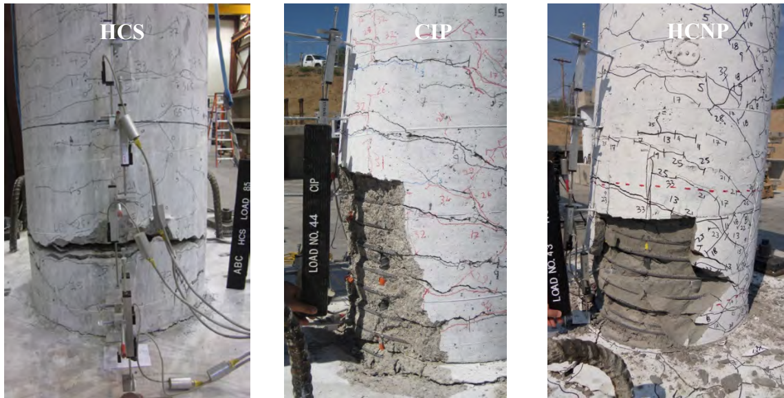
Figure 5.32- HCS, CIP, and HCNP Columns Plastic Hinge Damage at Second Push of 10% Drift
