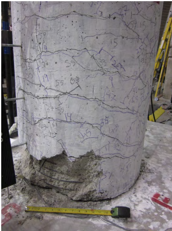
Figure 5.2- PNC (Left) and CIP (Right) Columns Plastic Hinge Damage at Second Pull of 5% Drift
