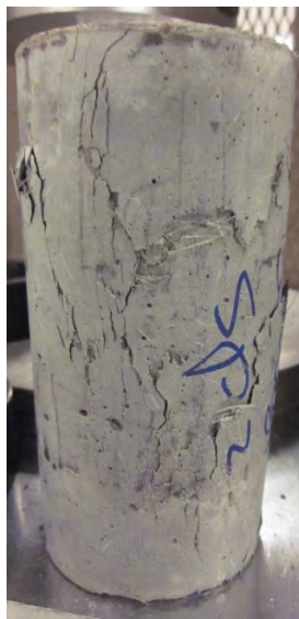
Figure 4.2- UHPC Compressive Mode of Failure
