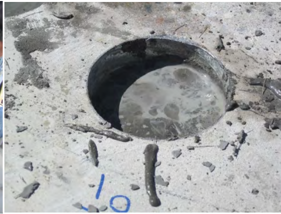
(b) Duct Filled w/ UHPC
