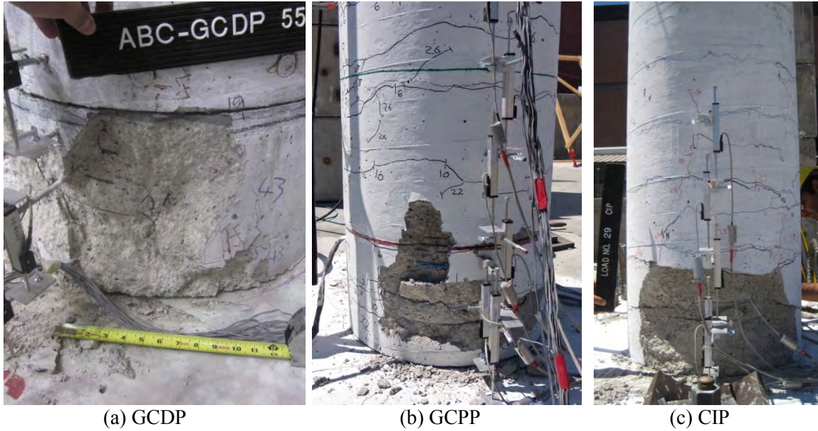
Figure B.7 GCDP, GCPP, and CIP Columns Plastic Hinge Damage after Full Cycles of 4.0% Drift
