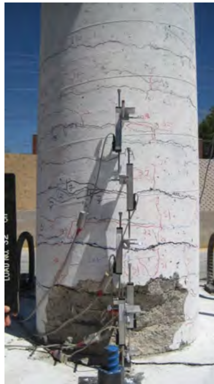
Figure 5.1- PNC (Left) and CIP (Right) Columns Plastic Hinge Damage at Second Push of 5% Drift
