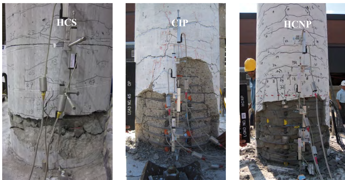
Figure 5.33- HCS, CIP, and HCNP Columns Plastic Hinge Damage at Second Pull of 10% Drift
