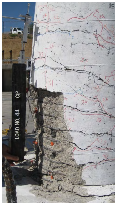
Figure 5.5- PNC (Left) and CIP (Right) Columns Plastic Hinge Damage at Last Push of 10% Drift
