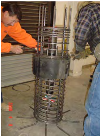
(a) Rubber Pad Placed in Steel Cage
