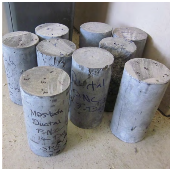
Figure 4.2- UHPC Compressive Mode of Failure
