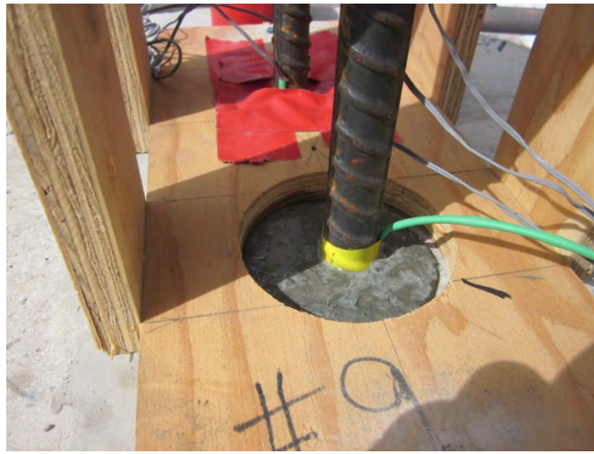
(b) Bar Frame for Double-Duct
