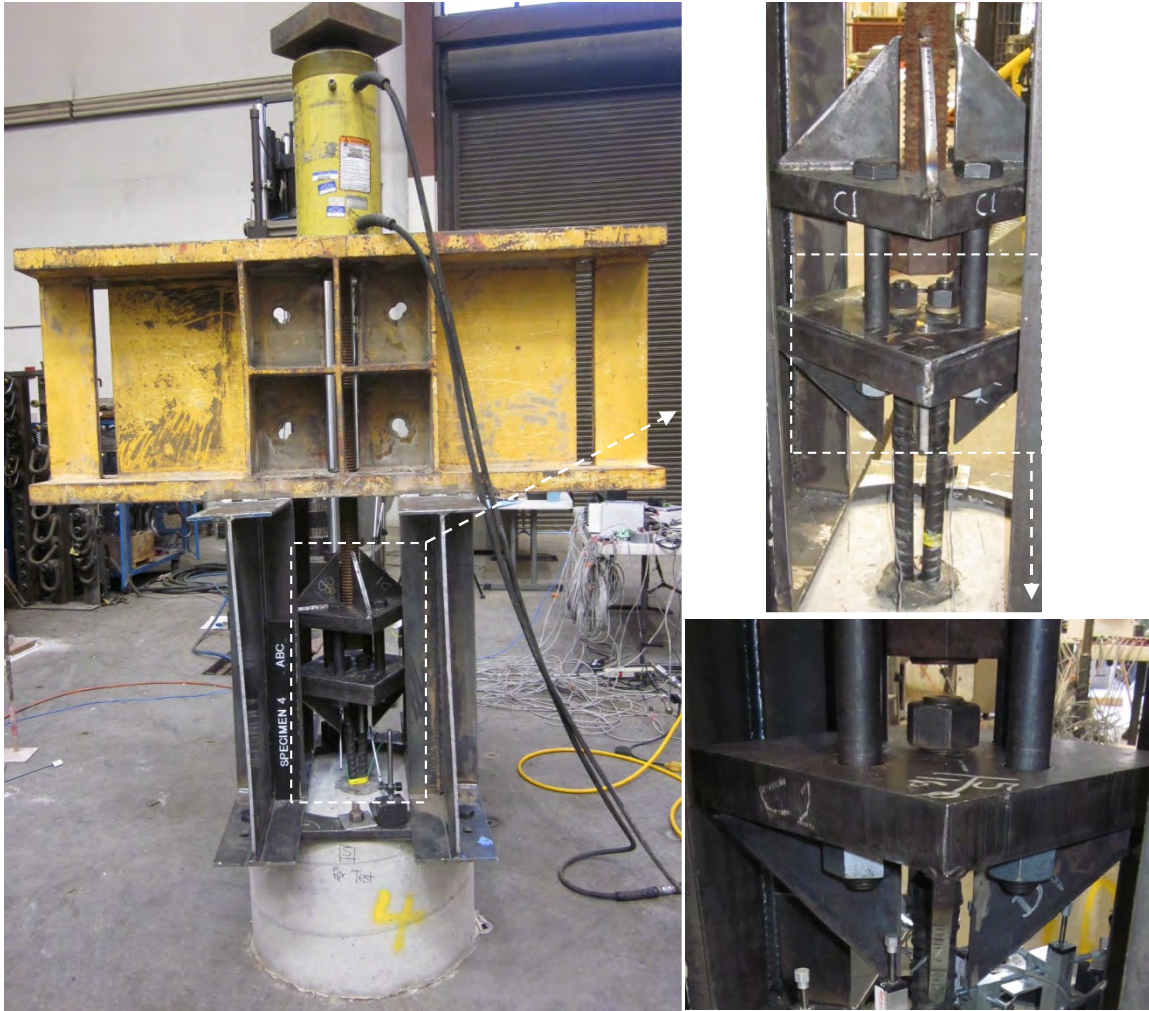
Figure 2.20- Photographs of Pullout Test Setup
