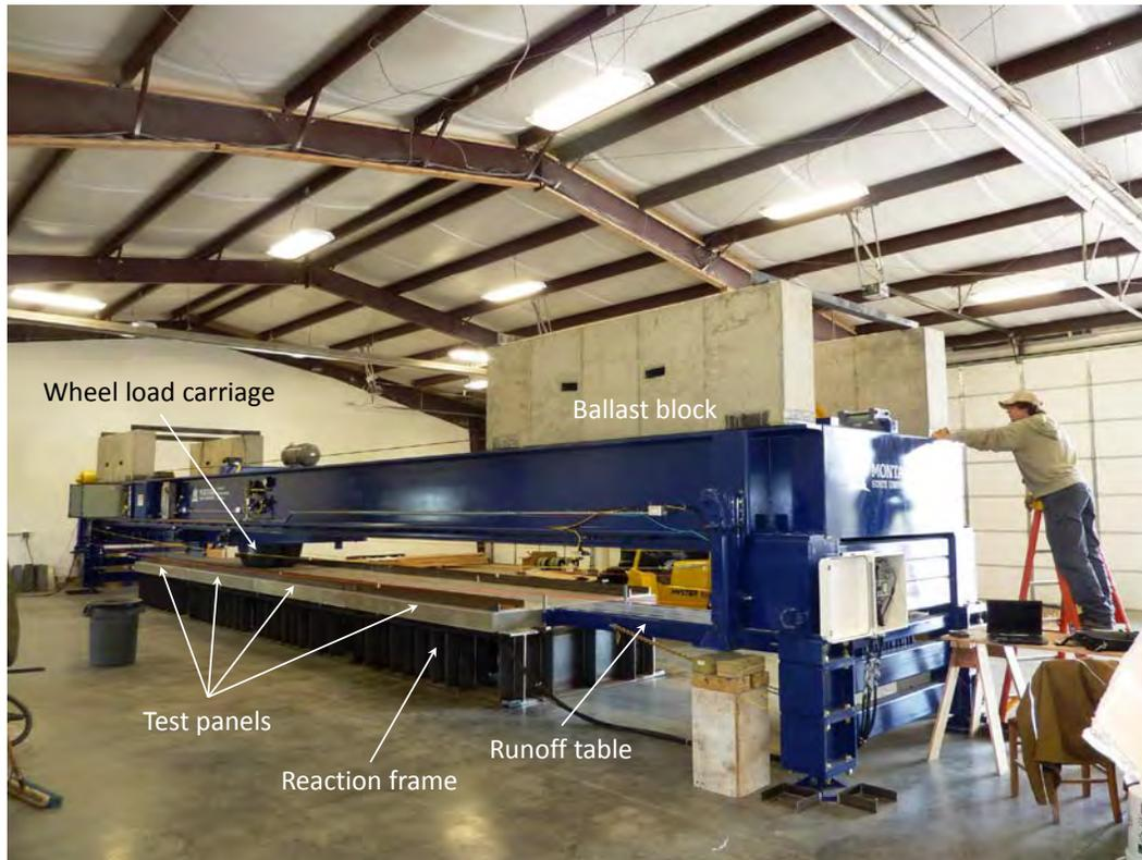
**Figure 14: Automated bridge deck tester.**
