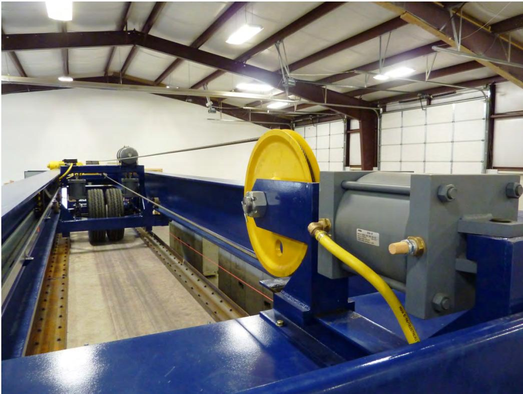
**Figure 23: Drive cable and carriage assembly.**
