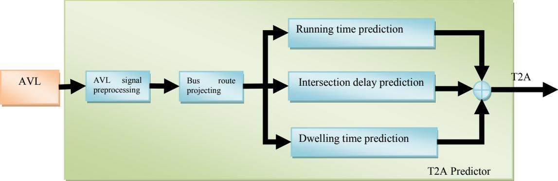
**Figure 1-7 Structure of an Integrated Time-to-Arrival Estimator**
