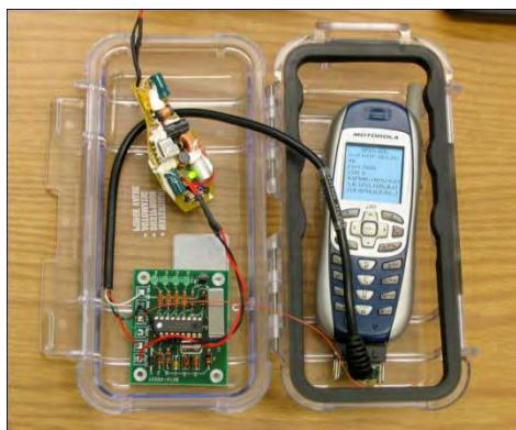
Figure 5-4 Cell-Phone based AVL System
