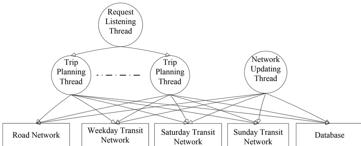
**Figure 2-14 The Architecture of the Trip Planning Server**
