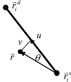
Figure 3-9 Projection of GPS Point onto Bus Route
