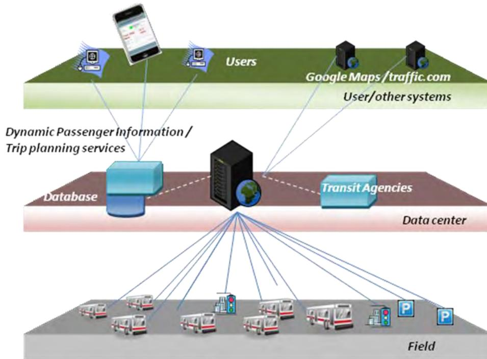
**Figure 2-8 System Components**
