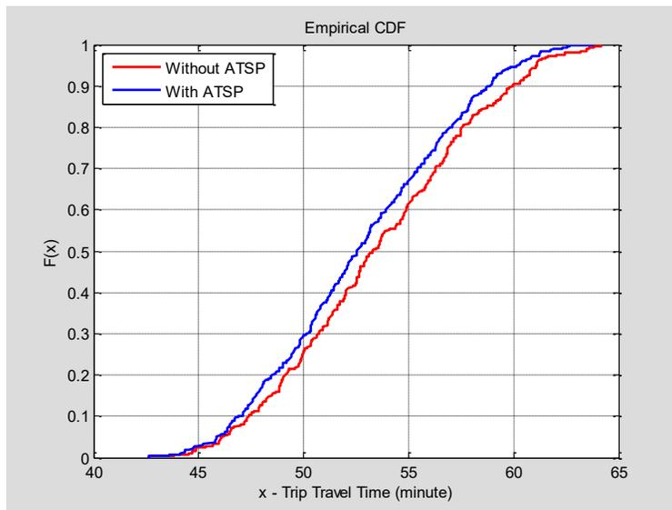
Figure A-2 Comparison of Bus Trip Time (Northbound)
