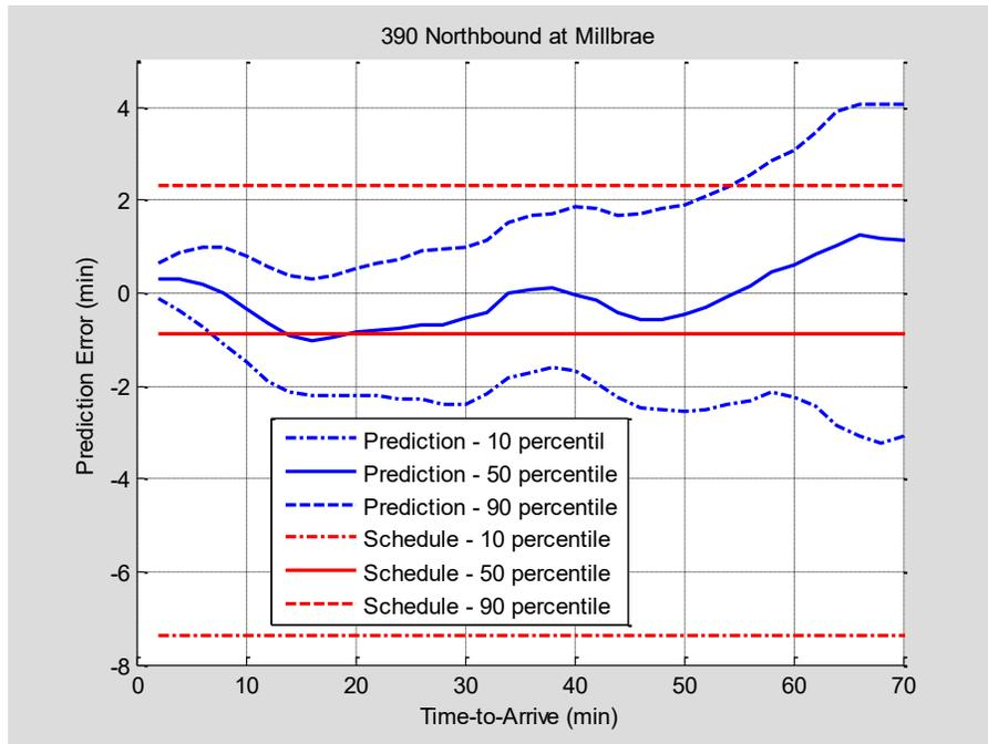
**Figure 5-10 Prediction Error vs. Actual Travel Time to Bus-Stop (Case 1)
