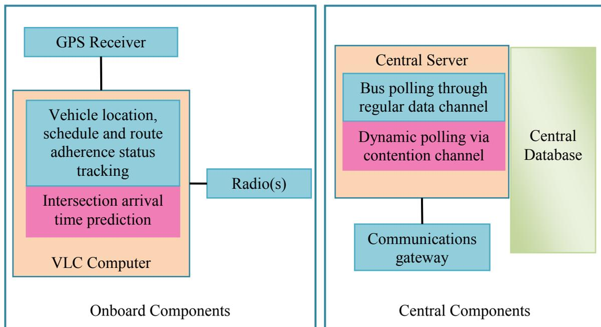
**Figure 4-1 AVL/ACS System Components for Integrated ATSP/DPI**
