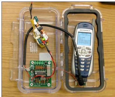
Figure 5-4 Cell-Phone based AVL System
