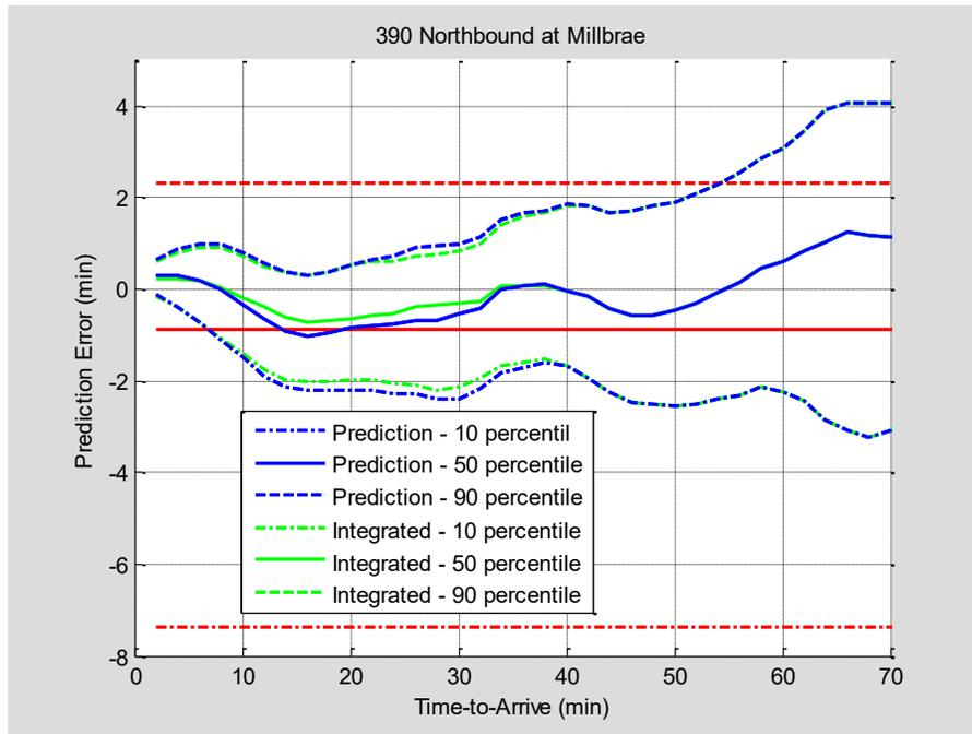
**Figure 5-11 Prediction Error vs. Actual Travel Time to Bus-Stop (Case 2)
