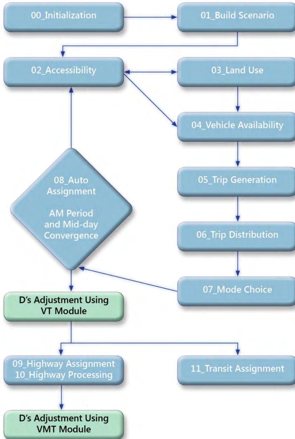
**Figure 14. Activity-Based TDF Model Flowchart**
