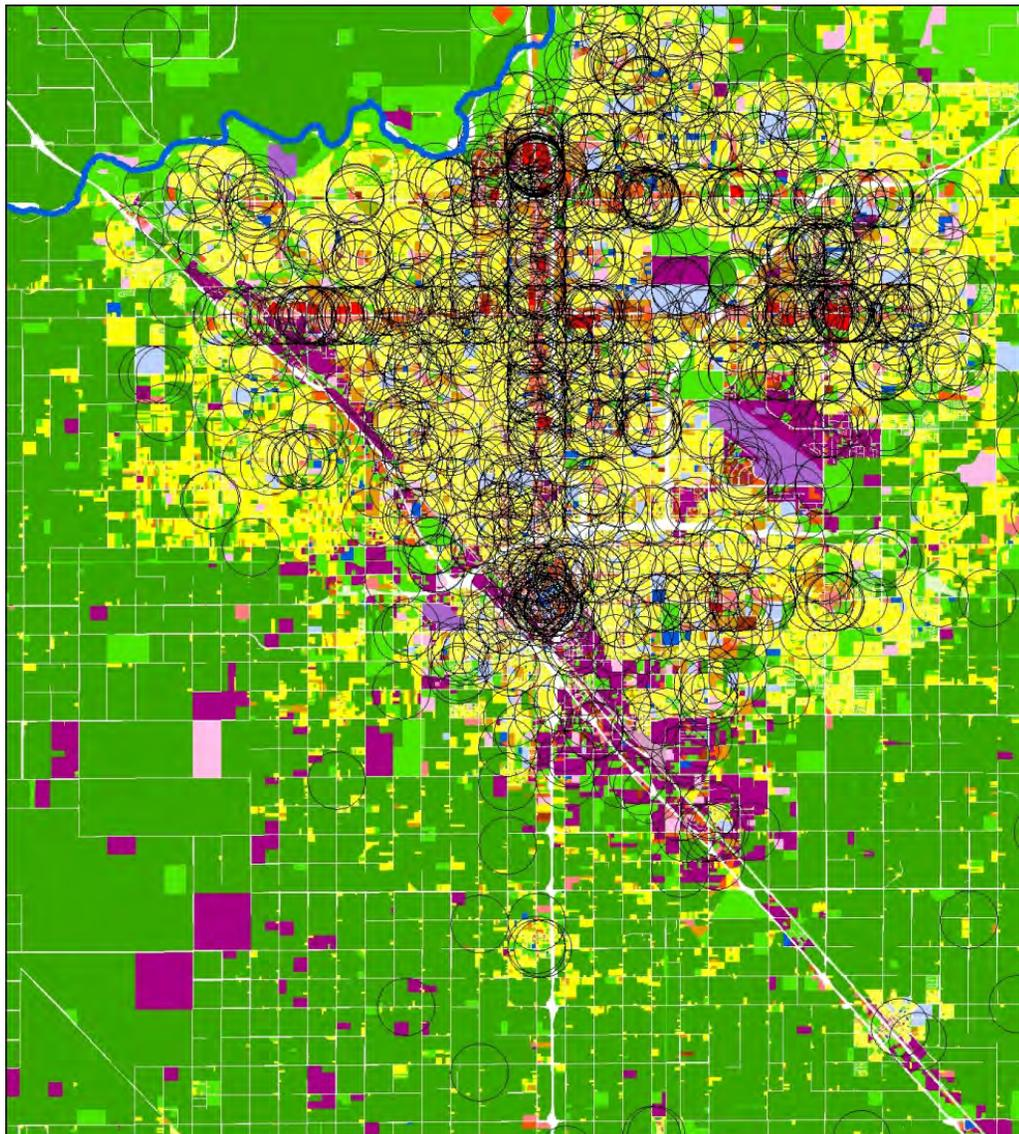
Figure 1. Fresno land cover (parcel based) with 804m buffer radii around trip end locations
