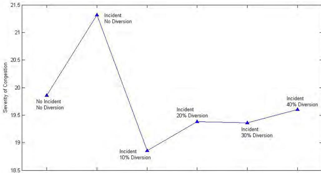
Figure 9-21: Severity of congestion for different diversion rates
