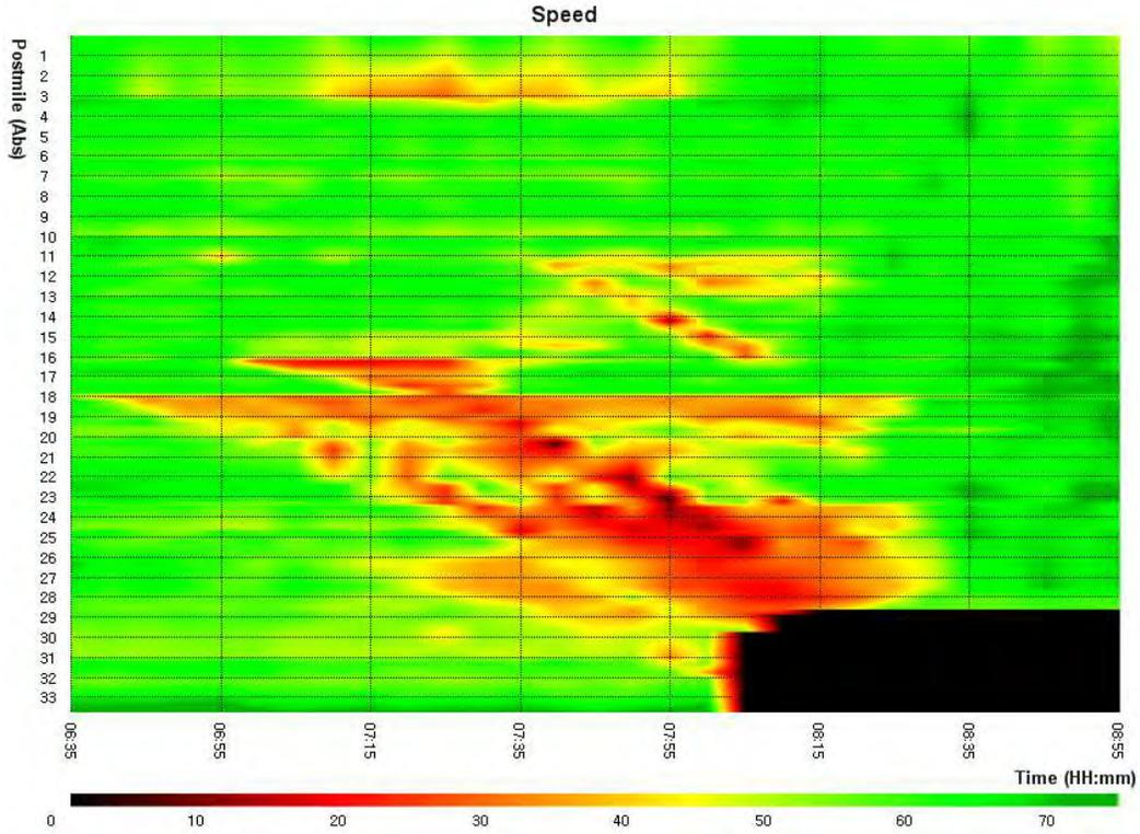
Figure 16-3: Speed contour for I-880: Incident and 30% diversion
