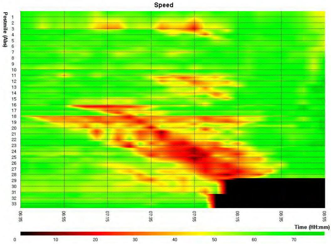
Figure 16-5: Speed contour for I-880: incident and 20% diversion and familiarity 5
