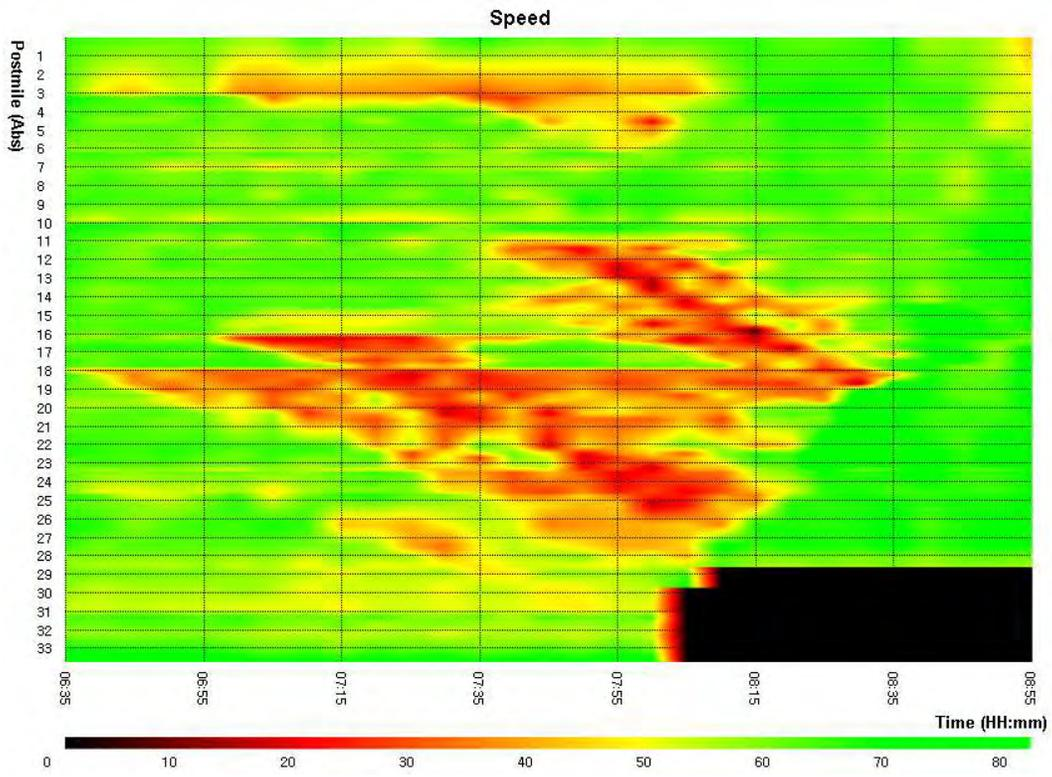
Figure 16-10: Speed contour for I-880: Incident and 30% diversion and familiarity 20
