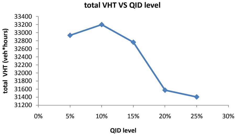
Figure 9-15: Average vehicle-hour-traveled for different QID levels
