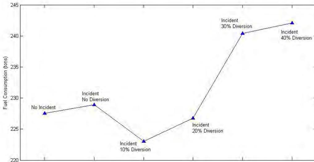
Figure 9-25: Fuel consumption for different CMS diversion rate
