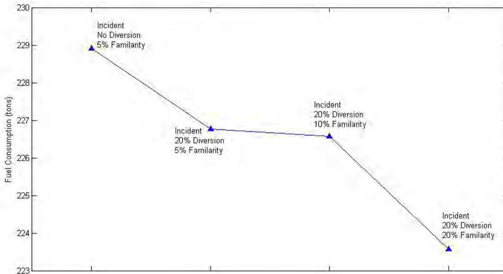
Figure 9-27: Fuel consumption for different QID level self-diversion
