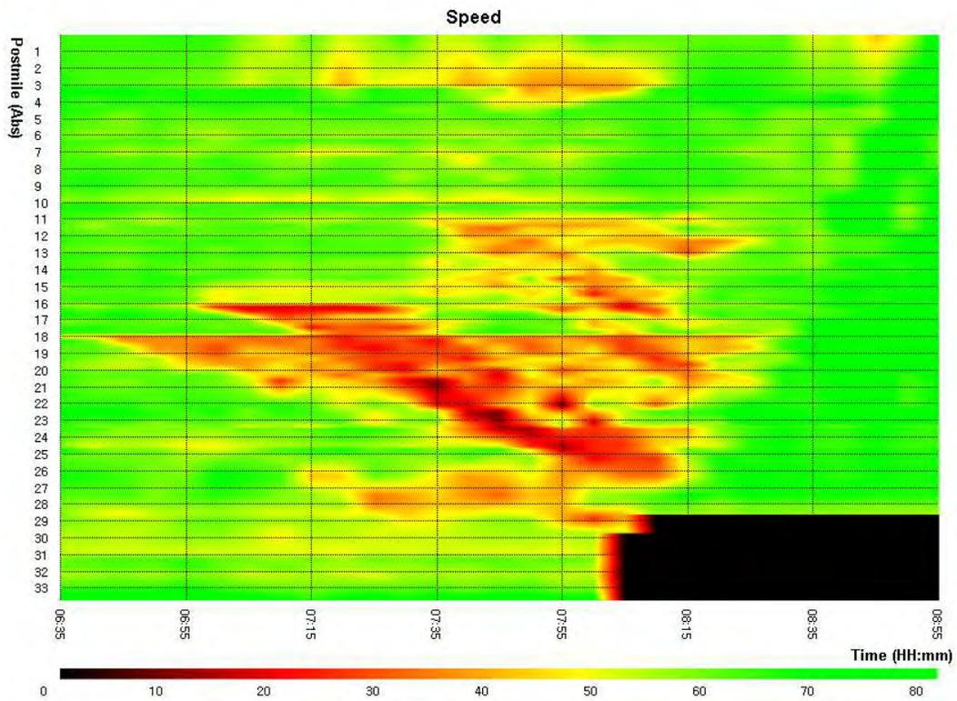
Figure 9-19: Speed contour for I-880, Scenario 4: Incident and 20% QID
