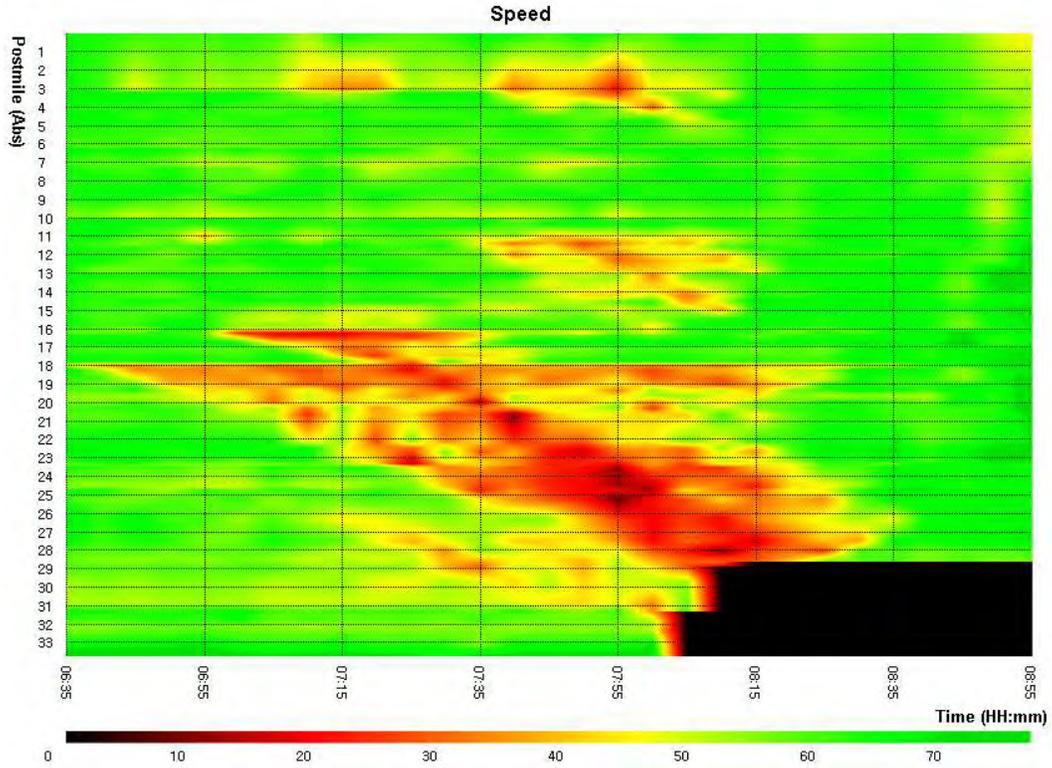
Figure 9-18: Speed contour for I-880, Scenario 3: Incident and 20% diversion
