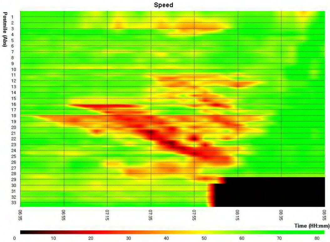
Figure 16-11: Speed Contour for I-880: Incident and no diversion and familiarity 20
