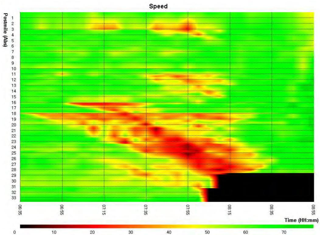
Figure 16-2: Speed contour for I-880: Incident and 20% diversion
