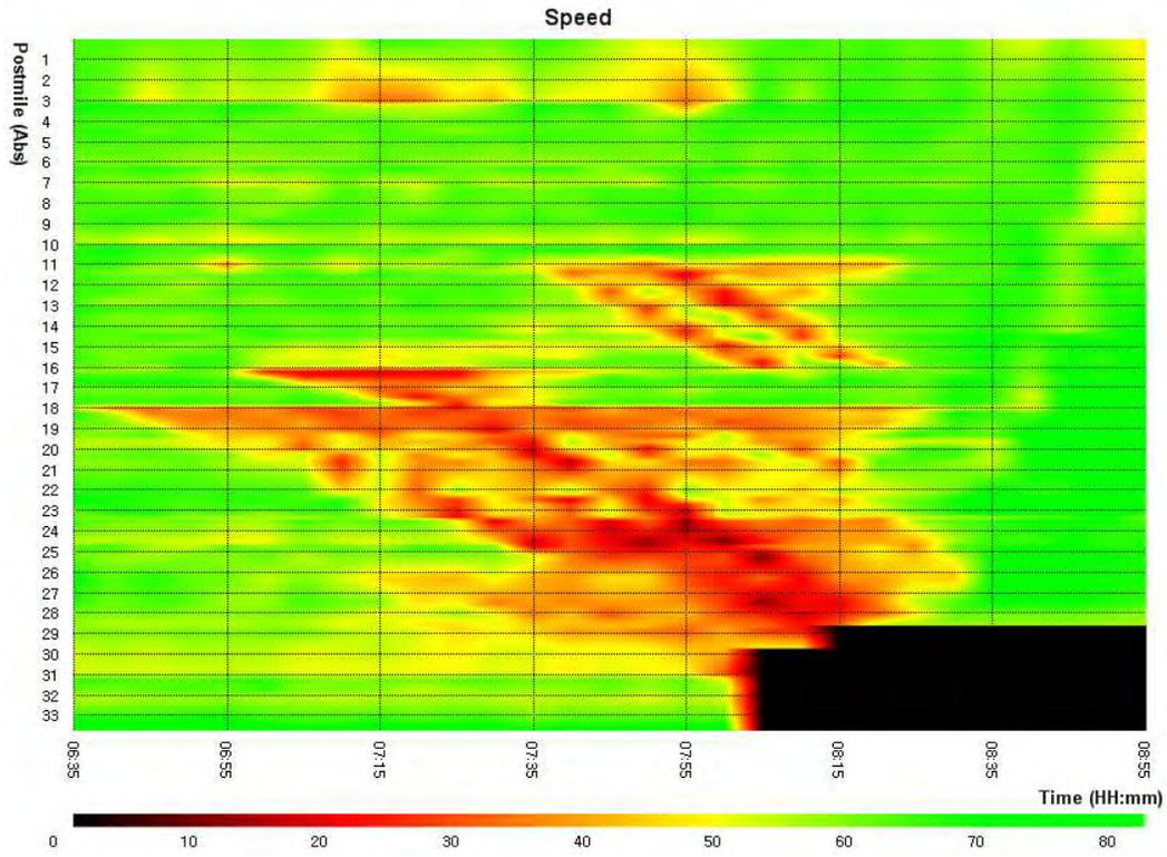
Figure 16-4: Speed Contour for I-880: Incident and 40% diversion
