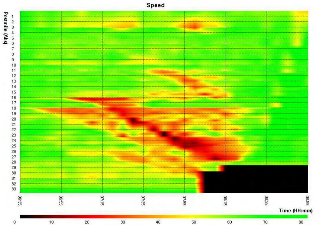
Figure 16-6: Speed contour for I-880: Incident and 20% diversion and familiarity 10
