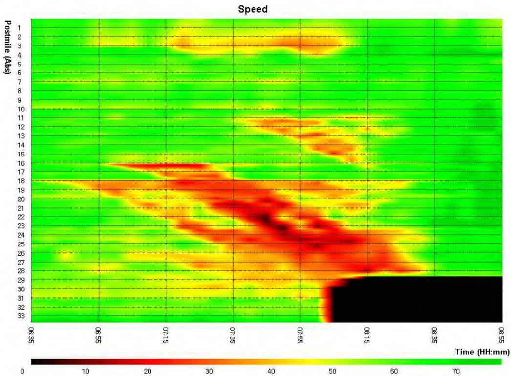
Figure 9-17: Speed contour for I-880, Scenario 2: Two-lane-closure incident
