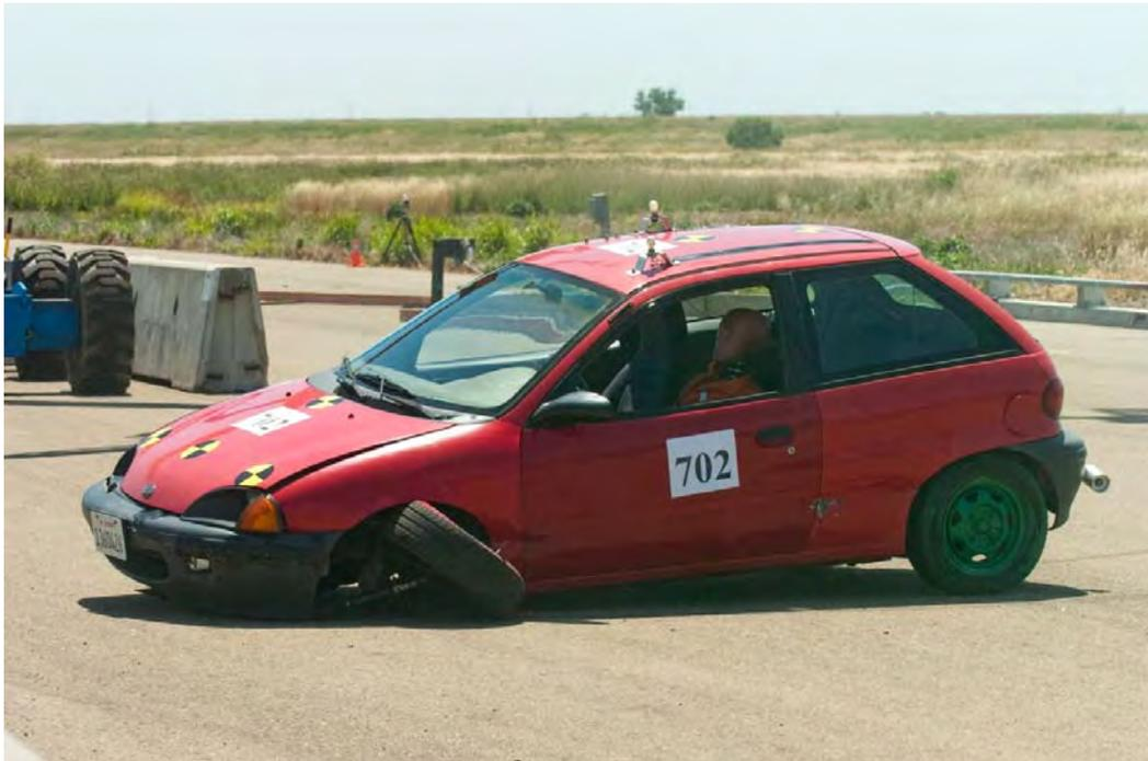
Figure 3-12. Test 702 Side Damage
