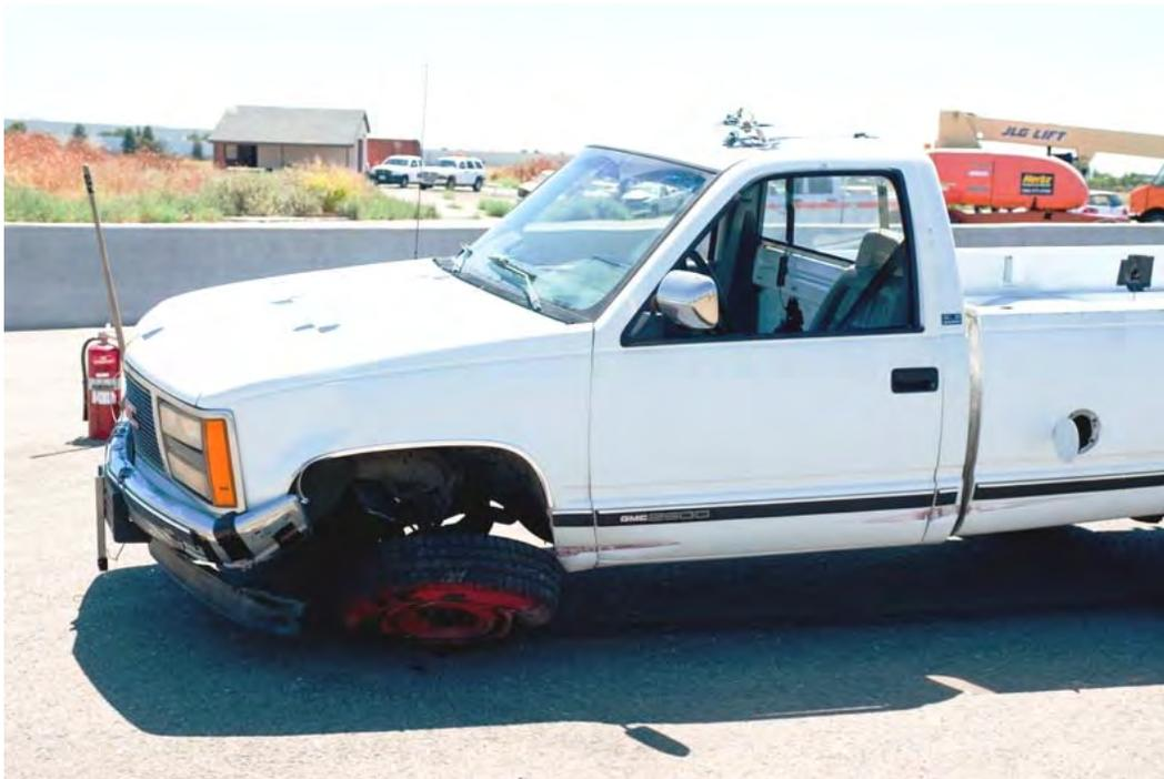
Figure 3-4. Test 701 Front Left Damage
