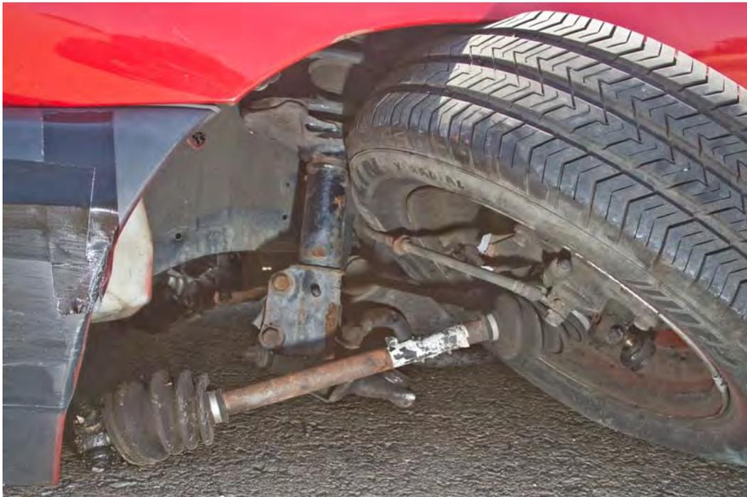
**Figure 3-14. Test 702 Front Left Wheel Damage**
