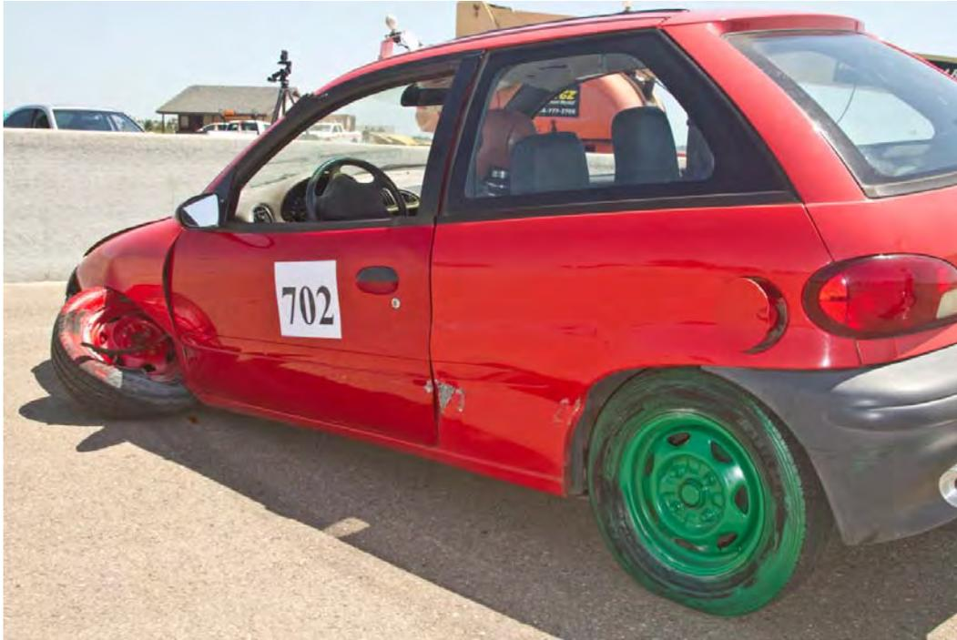
**Figure 3-13. Test 702 Rear View Side Damage**
