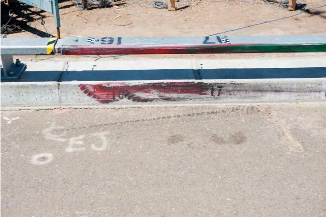
Figure 3-2. Test 701 - Front Wheel (red) / Rear Wheel (green)
