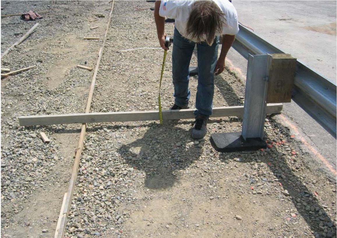
Figure 2-10 – Checking CRMCrete Depth for Test 658
