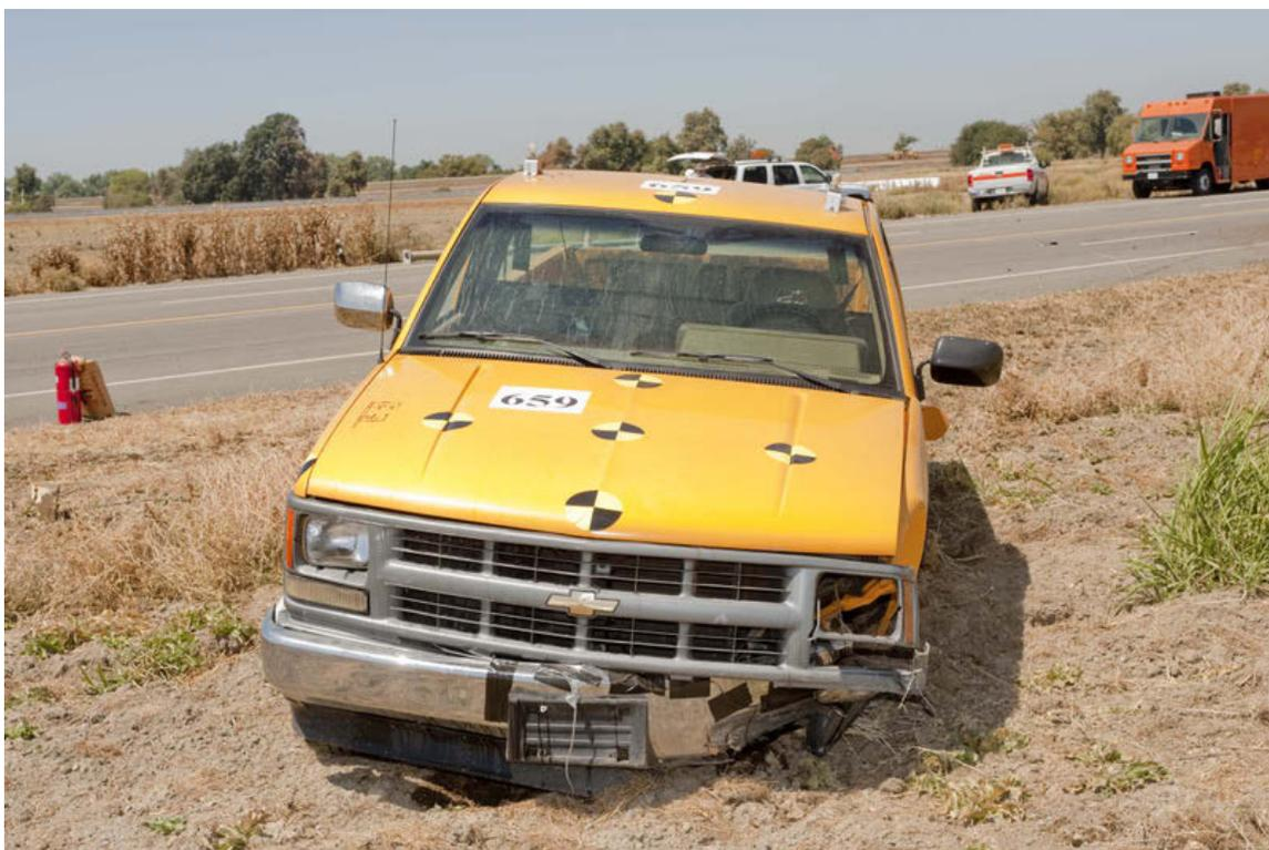
Figure 2-37 – Front of Test Vehicle after Test 659
