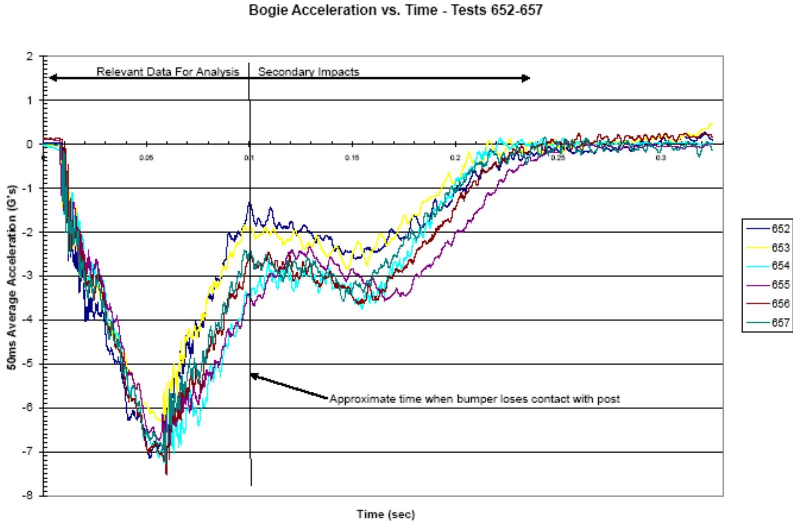
Figure 7-10 – Longitudinal Bogie Acceleration vs. Time
