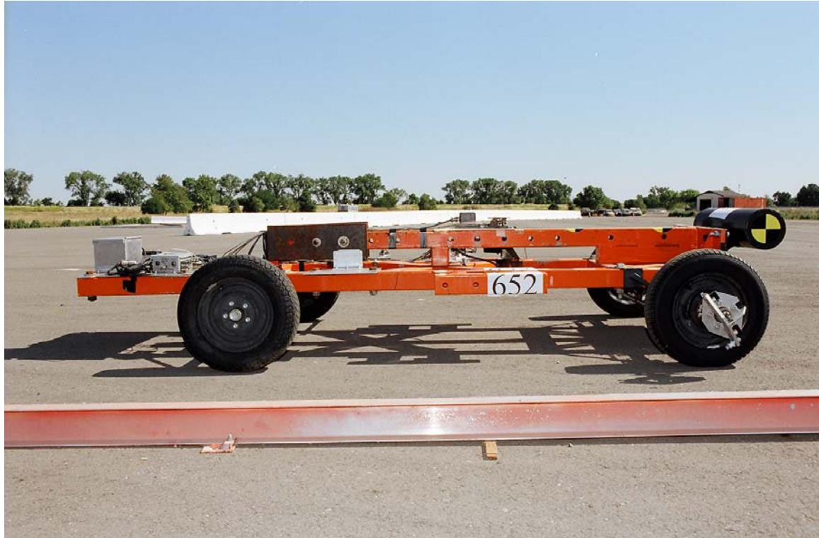
Figure 2-1 – Lightweight Bogie
