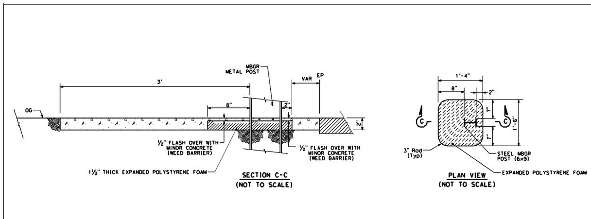
Figure 2-25 – Test 659 Post Leave-out Plan and Cross Section
