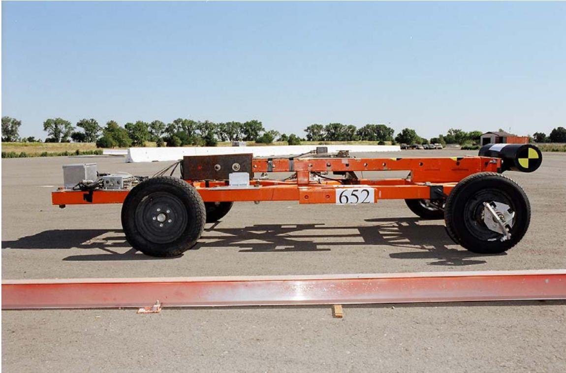
Figure 2-1 – Lightweight Bogie
