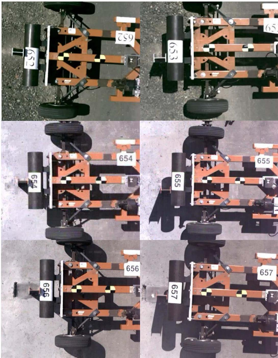
Figure 2-8 – Bogie Tests at Impact
