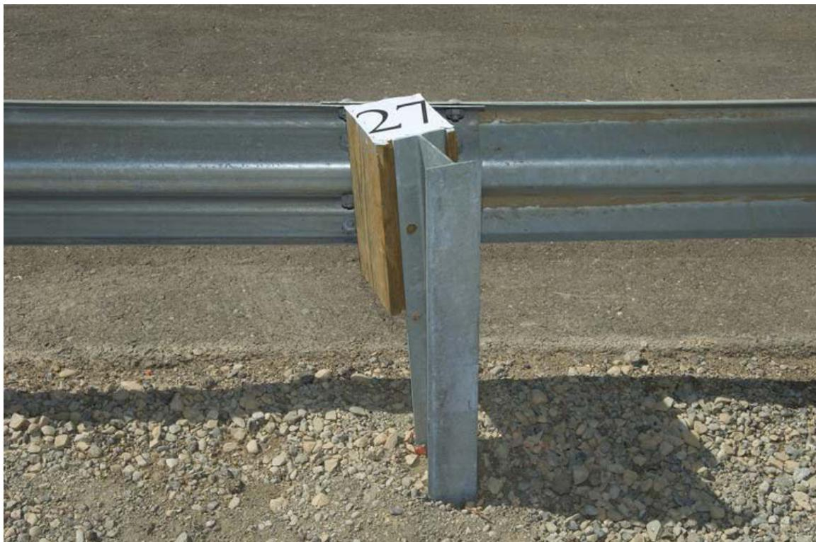
Figure 2-23 – Typical Twisted Post after Test 658
