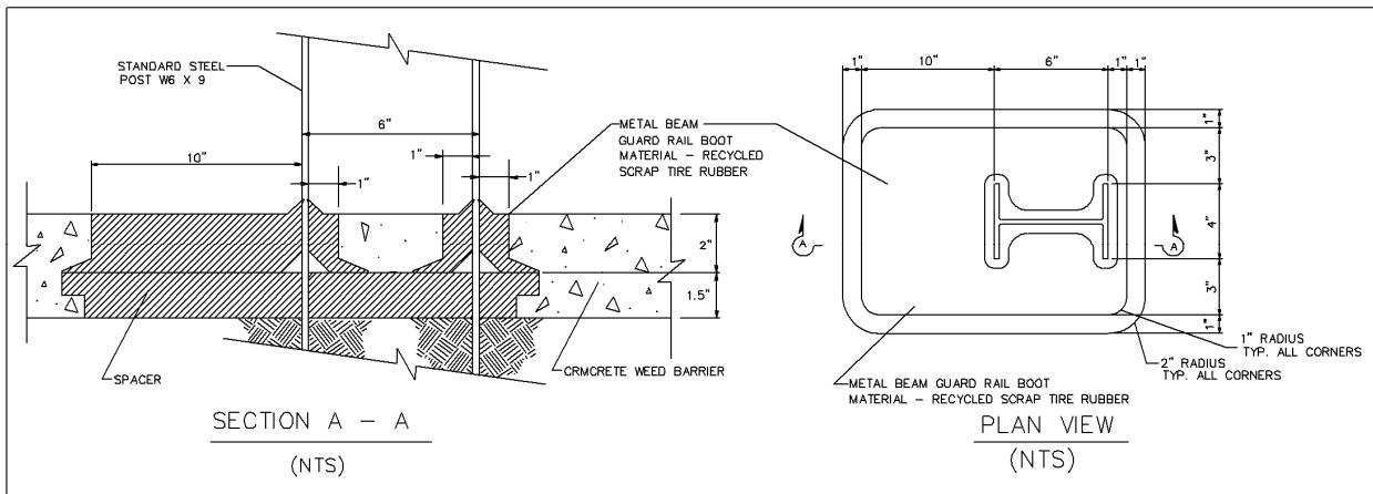
Figure 2-3 – CRMCrete Boot Details for Tests 656 and 657
