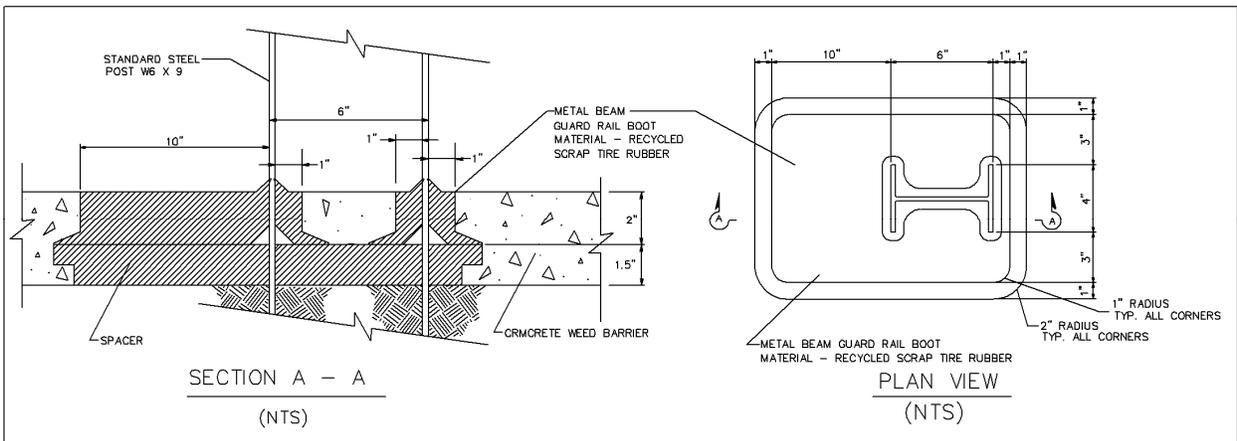
Figure 2-3 – CRMCrete Boot Details for Tests 656 and 657
