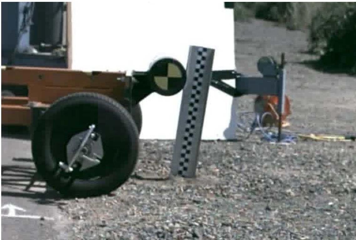
Figure 2-7 – Typical Bogie Impact – Side View
