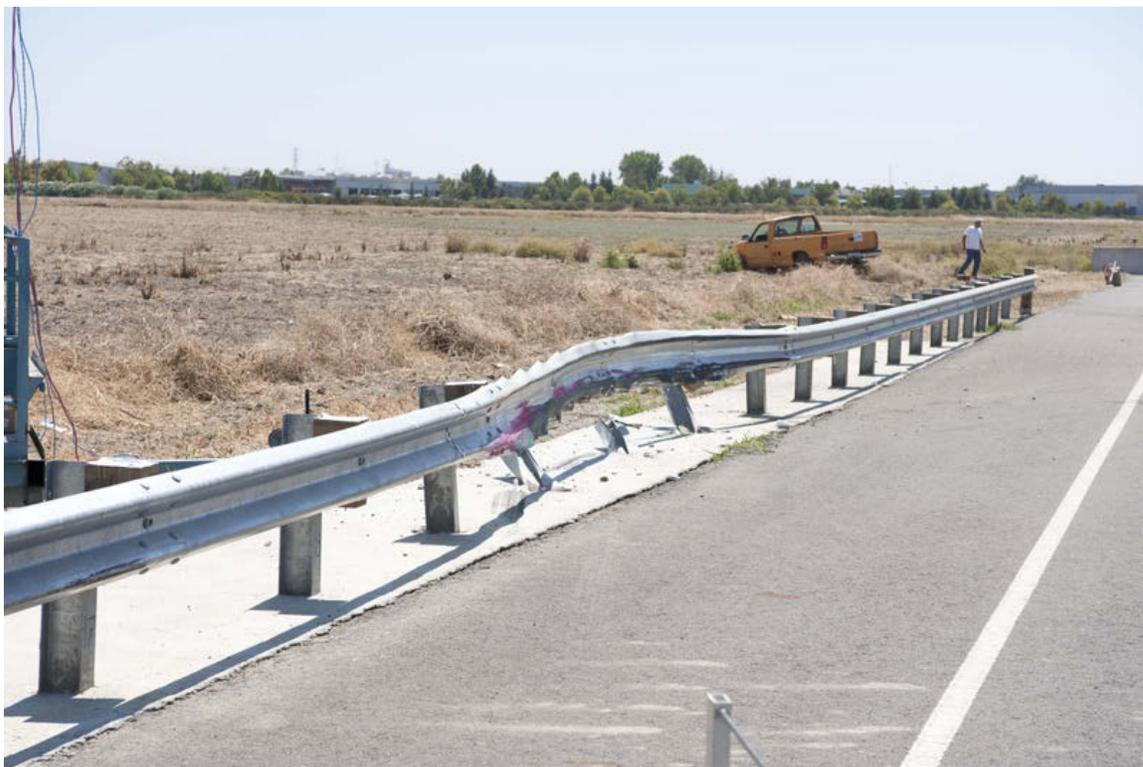
Figure 2-38 – Test Article Overview after Test 659
