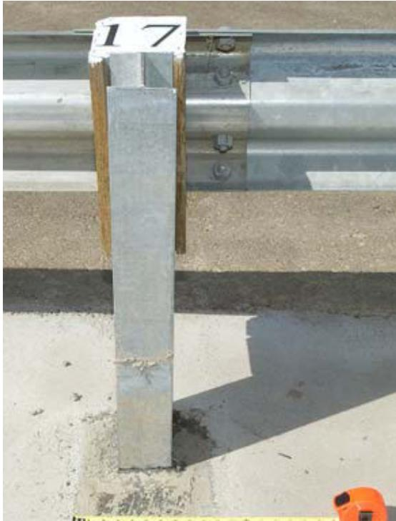
Figure 2-13 – Test 658 Leave-out Area on Sides of Post
