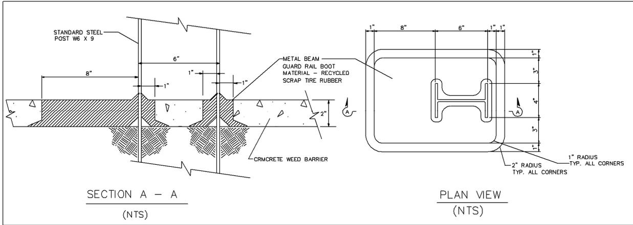
Figure 2-2 – CRMCrete Boot Details for Tests 654 and 655
