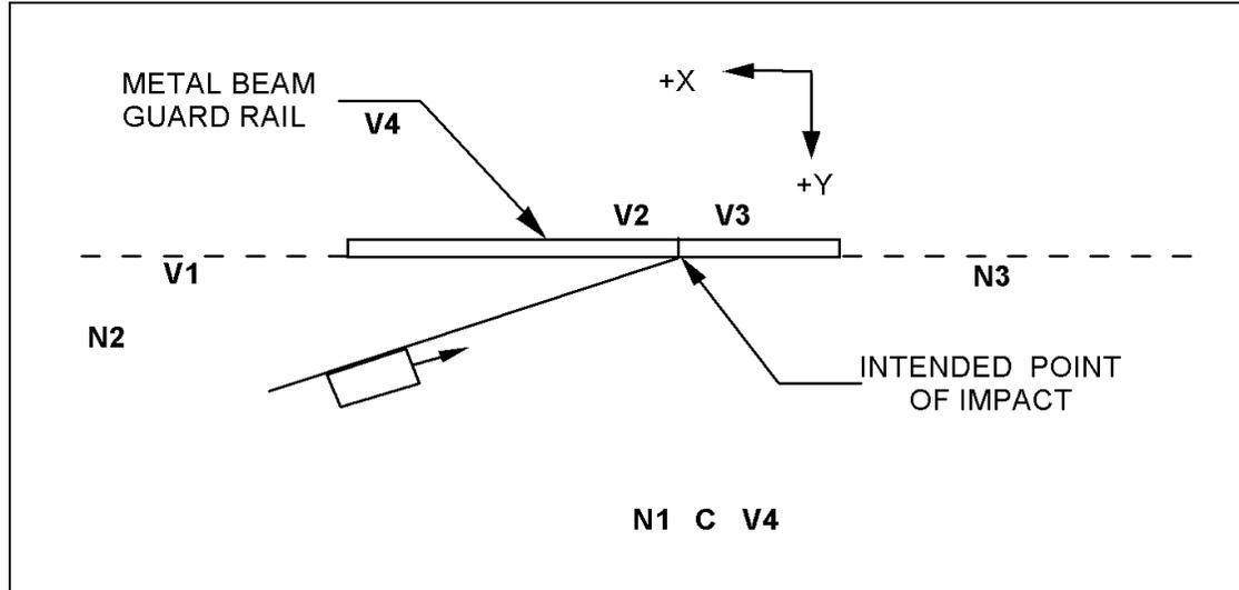
Figure 7-1 – Camera Locations for Test 659
