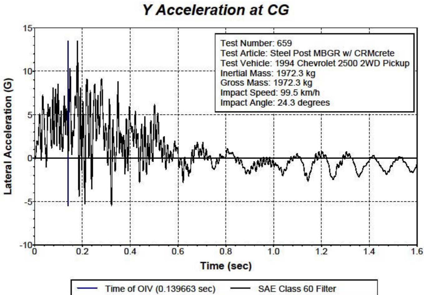
Figure 7-5 – Test 659 Vehicle Y (Lateral) Acceleration Vs Time
