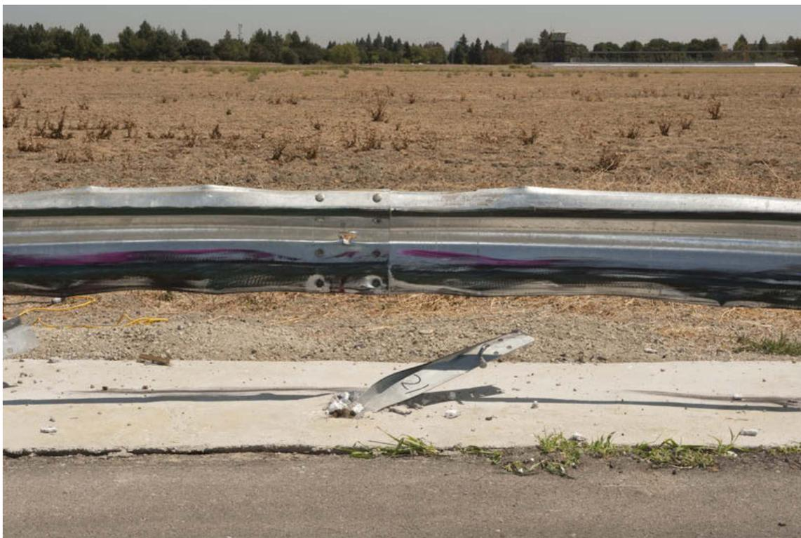
Figure 2-40 – Post 21 (Downstream of Impact Point) after Test 659
