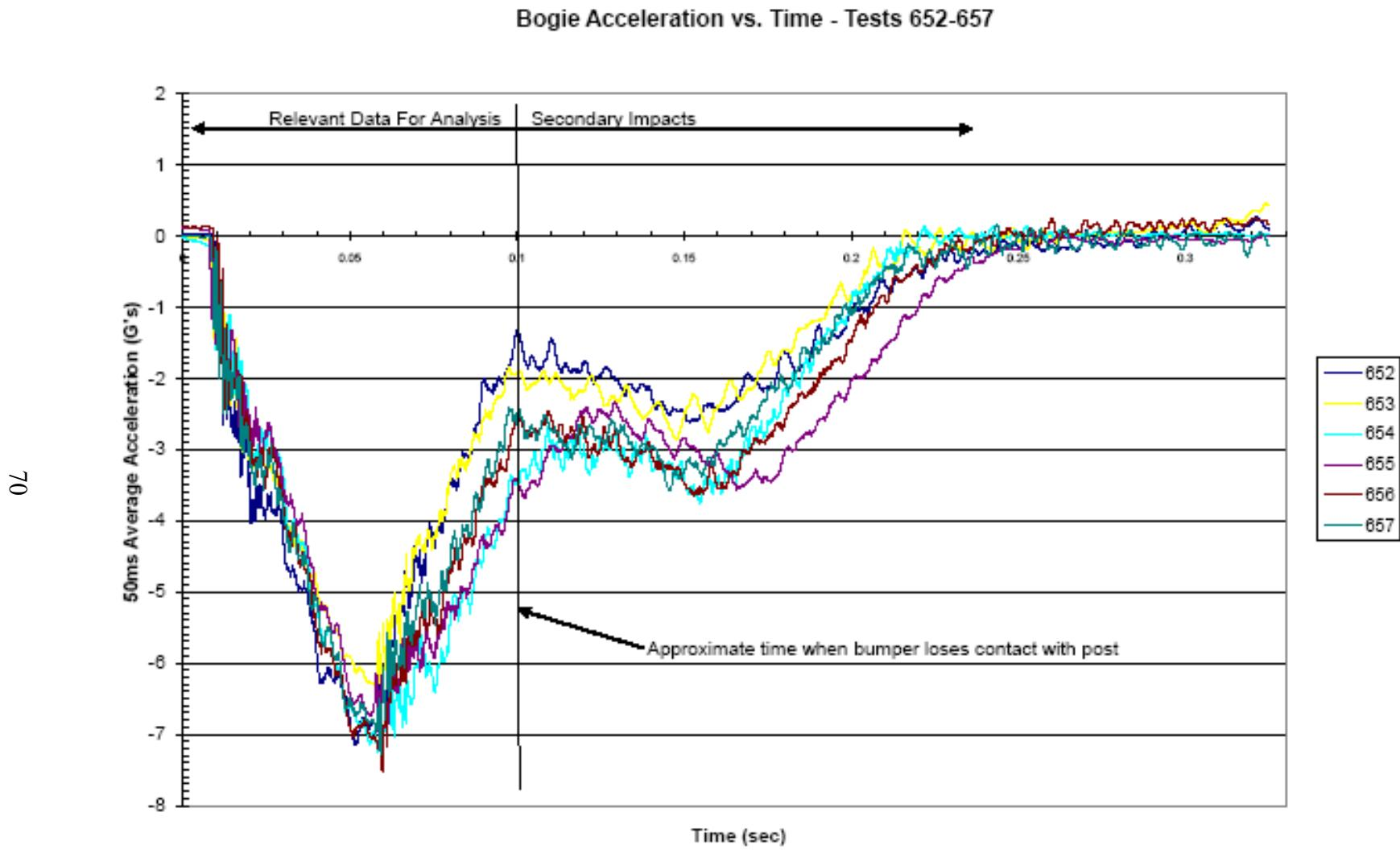
Figure 7-10 – Longitudinal Bogie Acceleration vs. Time
