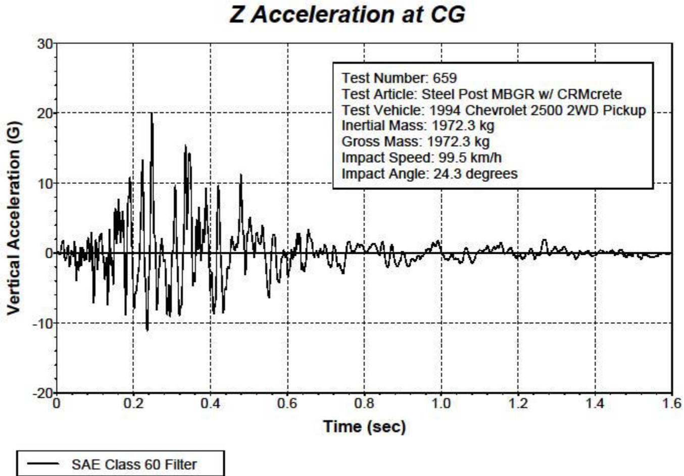
Figure 7-6 – Test 659 Vehicle Z (Vertical) Vs Time
