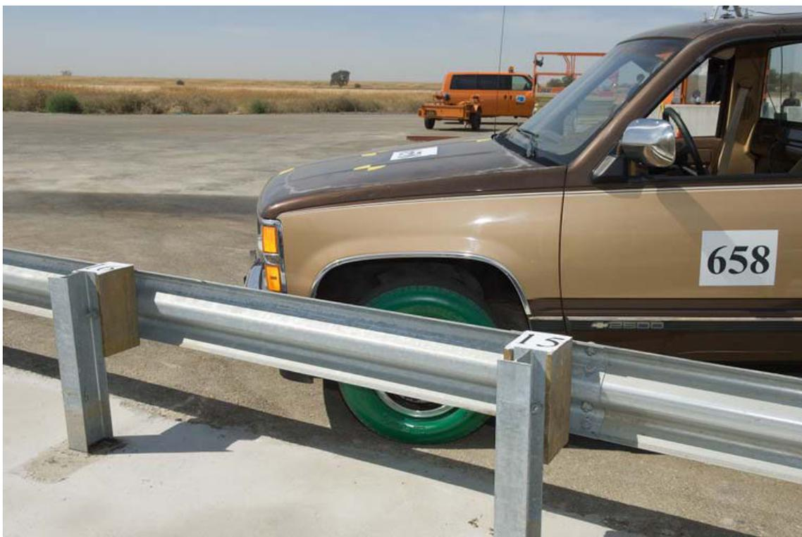
Figure 2-17 – Impact Point for Test 658
