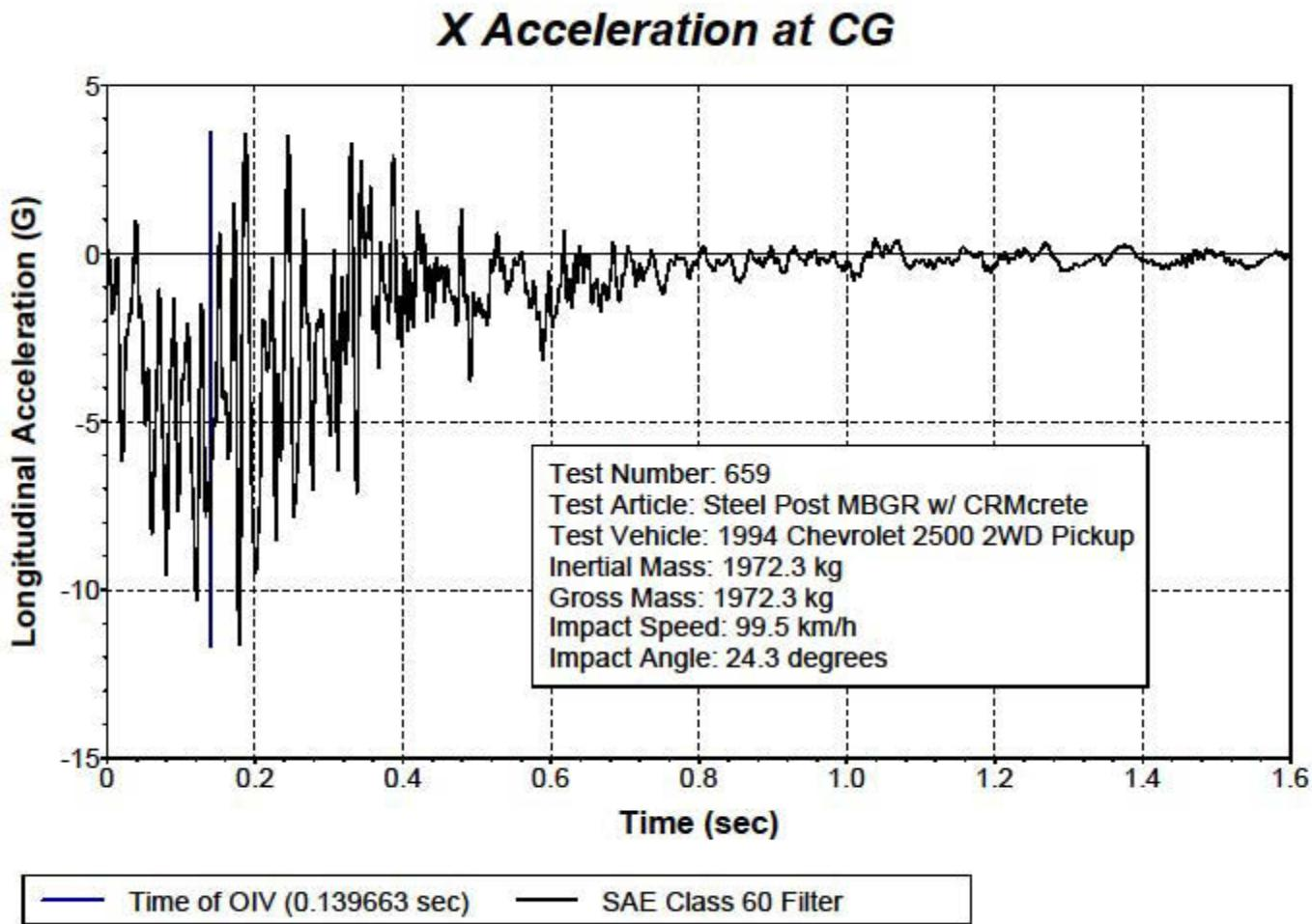
Figure 7-4 – Test 659 Vehicle X (Longitudinal) Acceleration Vs Time
