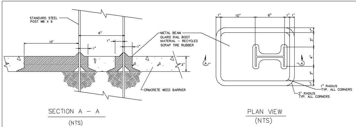
Figure 2-9 – CRMCrete Boot Details for Test 658
