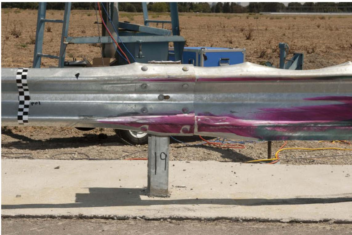
Figure 2-39 – Impact Point after Test 659
