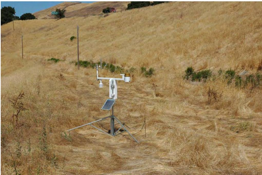
Figure 4. Evaporation measurement station at Contra Costa highway 4.
