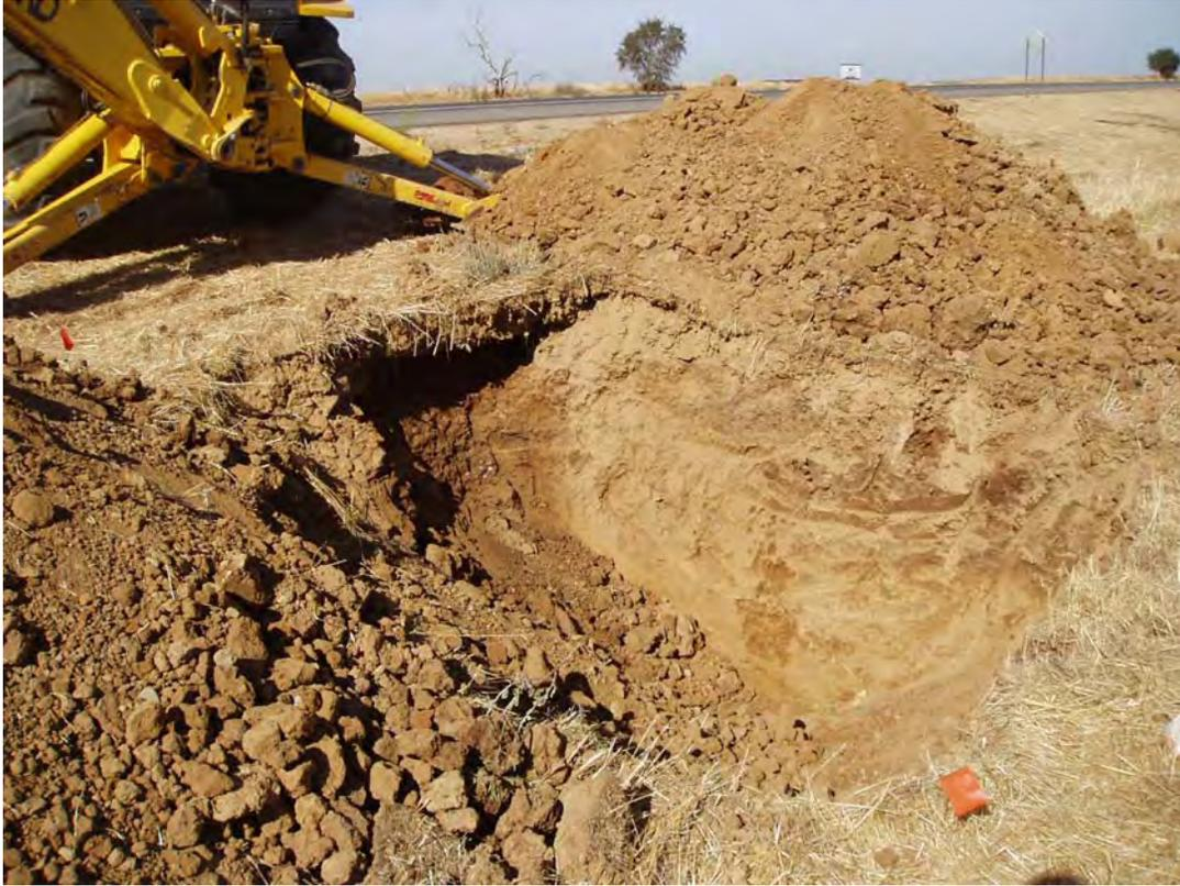
Figure 5. Compacted surface layer of Yuba SR 70 substrate that forms an overhanging ledge (nearest backhoe) and sheets water off the site during rains.
