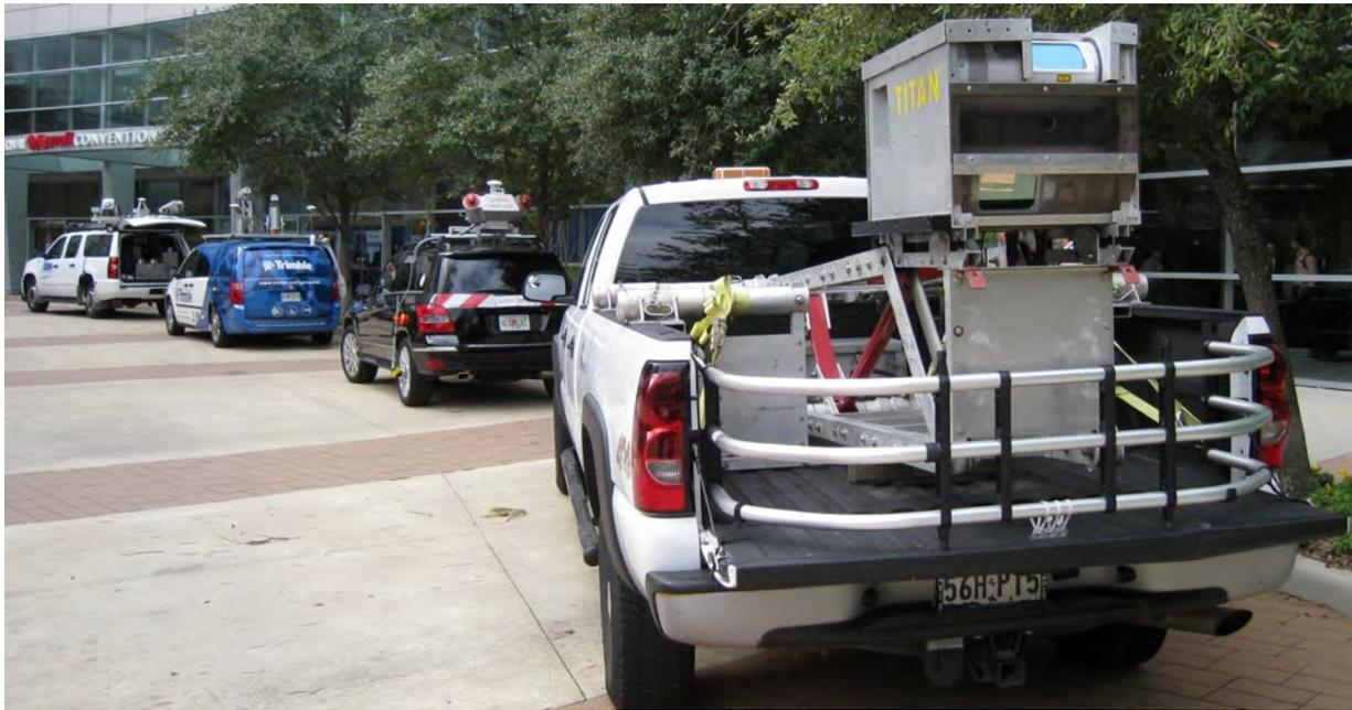
Figure 5.1: Commercial mobile LiDAR systems.
