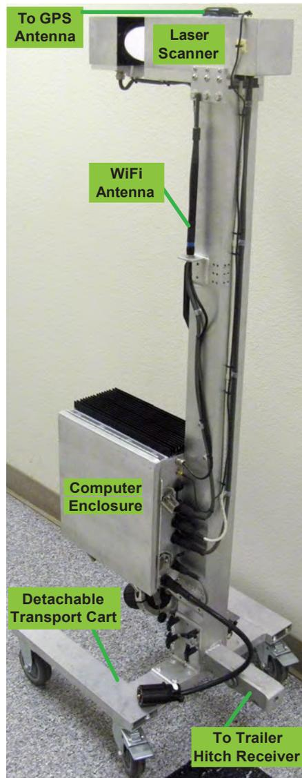
Figure 3.1: The second-generation profile sensing system.
