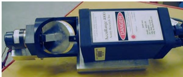
Figure 3.3: The scanning laser rangefinder.
