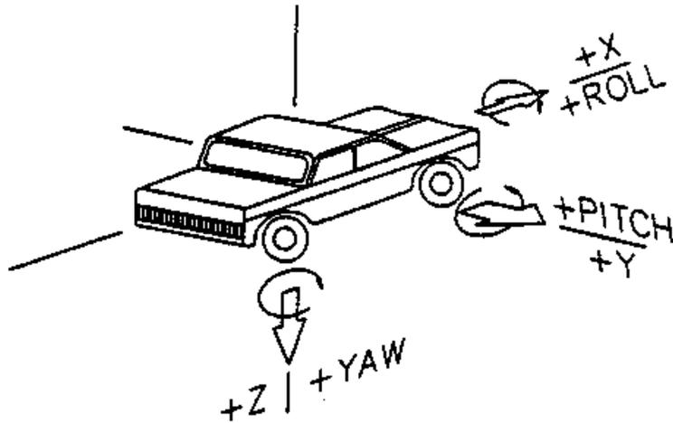
Figure 7-3 Vehicle Accelerometer Sign Convention
