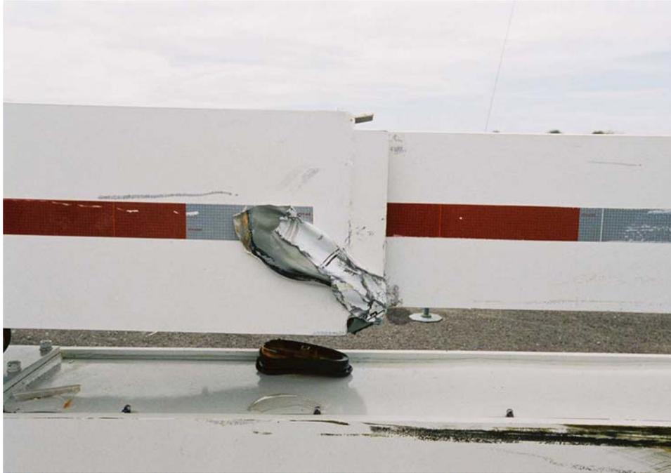
**Figure 2-18 Barrier After Test 641**
