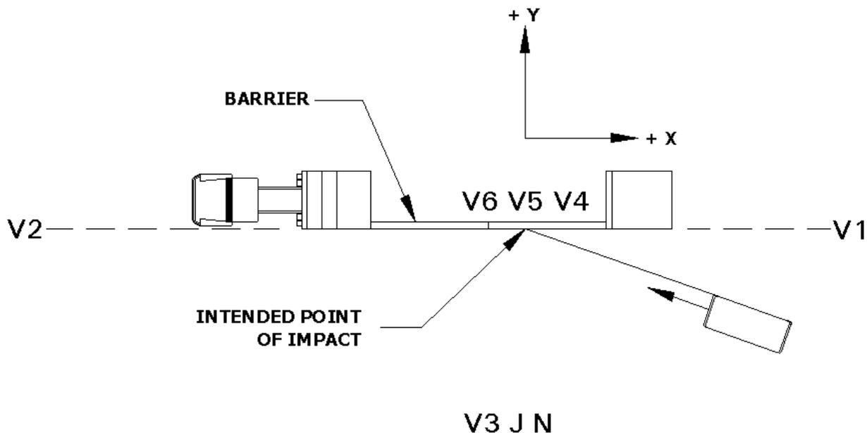
**Figure 7-2 Camera Locations Test 641 (Not to Scale)**
