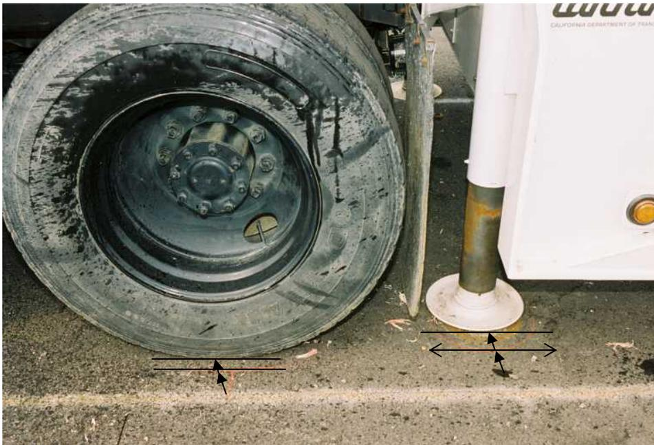
**Figure 2-32 Trailer Tire and Brace Displacement in Test 642**
