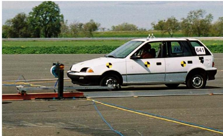
**Figure 7-1 Vehicle Guidance System**
