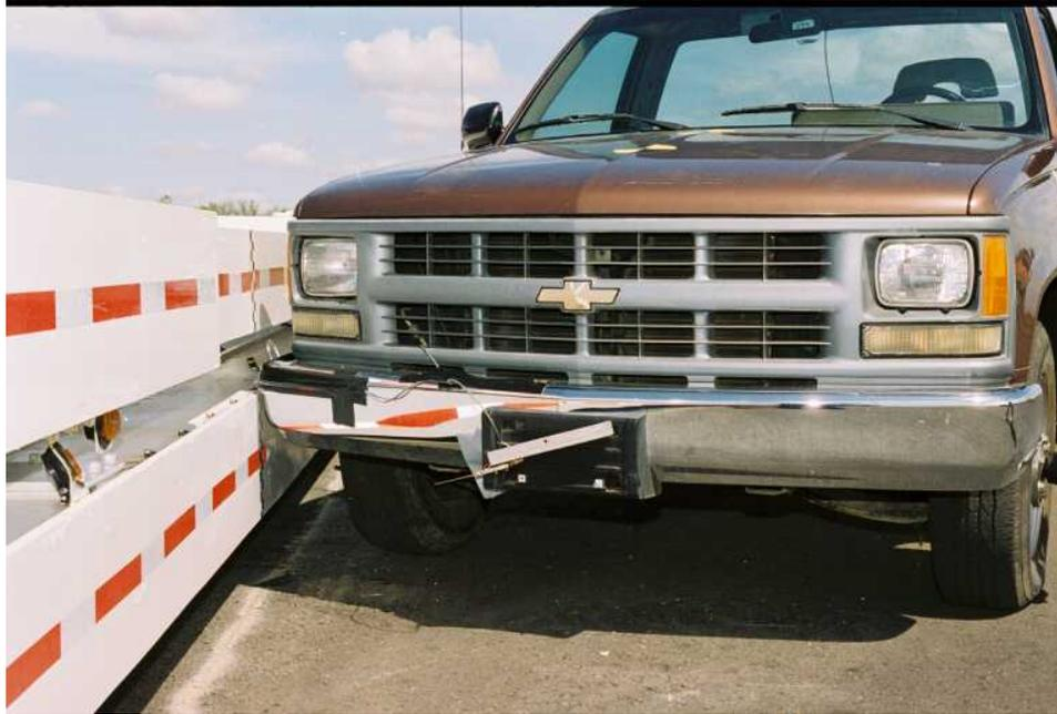
**Figure 2-23 Close-up of Impact Area Prior to Test 642**
