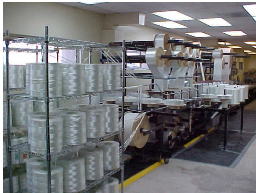
Figure 20 Global view of the Pultrusion Setup
