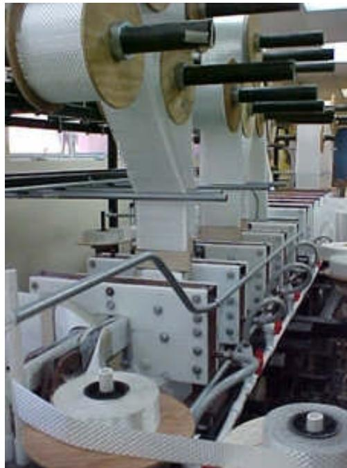
Figure 21 Detail of fiber Dispensing
