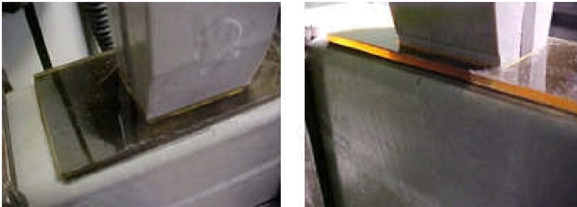
Figure 36 Photostress method Applied to Composite Snap-Fit
