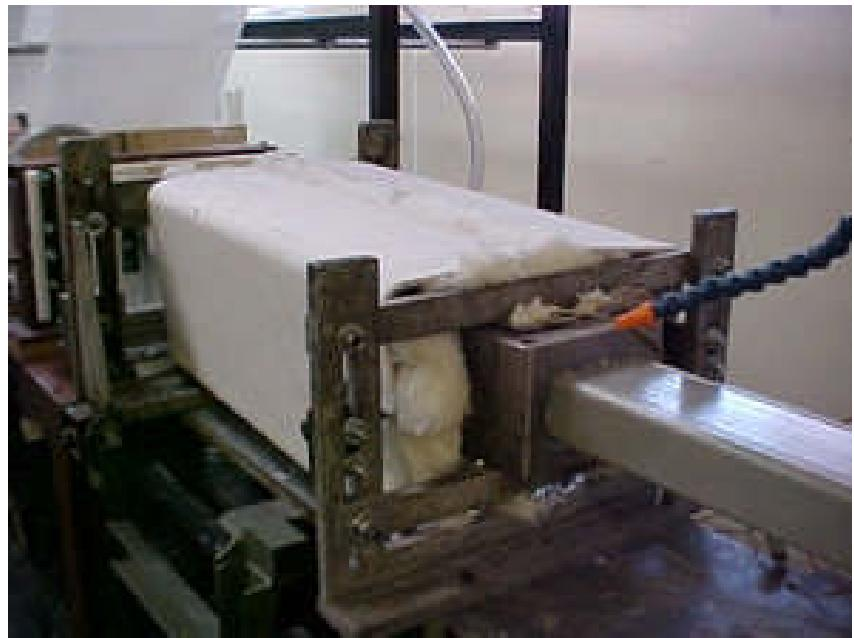
Figure 22 Pultruded Component Exiting the Die
