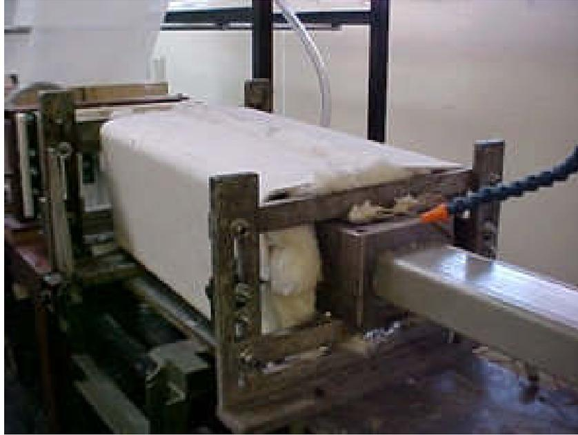
Figure 22 Pultruded Component Exiting the Die
