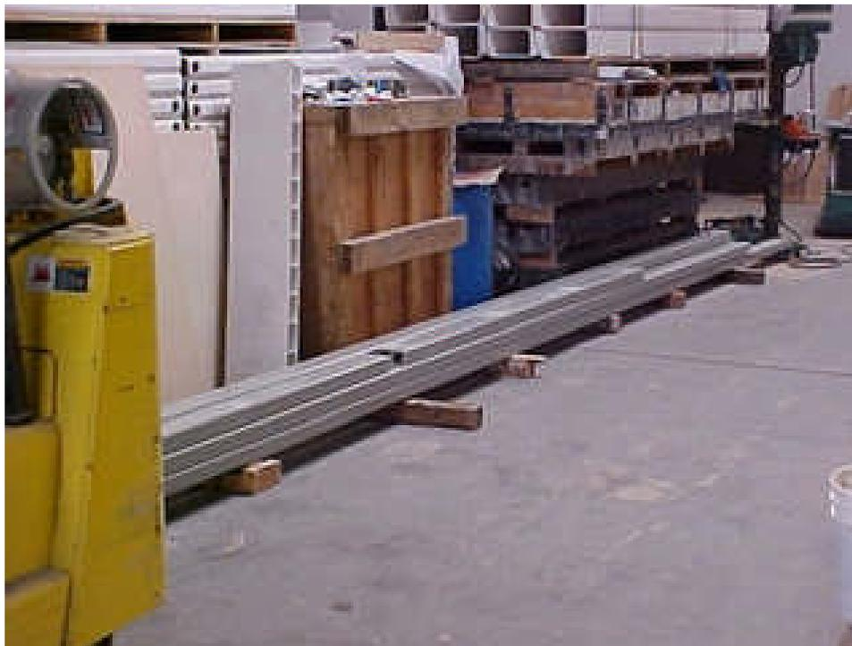
Figure 23 Finished Pultrusions
