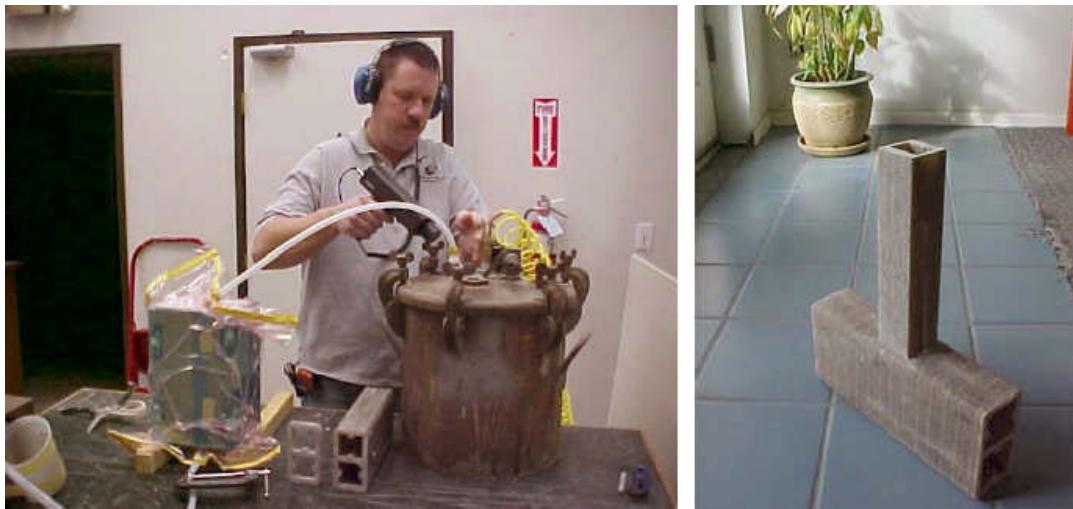
Figure 16 a, b Snap-joint infusion and finished snap joint assembly
