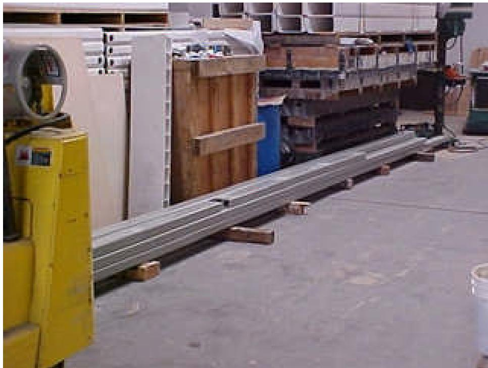
Figure 23 Finished Pultrusions
