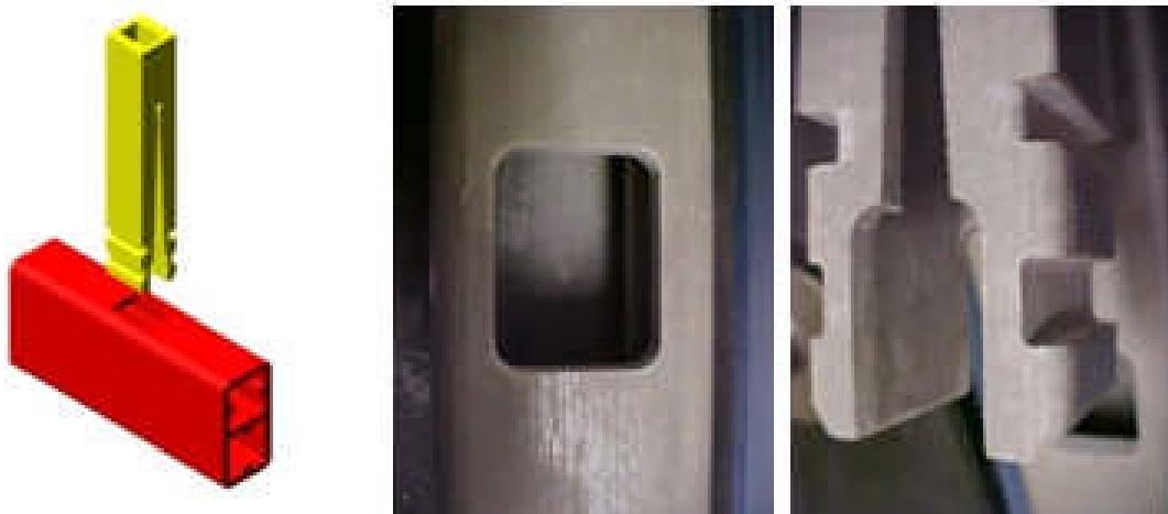
Figure 43 Snap-fit Geometry change for increased load capacity
