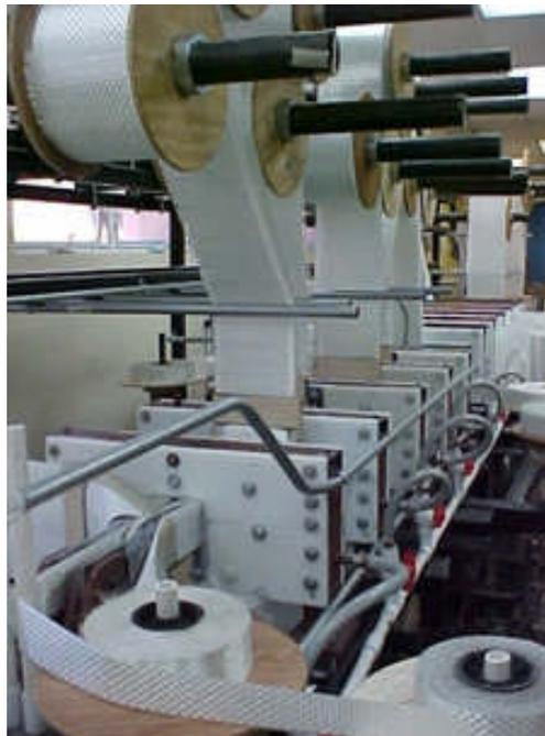
Figure 21 Detail of fiber Dispensing
