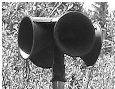
**Figure 1.** Acoustic horn configuration used for field recording of bird vocalizations. The PA3 microphone element is positioned at the junction of all four horns, at the top of the junction to prevent damage from moisture.
