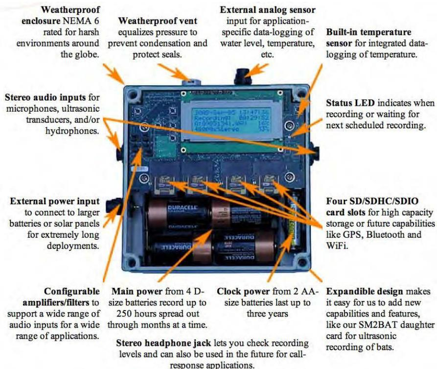
**Figure 6.** Wildlife Acoustics Song Meter SM2 recorder. The SM2 can be programmed to record on simple time-of-day schedules or more complex monitoring protocols such as recording relative to local sunrise, sunset and twilight.
