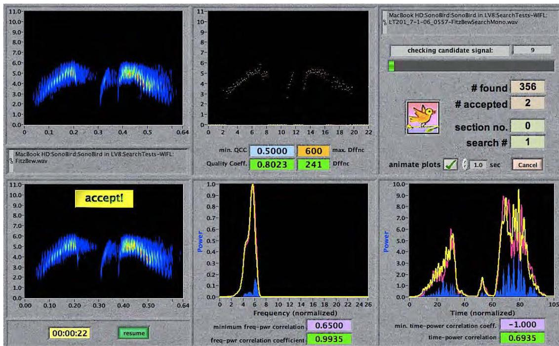
**Figure 8.** SonoBird search panel. SonoBird seeks for signals similar to a known species search term (upper left sonogram) by first running a coarse search to select file segments having basic similarity, then performs a more discriminating comparison with the candidate signal (lower left sonogram) using user-defined criteria. SonoBird saves search criteria in the search term file to facilitate repeated searches. See Appendix C for a full description and guide for use.
