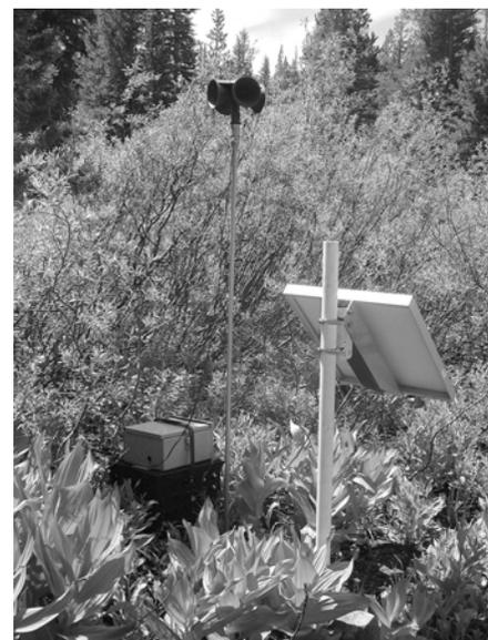
**Figure 1.** Acoustic horn configuration used for field recording of bird vocalizations. The PA3 microphone element is positioned at the junction of all four horns, at the top of the junction to prevent damage from moisture.
