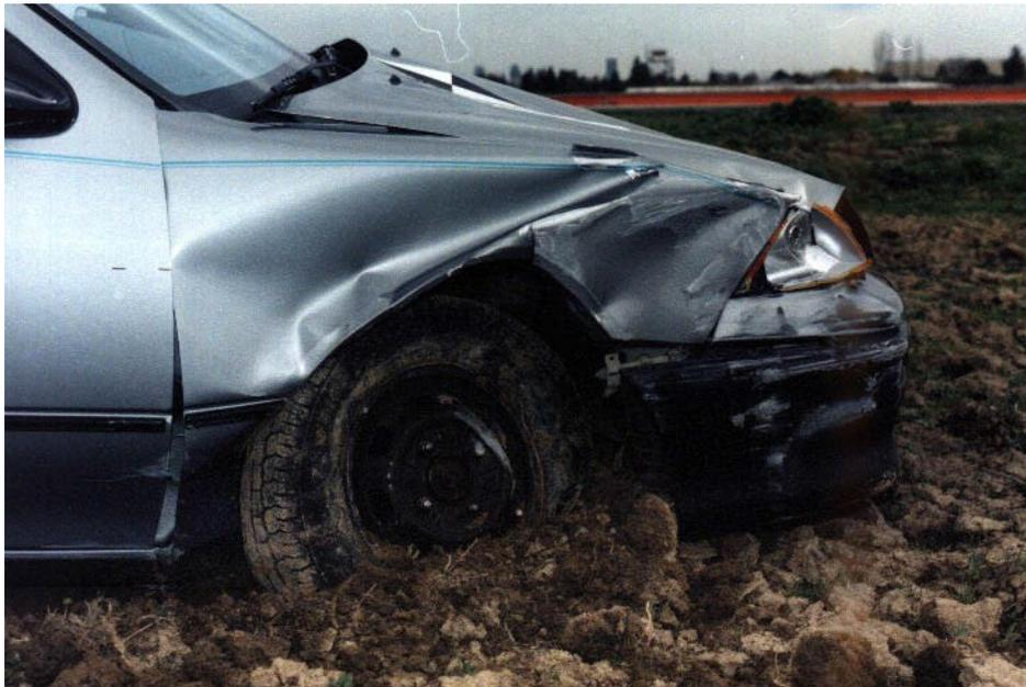
Figure 2-25 - Side Impact Damage
