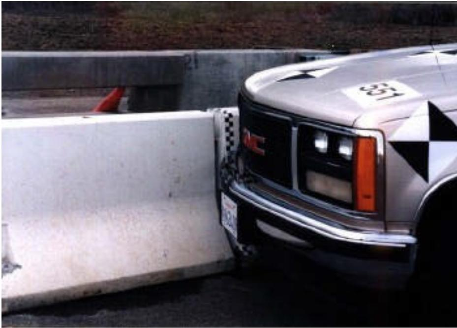
Figure 2-7 - Vehicle 551 At Point Of Impact
