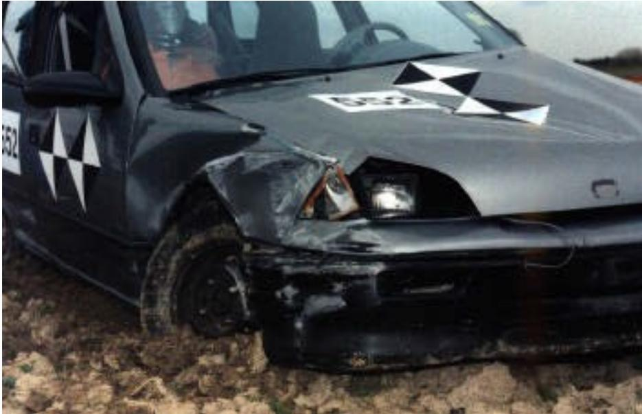
Figure 2-24 -Front View of Vehicle Impact Damage
