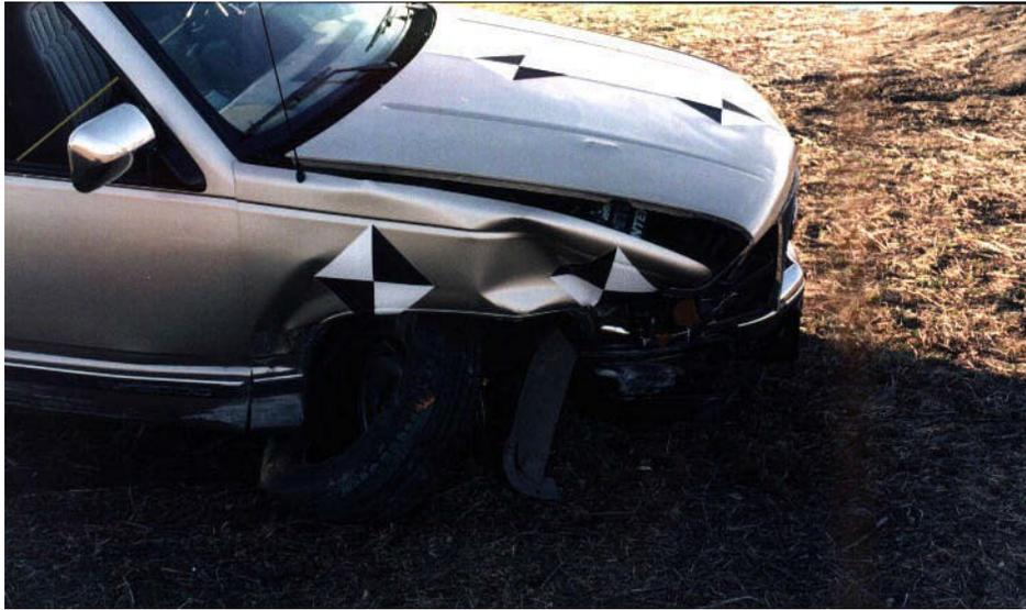
Figure 2-10 - Front Impact Side of Vehicle
