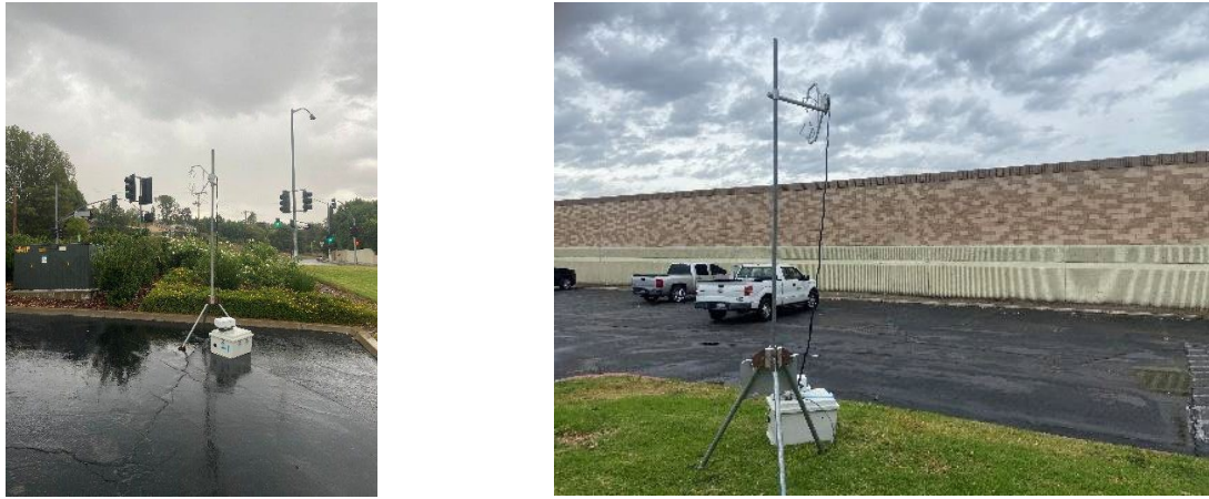
Figure 4.6. Left panel shows downwind sonic anemometer located in the open section. Right panel shows upwind sonic located west of SR-55.
