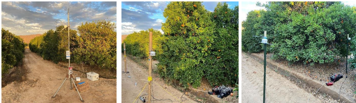
Figure 4.1. Typical setup of studies conducted at the UCR Agricultural Station. Top panel shows the location on Iowa Avenue, Riverside, CA. Bottom panel shows mounting of the PurpleAir sensors between tree rows.
