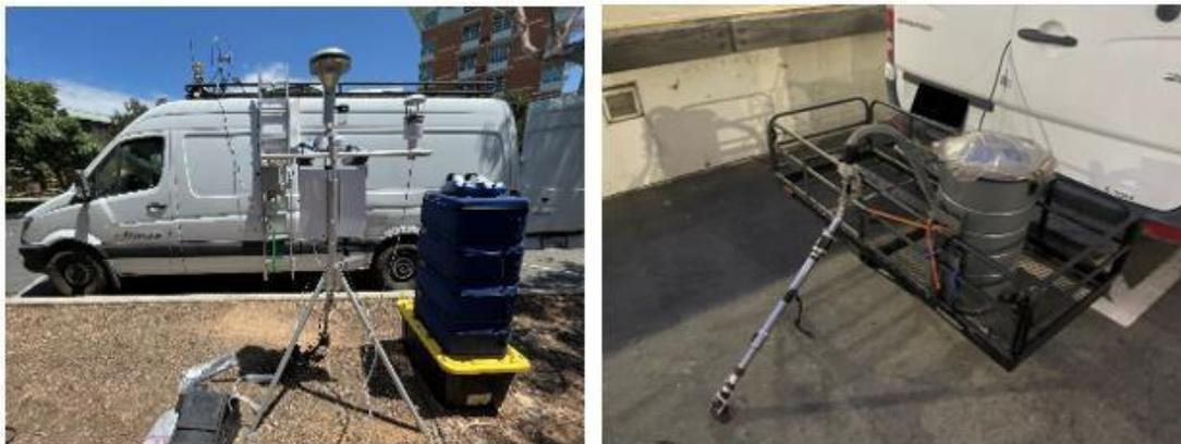
**Figure 2.1** *The left panel shows the mobile platform with a 2-D sonic anemometer mounted at 3 m. The right panel shows the dust collection system mounted on the platform.*
