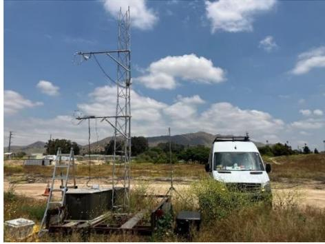
**Figure 2.3** Experimental setup to compare meteorological parameters derived from the 3D sonic anemometer with those from the mobile platform meteorological sensors.
