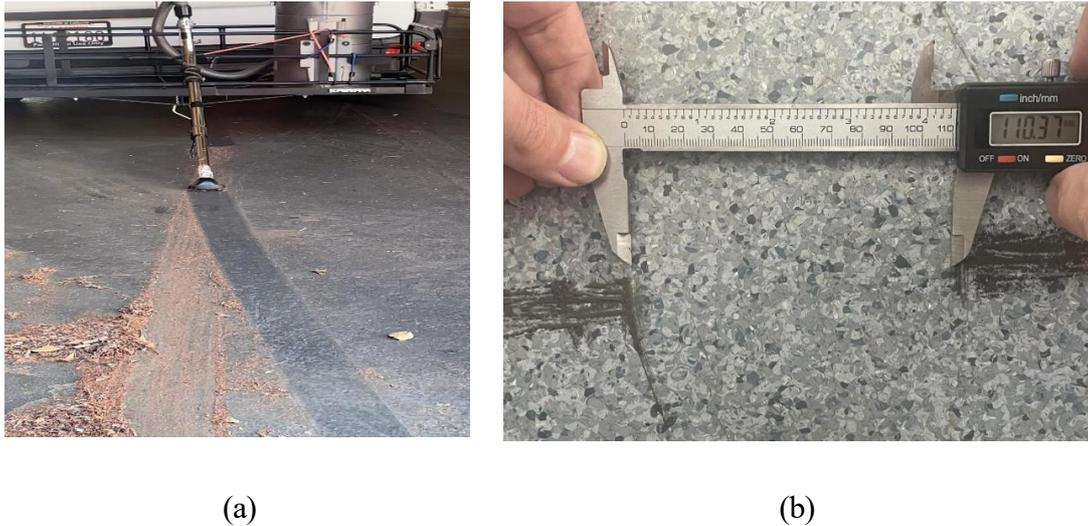
**Figure 2.6** a) Area vacuumed by the dust collection system, and b) Width of vacuumed area.
