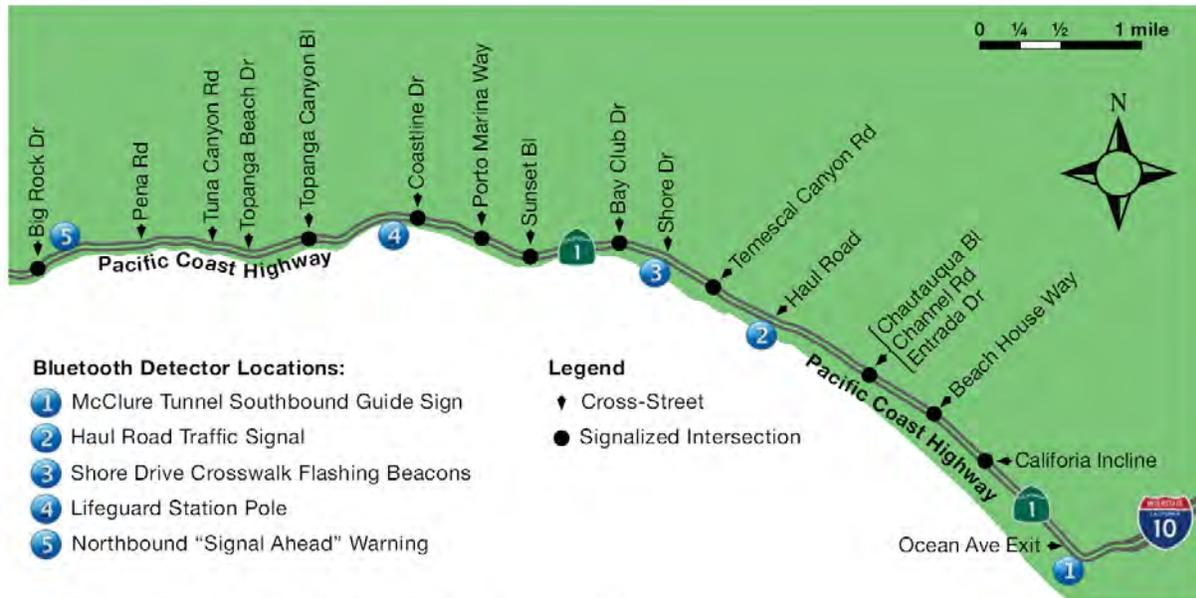
**Figure 3.11 Bluetooth Detector Locations on PCH**
