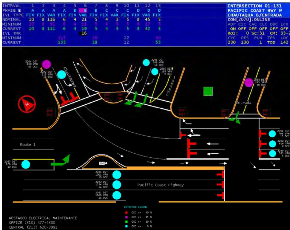
Figure 2.2 PCH/Chautauqua Blvd Intersection Display: Signal Settings and Detector Locations
