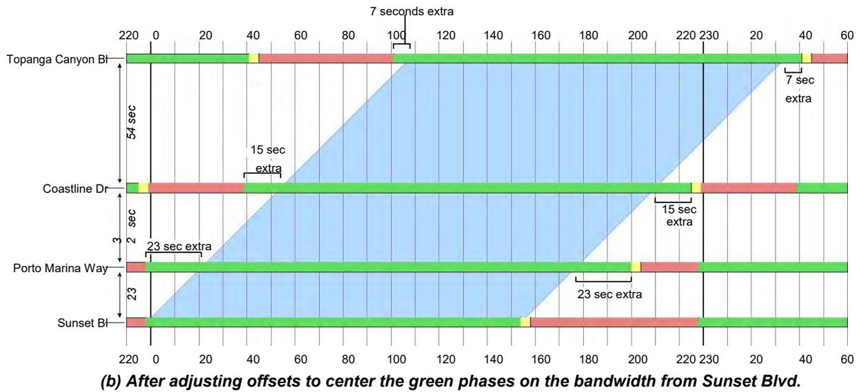
Figure 4.10 Offsets for Intersections downstream of Sunset Blvd—TOD 230 Plan, PM Peak
