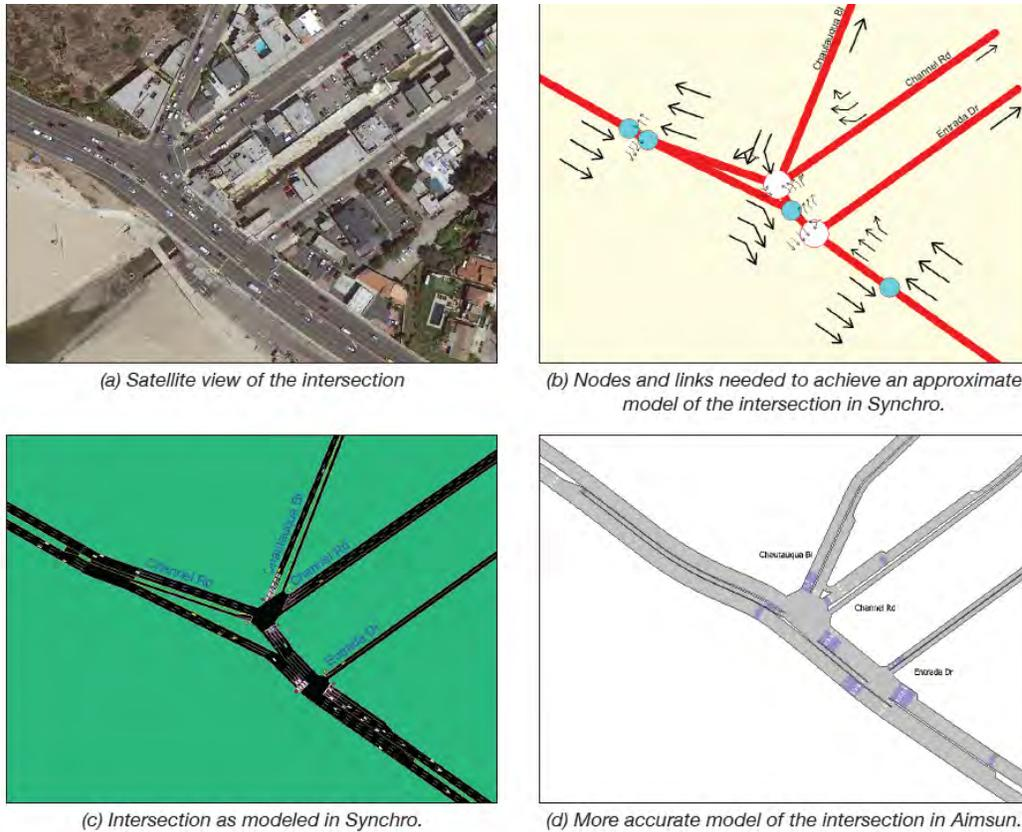
**Figure 4.1 Modeling the Intersection of Chautauqua Blvd, Channel Rd, and Entrada Dr.**
