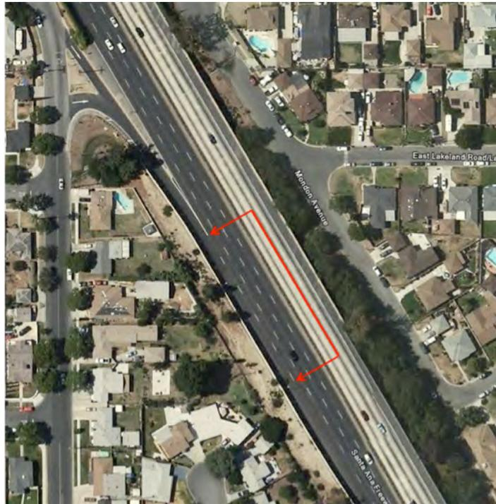
Figure 21. Example of an acceleration lane and its length
