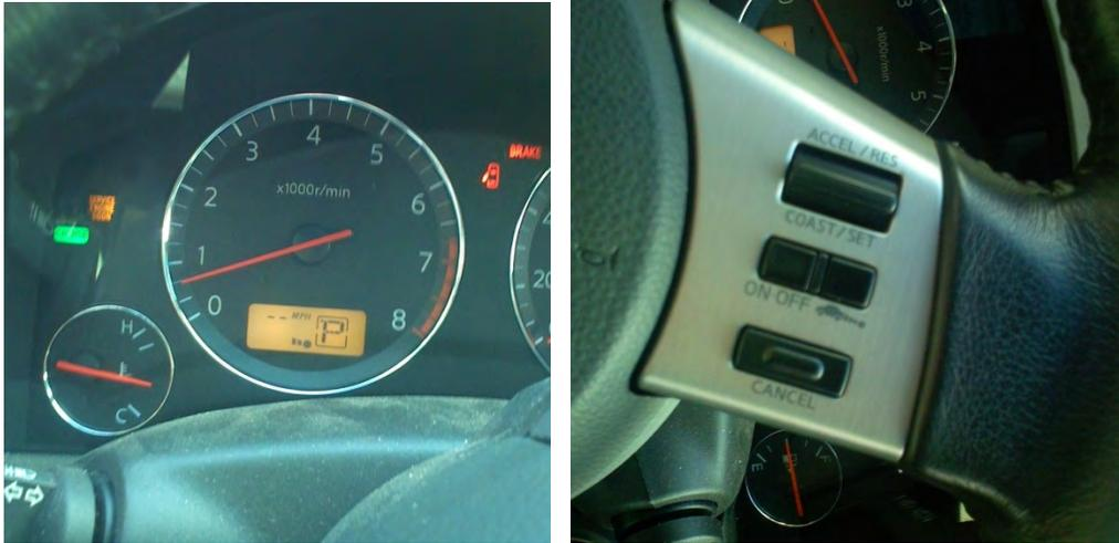
**Figure 11: ACC displays (left) and controls (right)**
