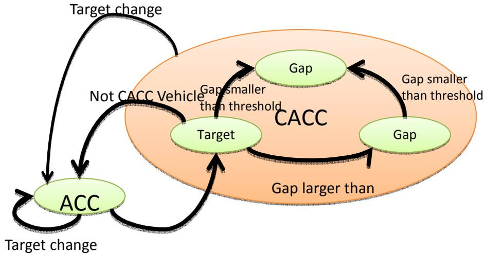
**Figure 5: State Machine for PATH CACC controller**
