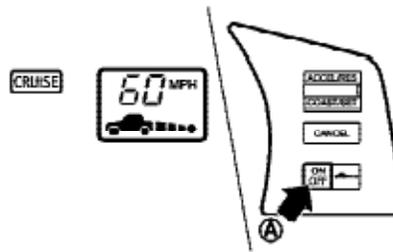
**Figure 10: ACC display and controls as illustrated in vehicle owner’s manual**
