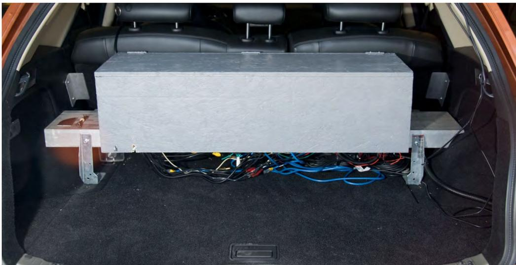
**Figure 15: Computer enclosure in luggage compartment behind rear seat of vehicle, with cover closed**
