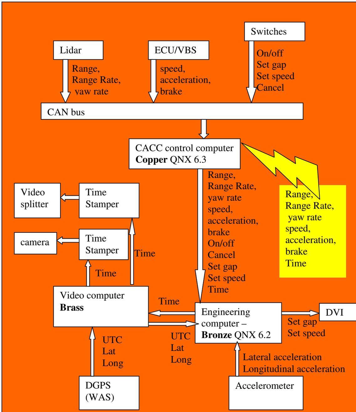
Figure 19: DAS Data flow for CACC Vehicle
