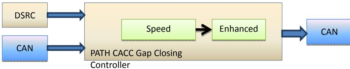
Figure 7: PATH CACC Gap Closing Controller
