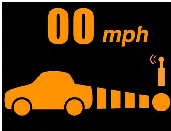
**Figure 13: CACC Driver Vehicle Interface**
