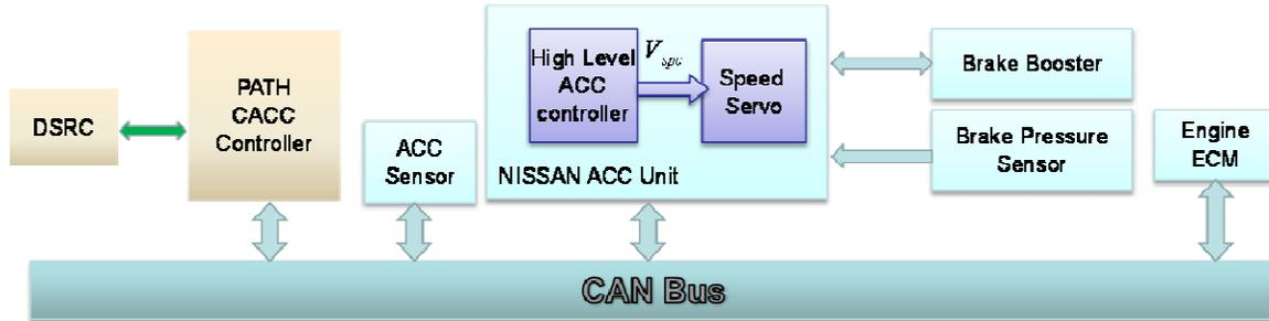
**Figure 4: Add-on System Design for PATH CACC**
