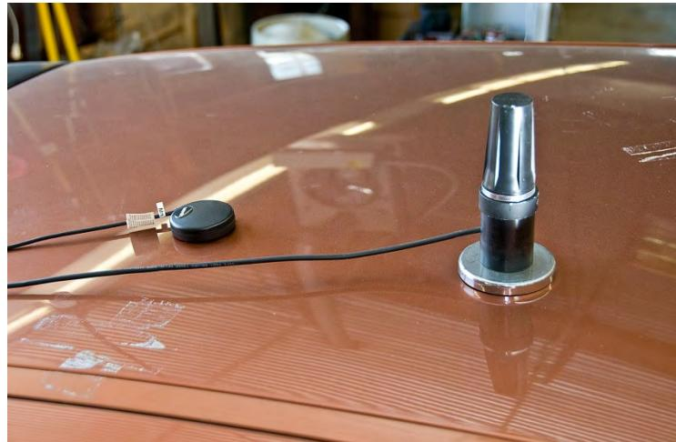
**Figure 16: DGPS Antenna (left) and DSRC Communication Antenna (right)**
