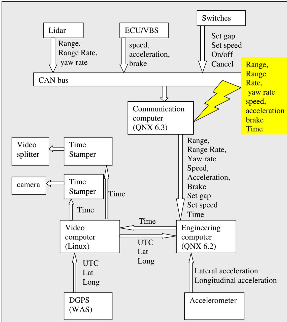
Figure 18: DAS Data Flow for ACC
