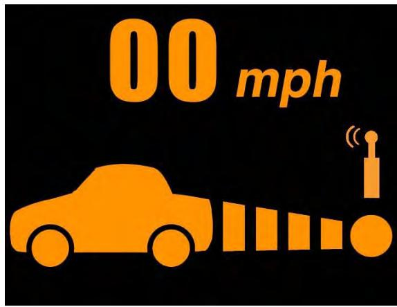
Figure 13: CACC Driver Vehicle Interface
