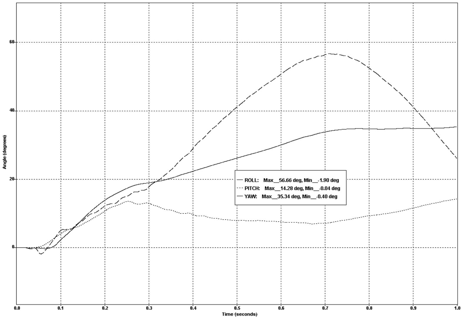
Figure 7-21. Test 672 Vehicle Roll, Pitch, and Yaw Vs Time
