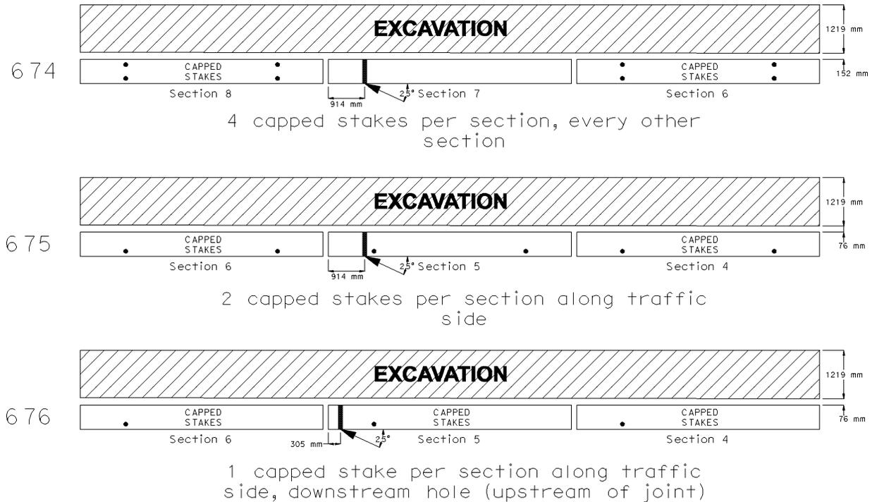
Figure 2-5. Staking Configurations Layout
