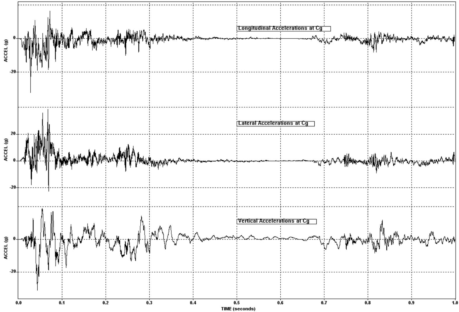
Figure 7-38. Test 676 Vehicle Accelerations Vs Time
