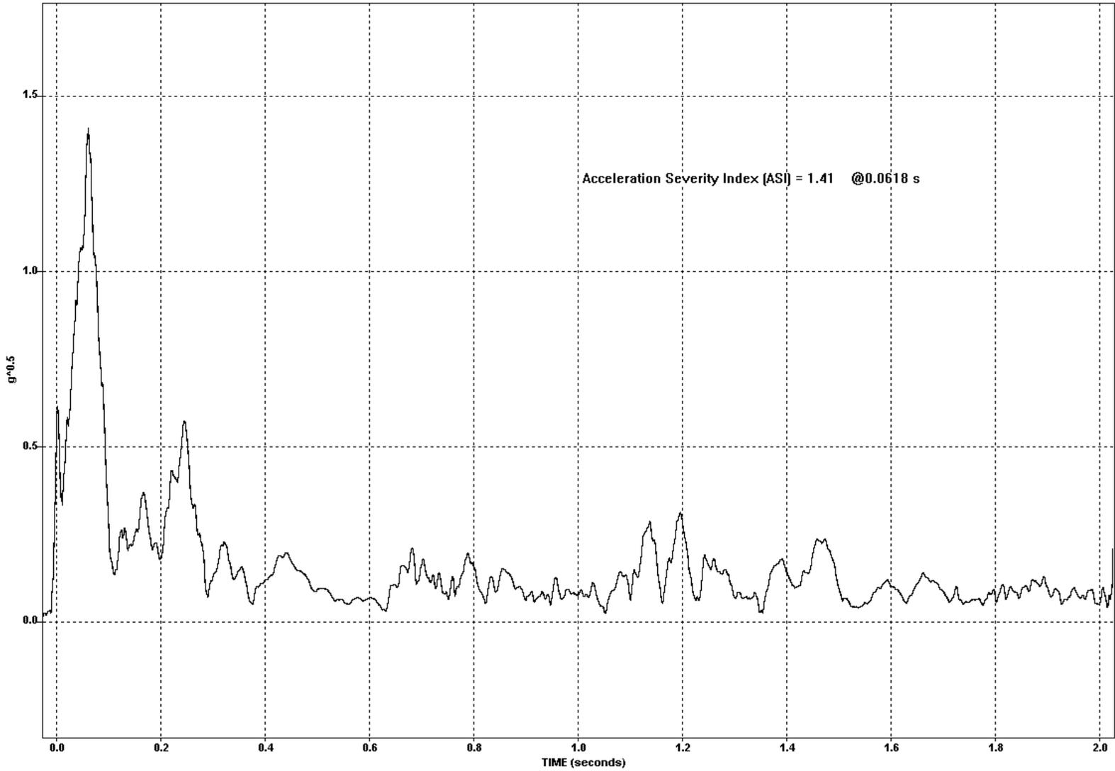
Figure 7-16. Test 671 Acceleration Severity Index Vs Time
