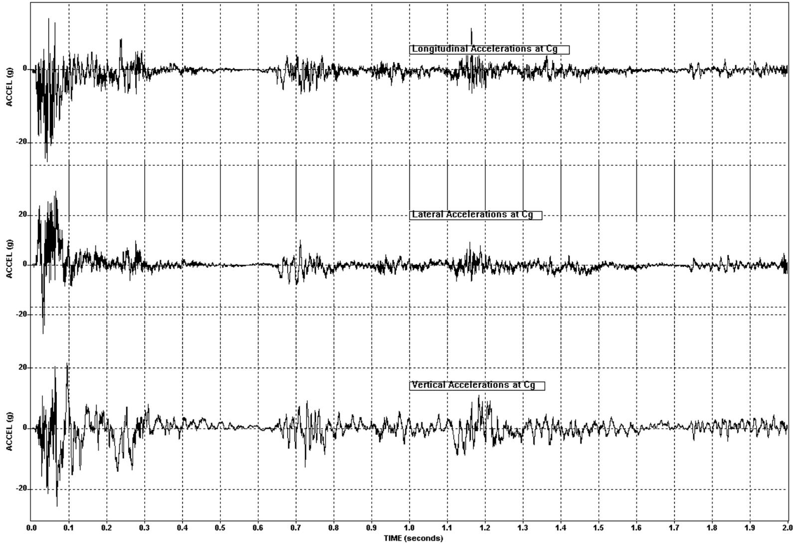
Figure 7-13. Test 671 Vehicle Accelerations Vs Time
