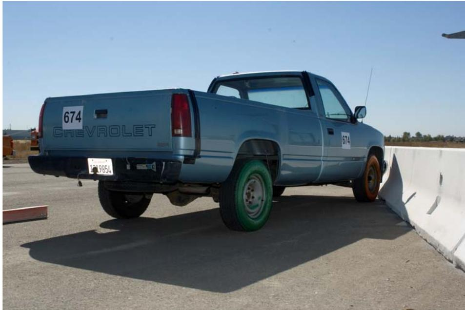
Figure 2-45. Test 674 - Vehicle at Impact Location Pre-Impact
