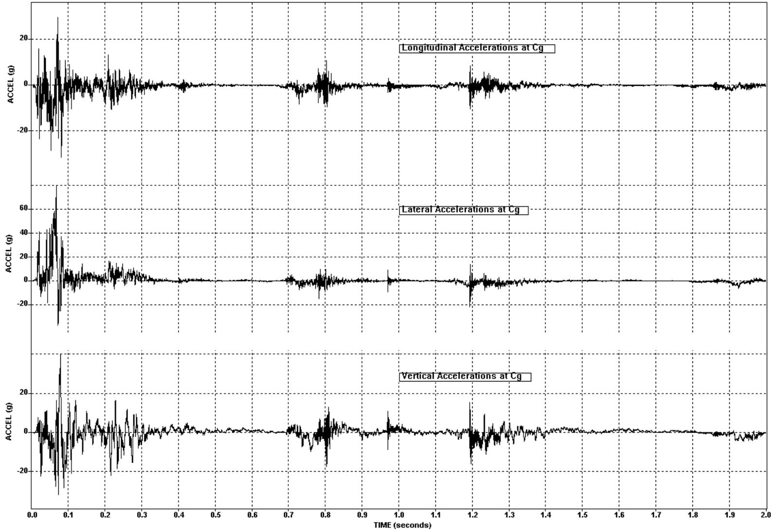
Figure 7-29. Test 674 Vehicle Accelerations Vs Time
