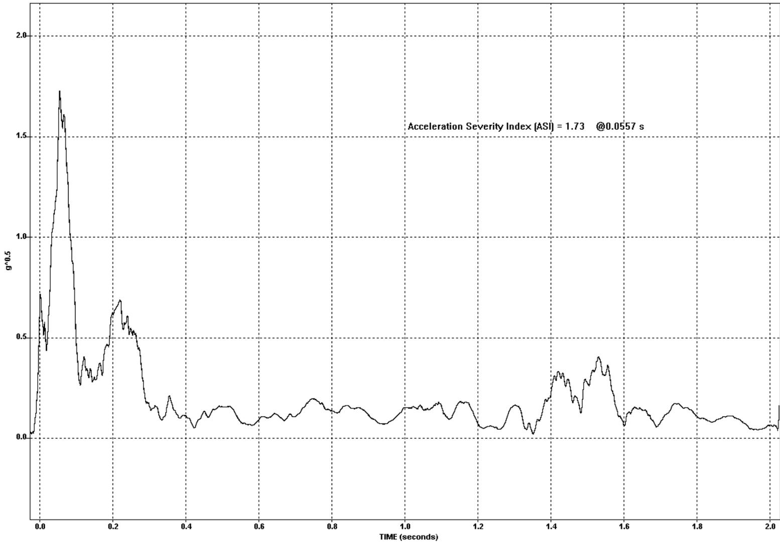
Figure 7-27. Test 673 Acceleration Severity Index Vs Time
