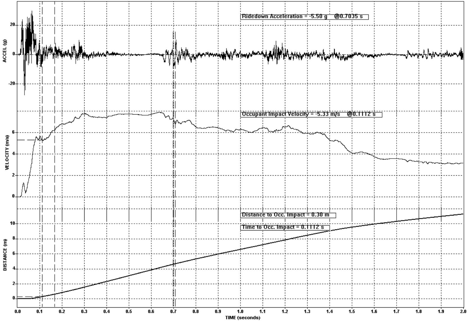
Figure 7-15. Test 671 Vehicle Lateral Acceleration, Velocity, and Distance Vs Time
