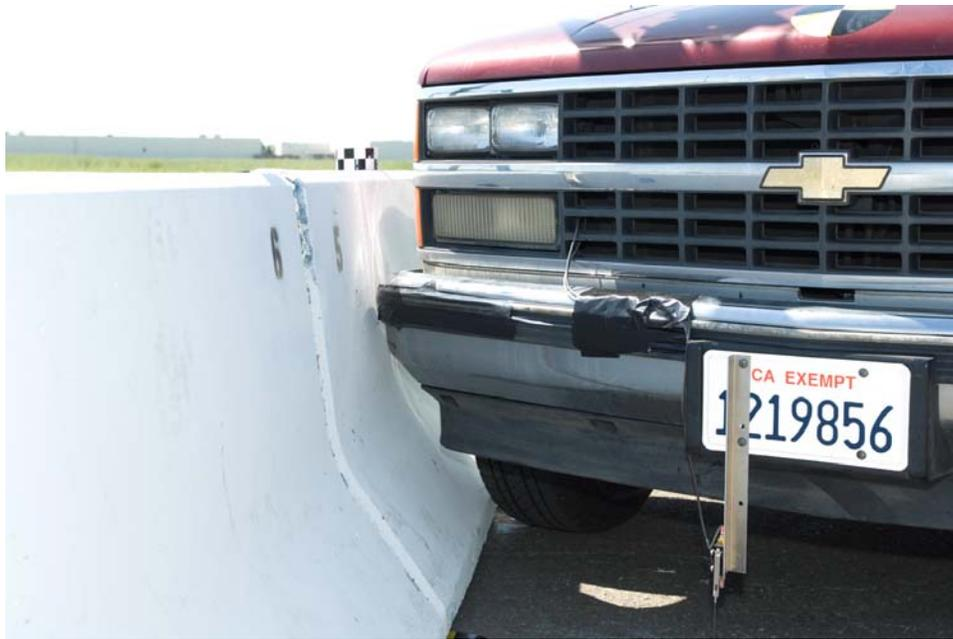
Figure 2-74. Test 676 - Close-up View of Vehicle at Impact Location
