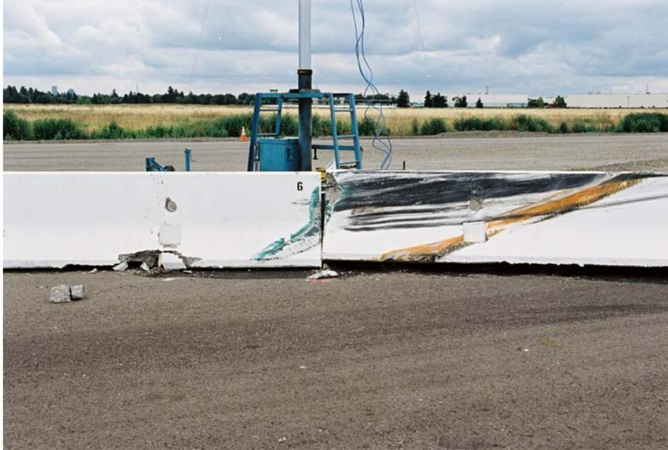
Figure 2-12. Test 671 - Impact Location Post-Impact
