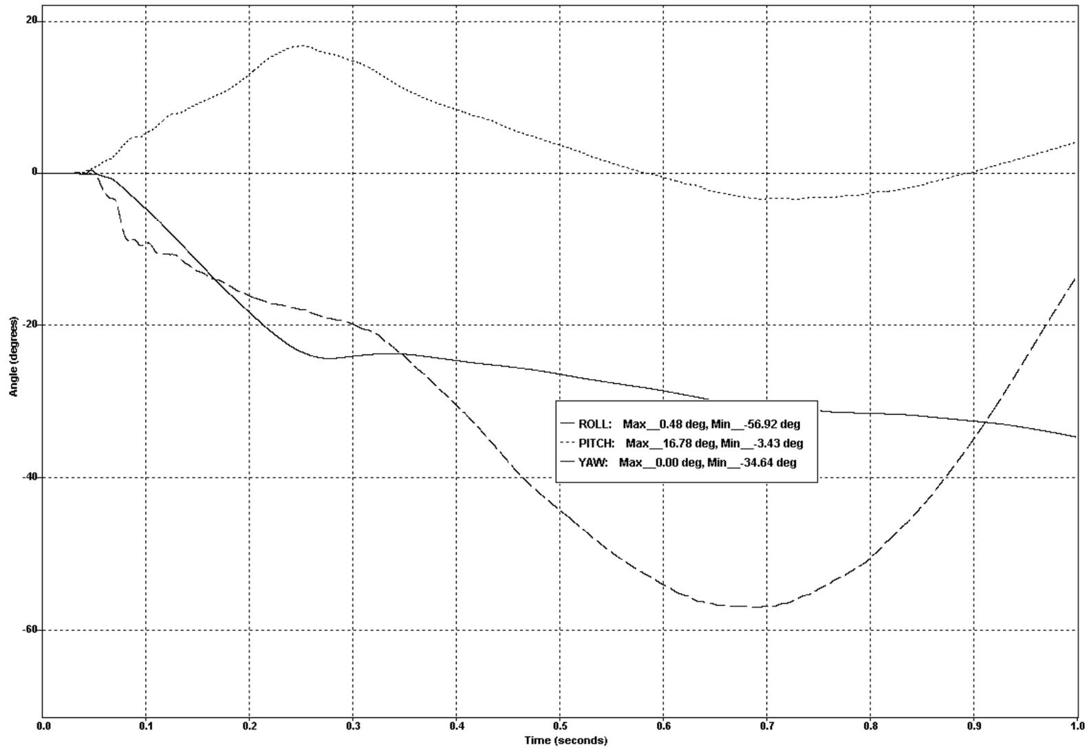
Figure 7-34. Test 675 Vehicle Roll, Pitch, and Yaw Vs Time
