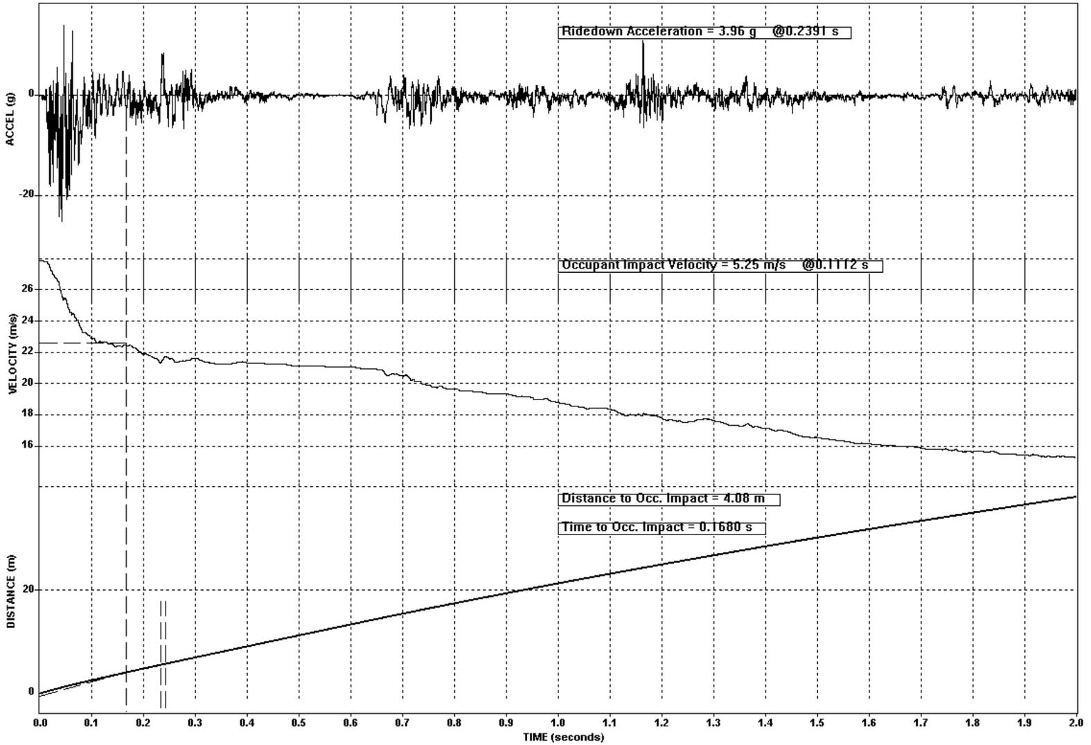
Figure 7-14. Test 671 Vehicle Longitudinal Acceleration, Velocity, and Distance Vs Time
