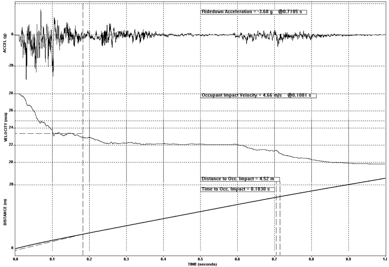
Figure 7-37. Test 675 Vehicle Longitudinal Acceleration, Velocity, and Distance Vs Time
