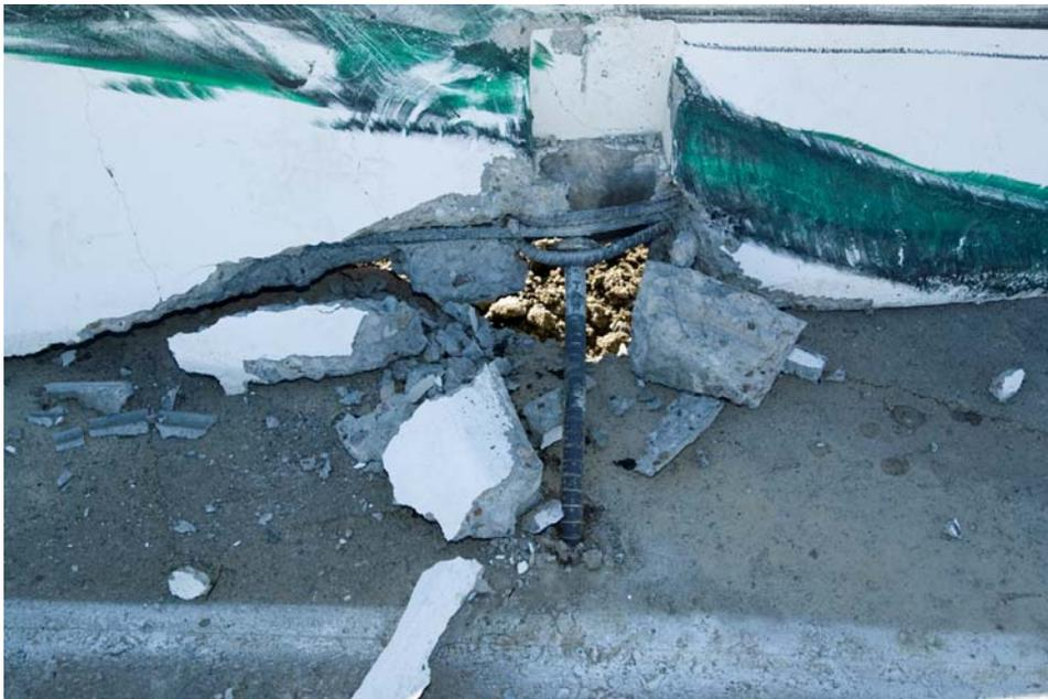
Figure 2-52. Test 674 - Upstream, Impact-side Stake in Section 8 Post-Impact
