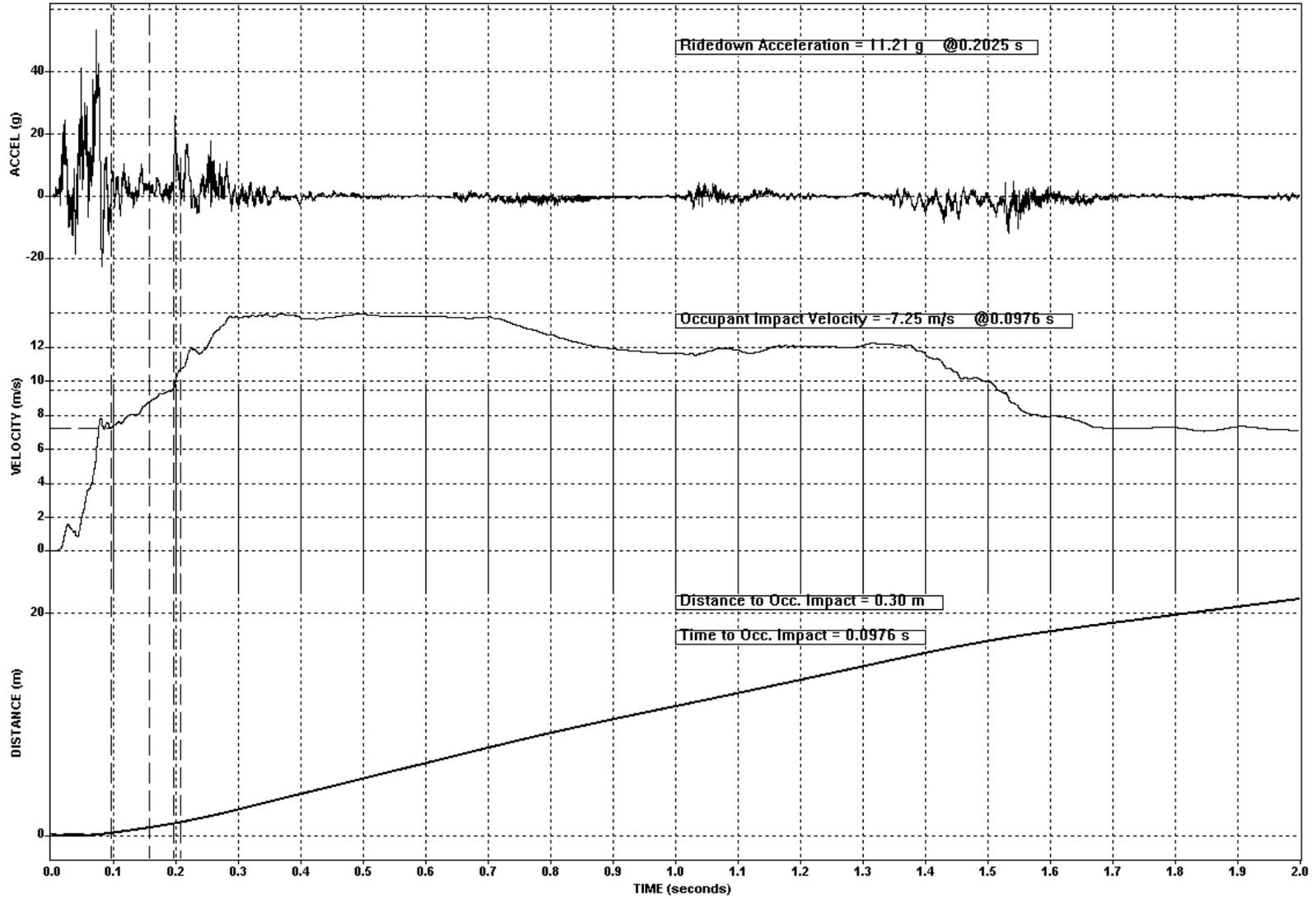
Figure 7-25. Test 673 Vehicle Lateral Acceleration, Velocity, and Distance Vs Time
