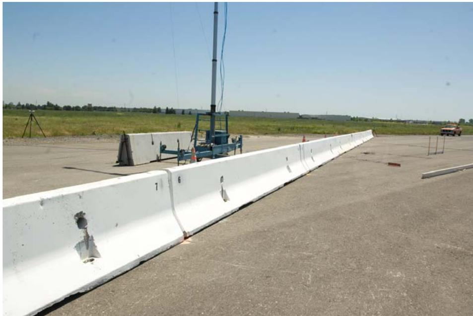
Figure 2-75. Test 676 - Barrier Pre-Impact
