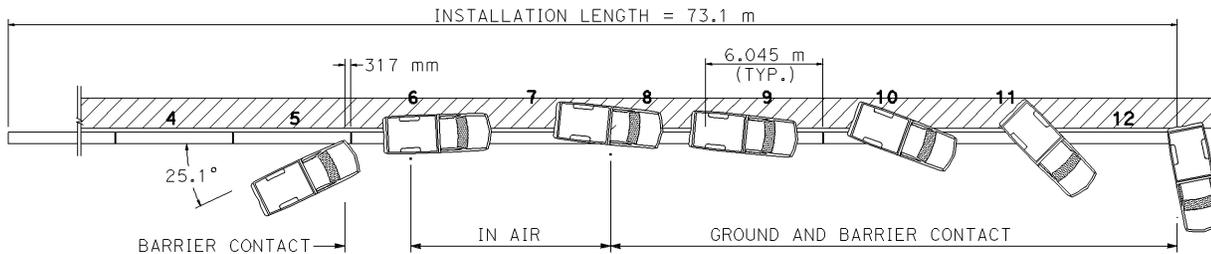
Figure 2-82. Test 676 - Impact sequence and diagram
