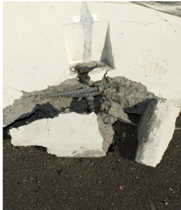
Figure 2-68. Test 675 - Stake Downstream from Impact Point
