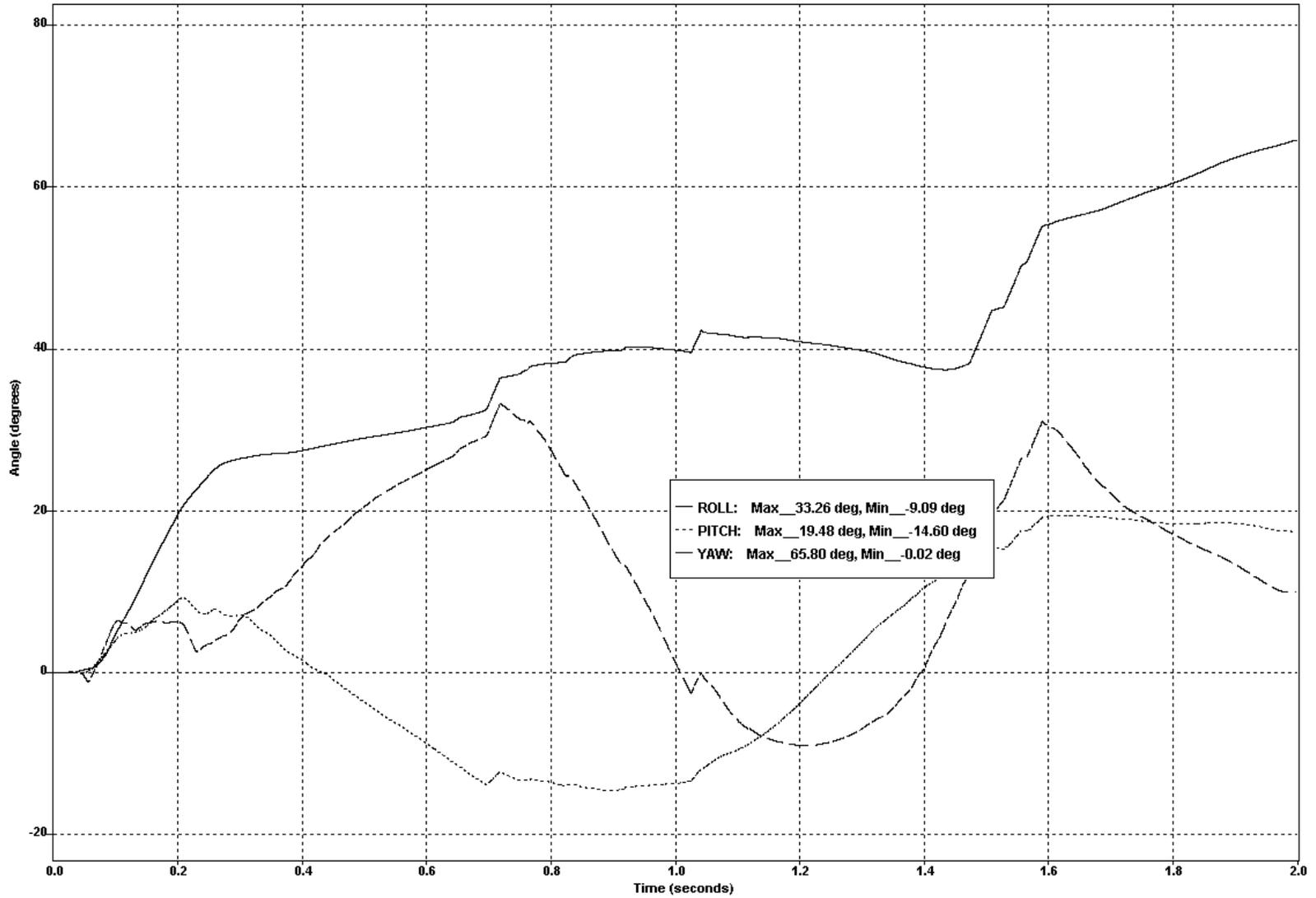
Figure 7-26. Test 673 Vehicle Roll, Pitch, and Yaw Vs Time
