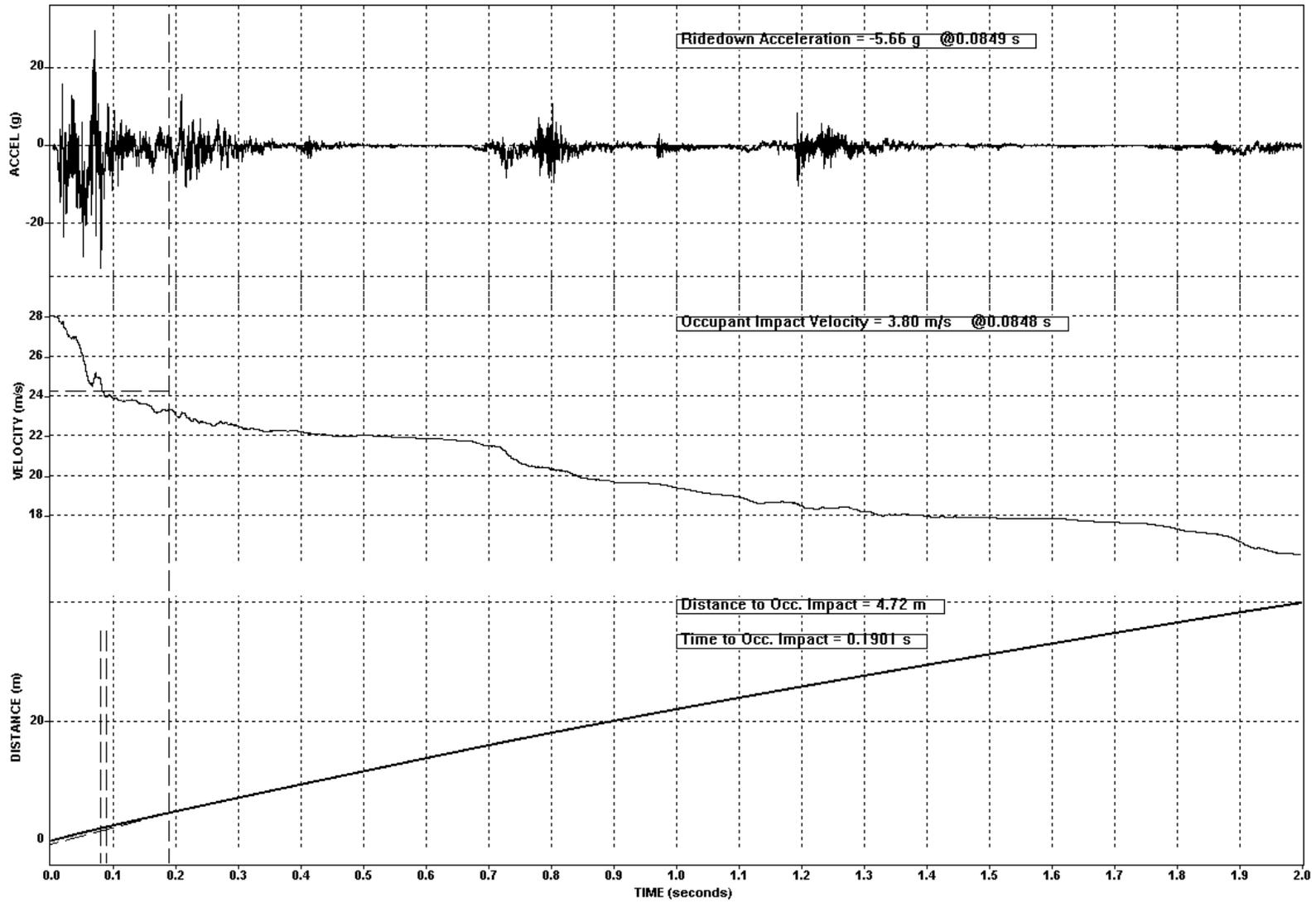
Figure 7-28. Test 674 Vehicle Longitudinal Acceleration, Velocity, and Distance Vs Time
