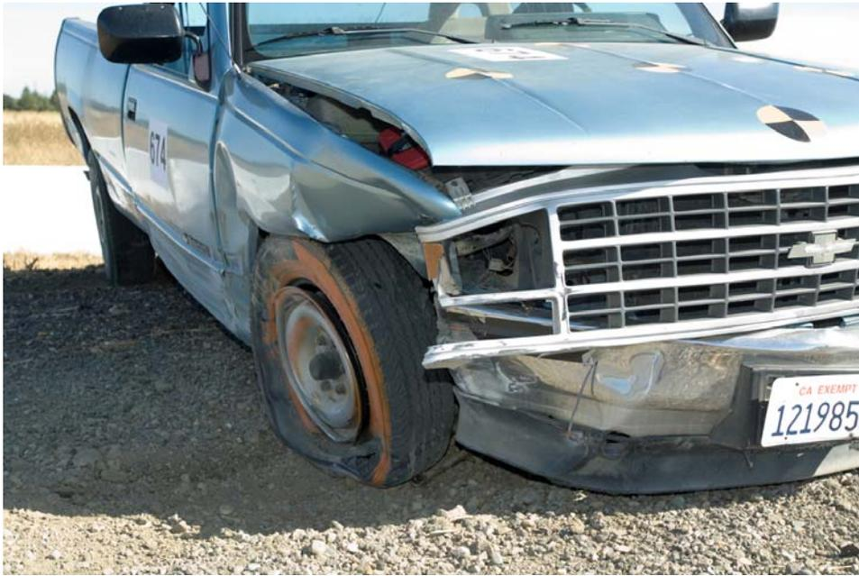
Figure 2-57. Test 674 - Front-right View of Vehicle Post-Impact
