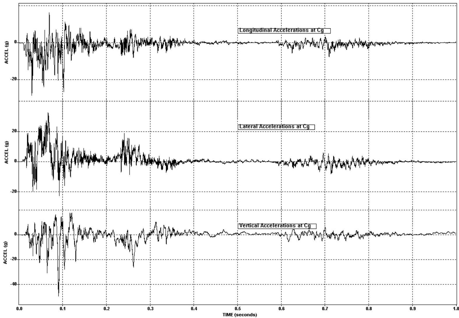
Figure 7-35. Test 675 Vehicle Accelerations Vs Time
