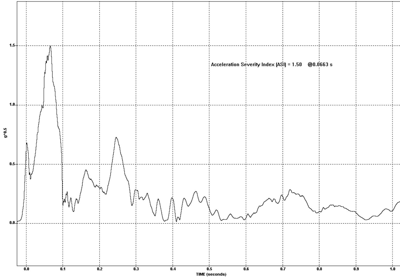
Figure 7-22. Test 672 Acceleration Severity Index Vs Time
