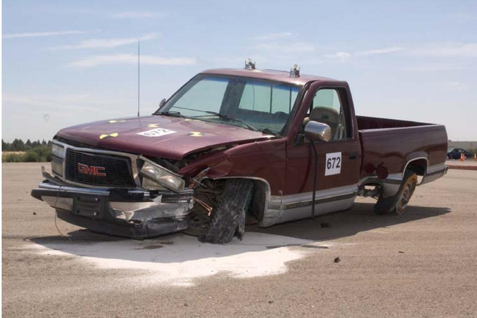
Figure 2-29. Test 672 - Front-left View of Vehicle Post-Impact
