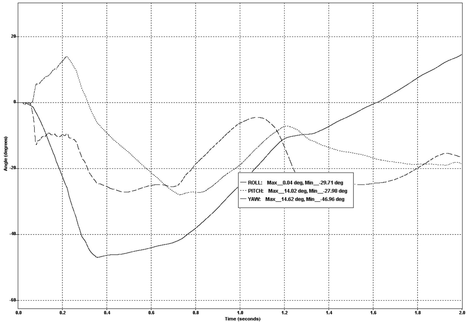
Figure 7-31. Test 674 Vehicle Roll, Pitch, and Yaw Vs Time
