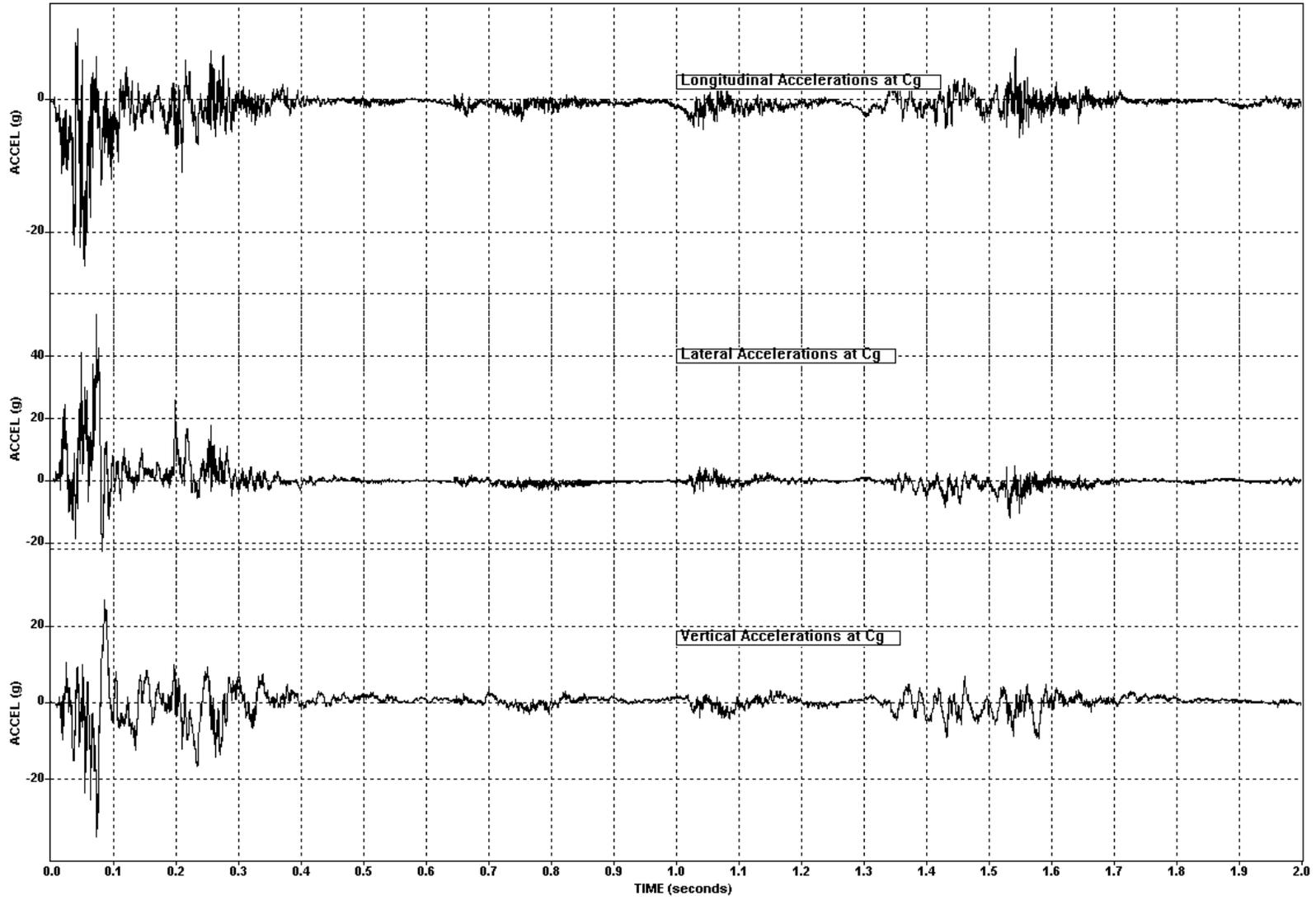
Figure 7-23. Test 673 Vehicle Accelerations Vs Time
