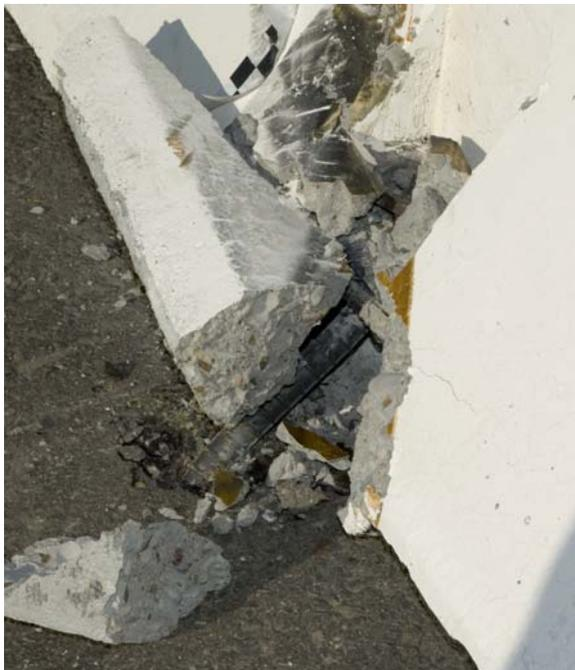
Figure 2-67. Test 675 - Stake at Impact Point
