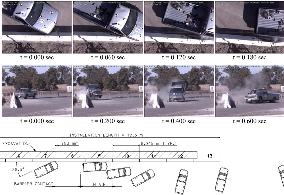
Figure 2-58. Test 674 - Impact sequence and diagram
