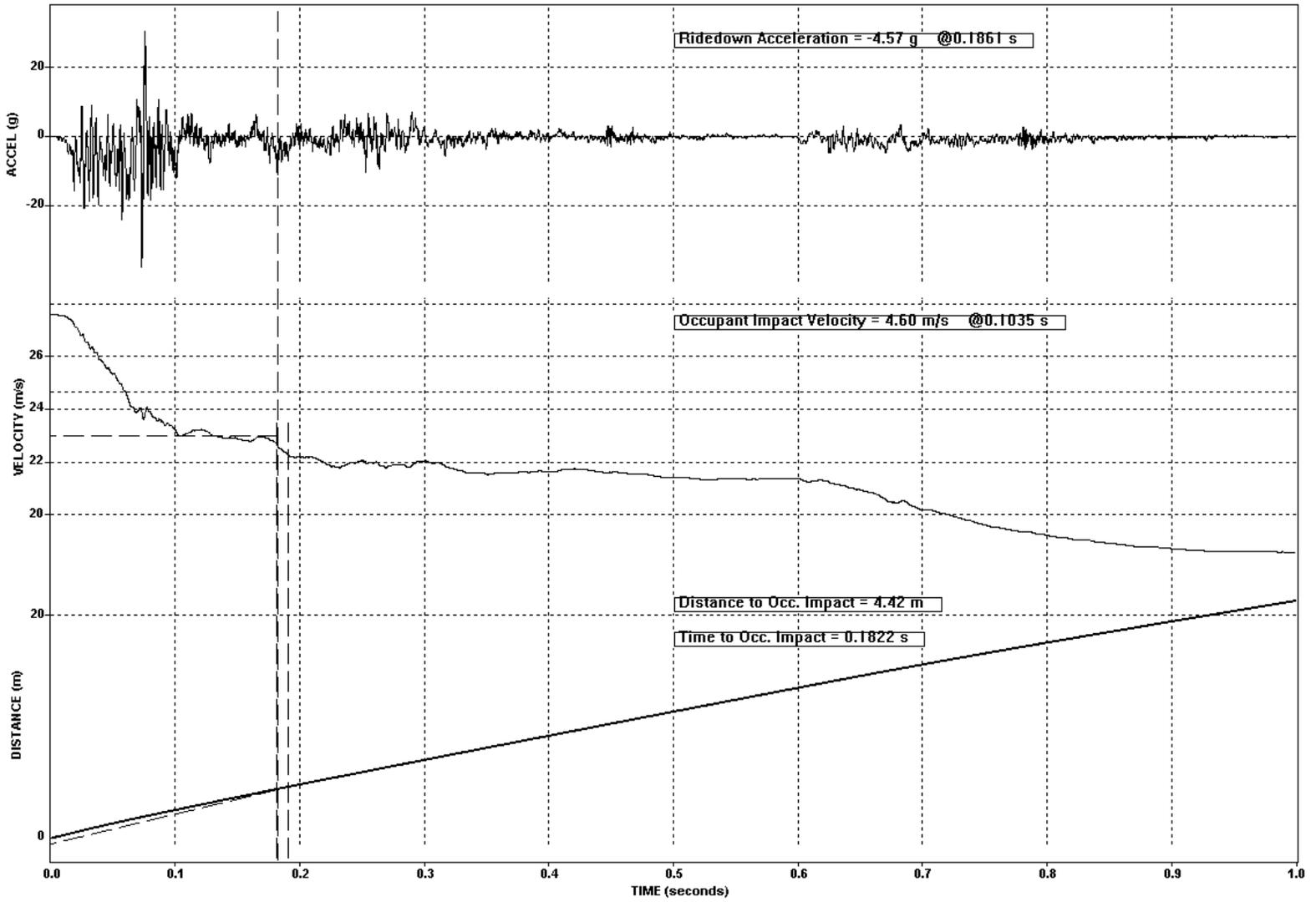
Figure 7-19. Test 672 Vehicle Longitudinal Acceleration, Velocity, and Distance Vs Time
