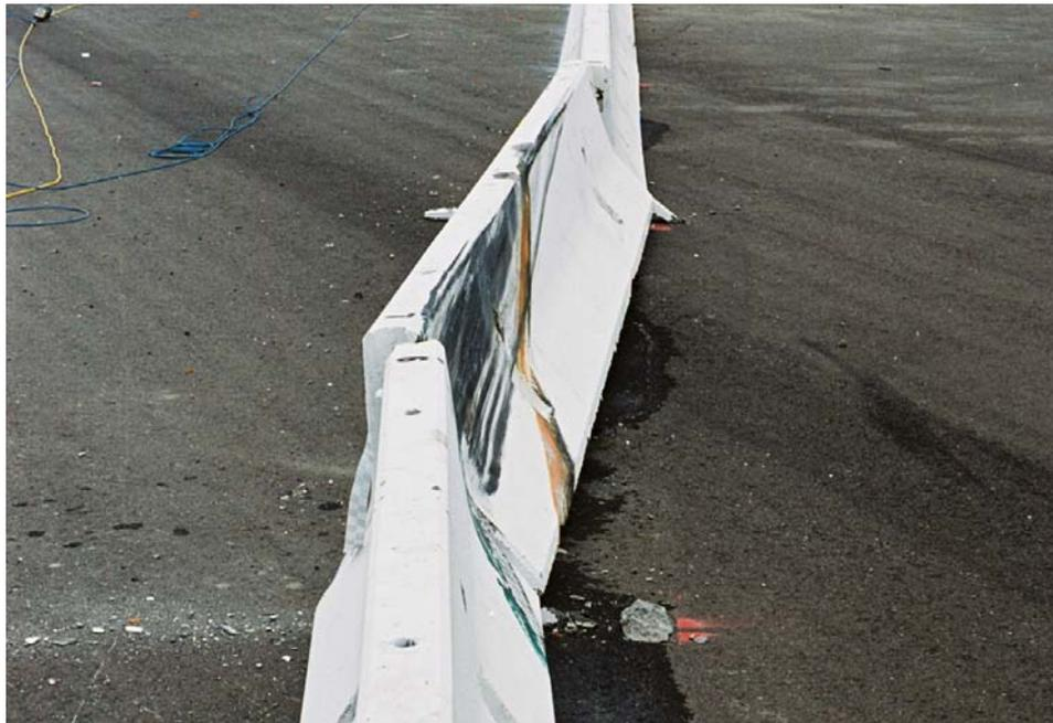
Figure 2-11. Test 671 - Downstream View of Barrier Post-Impact
