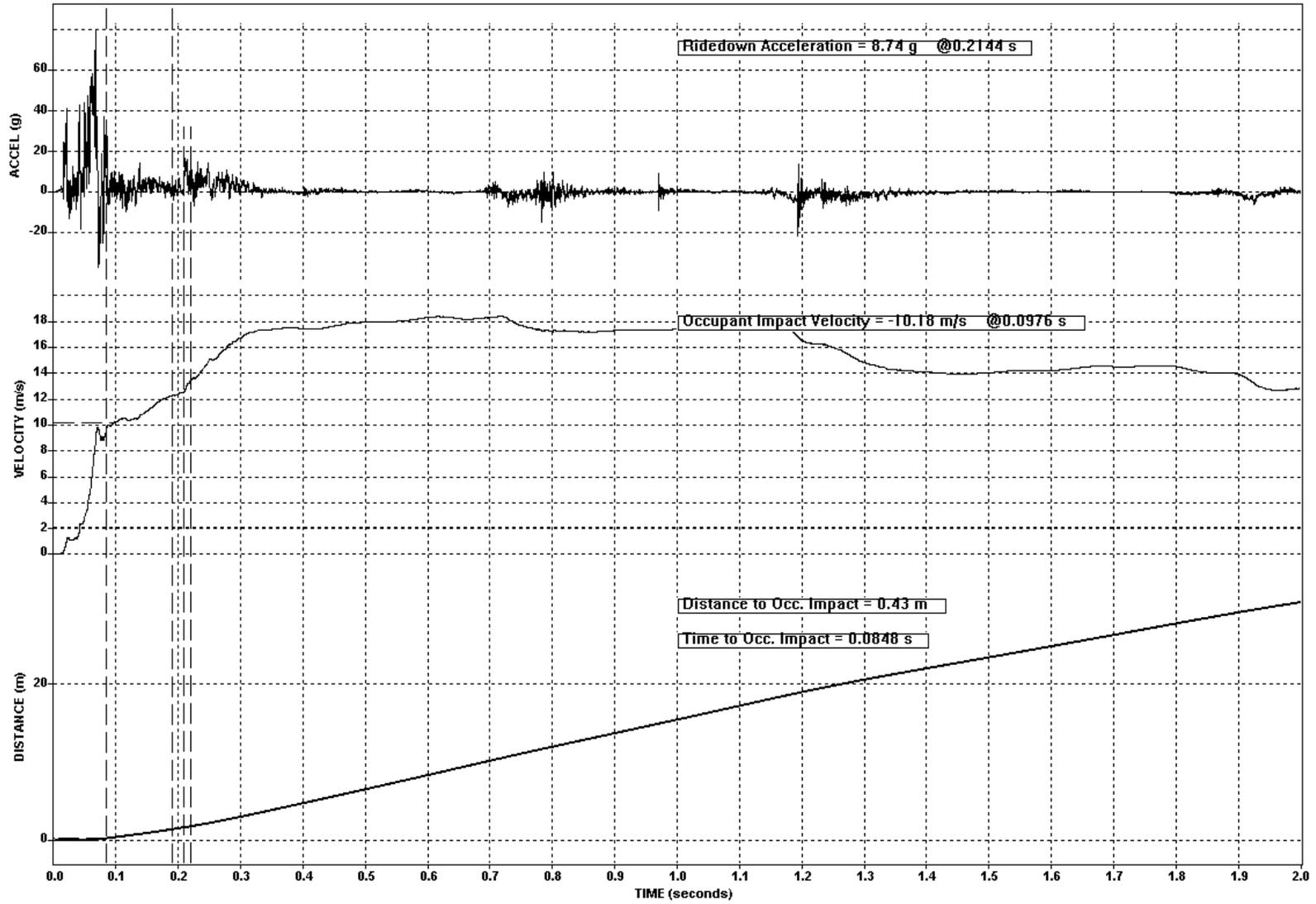
Figure 7-30. Test 674 Vehicle Lateral Acceleration, Velocity, and Distance Vs Time
