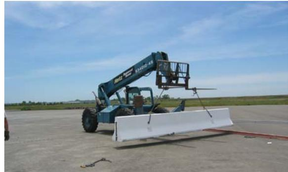
Figure 7-8. Forklift Carrying K-rail
