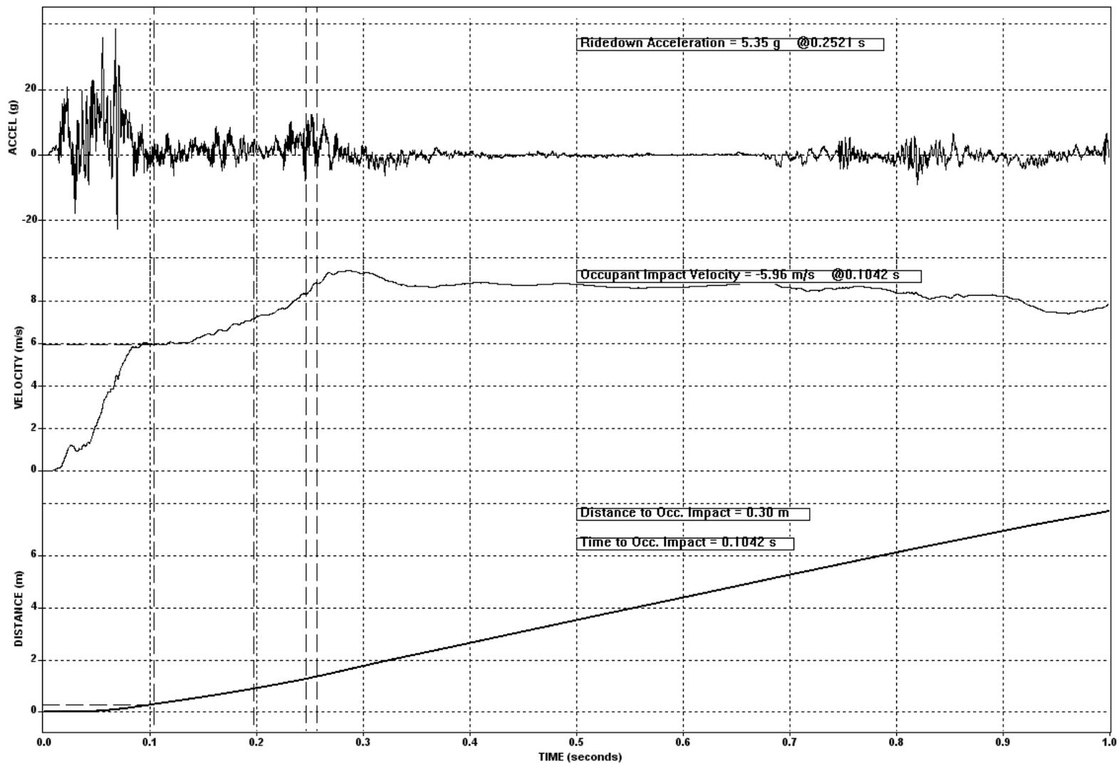
Figure 7-40. Test 676 Vehicle Lateral Acceleration, Velocity, and Distance Vs Time
