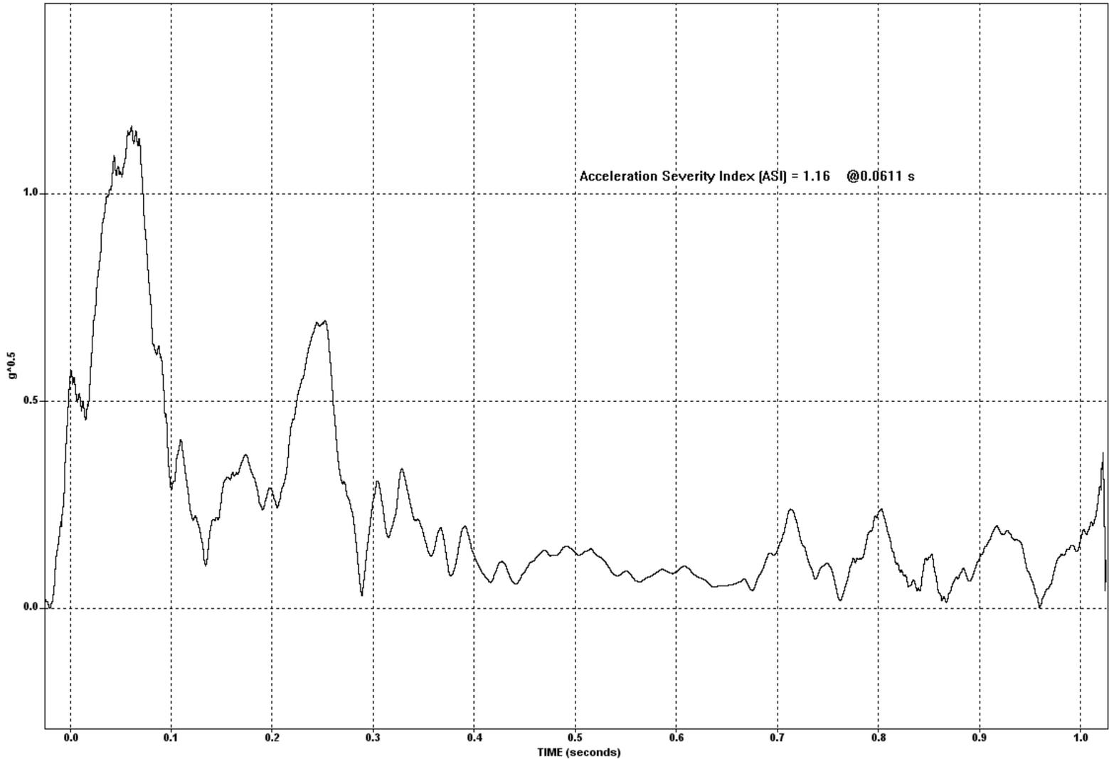
Figure 7-42. Test 676 Acceleration Severity Index Vs Time
