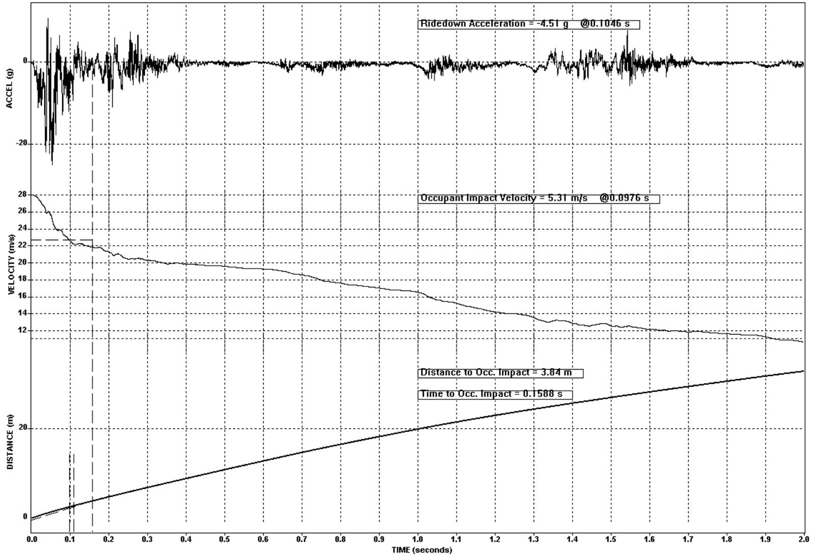
Figure 7-24. Test 673 Vehicle Longitudinal Acceleration, Velocity, and Distance Vs Time
