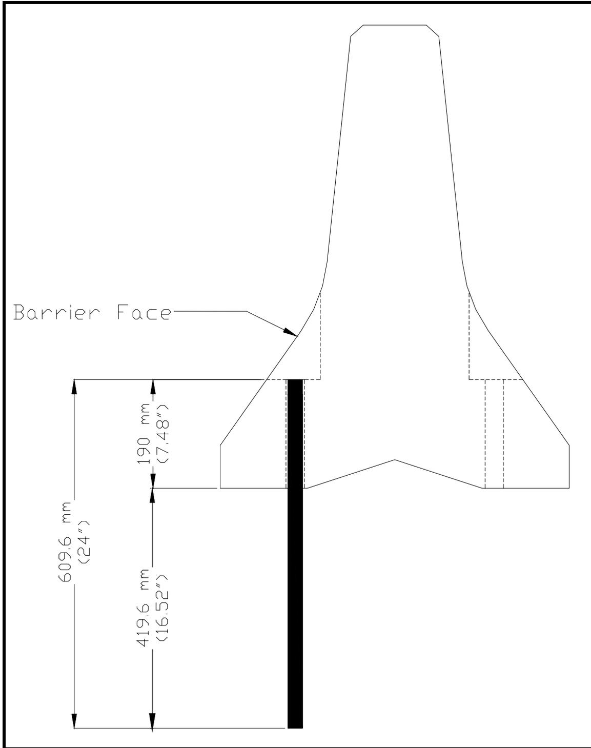
Figure 7-4. Typical Uncapped Stake Installation Layout
