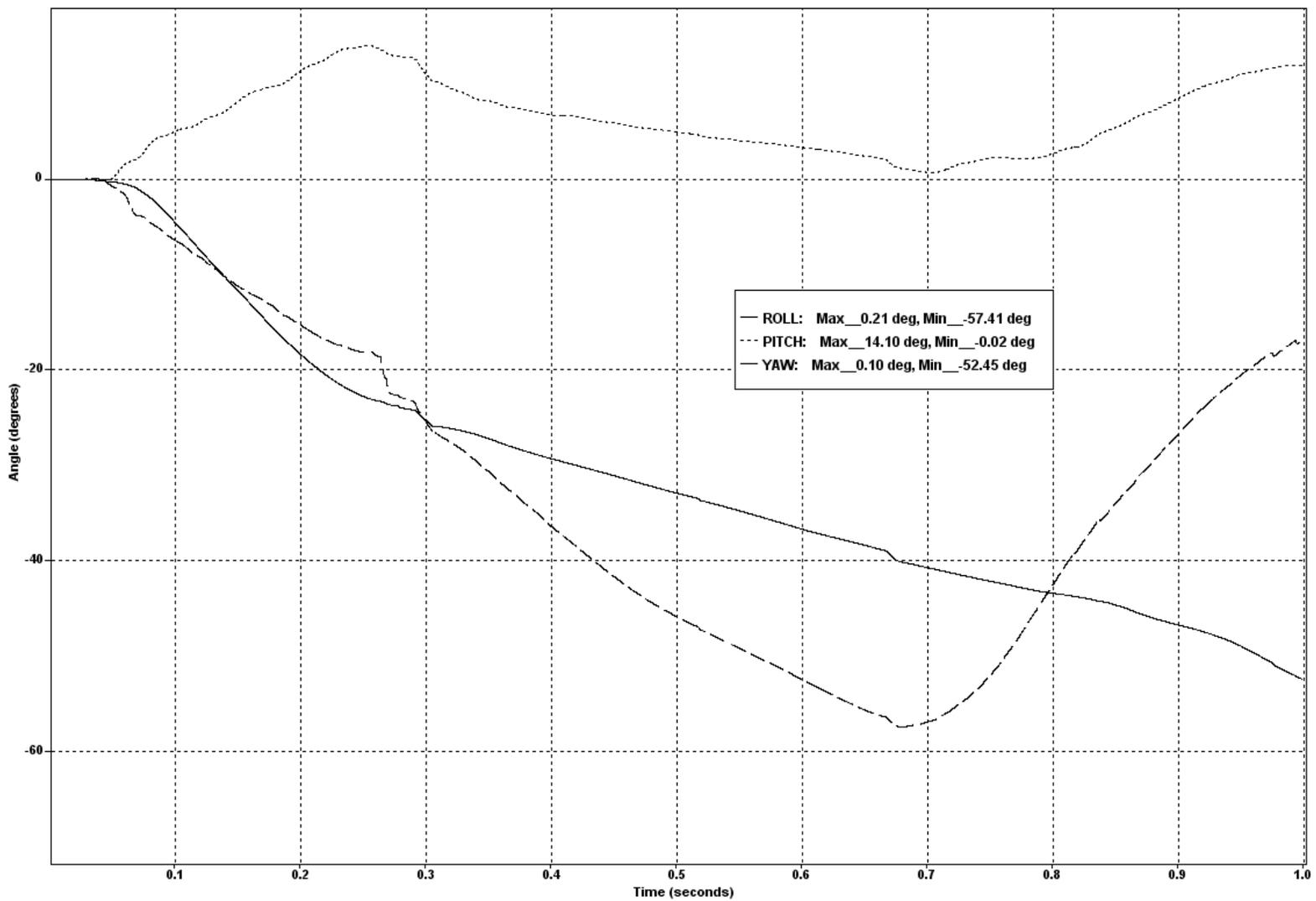
Figure 7-41. Test 676 Vehicle Roll, Pitch, and Yaw Vs Time
