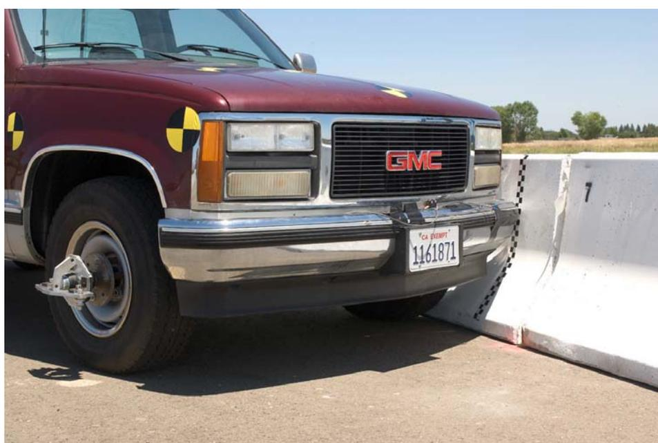
Figure 2-20. Test 672 - Close-up View of Vehicle at Impact Location
