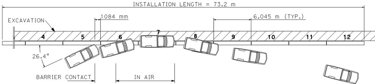
Figure 2-71. Test 675 - Impact sequence and diagram
