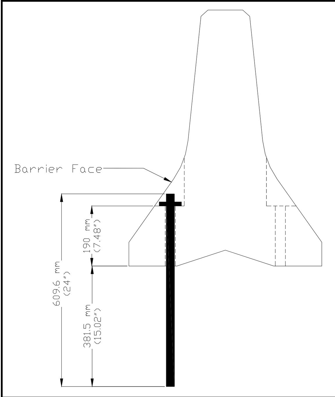
Figure 7-5. Typical Capped Stake Installation Layout
