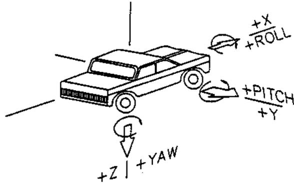
Figure 7-12. Vehicle Accelerometer and Gyro Sign Convention
