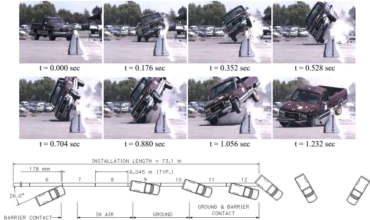
Figure 2-30. Test 672 - Impact sequence and diagram
