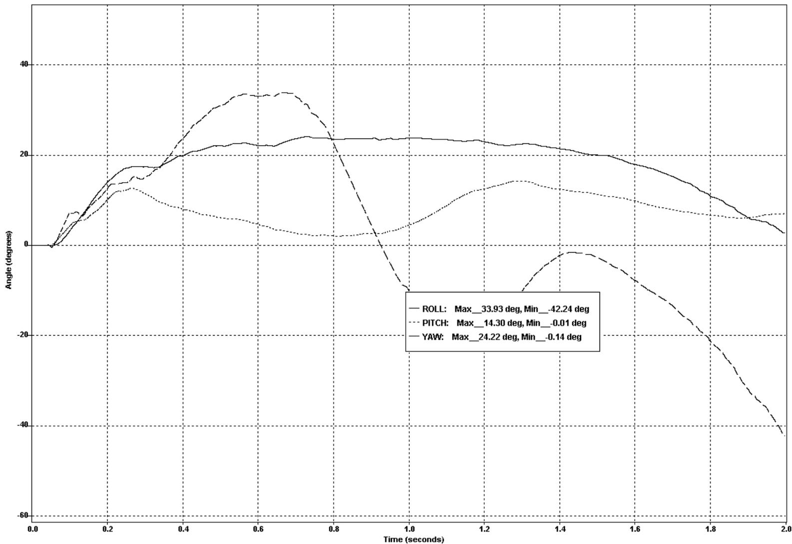
Figure 7-17. Test 671 Vehicle Roll, Pitch, and Yaw Vs Time
