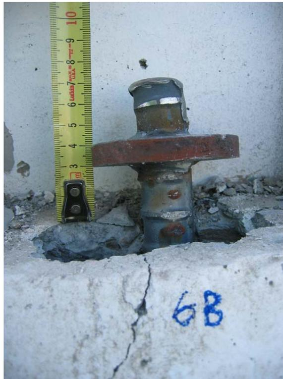
Figure 2-39. Test 673 - Stake #6B Post-Impact
