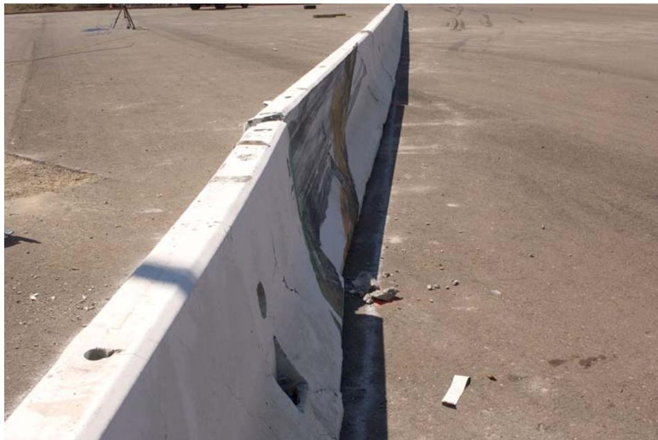
Figure 2-37. Test 673 - Downstream View of Barrier Post-Impact
