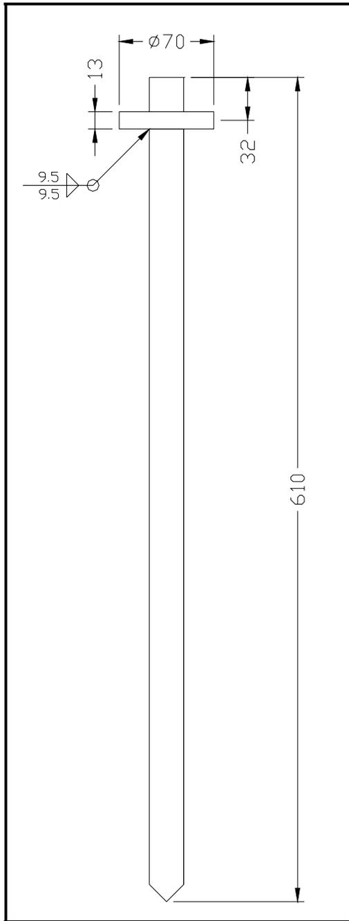
Figure 7-6. Capped Stake Dimensions [mm]
