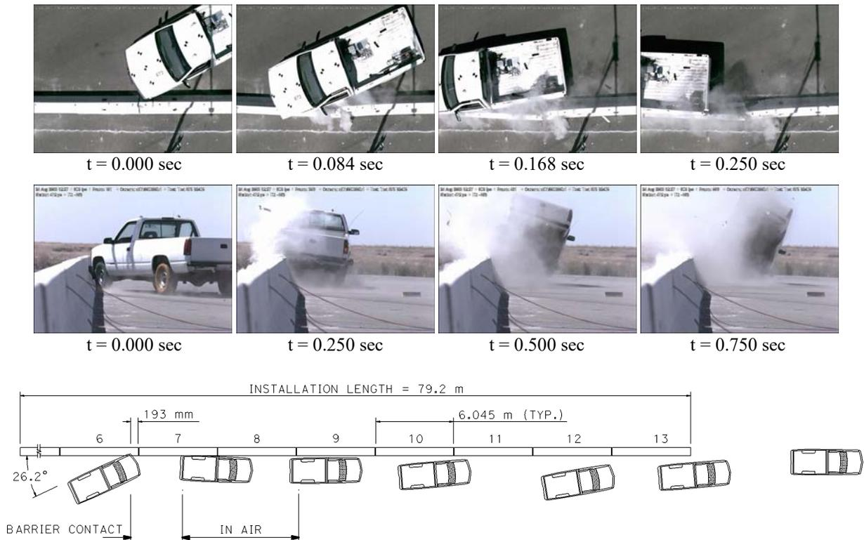
Figure 2-43. Test 673 - Impact sequence and diagram
