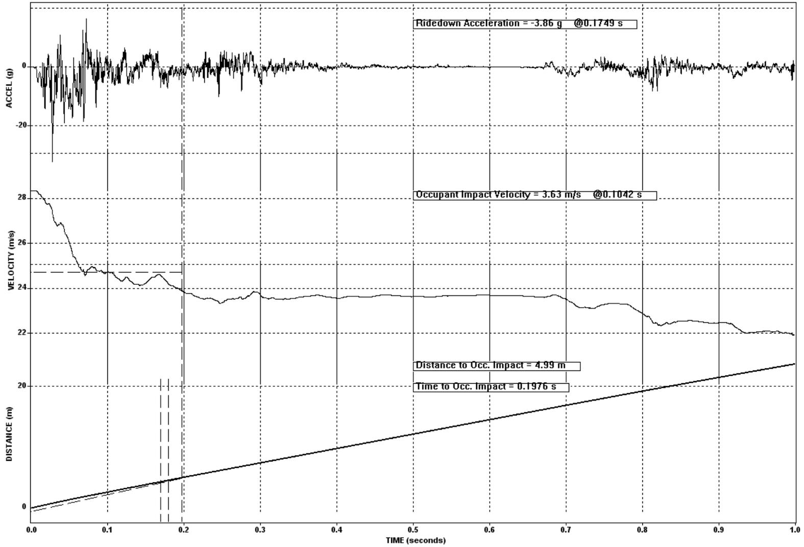
Figure 7-39. Test 676 Vehicle Longitudinal Acceleration, Velocity, and Distance Vs Time
