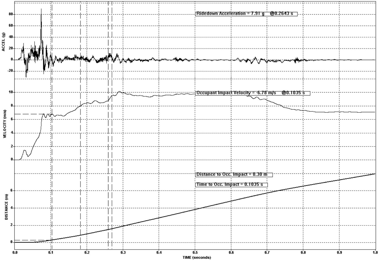
Figure 7-20. Test 672 Vehicle Lateral Acceleration, Velocity, and Distance Vs Time
