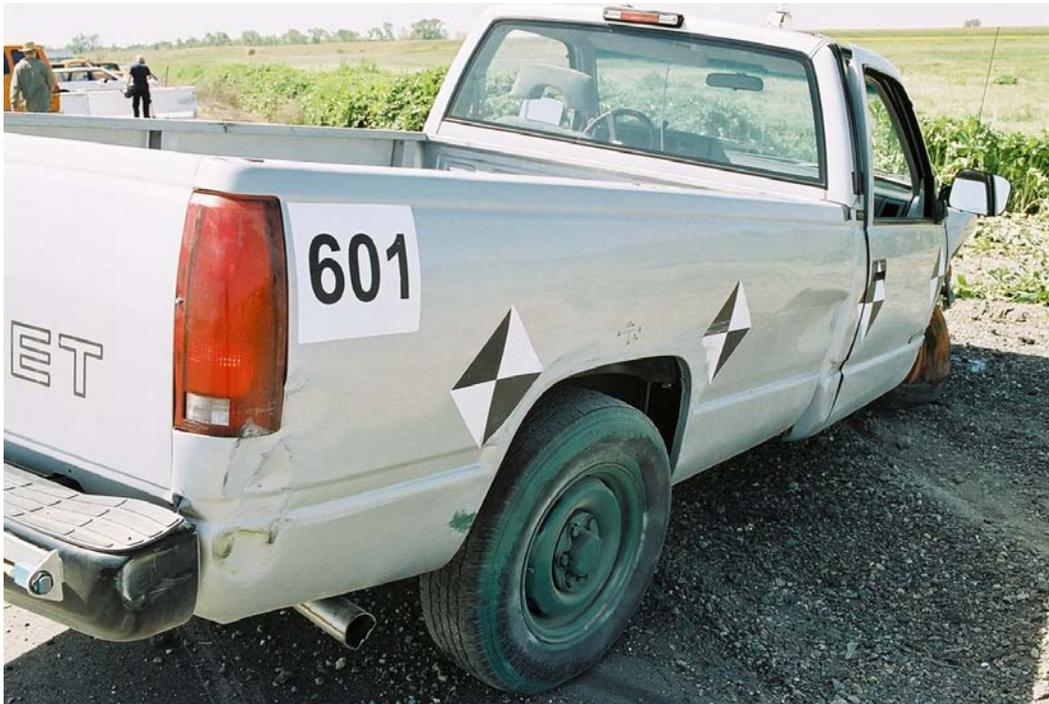
Figure 2-11 – Rear Right Side of Test Vehicle Post-Impact
