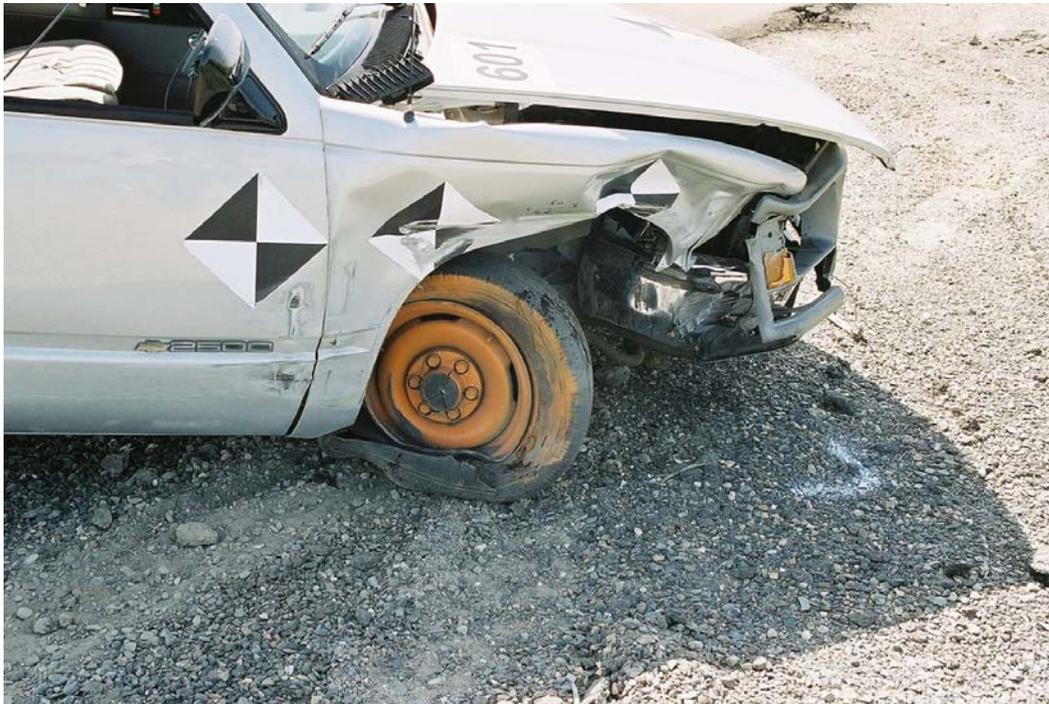
Figure 2-9 – Front Wheel of Test Vehicle Post-Impact
