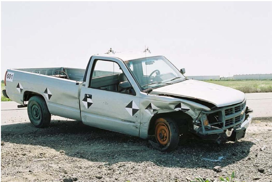
Figure 2-10 – Front Right Corner of Test Vehicle Post-Impact
