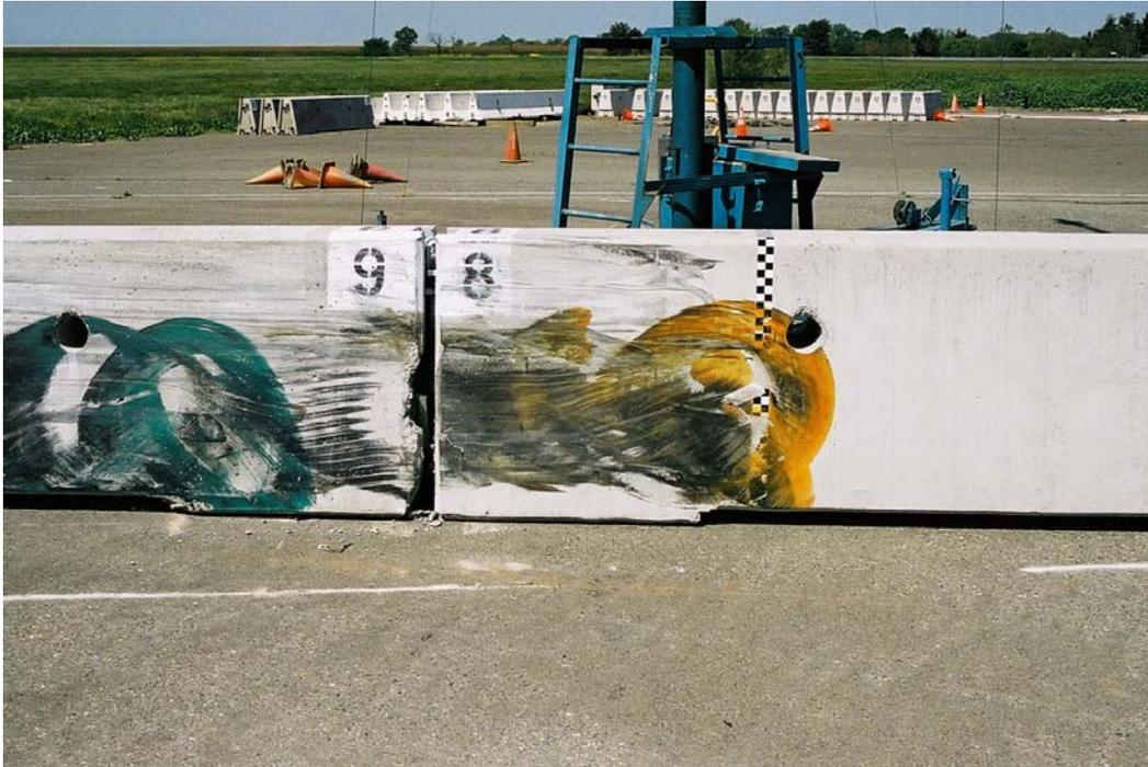
Figure 2-13 – Barrier Damage near the Impact Point
