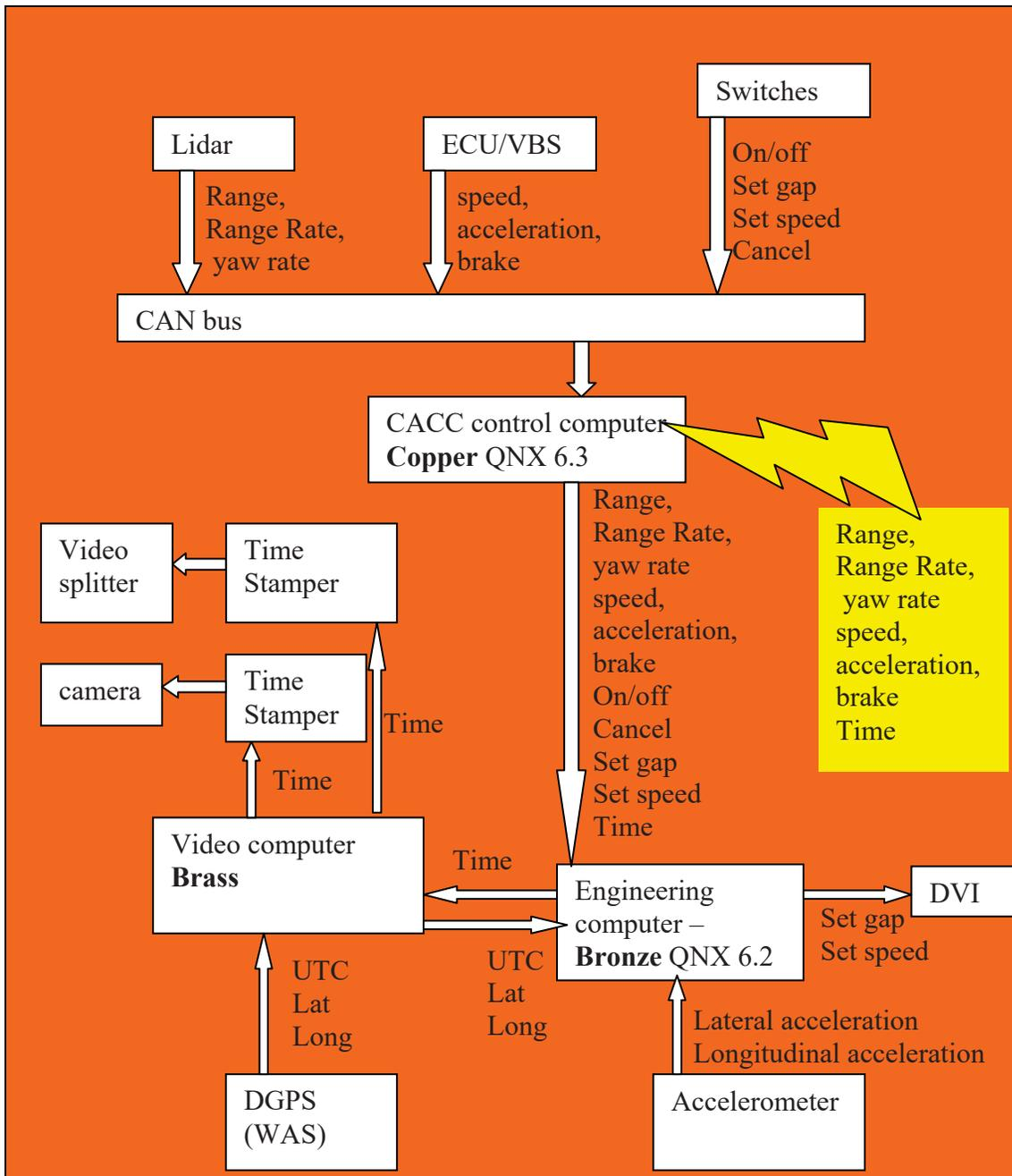
Figure 34: DAS Data flow for Copper (CACC) Vehicle
