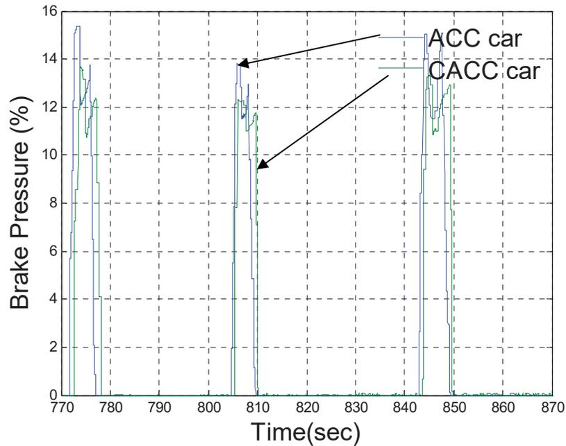
**Figure 24: Three car platoon test – brake pressure**
