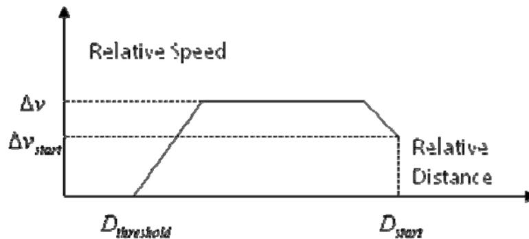
**Figure 9: Trajectory Planning for CACC Gap Closing Controller**
