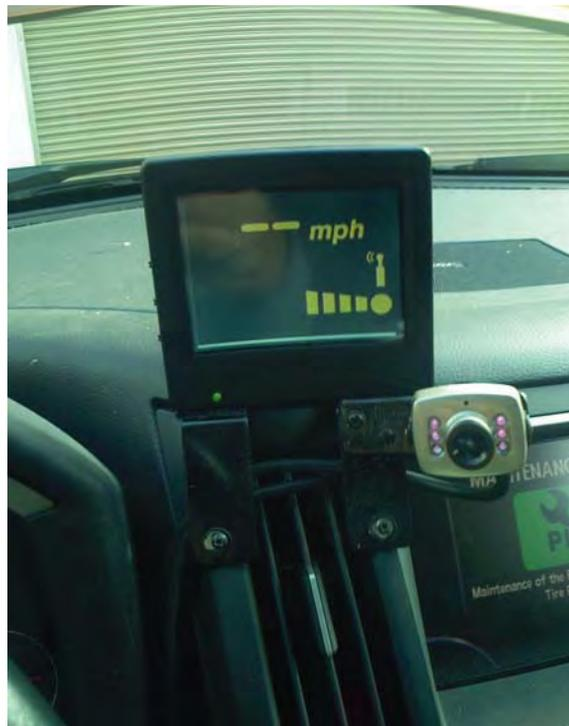
**Figure 27: CACC display (right of steering wheel)**
