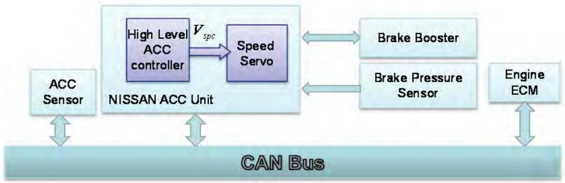
**Figure 3: Configuration of Existing Nissan ACC Controller**
