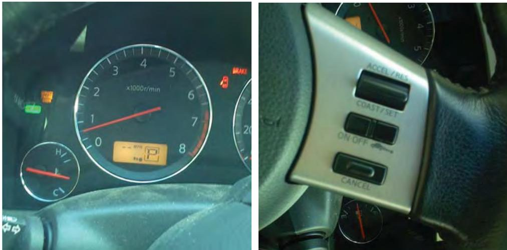
**Figure 26: ACC displays (left) and controls (right)**
