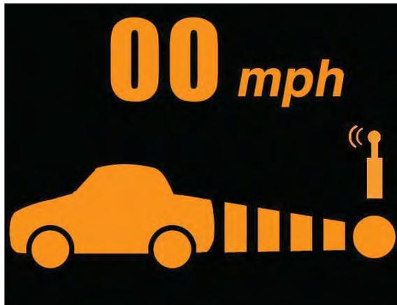
**Figure 28: CACC Driver Vehicle Interface**
