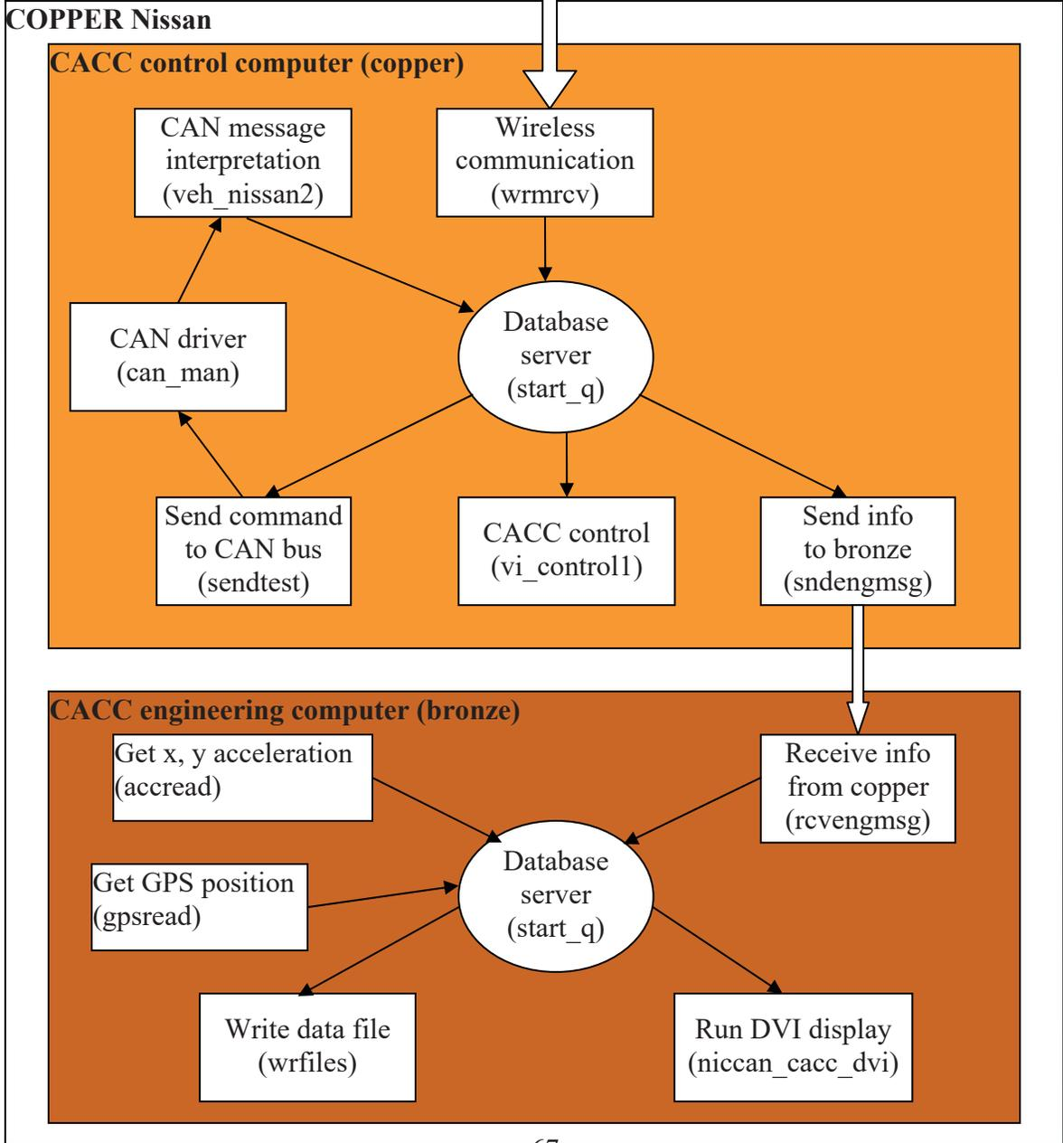
Processes on the Copper Nissan **copper** computer (CAN Message contents):
