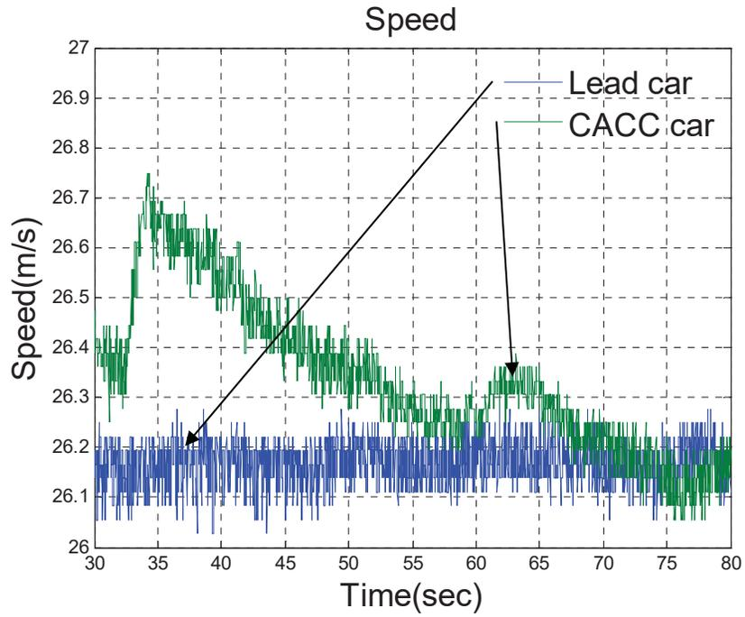
**Figure 10: Proving ground test: steady state speed performance**
