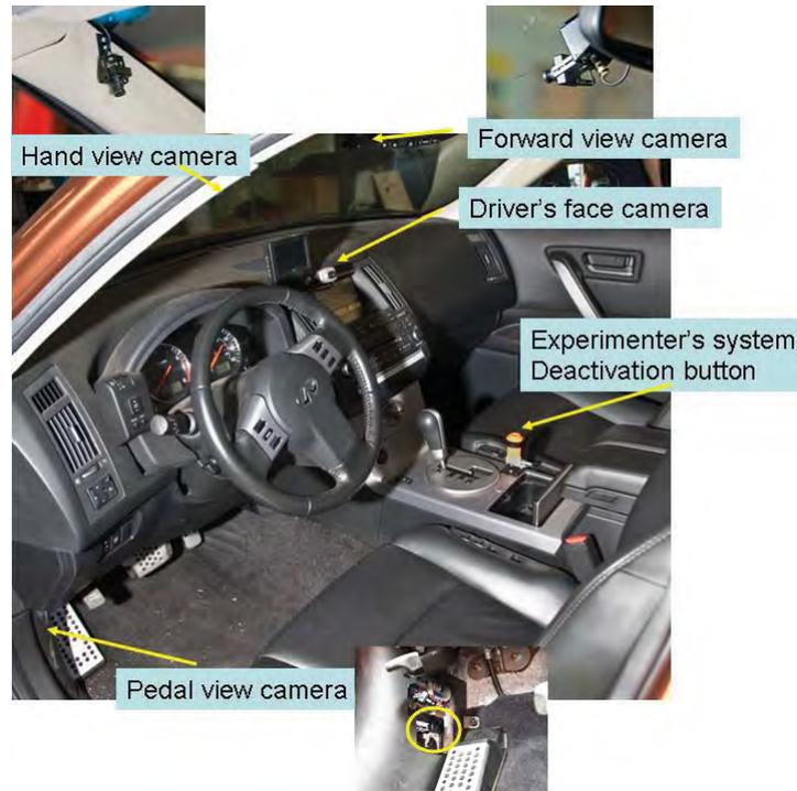
**Figure 32: Vehicle Interior, Showing Locations of Video Cameras**
