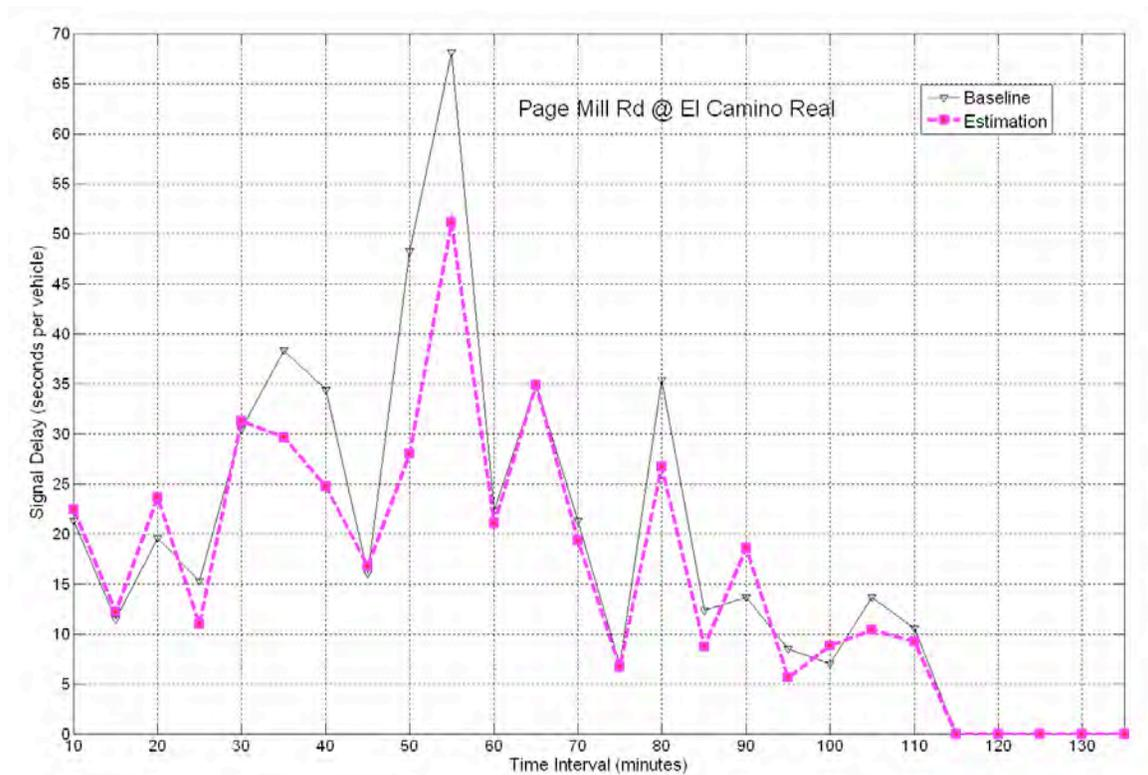
**Figure 3-4 Estimation of signal delay for Page Mill Rd @ ECR (heavy traffic)**
