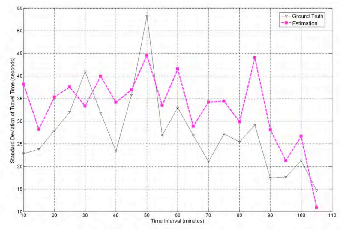
**Figure 3-7 Estimated standard deviations for arterial travel times**
