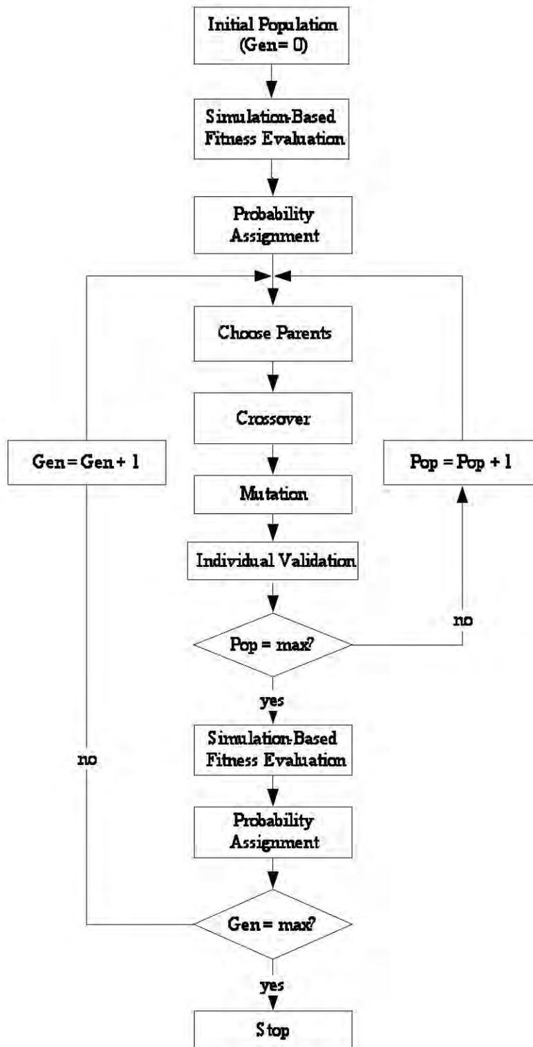
**Figure 6-7** Flow Chart of the Simulation-Based GA
