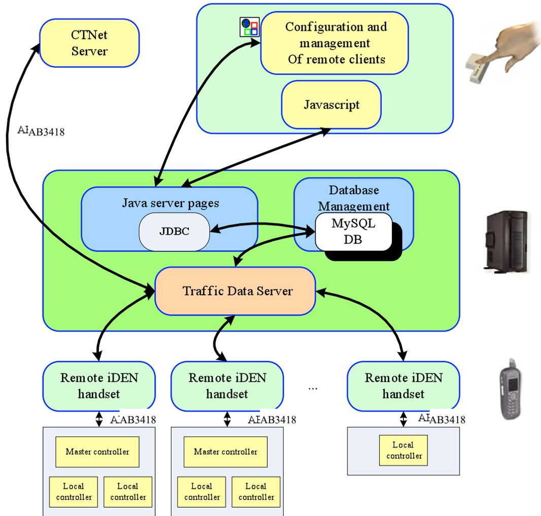
**Figure 2-2 System architecture**
