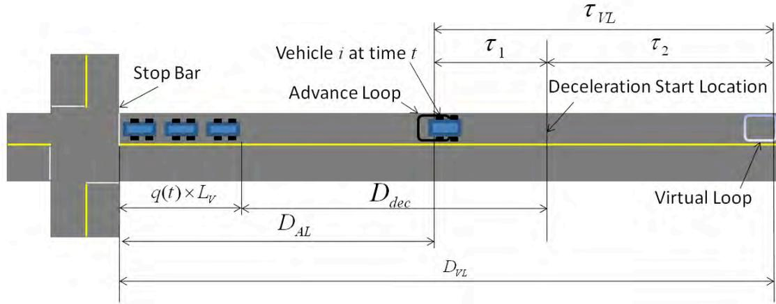
**Figure 3-2 Virtual loop method for Scenario I**
