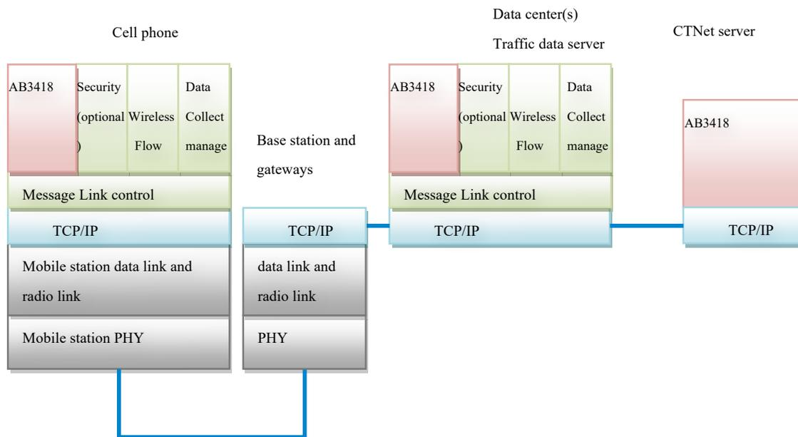
**Figure 2-16 Protocol stack and traffic data server**
