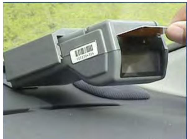
**Figure 4: Transponder and Smart Card (EPVIS 2002)**
