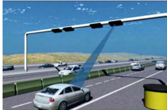
**Figure 2: Roadside antenna communicates with vehicle-mounted transponder via DSRC (TransNet 2008)**
