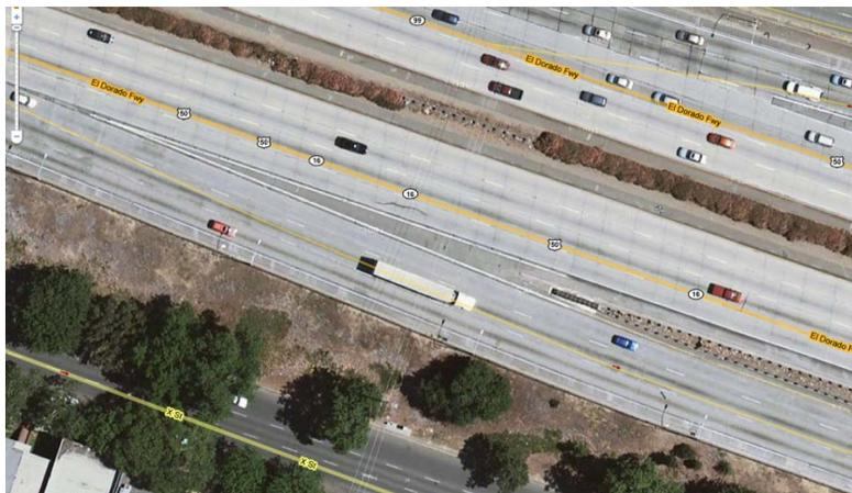
**Figure 9: Shows the attenuator's location and the associated virtual gore point. The virtual gore point is the point where the lane lines diverge to direct traffic. The term "virtual" is used since there is no physical barrier.**
