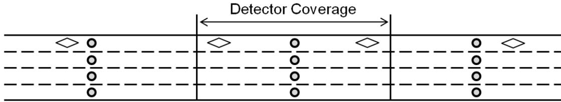
**Figure 5. Detector coverage**
