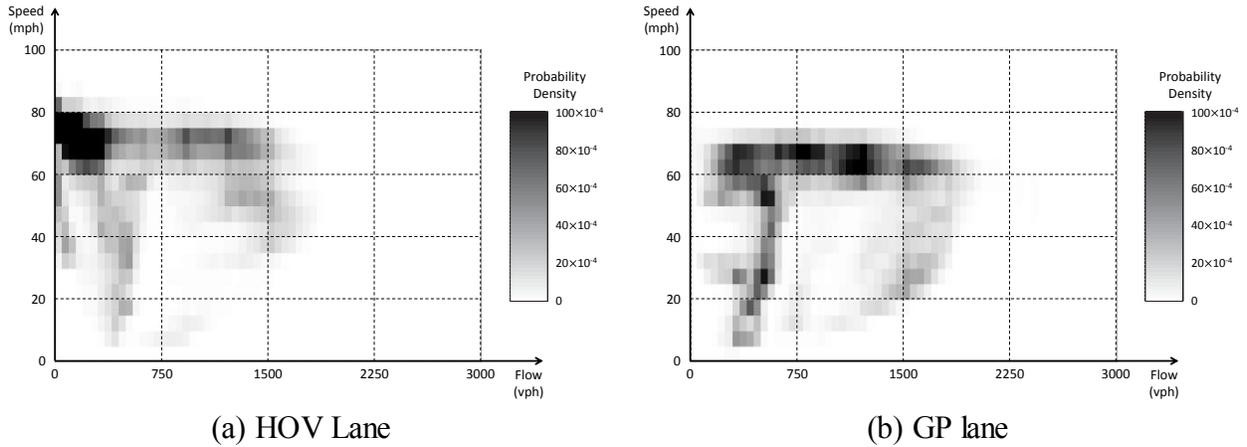
**Figure B1. Probability density of speed-flow: (a) HOV lane, and (b) GP lane (Interstate 80 Eastbound, District 4)**
