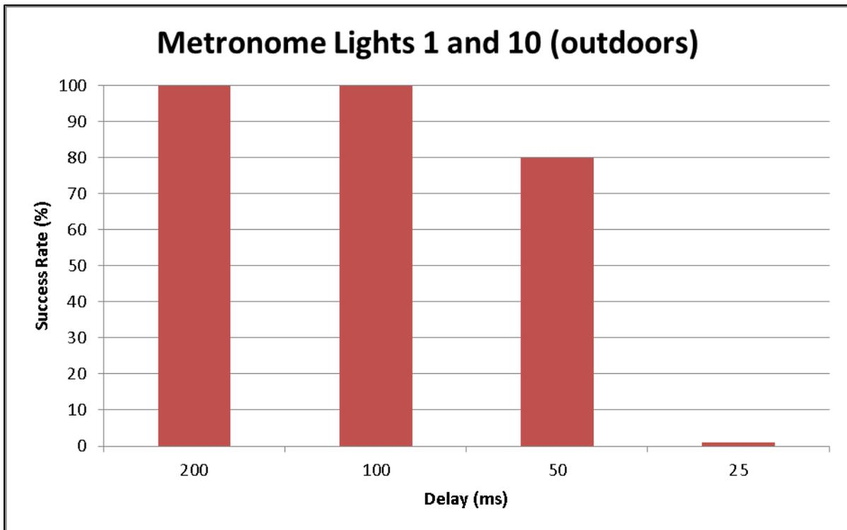
Figure 16: Outdoor Metronome Test Results
