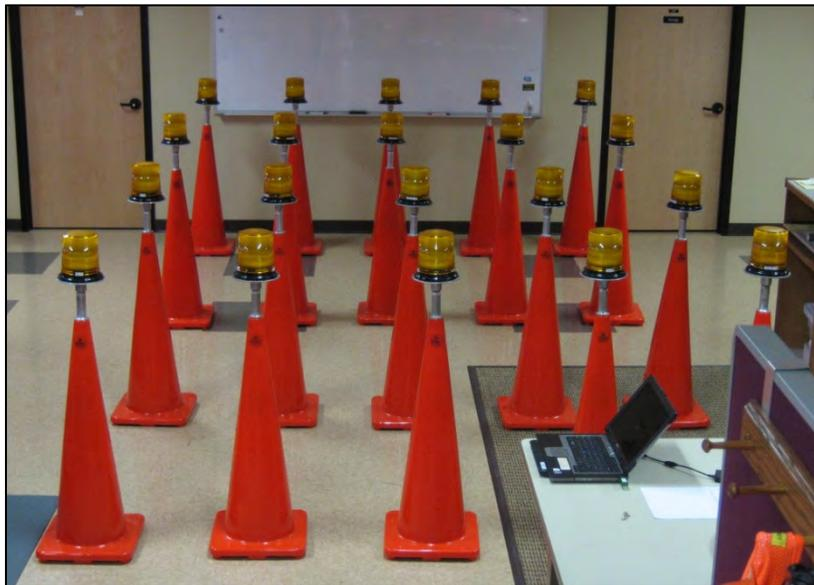
**Figure 13: Laboratory Light Pattern Testing - WTI Photo**
