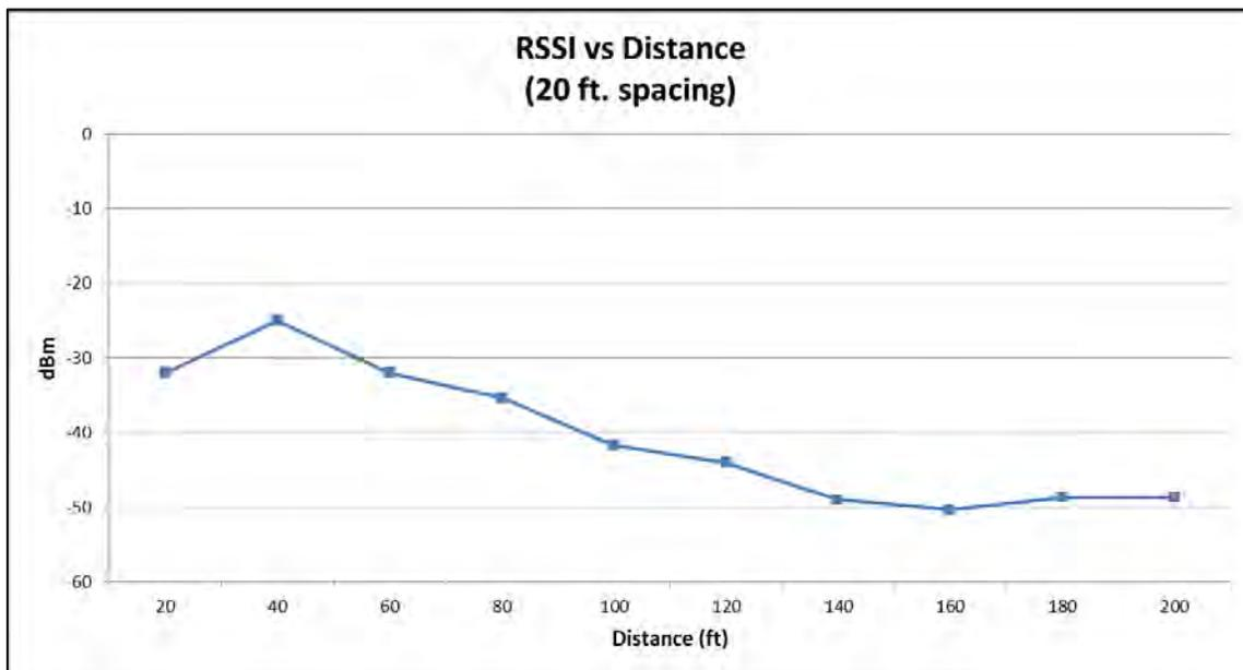
Figure 12: RSSI Values for 20 feet Spacing
