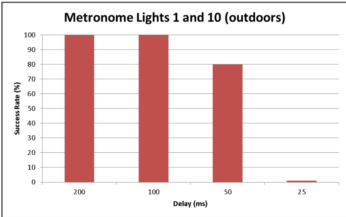
Figure 16: Outdoor Metronome Test Results
