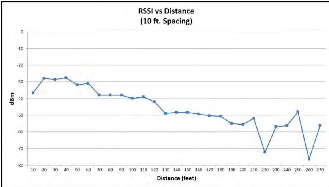
Figure 11: RSSI Values for 10 feet Spacing
