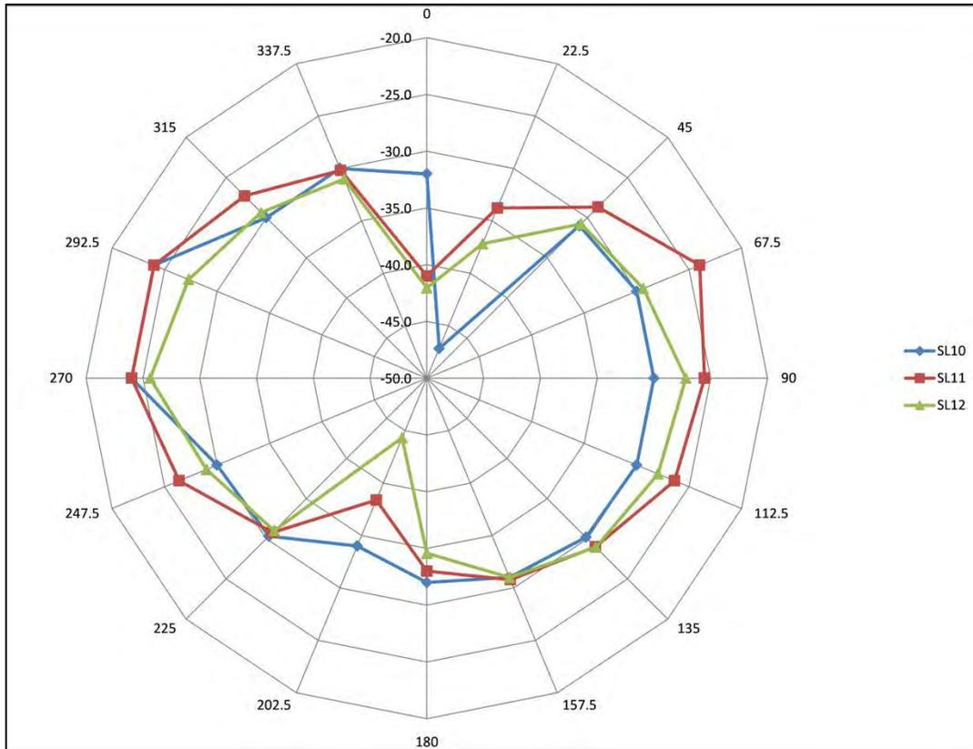
**Figure 9: XBee Radio Antenna Patterns**
