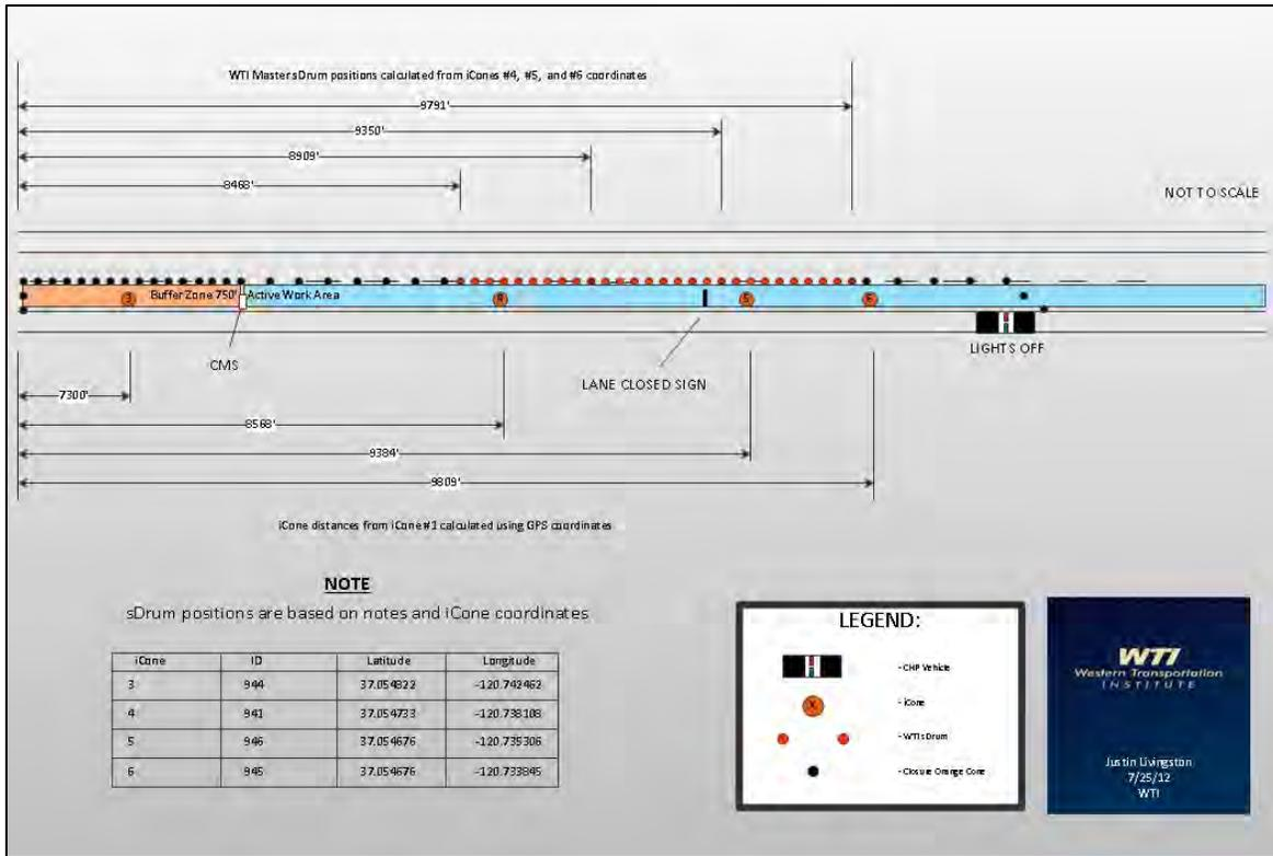
Figure 63: sDrum and iCone Locations for 6/22/12
