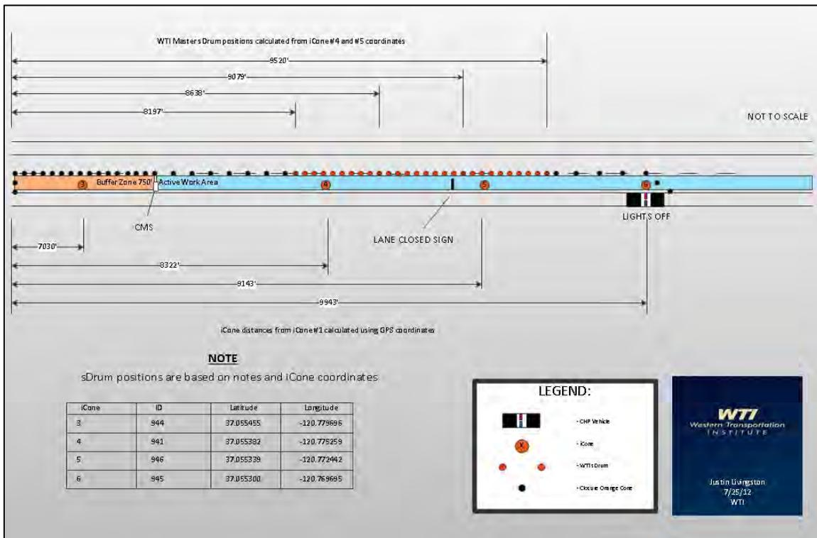
Figure 62: sDrum and iCone Locations for 6/21/12
