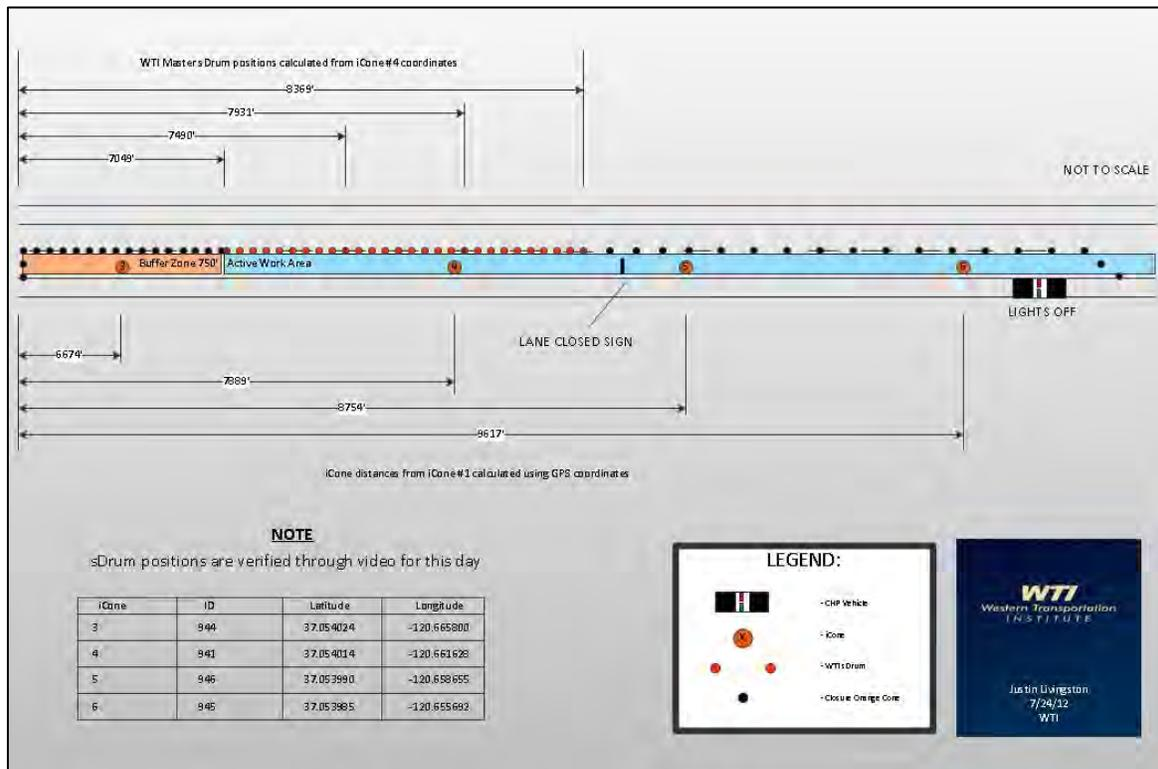
Figure 58: sDrum and iCone Locations for 6/15/12
