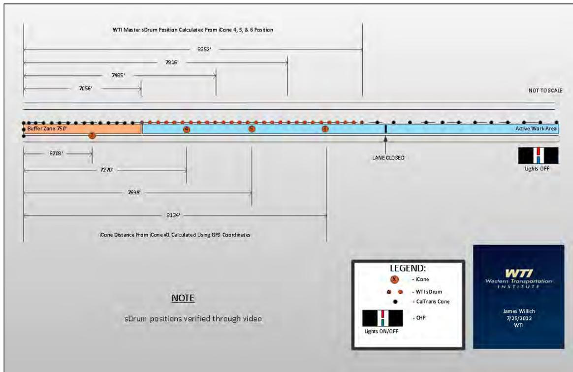
Figure 48: sDrum and iCone Locations for 5/17/12
