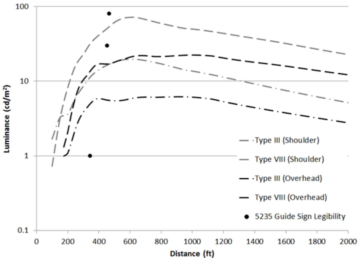
Figure 2.1. ASTM Type and Legibility Distance versus Luminance.
