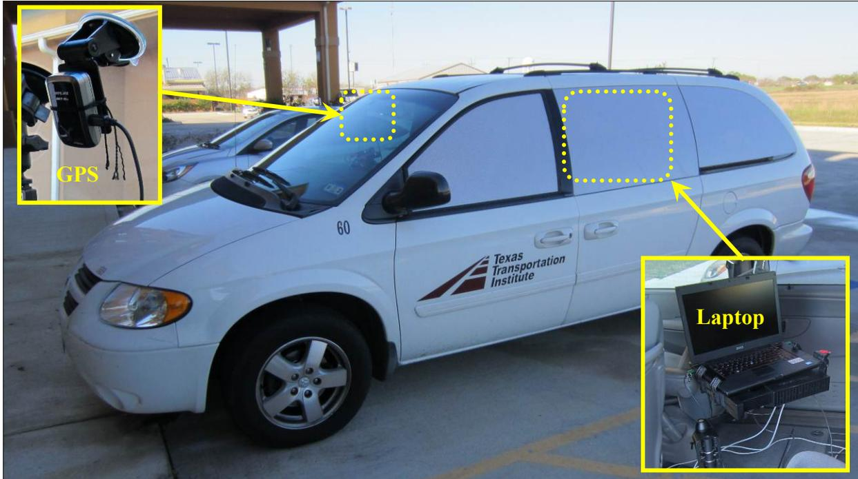
**Figure 3.6. Instrumented Vehicle.**
