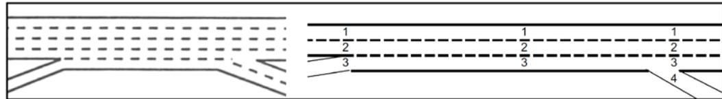
**Figure 6.1 Typical Balanced Weaving Sections**
