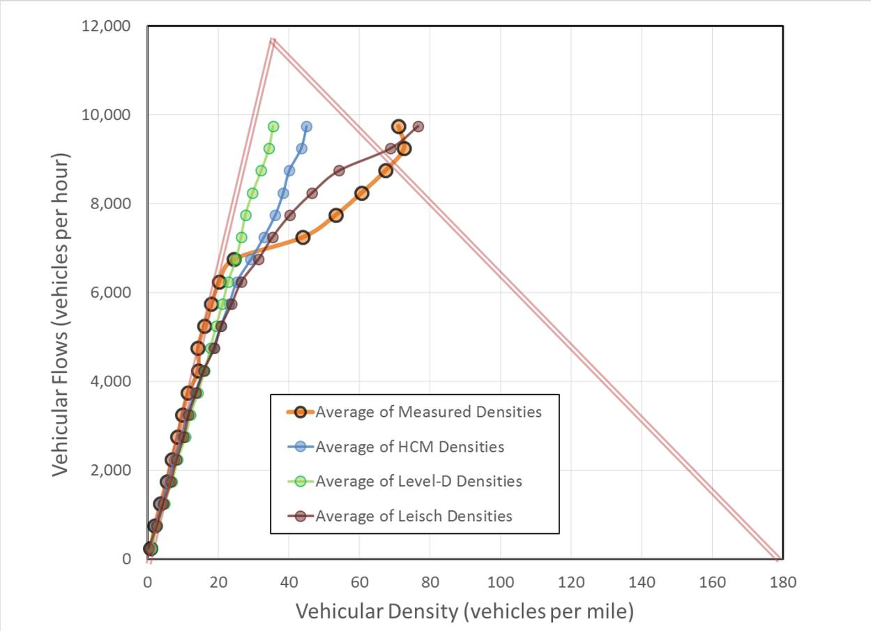
**Figure 5.6 Site #3, Density-Flow-Diagram with Trend-lines for Measured and Predicted Densities**
