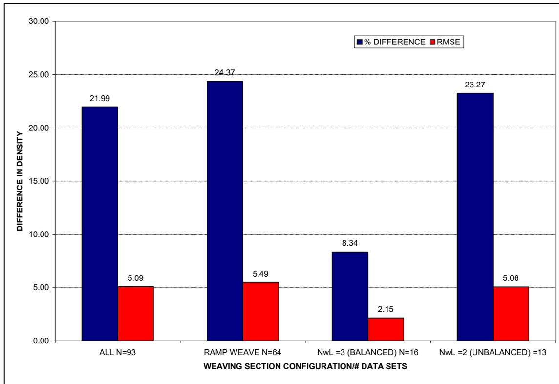
**Figure 3.1 Measured vs. HCM2010 Predicted Densities**
