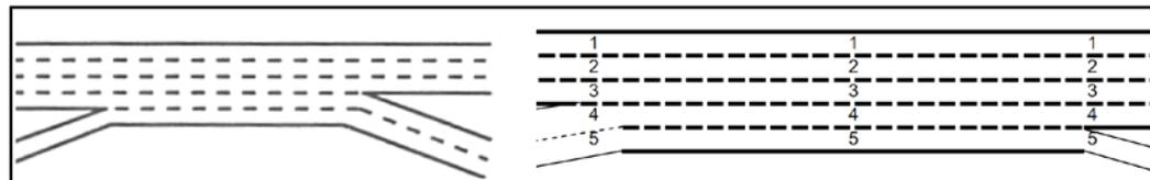
**Figure 6.2 Typical Unbalanced Weaving Sections**
