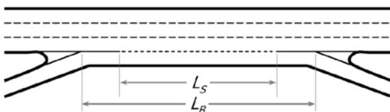
**Figure 2.2 Weaving Section Length (source: Exhibit 12-2, HCM2010)**
