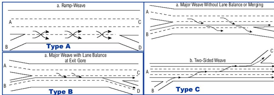
**Figure 2.1 Configurations of Freeway Weaving Sections (HCM2000/1985)**
