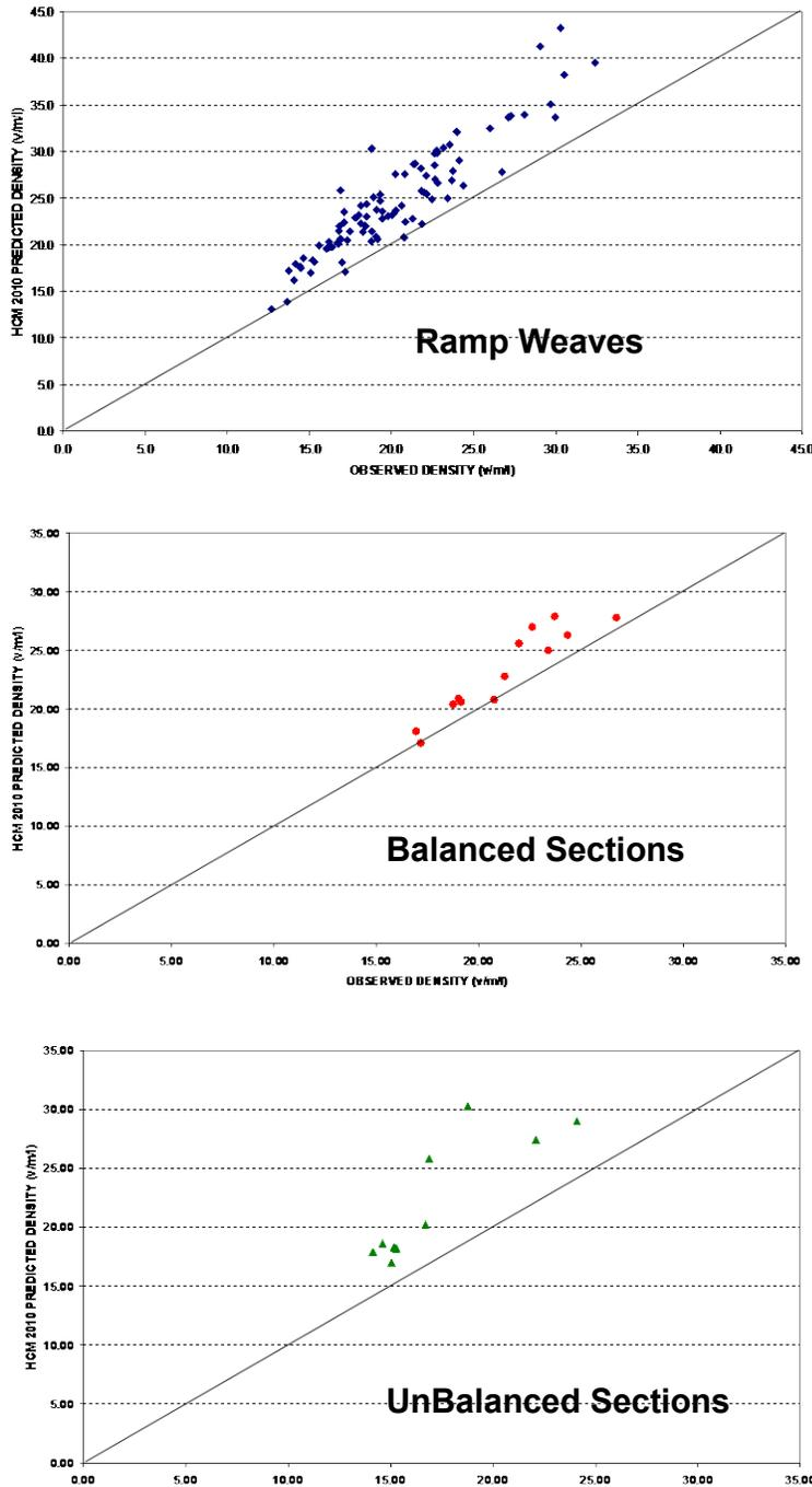
Figure 3.2 Measured vs. HCM2010 Predicted Densities per Weaving Section Configuration
