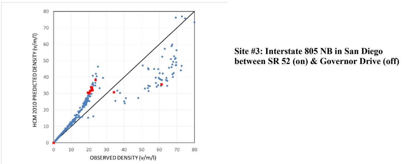
**Figure 5.3 Measured vs. Leisch Predicted Densities for Ramp Weave Site #3**
