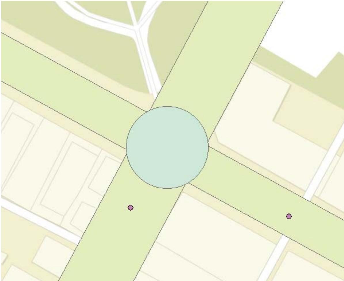
*Figure 19. Two screenline counts, located on segments. Each count informs the segment on which the count is located, as well as the segment directly on the other side of the intersection that is between them. Together, the counts inform the intersection.*
