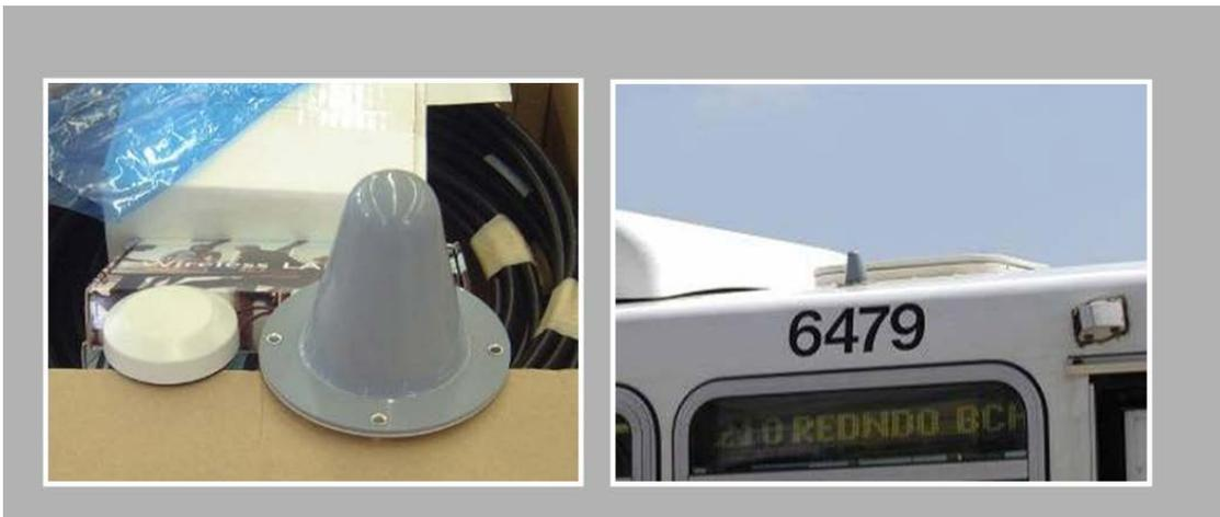
**Figure 4-10: Typical GPS and Wireless Communications Antenna Installation**
