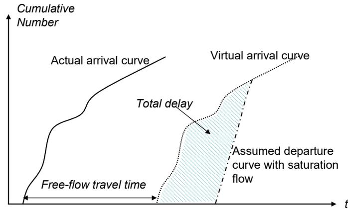
**Figure 5-7: Delay Calculation Concept using only Advance Loop Counts**
