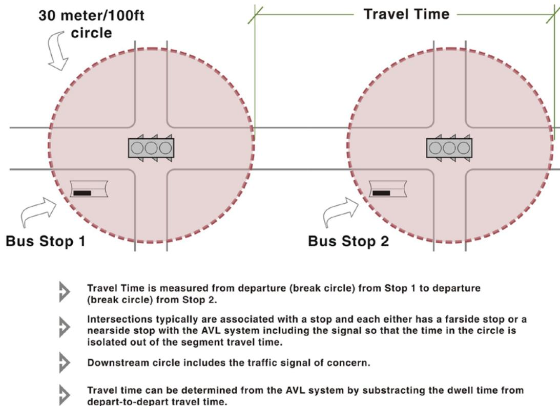
**Figure 4-30: Sample Segment Analysis Using AVL System**
