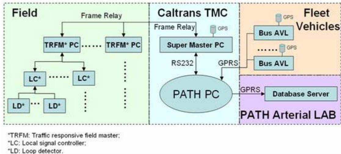
**Figure 4-24: System Architecture of the ATSP System**
