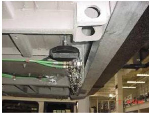
**Figure 4-21: Inductive Loop Transponder Mounted on Underside of a Bus**
