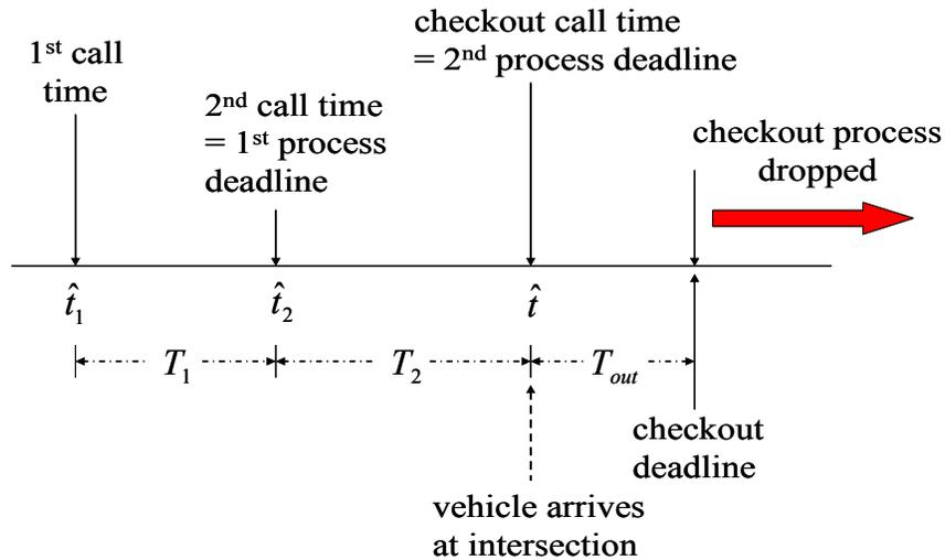
**Figure 7-15 Timelines of multiple priority request processes**
