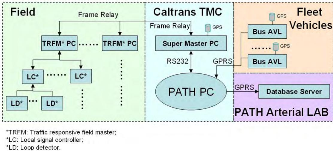
Figure 5-1 ATSP System Hardware Architecture
