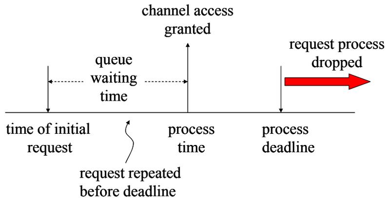
**Figure 7-10 Timeline of a single priority request process**
