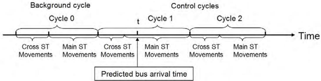
**Figure 4-5 Background cycle and control cycles**
