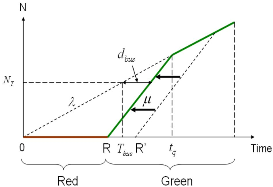
**Figure 4-6 N-T curve for bus movement with TSP**
