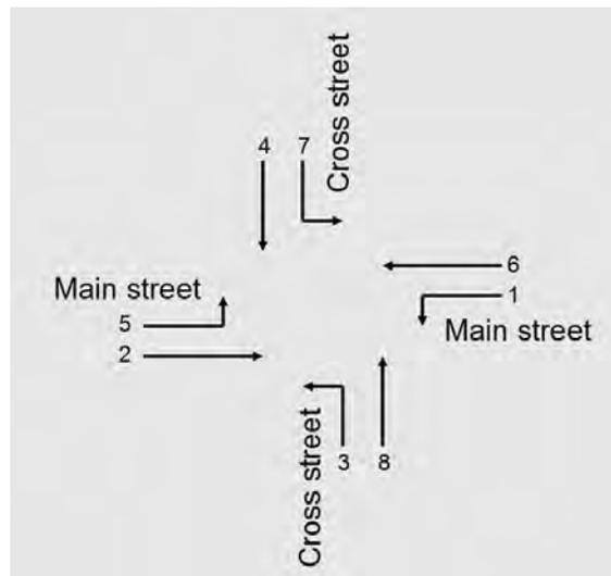
**Figure 4-1 Definitions of standard NEMA 8 movements**
