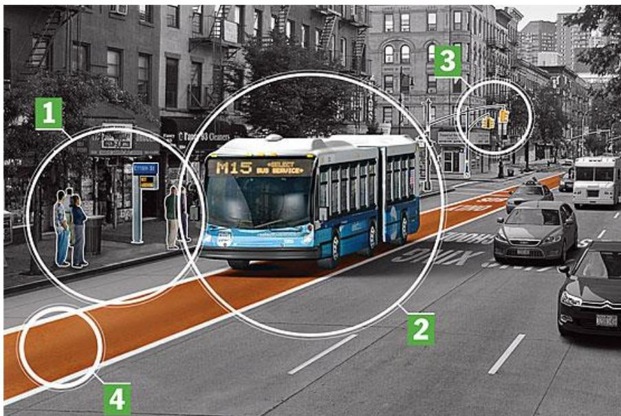
**Figure 2:** *New York City’s Select Bus Service represents an enhancement of the city’s local buses. The labels refer to (1) off board fare collection, (2) ability to board at any door, (3) signal priority and restricted left turns, and (4) a dedicated and camera enforced bus lane.*
