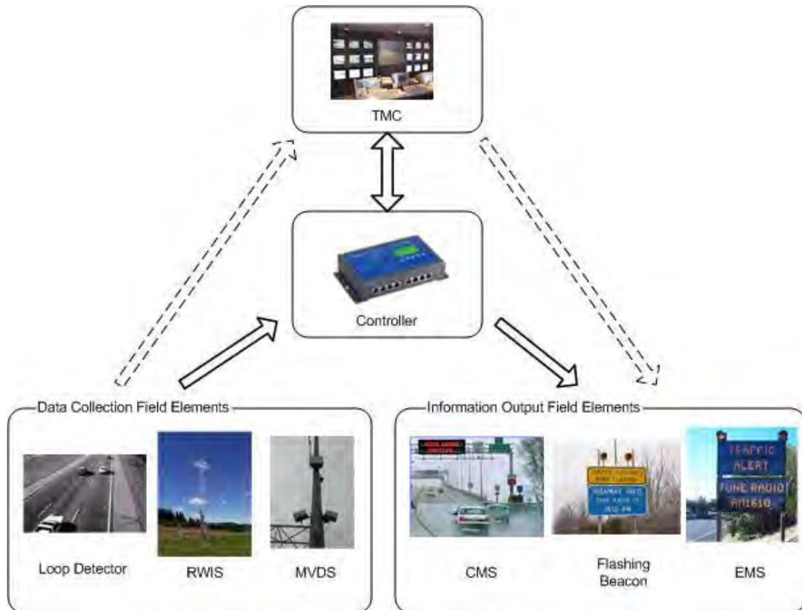
Figure 1: Controller Interaction with TMC and Field Elements
