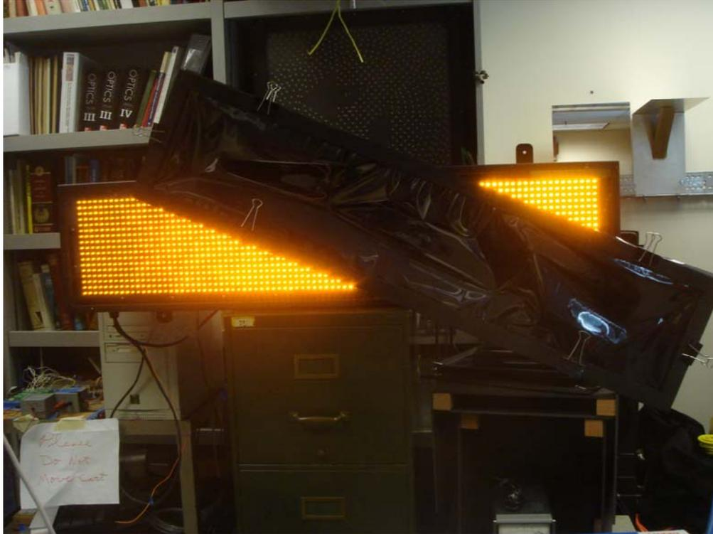
**Figure 19:** A demonstration of how effectively the plastic sheeting can attenuate the light.
