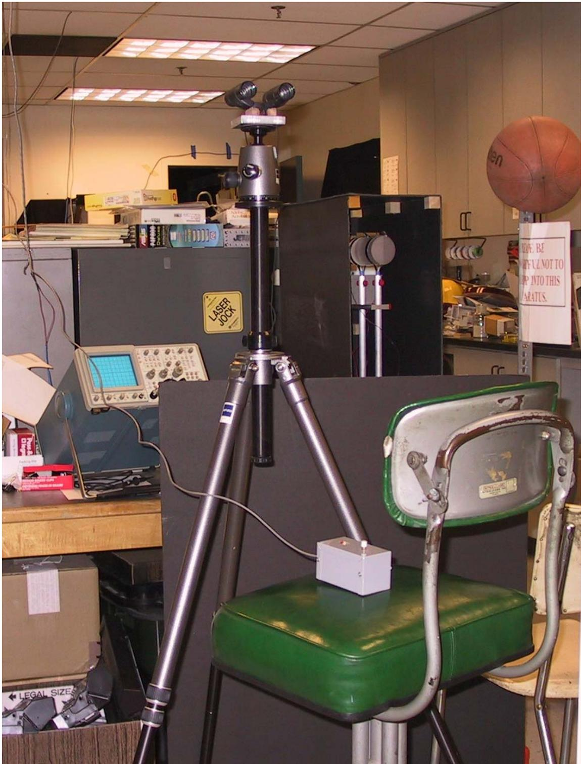
**Figure 21: The subject's high chair and reaction time response button at the opposite end of the room about 25 feet from the light bar. (The inverted binoculars mounted on a tripod were not used nor present during the test.)**
