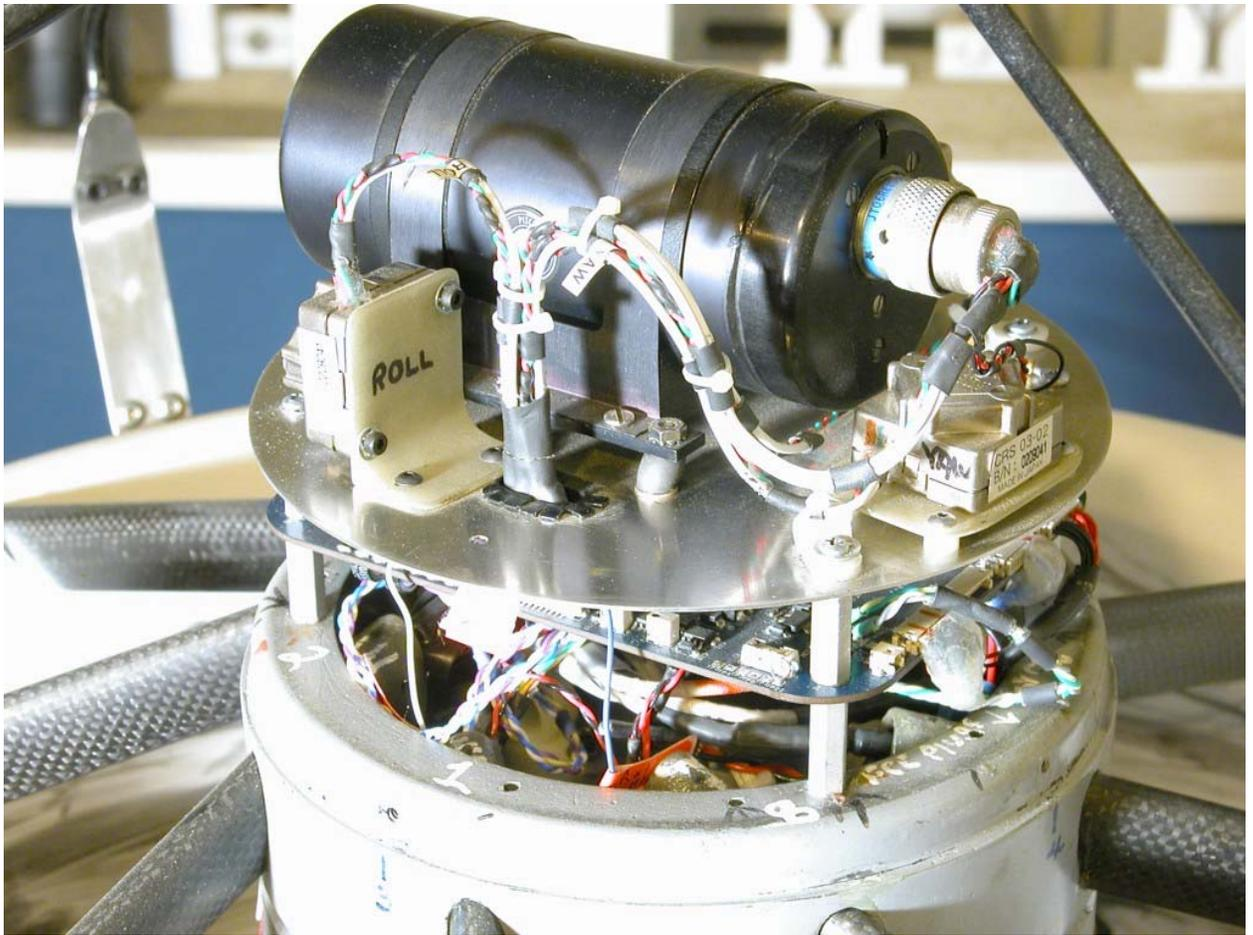
The sensor signals are passed through low-pass filters before entering the micro controller to reduce the effects of high frequency noise that could provide a false signal down into the control system bandwidth due to the limited sampling rate of the micro controller.
