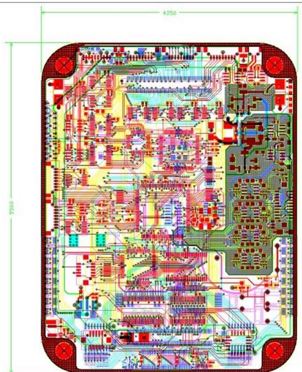
The FCC features a dual-channel high speed communications chip, an 8-Channel Octart chip (controls scoop command channels), 512 K Byte SRAM, 512 K Byte Flash program/parameter storage, programmable logic & decode, 8 K Byte program variable SRAM, and Analog signal conditioning circuits.
