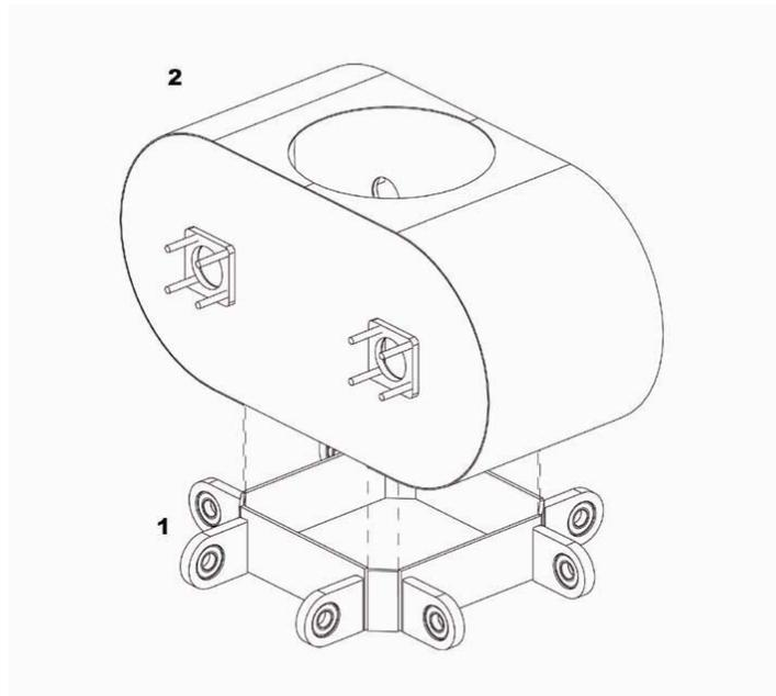
Figure 8.5 Housing assembly: 1) arm mounting ring & 2) cutter housing
