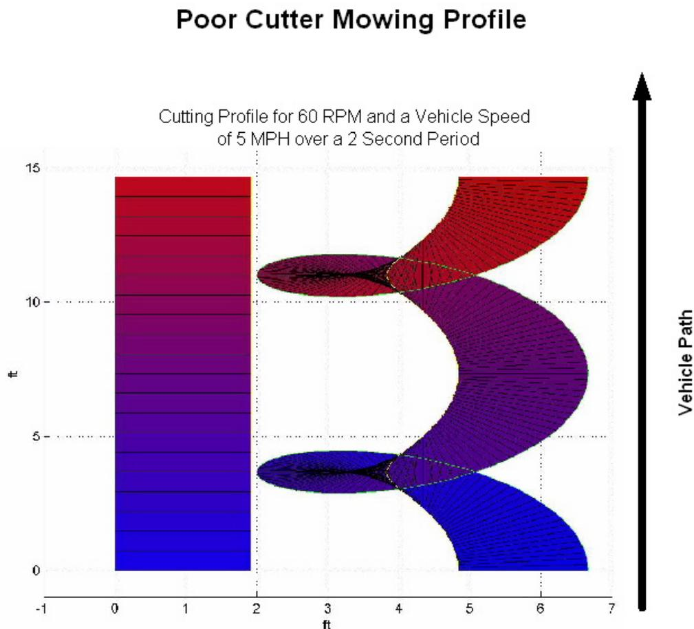
Figure 4.13 A poor cutter mowing profile.
