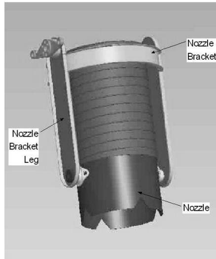
*Figure 3.11 Original Nozzle assembly.*
