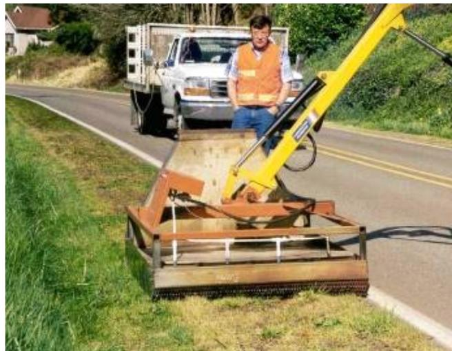
*Figure 2.7 Infrared vegetation control unit*
