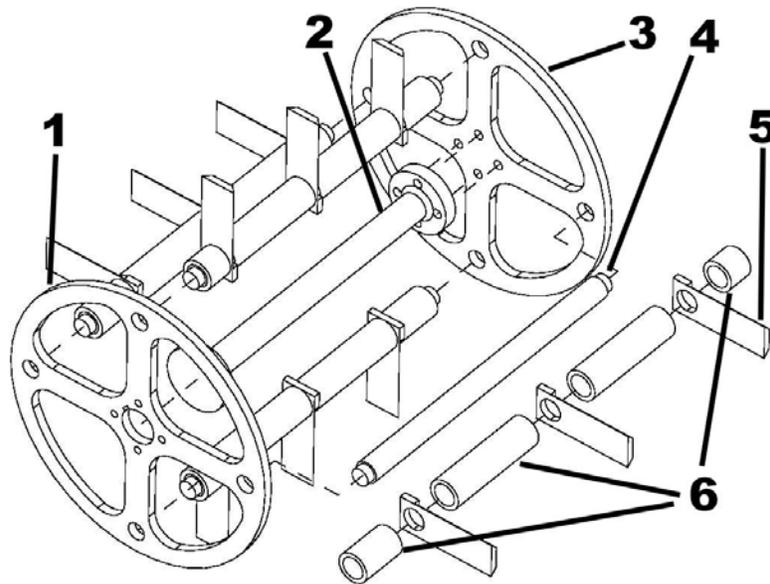
Figure 8.4 Cutter: 1) Motor Flywheel, 2) Drive Shaft, 3) Rear Flywheel, 4) Knife Shaft, 5) Blade, & 6) 3 Spacer sizes
