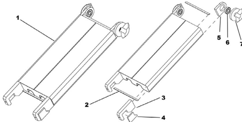
*Figure 8.9 Conveyor Belt Arm: an unassembled arm is on the left, and to the right is an exploded view of the unassembled arm. 1) Arm Frame, 2) Belt Scoop, 3) Tension Bracket, 4) Bracket Stiffener Plate, 5) Pillow Block, 6) Arm Bearing, & 7) Mitre Gear*
