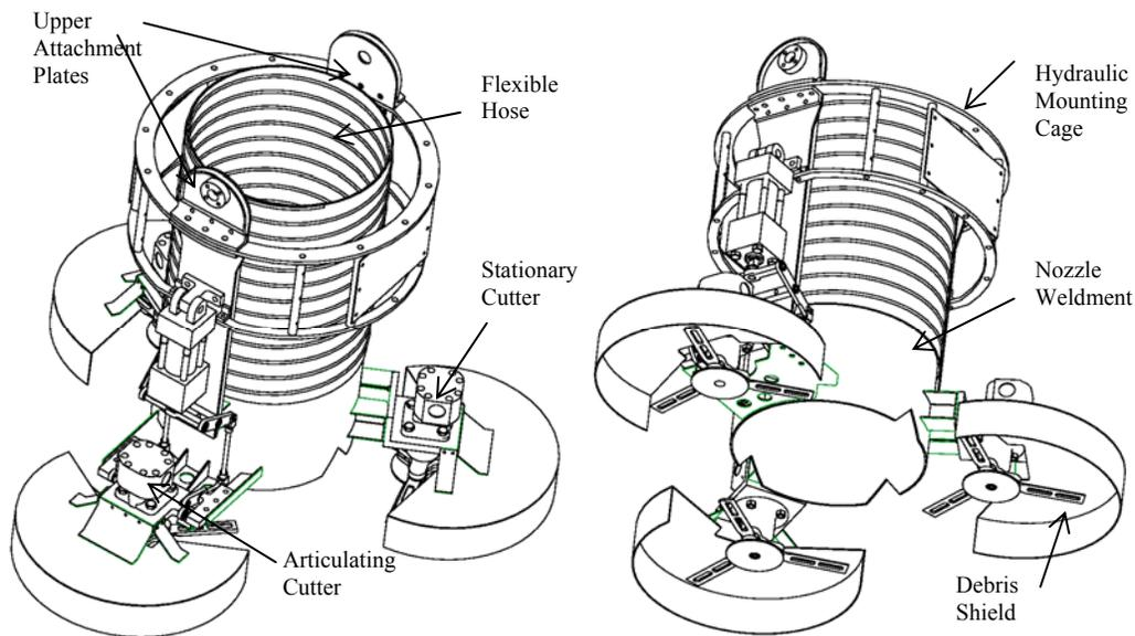
Figure 5.1 Rotary Impact Cutting Fixture Final Assembly
