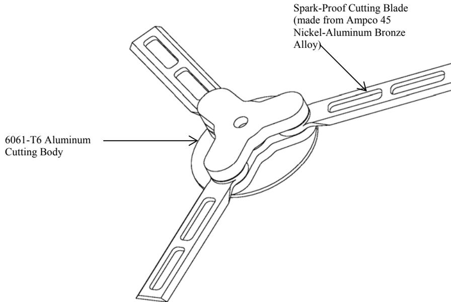
*Figure 7.12 Industrial High Performance (IHP) Cutting Head*
