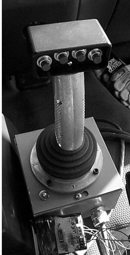
*Figure 3.15 Three-axis joystick controlling motions 5 – 7*
