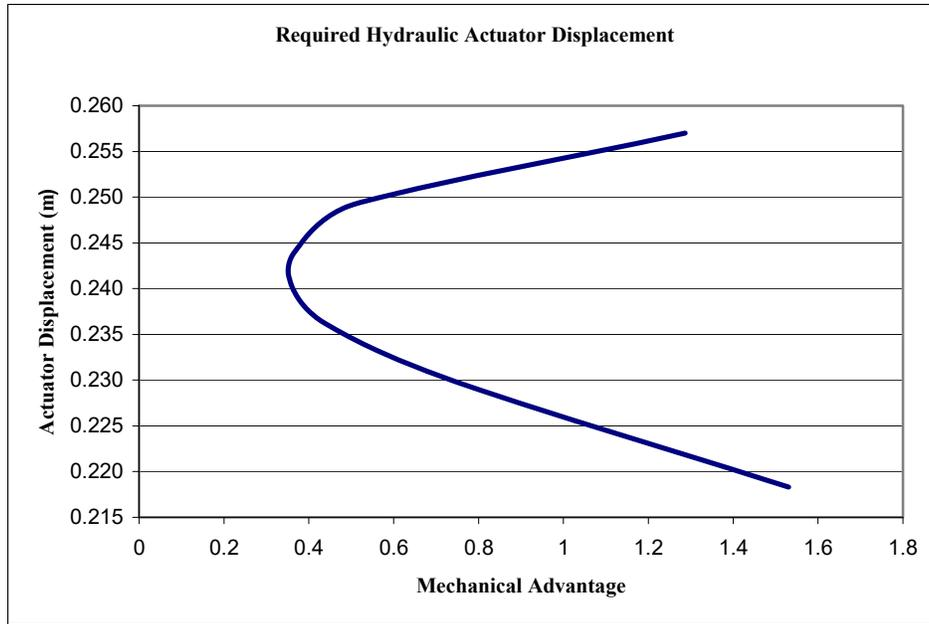
Figure 5.5 Mechanical Advantage for Full Actuator Input Displacement
