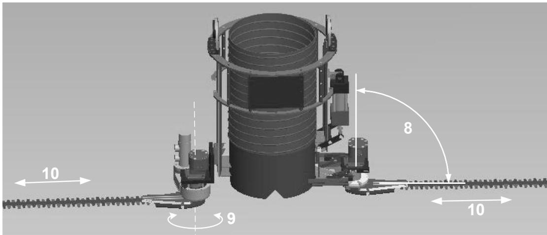
*Figure 4.5 Motions 8-10 of oscillating cutter system.*
