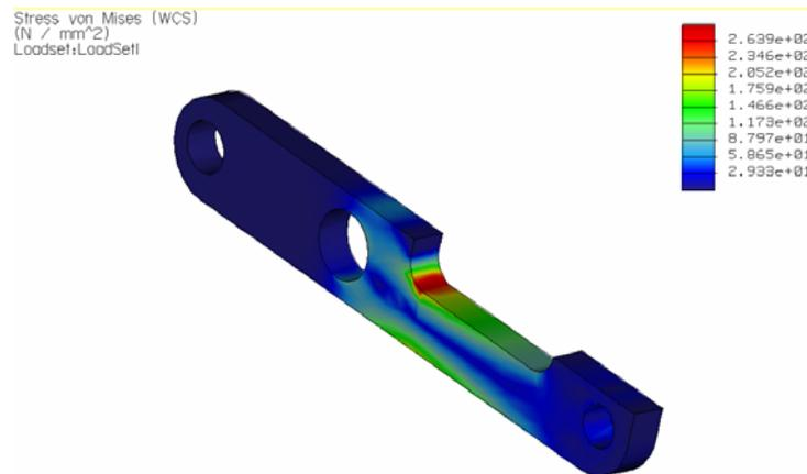
Figure 6.9 Result from Finite Element Analysis on Link-three
