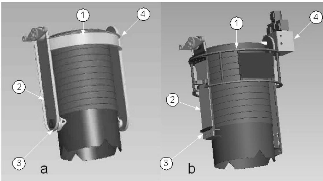
Figure 4.14 Four significant Nozzle Tip changes from the old design (a) to the new design (b).
