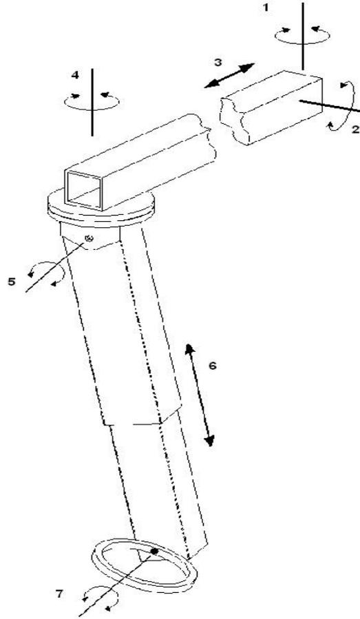
*Figure 3.5 Initial end-effector motion*
