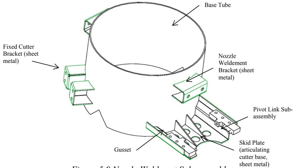
*Figure 5.9 Nozzle Weldment Sub-assembly*
