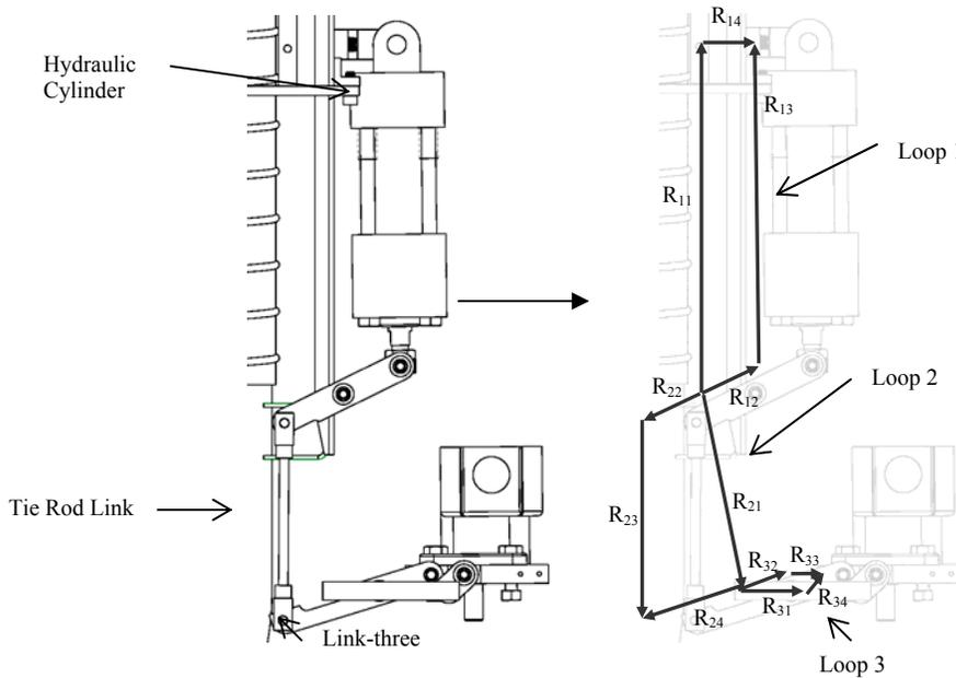
Figure 5.2 Mechanical Linkage and Corresponding Kinematical Vector Loops
