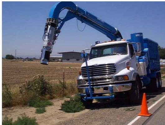
*Figure 3.3 Industrial vacuum vehicle with articulated boom.*
