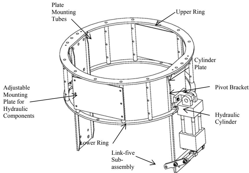
*Figure 5.7 Hydraulic Mounting Cage Sub-assembly*
