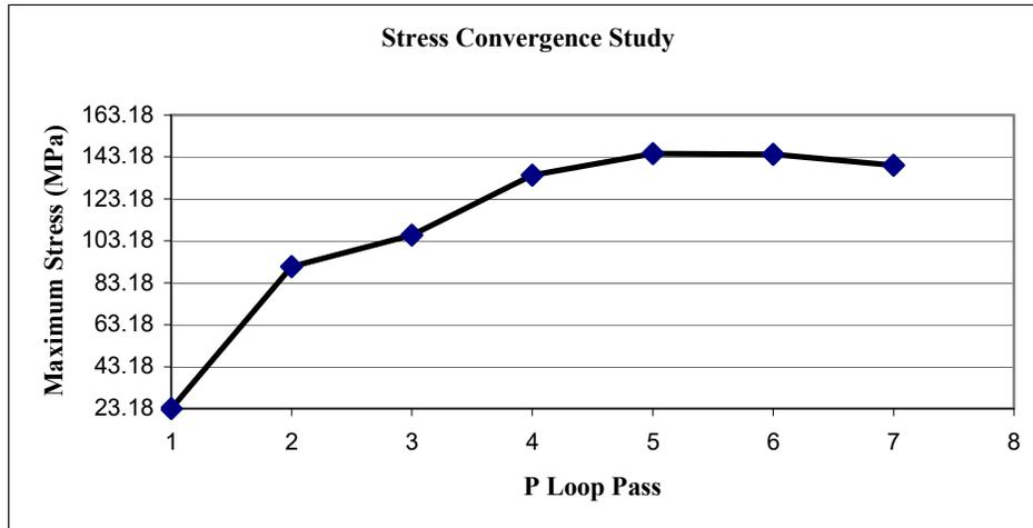
Figure 6.3 Stress Convergence for Skid Plate with Gussets
