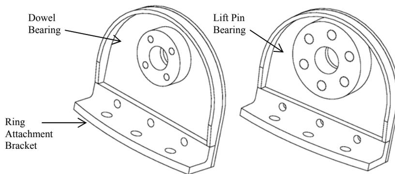
Figure 5.6 Upper Attachment Plate Sub-assemblies
