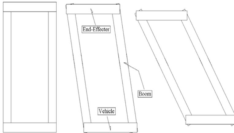
*Figure 3.6 Parallelogram maintains constant forward sweeping orientation.*
