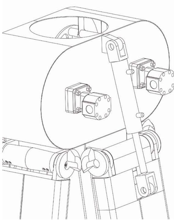
*Figure 8.20 Actuating Cylinder*
