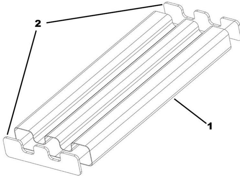
*Figure 8.7 Arm Frame: 1) Frame & 2) End Caps*
