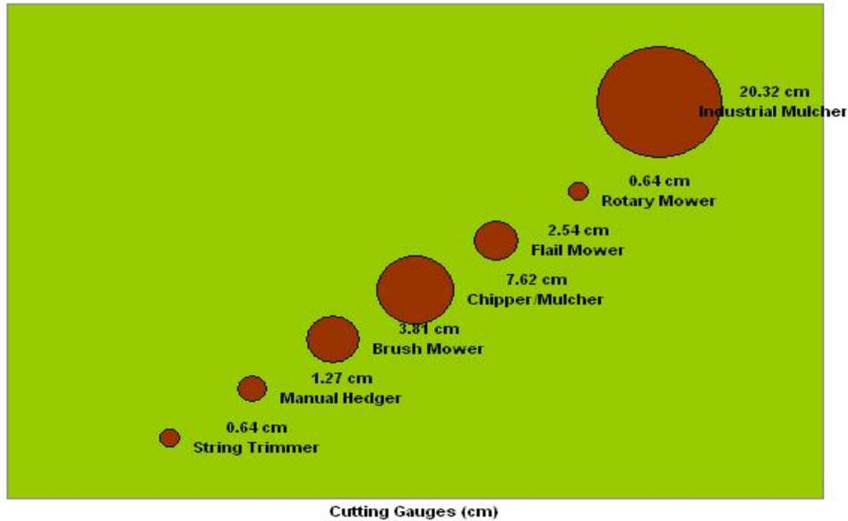
Table 4.3 Richardson's cutting gauge comparison.
