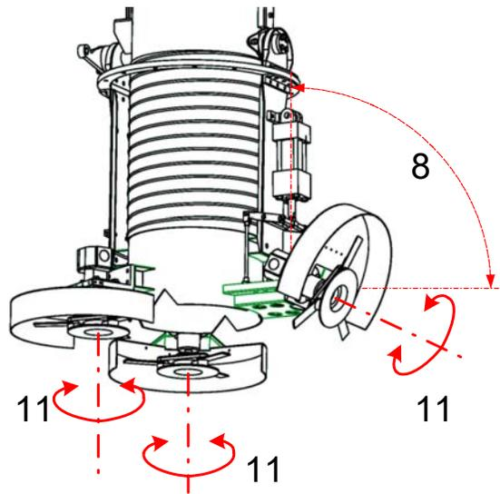
Figure 4.6 Motions 8 and 11 of the rotary cutter system.
