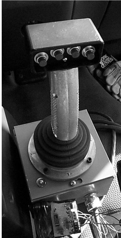
*Figure 3.15 Three-axis joystick controlling motions 5 – 7*
