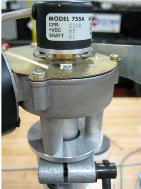
**Figure 3-14: Encoder attached to back of motor**
