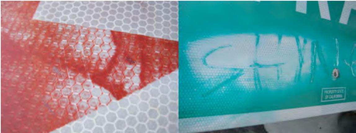
**Figure 1-6: Damage to graphics from abrasion and chemicals**
