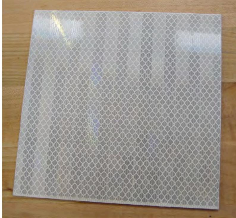
**Figure 3-2: Typical sign sample used in test**
