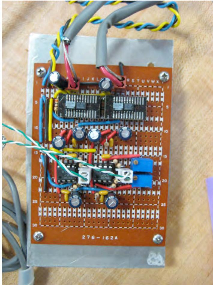
**Figure 3-15: Filtration and amplification circuit for instrumentation**
