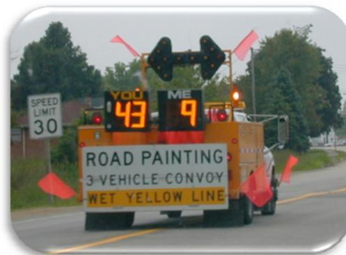
**Figure 13. Truck-Mounted DSDs Evaluated in Wisconsin.**
