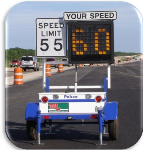
Speed display trailers are more effective at locations where the sign supports a clear and real need for a driver to reduce their speed or where the perception of regular enforcement exists. The effect of speed display trailers over time (especially if left at a location continuously and not enforced) is uncertain but believed to diminish as drivers become more accustomed to their presence in the work zone.
