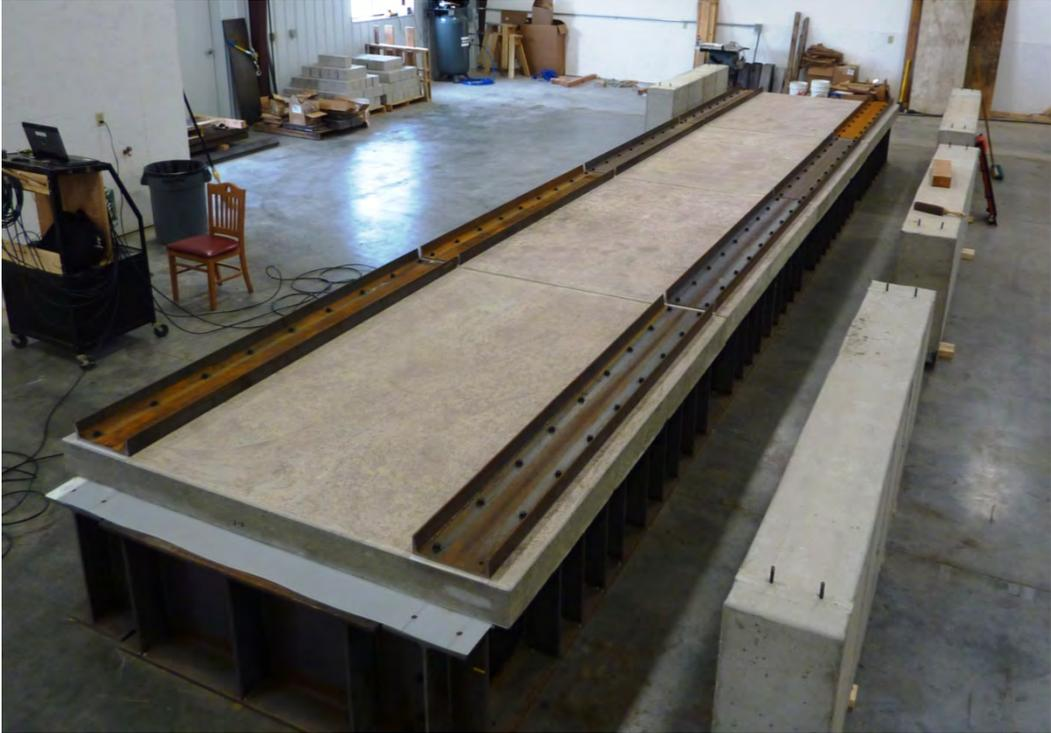
Figure 16: Test slabs mounted on reaction frame.
