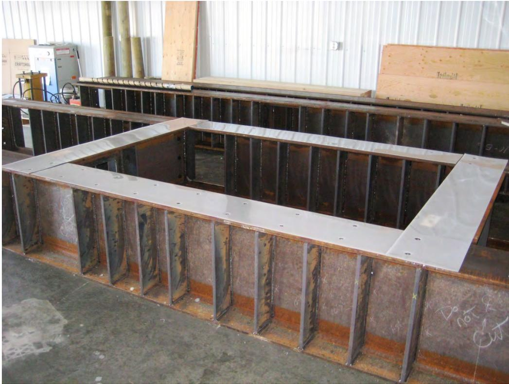
**Figure 18: Frame setup showing LDPE pads for single panel.**
