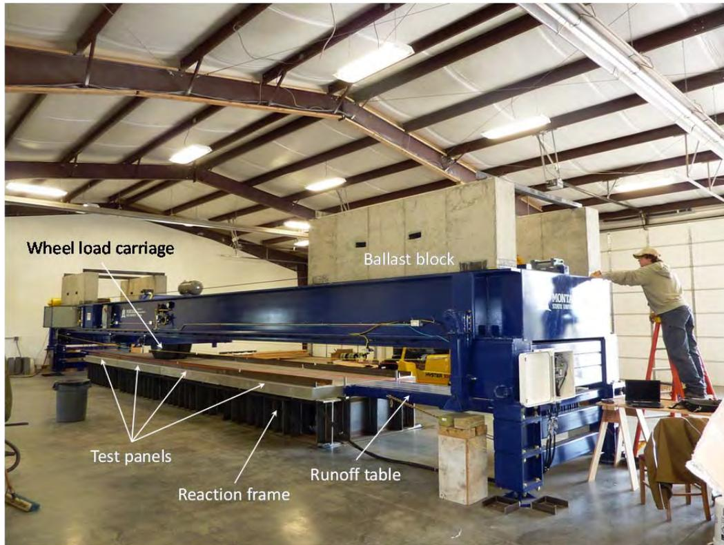
**Figure 14: Automated bridge deck tester.**
