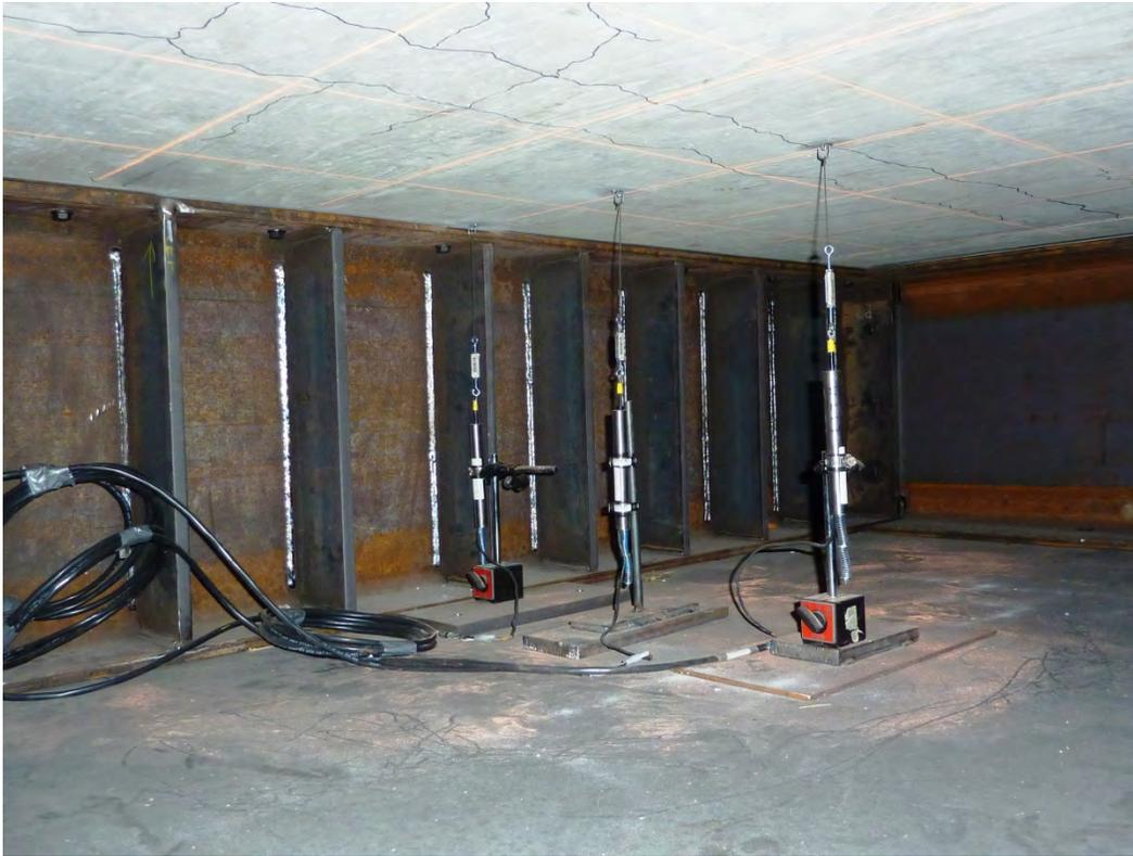
**Figure 25: Photo of LVDT sensors attached to underside of a test panel.**
