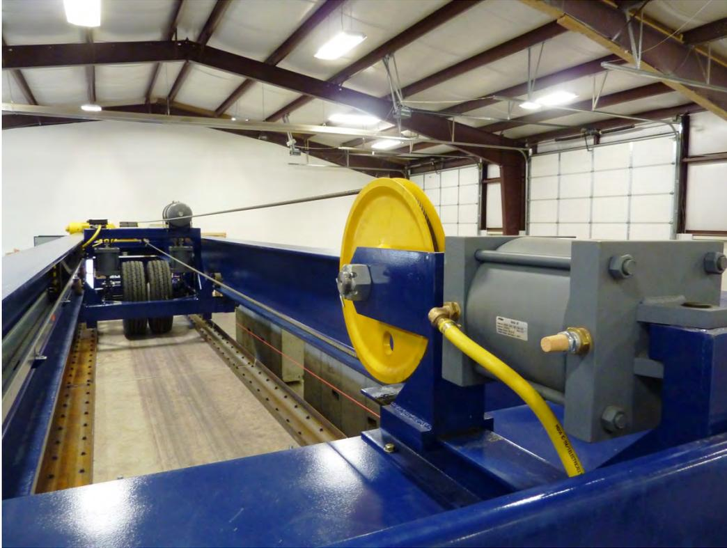
**Figure 23: Drive cable and carriage assembly.**
