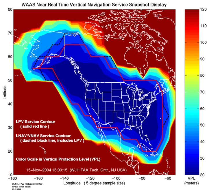
**Figure 2.1: WAAS GPS Vertical accuracy map**
