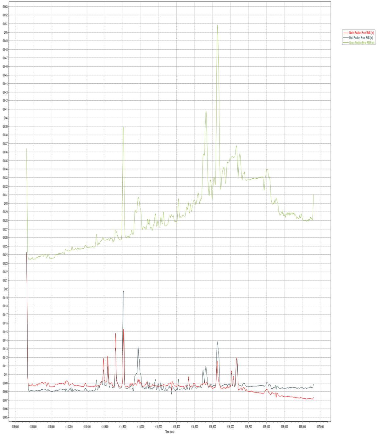
**Figure 4.5: Estimated position errors (X, Y, and Z) vs. time of the vehicle trajectory determined from GNSS/IMU post-processing with CORS P636 base station using POSPac software. The green line represents the estimated vertical error (< 0.06 meters). The red and black lines represent the estimated horizontal (X and Y) errors (< 0.025 meter).**
