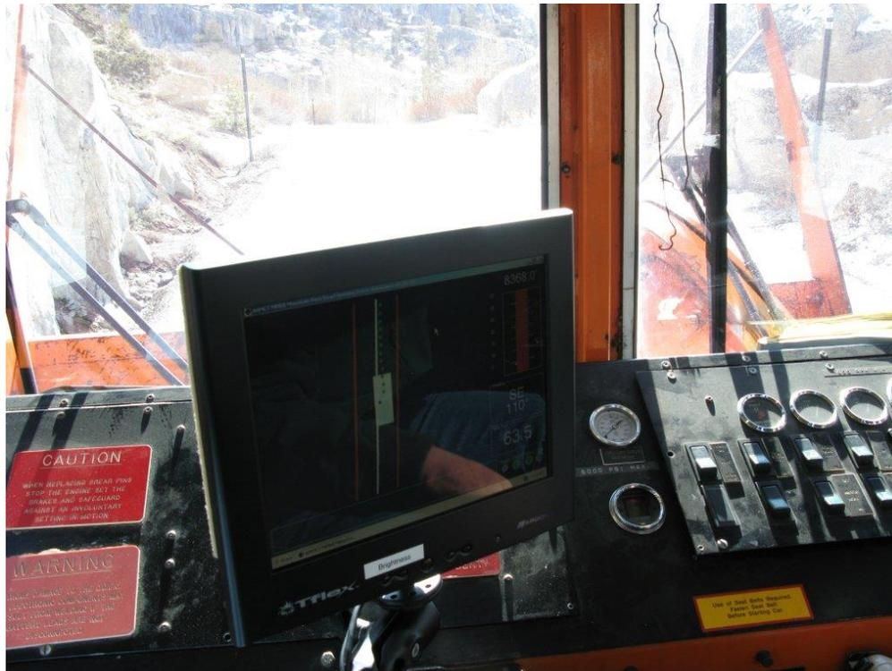
Figure 3.6: System installation showing LCD screen location
