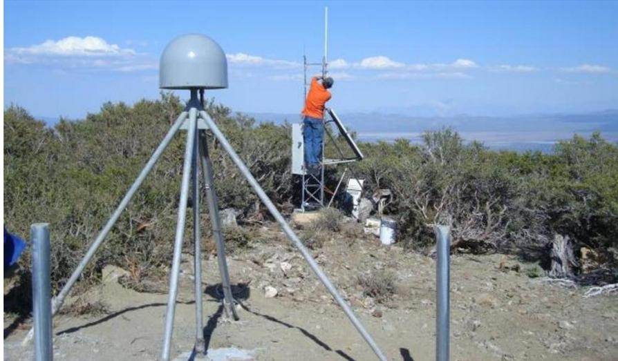
**Figure 4.3: CORS station P636 setup (Image from <http://www.ngs.noaa.gov/cgi-cors/corsage.prl?site=P636>)**
