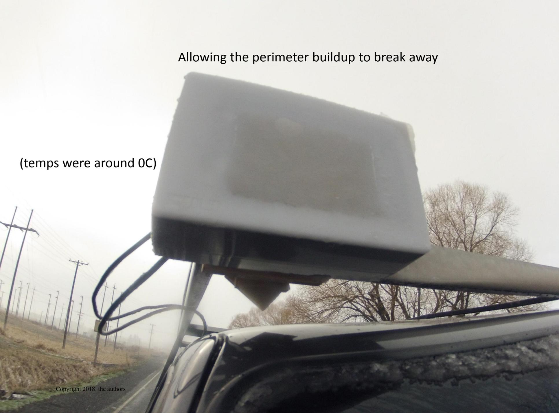
As the internal housing temp builds, the interface liquifies and the snow patch begins to descend
