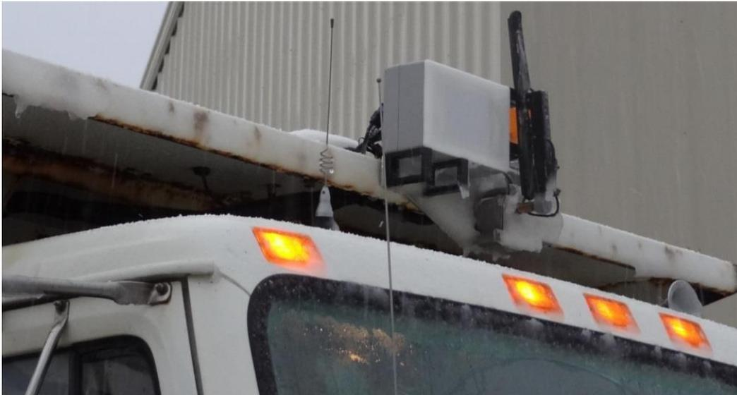
**Figure 4.14: Final wiper design with heated wiper blade**
