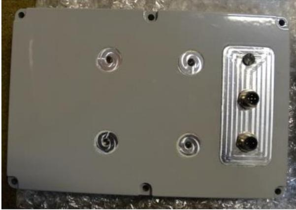
**Figure 4.1: Heated enclosure back**
