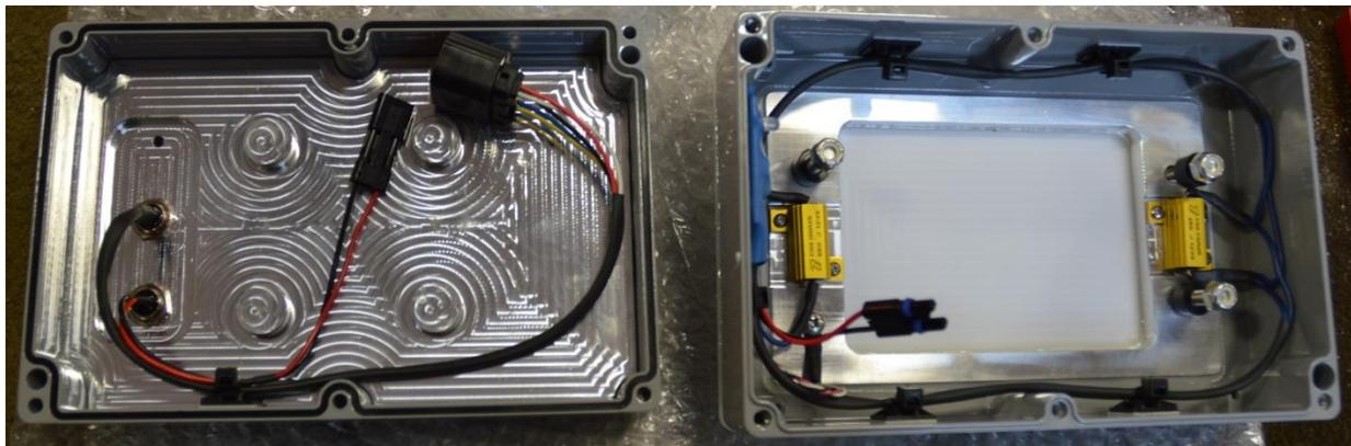
**Figure 4.3: Inside of the ESR heated enclosure**
