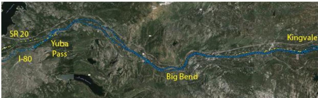
**Figure 5.6: GNSS RTK solution status on I-80 from SR 20 intersection to Kingvale overlaid on a Google hybrid map**
