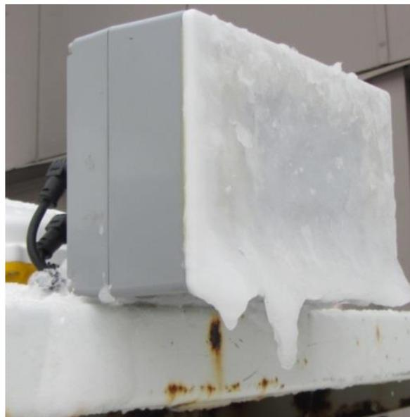
**Figure 4.5: Icing on the heated radar enclosure**
