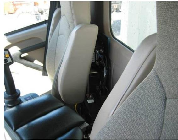
**Figure 1.2: UM DAS installed behind passenger seat**
