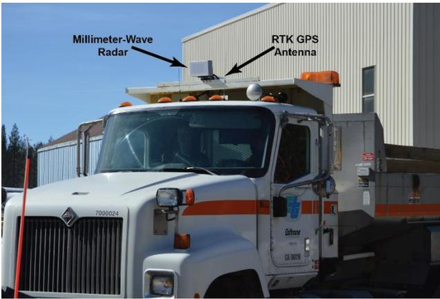
**Figure 1.1: University of Minnesota (UM) DAS exterior components**
