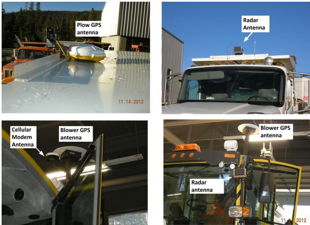
Figure B.1: System components mounted on the outside of the vehicles
