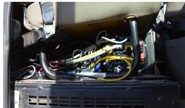
**Figure 2.7: DAS equipment installed under the passenger seat**
