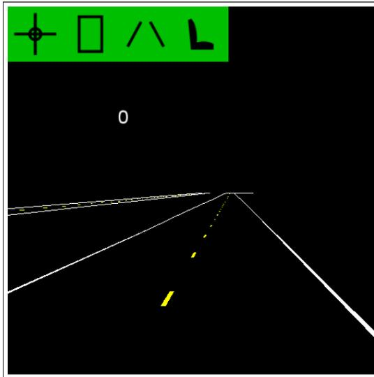
This image represents the typical computer generated view seen through the HUD. In this view the driver can see two lanes of traffic in their direction, separated by a yellow skip line and delineated by white fog lines. More traffic lanes can be seen across the median.
