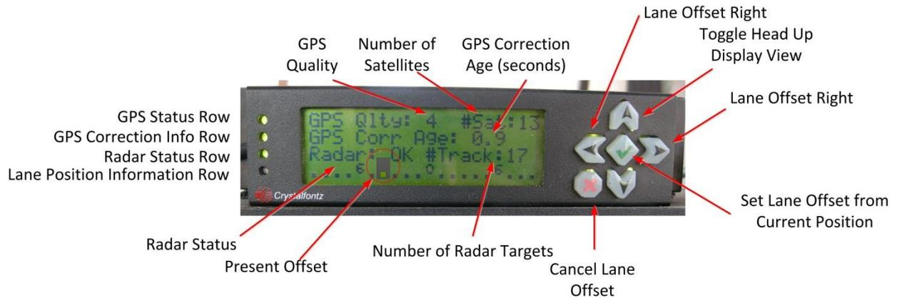
**Figure B.6: DAS LCD control panel. Display shows status, and the buttons allow the driver to change the desired location of the virtual lane boundary to facilitate the plowing of shoulders or clearing over the centerline.**
