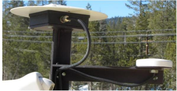
**Figure 2.9: GNSS antenna & modem antenna mounted on snow blower**
