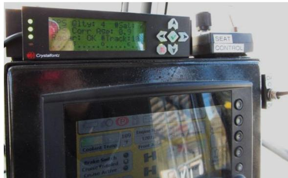
**Figure 2.13: DAS control interface in the snow blower**
