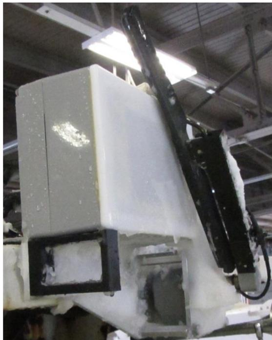
**Figure 4.13: Third-generation wiper design (wiper motor mounted on bottom) with heated wiper blade**
