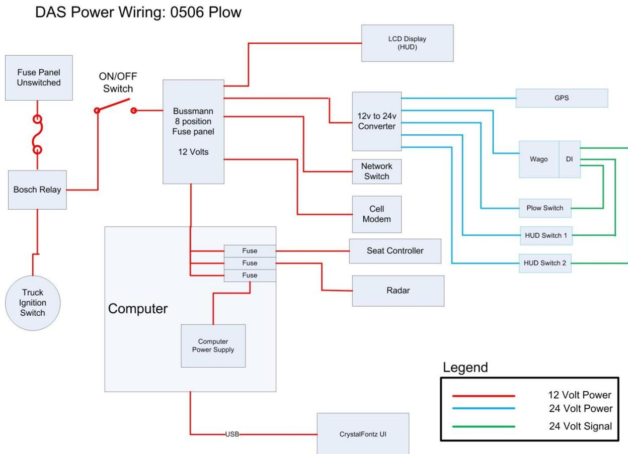
**Figure B.13: Power wiring diagram for plow 0530506. The plow switch is used by AHMCT to determine how often the DAS is used while plowing snow.**
