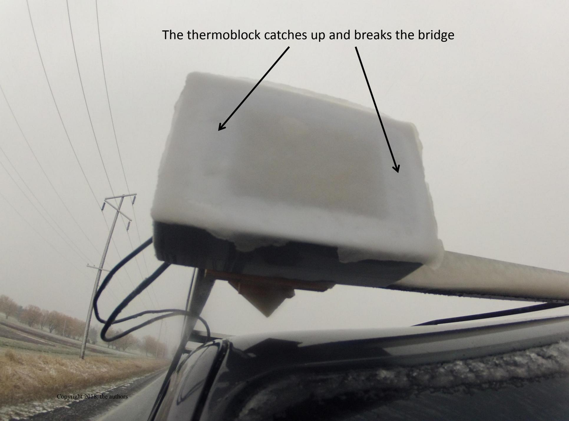
Allowing the perimeter buildup to break away
