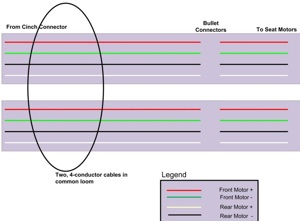
Figure B.11: Wiring between seat actuators and seat controller Cinch connector
