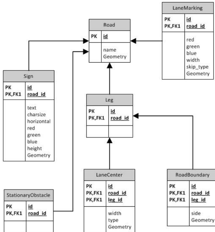
**Figure D.2: DAS Data Model with entity relationships and attributes. PK is primary key; FK1 is foreign key (a primary key from another entity). Together the primary key and the foreign keys uniquely identify the object with the database.**
