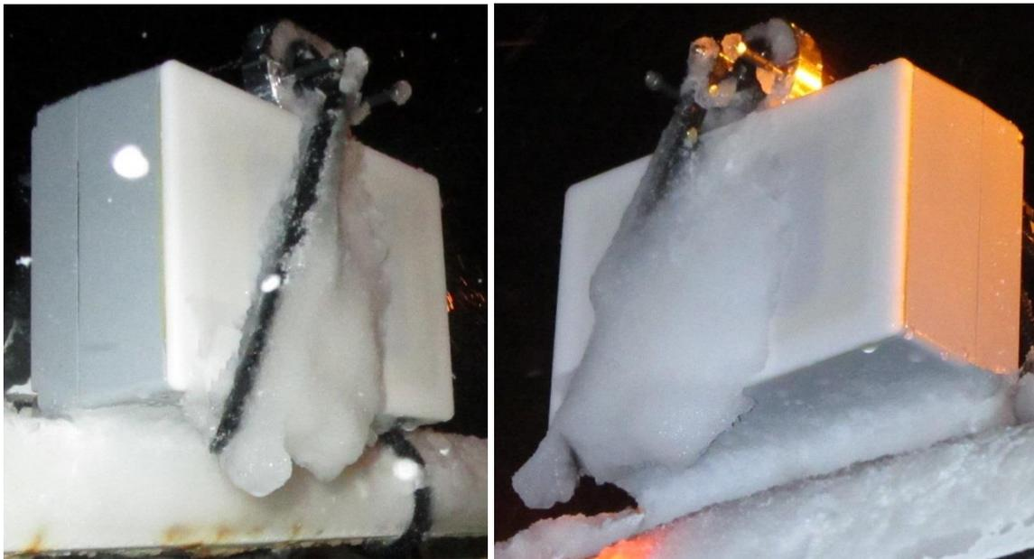
**Figure 4.10: First-generation wiper / heated enclosure system**
