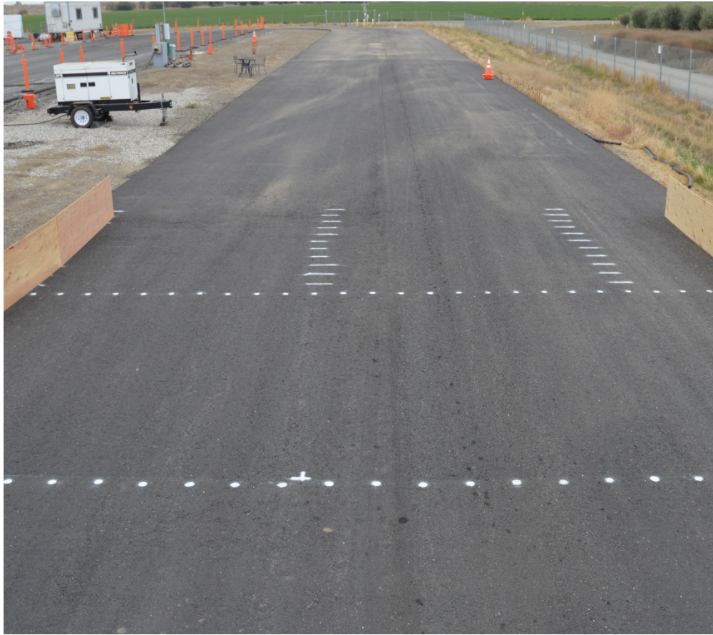
Figure 6.7: Sand Striping Observed on Test Track for Epoke Test #3
