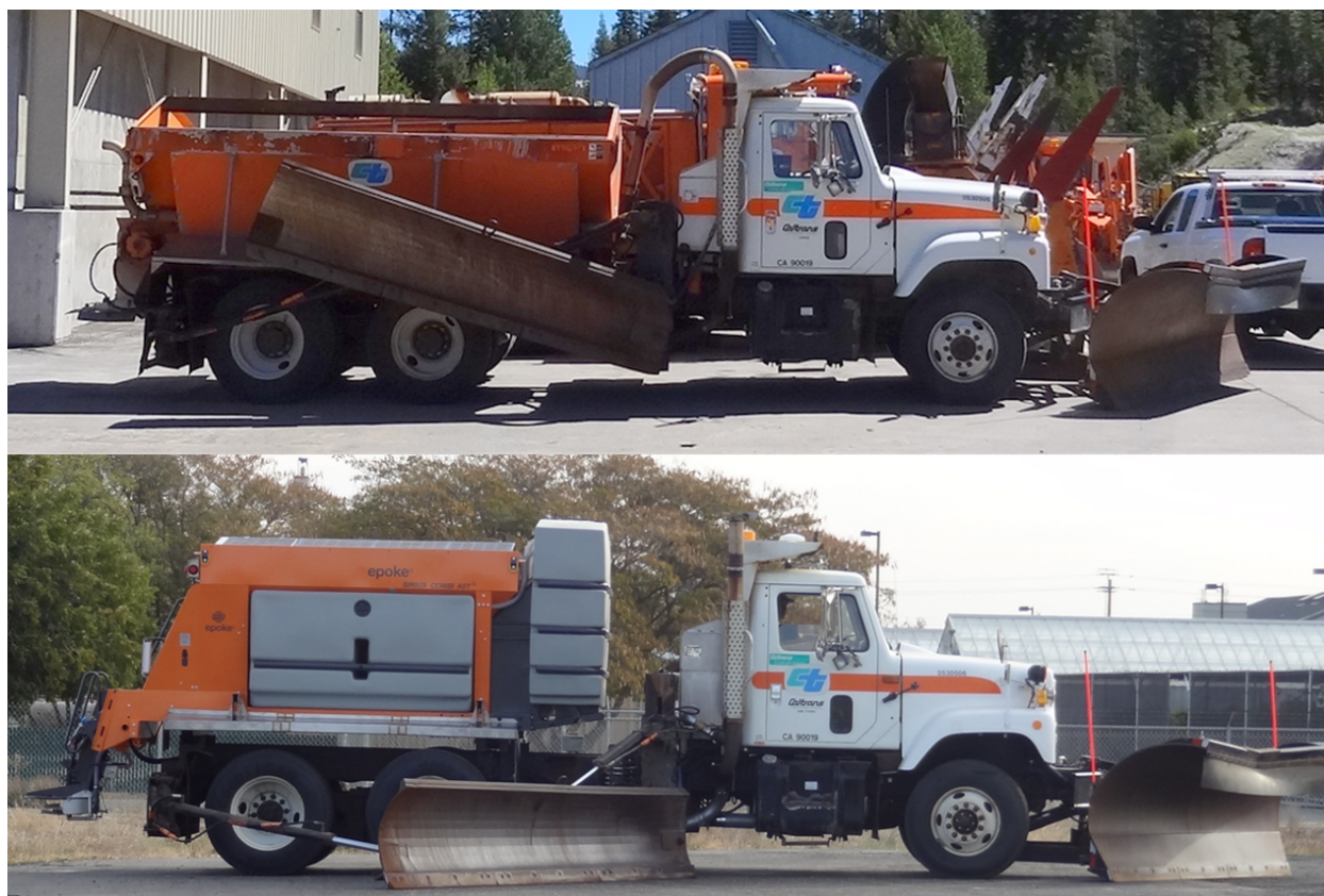
Figure 7.5: Profile of Kingvale Plow Truck with V-Box (above) and Epoke (below) Spreaders Installed
