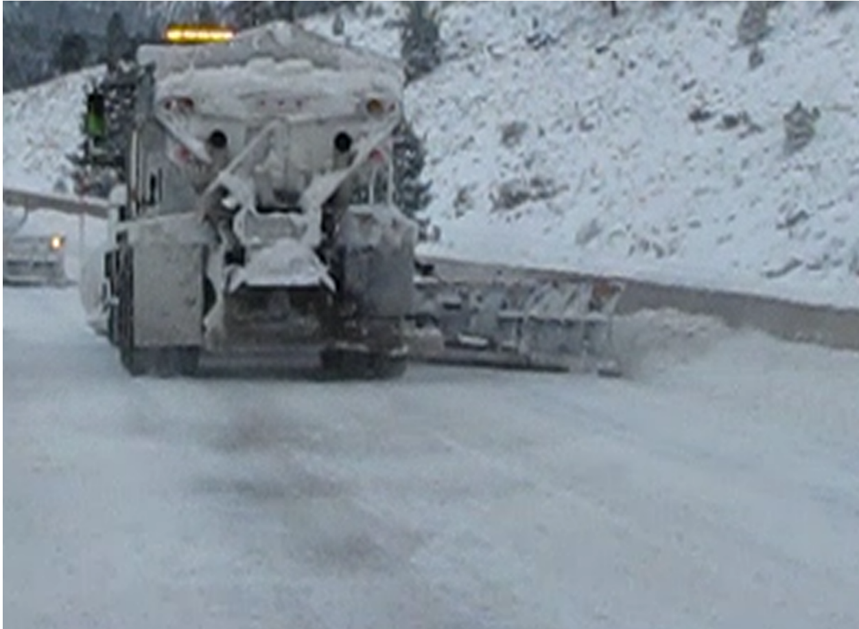
Figure 7.2: Irregular Placement of Sand Seen Behind V-Box
