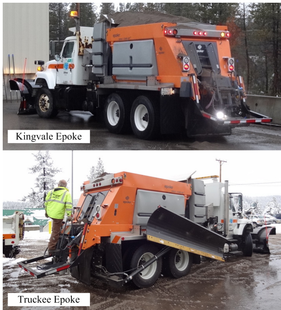
Figure 7.1: Caltrans Plow trucks Outfitted with Epoke Spreaders.
