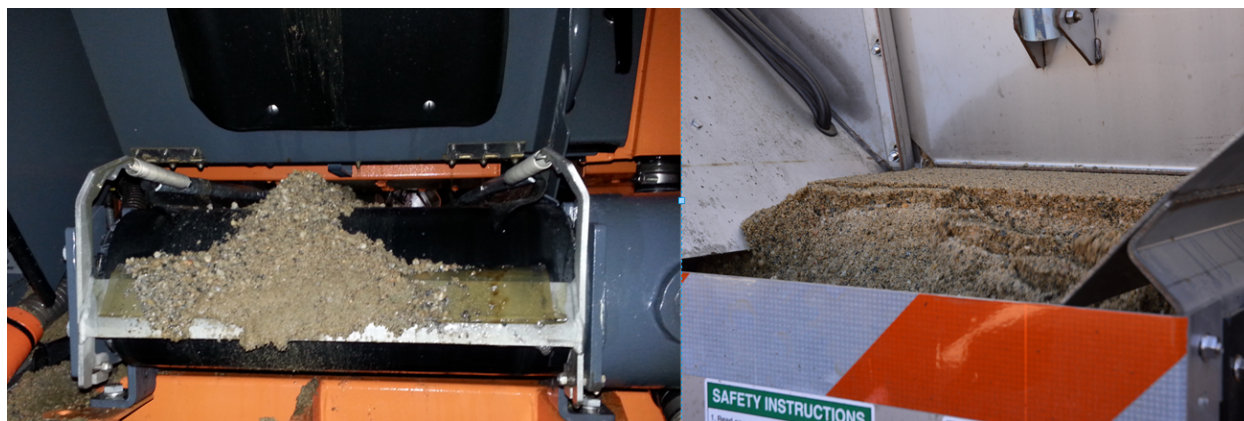
Figure 7.3: Comparing Load on Belt—Epoke (left), V-Box (right)
